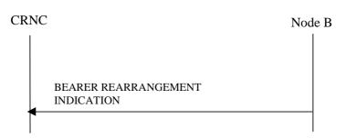
Figure 47C: Bearer Re-arrangement Indication, Successful Operation
