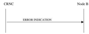
Figure 50: Error Indication procedure (CRNC to Node B), Successful Operation
