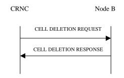
Figure 20: Cell Deletion procedure, Successful Operation
