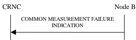
Figure 15: Common Measurement Failure procedure, Successful Operation
