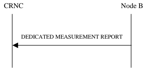
Figure 40: Dedicated Measurement Reporting procedure, Successful Operation
