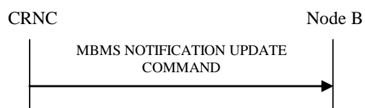
Figure 27Q: MBMS Notification Update procedure, Successful Operation
