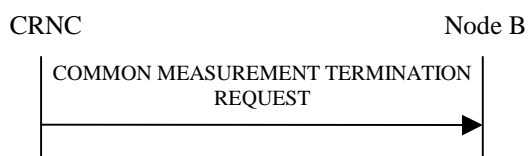
Figure 14: Common Measurement Termination procedure, Successful Operation
