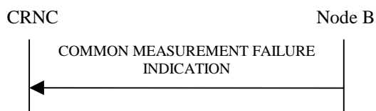
Figure 15: Common Measurement Failure procedure, Successful Operation
