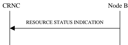
Figure 21: Resource Status Indication procedure, Successful Operation
