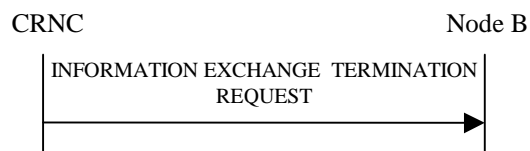
Figure 27O: Information Exchange Termination procedure, Successful Operation
