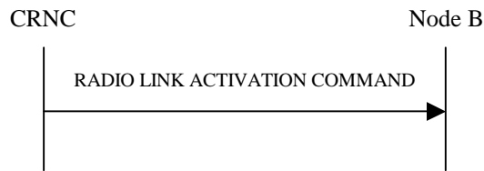
Figure 47D: Radio Link Activation procedure
