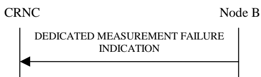
Figure 42: Dedicated Measurement Failure procedure, Successful Operation
