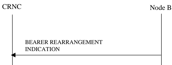
Figure 47C: Bearer Re-arrangement Indication, Successful Operation
