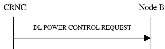
Figure 37: Downlink Power Control procedure, Successful Operation
