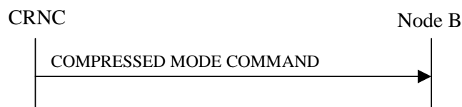
Figure 47: Compressed Mode Command procedure, Successful Operation
