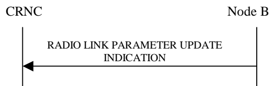
Figure 48: Radio Link Parameter Update Indication, Successful Operation
