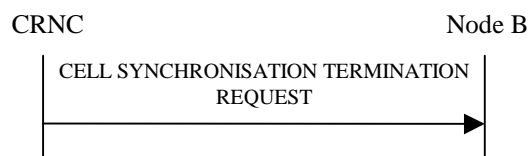
Figure 27H Cell Synchronisation Termination procedure, Successful Operation
