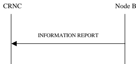
Figure 27N: Information Reporting procedure, Successful Operation
