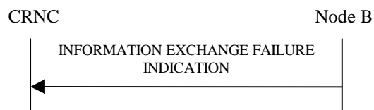
Figure 27P: Information Exchange Failure procedure, Successful Operation
