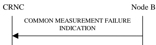
Figure 15: Common Measurement Failure procedure, Successful Operation
