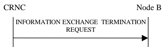
Figure 27O: Information Exchange Termination procedure, Successful Operation
