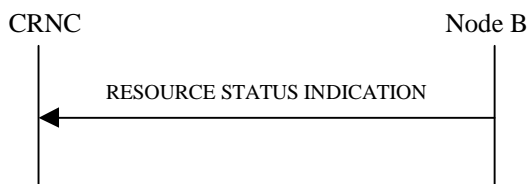
Figure 21: Resource Status Indication procedure, Successful Operation
