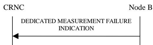
Figure 42: Dedicated Measurement Failure procedure, Successful Operation
