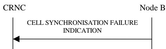
Figure 27I Cell Synchronisation Failure procedure, Successful Operation
