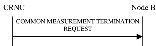
Figure 14: Common Measurement Termination procedure, Successful Operation
