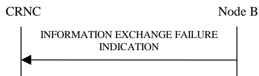
Figure 27P: Information Exchange Failure procedure, Successful Operation
