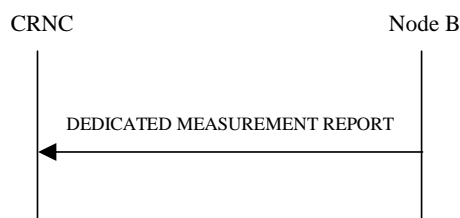
Figure 40: Dedicated Measurement Reporting procedure, Successful Operation
