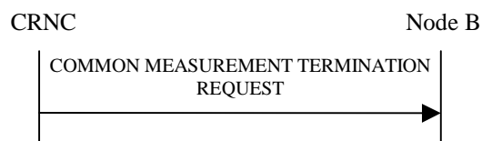
Figure 14: Common Measurement Termination procedure, Successful Operation
