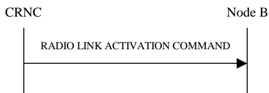
Figure 47D: Radio Link Activation procedure
