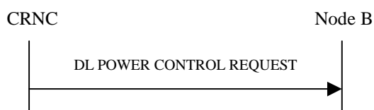
Figure 37: Downlink Power Control procedure, Successful Operation
