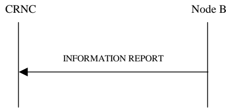
Figure 27N: Information Reporting procedure, Successful Operation
