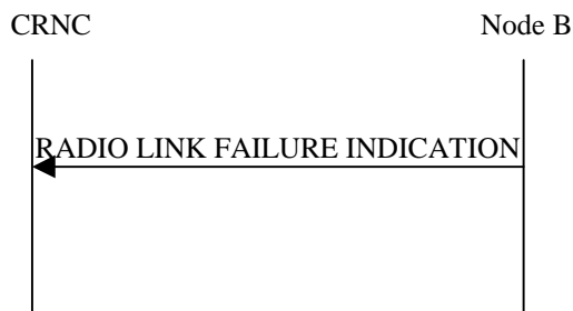
Figure 43: Radio Link Failure procedure, Successful Operation
