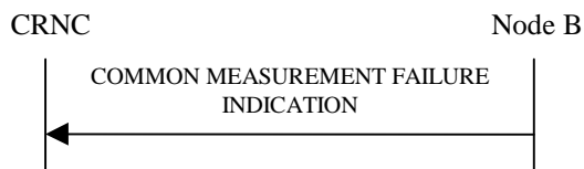
Figure 15: Common Measurement Failure procedure, Successful Operation
