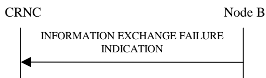
Figure 27P: Information Exchange Failure procedure, Successful Operation
