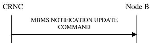
Figure 27Q: MBMS Notification Update procedure, Successful Operation
