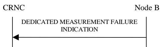
Figure 42: Dedicated Measurement Failure procedure, Successful Operation
