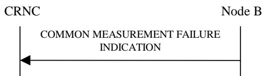
Figure 15: Common Measurement Failure procedure, Successful Operation
