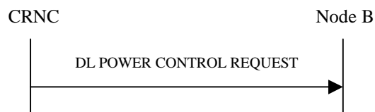
Figure 37: Downlink Power Control procedure, Successful Operation
