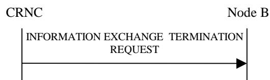
Figure 27O: Information Exchange Termination procedure, Successful Operation
