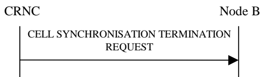
Figure 27H Cell Synchronisation Termination procedure, Successful Operation
