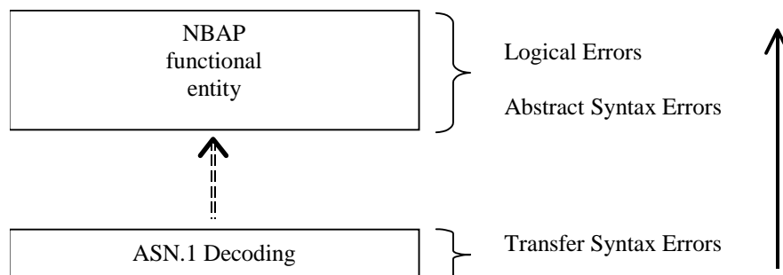
Figure 38: Protocol Errors in NBAP.
