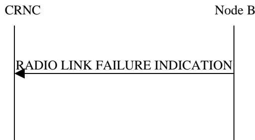
Figure 43: Radio Link Failure procedure, Successful Operation
