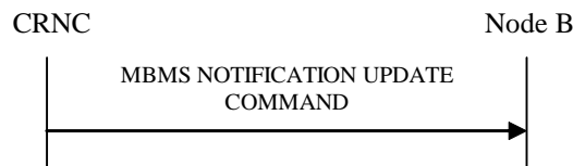
Figure 27Q: MBMS Notification Update procedure, Successful Operation
