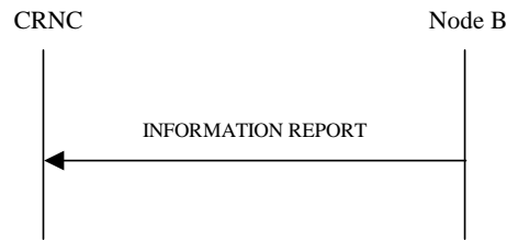
Figure 27N: Information Reporting procedure, Successful Operation
