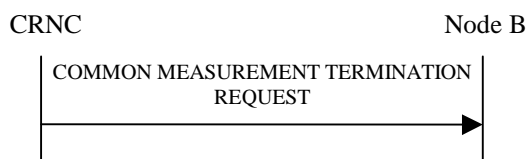
Figure 14: Common Measurement Termination procedure, Successful Operation
