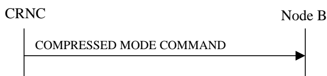
Figure 47: Compressed Mode Command procedure, Successful Operation
