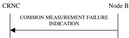
Figure 15: Common Measurement Failure procedure, Successful Operation
