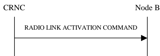
Figure 47D: Radio Link Activation procedure
