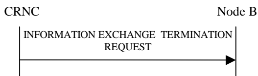
Figure 27O: Information Exchange Termination procedure, Successful Operation
