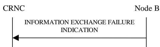
Figure 27P: Information Exchange Failure procedure, Successful Operation
