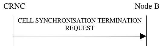
Figure 27H Cell Synchronisation Termination procedure, Successful Operation
