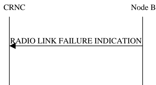
Figure 43: Radio Link Failure procedure, Successful Operation
