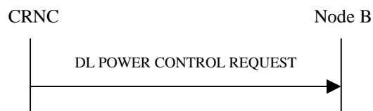
Figure 37: Downlink Power Control procedure, Successful Operation
