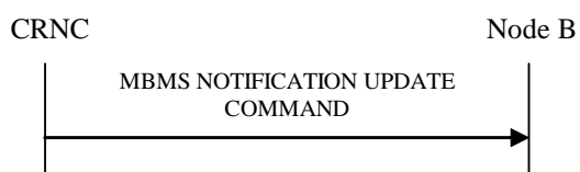
Figure 27Q: MBMS Notification Update procedure, Successful Operation
