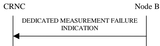
Figure 42: Dedicated Measurement Failure procedure, Successful Operation
