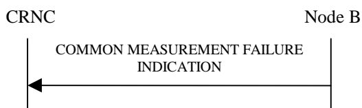
Figure 15: Common Measurement Failure procedure, Successful Operation
