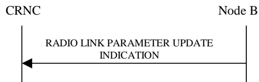
Figure 48: Radio Link Parameter Update Indication, Successful Operation
