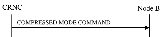
Figure 47: Compressed Mode Command procedure, Successful Operation
