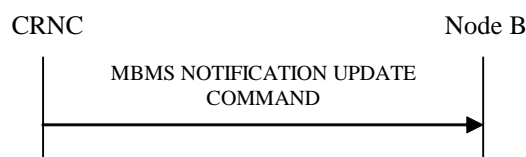
Figure 27Q: MBMS Notification Update procedure, Successful Operation
