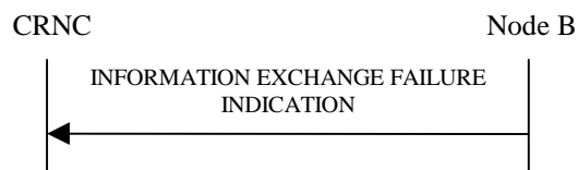
Figure 27P: Information Exchange Failure procedure, Successful Operation
