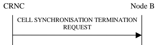
Figure 27H Cell Synchronisation Termination procedure, Successful Operation
