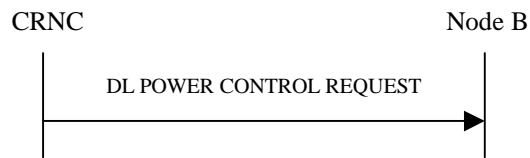
Figure 37: Downlink Power Control procedure, Successful Operation
