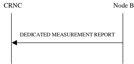
Figure 40: Dedicated Measurement Reporting procedure, Successful Operation
