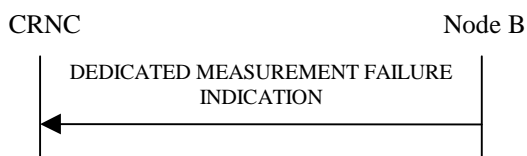
Figure 42: Dedicated Measurement Failure procedure, Successful Operation
