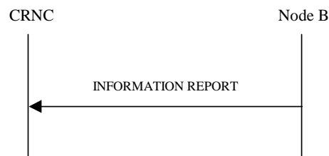
Figure 27N: Information Reporting procedure, Successful Operation
