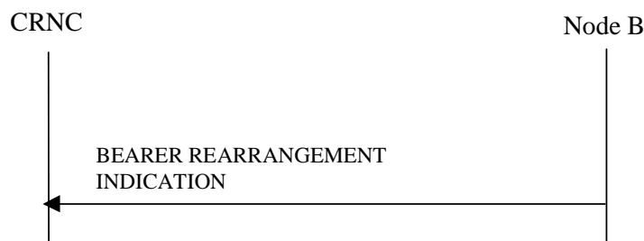
Figure 47C: Bearer Re-arrangement Indication, Successful Operation
