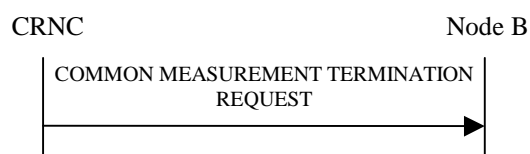
Figure 14: Common Measurement Termination procedure, Successful Operation
