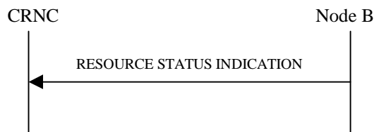
Figure 21: Resource Status Indication procedure, Successful Operation
