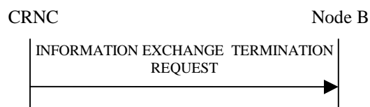
Figure 27O: Information Exchange Termination procedure, Successful Operation
