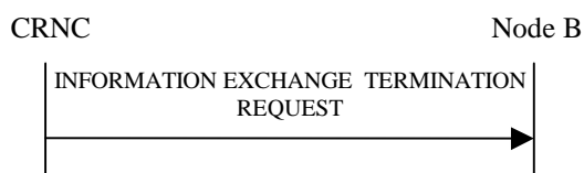
Figure 27O: Information Exchange Termination procedure, Successful Operation
