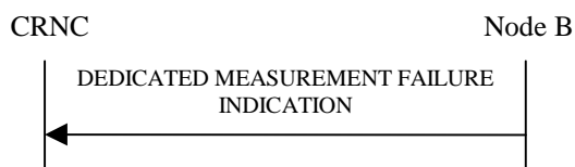
Figure 42: Dedicated Measurement Failure procedure, Successful Operation
