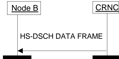
Figure 6A: HS-DSCH Data Transfer procedure
