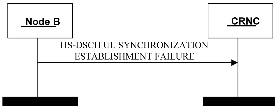
Figure 12D: HS-DSCH UL Synchronization Establishment Failure procedure
