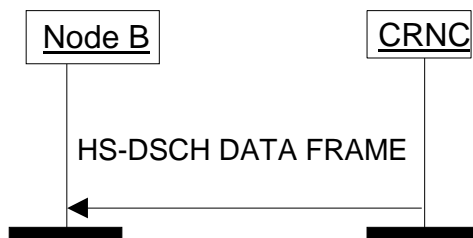
Figure 6A: HS-DSCH Data Transfer procedure
