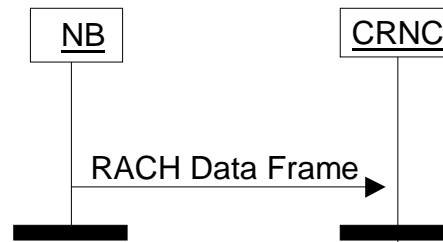
Figure 1: RACH Data Transfer Procedure
