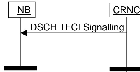
Figure 11: DSCH TFCI Signalling
