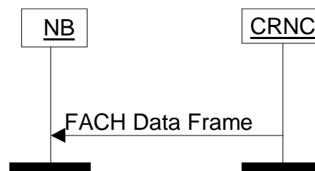
Figure 3: FACH Data Transfer Procedure
