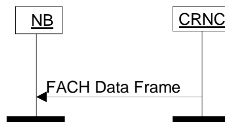
Figure 3: FACH Data Transfer Procedure
