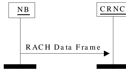
Figure 1: RACH Data Transfer Procedure
