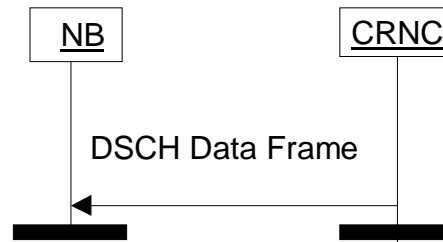
Figure 5: DSCH Data Transfer Procedure
