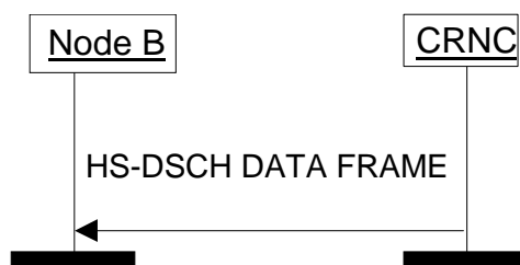
Figure 6A: DSCH Data Transfer procedure
