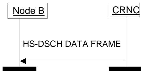
Figure 6A: HS-DSCH Data Transfer procedure
