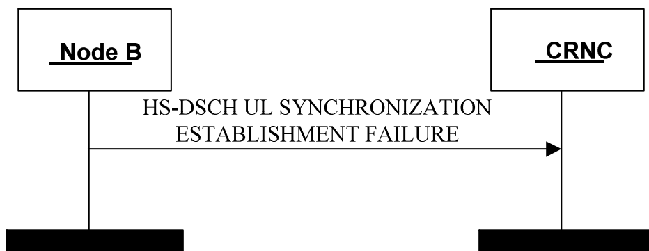
Figure 12D: HS-DSCH UL Synchronization Establishment Failure procedure
