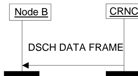
Figure 5: DSCH Data Transfer procedure
