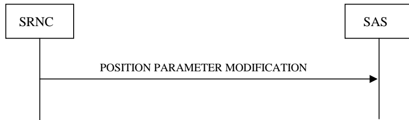
Figure 9e: Position Parameter Modification procedure, Successful Operation
