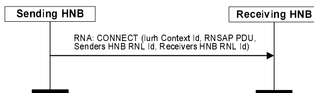
Figure 7.3.2.2.1-1: Signalling Connection Establishment – Direct Iurh-connectivity.
