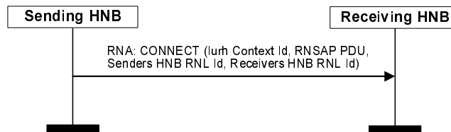
Figure 7.3.2.2.1-1: Signalling Connection Establishment – Direct Iurh-connectivity.
