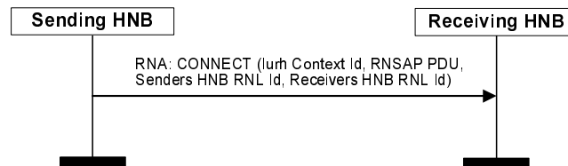
Figure 7.3.2.2.1-1: Signalling Connection Establishment – Direct Iurh-connectivity.
