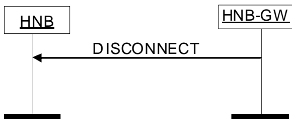
Figure 5: Disconnect to HNB
