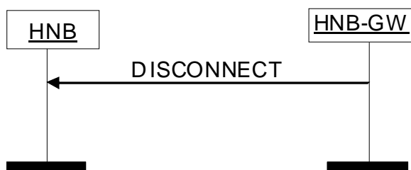
Figure 5: Disconnect to HNB
