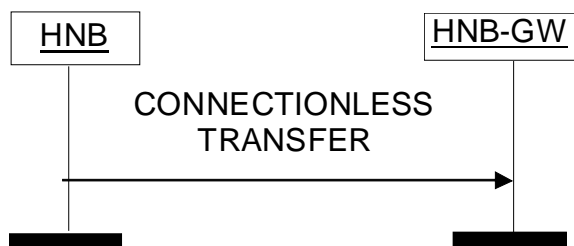
Figure 7: Connectionless Transfer to HNB-GW
