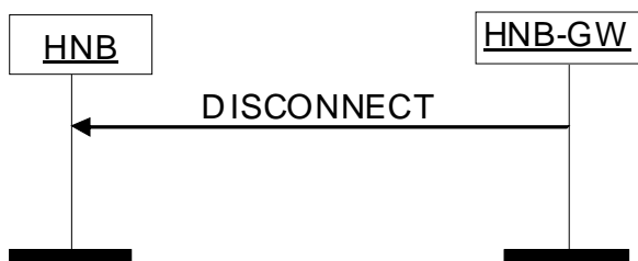
Figure 5: Disconnect to HNB
