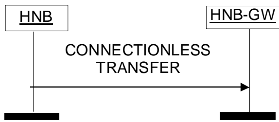
Figure 7: Connectionless Transfer to HNB-GW
