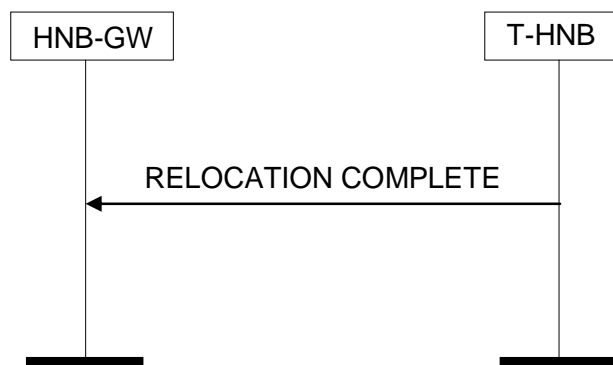
Figure 17: Relocation Complete procedure. Successful operation.
