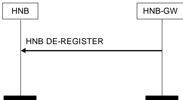
Figure 4: HNB De-register Procedure: Successful Operation
