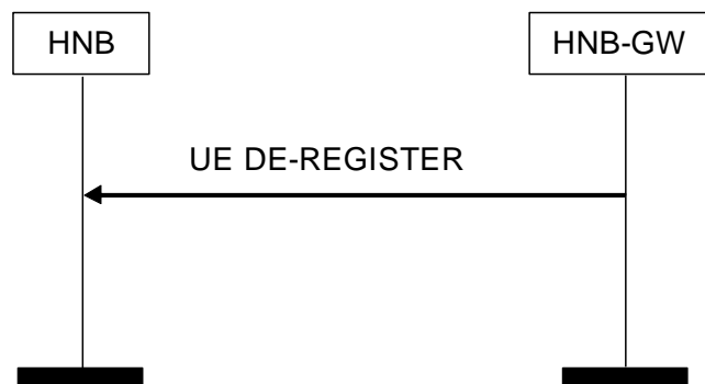
Figure 8 UE De-Register Procedure: HNB-GW Originated Successful Operation
