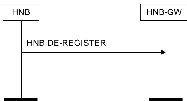
Figure 3: HNB De-register Procedure: Successful Operation
