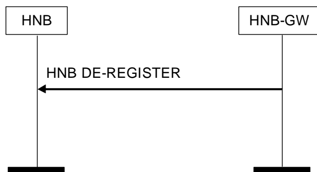
Figure 4: HNB De-register Procedure: Successful Operation
