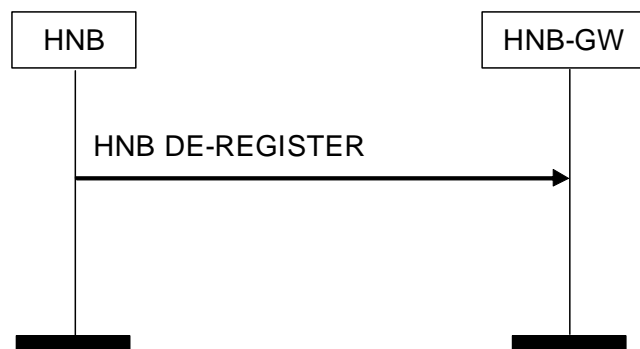
Figure 3: HNB De-register Procedure: Successful Operation
