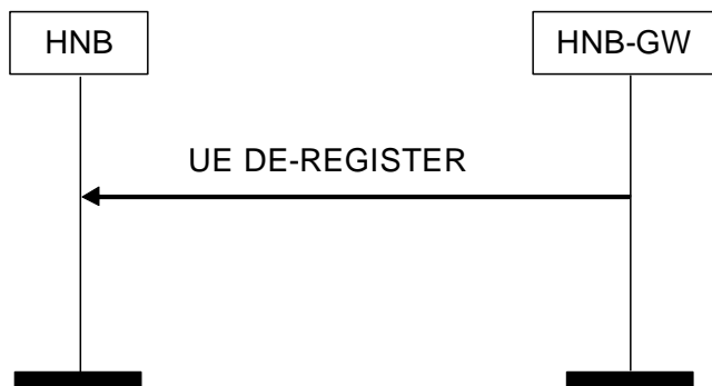
Figure 8 UE De-Register Procedure: HNB-GW Originated Successful Operation
