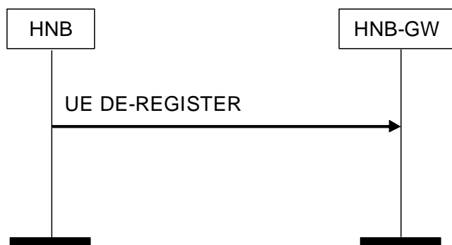
Figure 7 UE De-Register Procedure: HNB Originated Successful Operation
