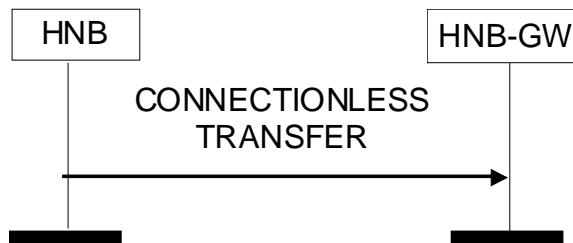
Figure 8.5.3-1: Connectionless Transfer procedure to HNB-GW
