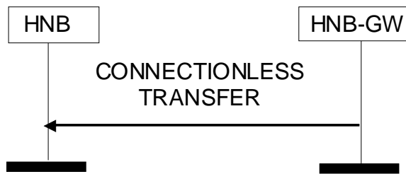
Figure 8.5.2-1: Connectionless Transfer procedure to HNB
