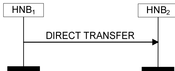
Figure 8.4.2.1-1. Direct Transfer procedure – HNB originated – direct Iurh connection.
