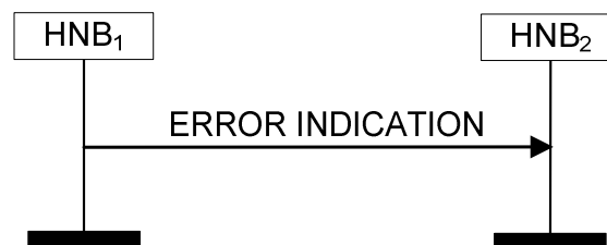
Figure 8.7.2-1. Error Indication procedure – HNB originated – direct Iurh connection.
