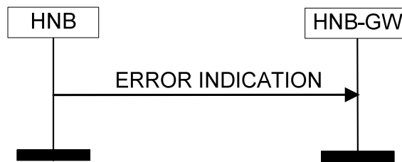
Figure 8.7.2-2. Error Indication procedure – HNB originated – lurch connection via the HNB-GW.
