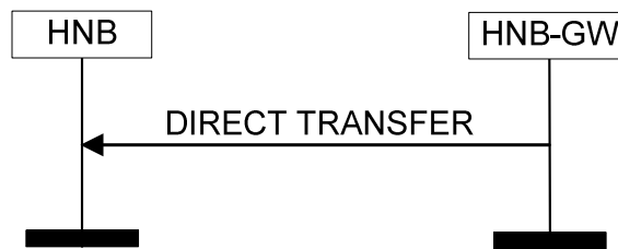
Figure 8.4.2.3-1. Direct Transfer procedure – HNB-GW originated – lurh connection via the HNB-GW
