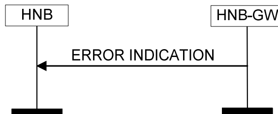
Figure 8.7.2-3. Error Indication procedure – HNB-GW originated – lurch connection via the HNB-GW
