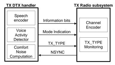
Figure 5: Block diagram of the transmit side DTX functions
