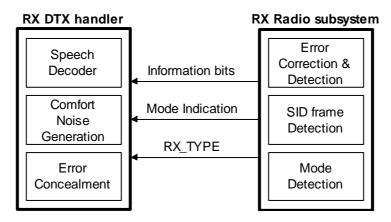
Figure 7: Block diagram of the receive side DTX functions
