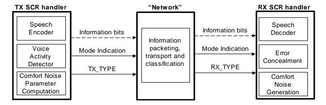
Figure 1: Block diagram of one link SCR operation
