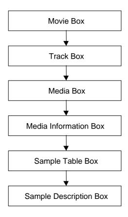
Figure 6.1: ISO File Format Box Structure Hierarchy
