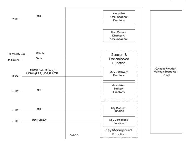
Figure 4: BM-SC sub-functional structure
