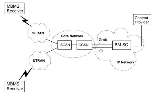
Figure 3: MBMS network architecture model for GPRS
