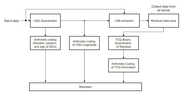
Figure 73: Block diagram for LSB TCQ for USQ encoding
