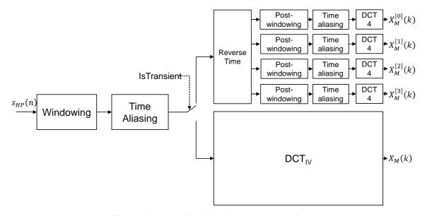
Figure 58: Adaptive time-frequency transform
