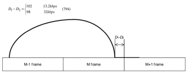
Figure 51: Windowing of the input high-pass filtered signal
