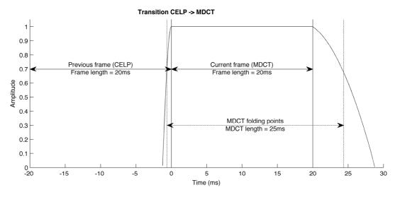
Figure 85: CELP to MDCT based TCX transition window (right part is here ALDO)
