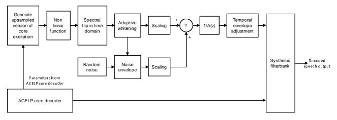
Figure 92: Time domain bandwidth extension decoder
