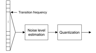
Figure 81: Noise level estimation done below the transition frequency
