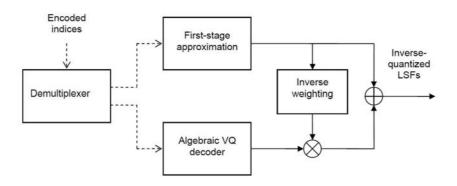
Figure 93: Overview high-rate LPC decoding
