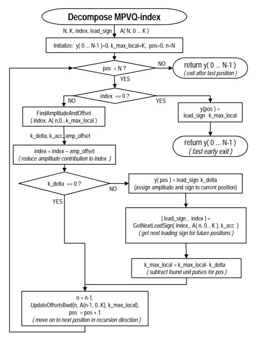
Figure 108: Detailed MPVQ-de-indexing
