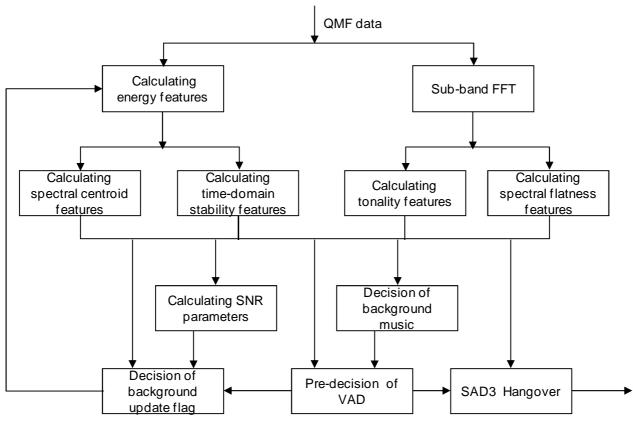
Figure 12: Block diagram of SAD3
