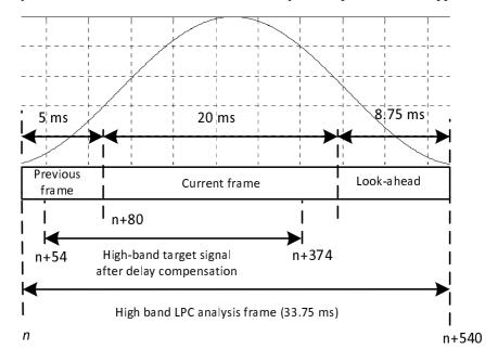
Figure 47: SWB Highband target signal buffers
