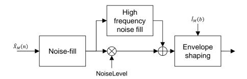
Figure 101: Spectrum filling block diagram
