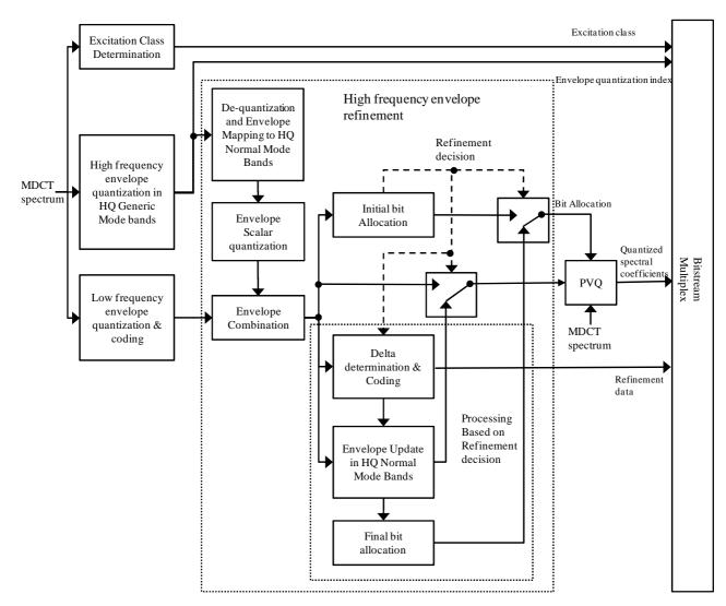
Figure 82: Generic mode Encoder Block Diagram
