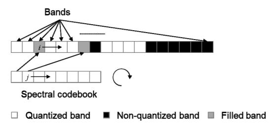
Figure 103: Noise filling from the spectral codebook up to the transition frequency
