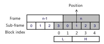
Figure 57: Transient information refinement for NB
