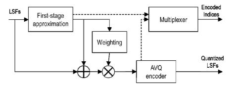
Figure 62: Principle of weighted algebraic LPC quantizer
