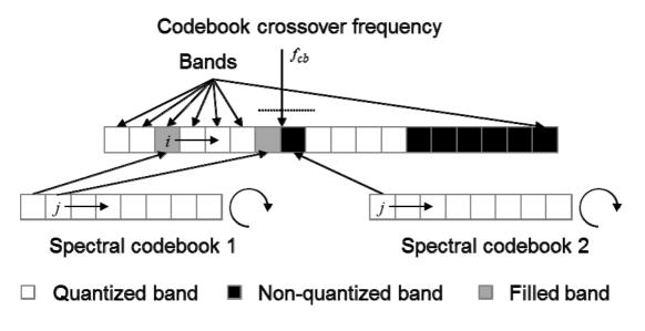
Figure 105: Creation of two parallel codebooks to handle sparse coded vectors.
