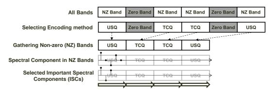
Joint USQ and TCQ Encoding + Lossless encoding (band by band)
