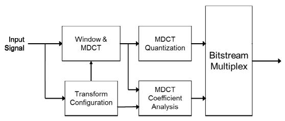
Figure 3: Frequency domain encoder
