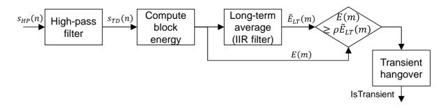
Figure 55: Transient detection algorithm
