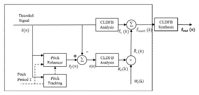
Figure 91: Block diagram of bass post-filter
