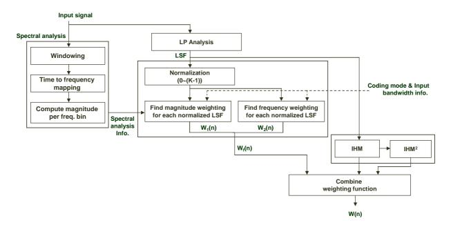
Figure 20: Block diagram of LSF weighting computation
