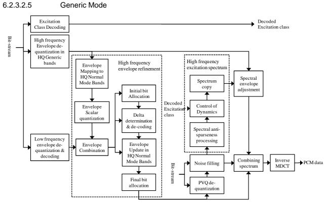
Figure 107: Generic mode Decoder Block Diagram
