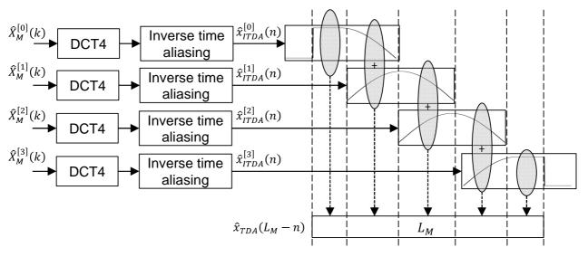
Figure 110: Algorithm for inverse transform in the case of transient mode.
