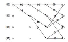
Figure 75: Trellis structure for the 4 states TCQ
