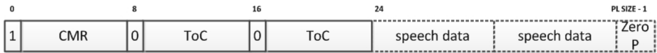
(d) Payload structure of Header-Full format with CMR + ToC multiple frames Figure A.3 Payload structure of Header-Full format
