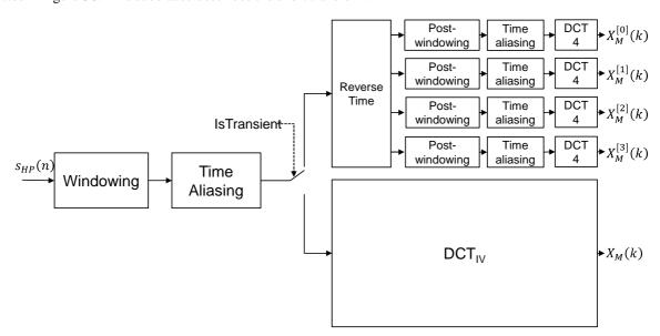
Figure 58: Adaptive time-frequency transform
