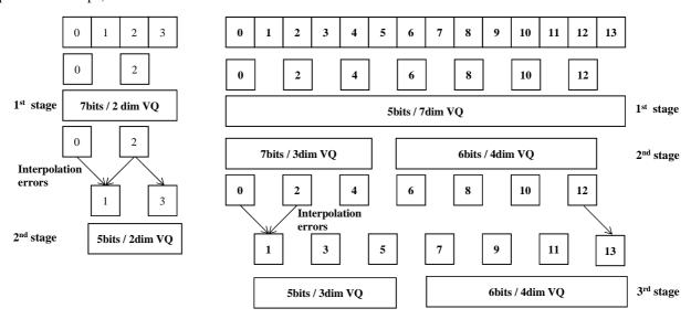
Figure 52: Envelope VQ in a TRANSIENT frame and a Non-TRANSIENT frame
