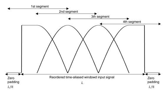
Figure 59: Higher time resolution, division into four segments
