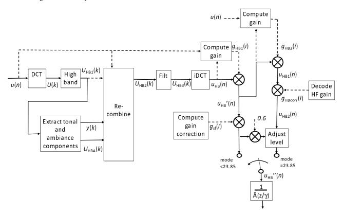
Figure 113: High-frequency band generation in AMR-WB IO modes
