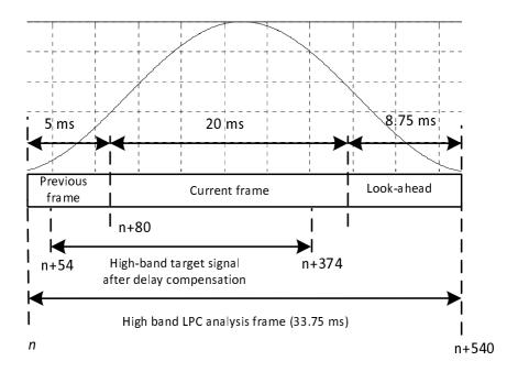
Figure 47: SWB Highband target signal buffers
