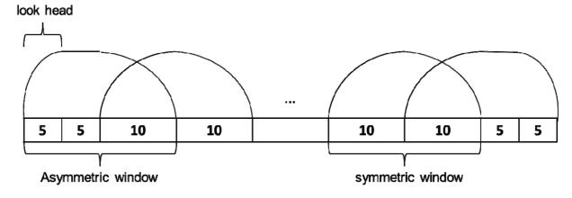
Figure 50: Asymmetric window and symmetric window
