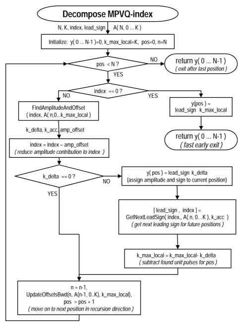
Figure 108: Detailed MPVQ-de-indexing
