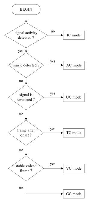
Figure 13: High-level diagram of the coding mode determination procedure
