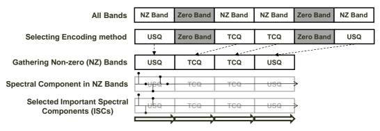
Joint USQ and TCQ Encoding + Lossless encoding (band by band)
