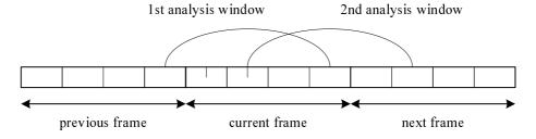
Figure 5: Relative positions of the spectral analysis windows
