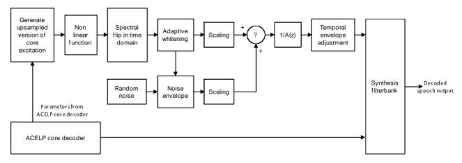
Figure 92: Time domain bandwidth extension decoder
