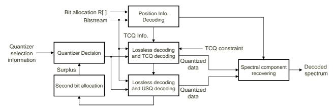
Figure 96: Block diagram of TCQ and USQ decoding with second bit allocation
