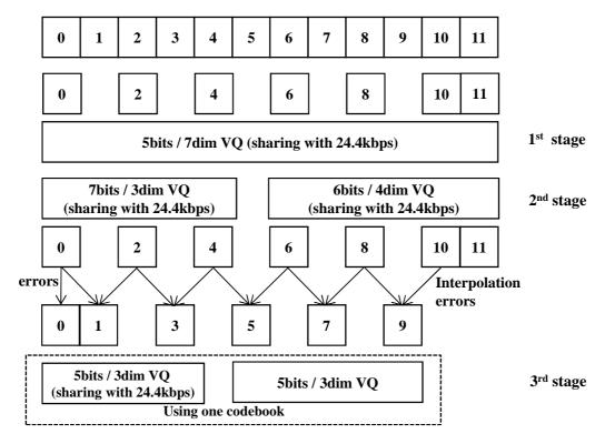
Figure 83: VQ for HQ generic mode at 32kbps
