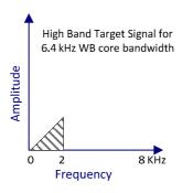
Figure 46: Generation of high band target signal for WB TBE
