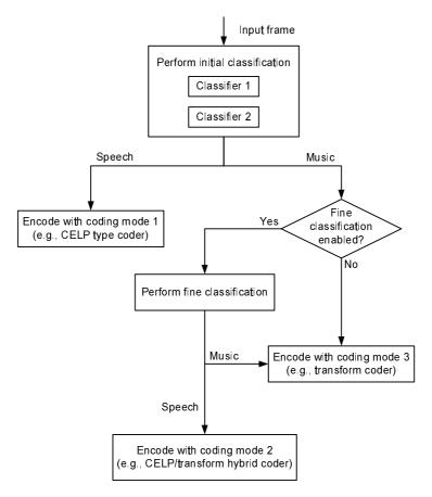
Figure 18: Multiple coding mode signal classification
