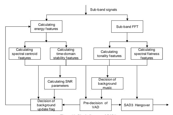
Figure 12: Block diagram of SAD3
