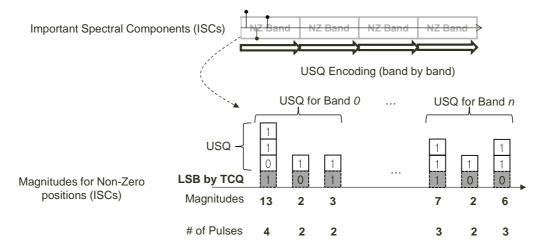
Figure 72: Concept of LSB coding
