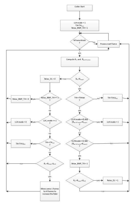
Figure 43: Average rate control in Variable Bit-Rate Coding
