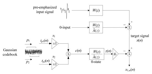
Figure 38: Schematic diagram of the excitation coding in UC mode
