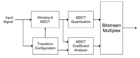
Figure 3: Frequency domain encoder
