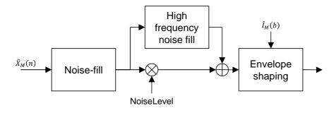
Figure 101: Spectrum filling block diagram
