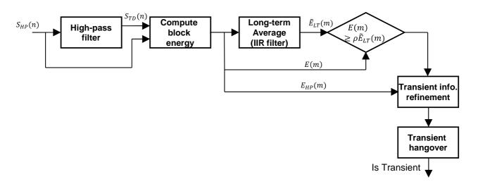
Figure 56: Transient detection algorithm for NB
