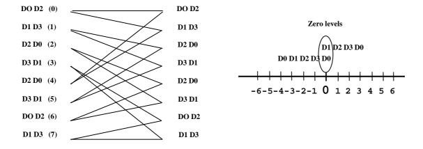
Figure 71: Trellis structure with 8 states 4-coset with 2 zero levels
