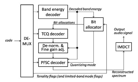
Figure 94: Block diagram of the Normal mode decoder overview
