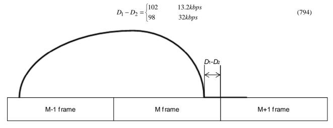
Figure 51: Windowing of the input high-pass filtered signal
