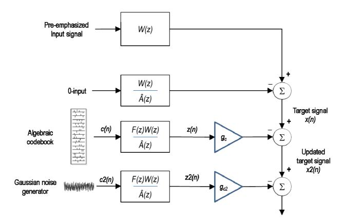
Figure 39: Schematic diagram of the excitation coding in UC and IC modes at 9.6 kbps
