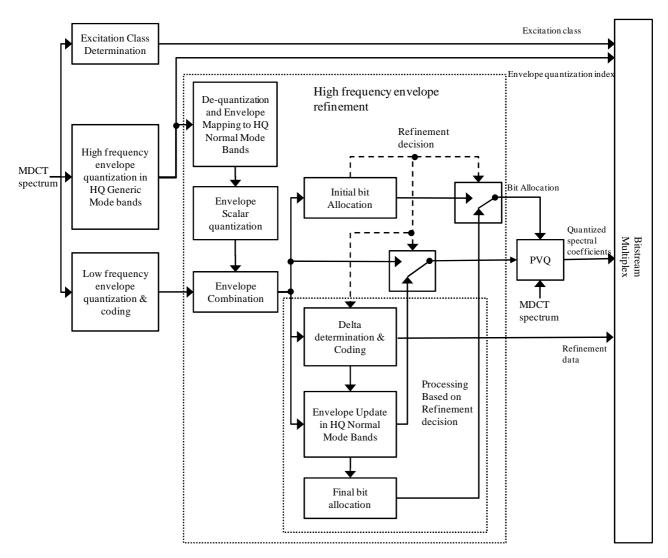
Figure 82: Generic mode Encoder Block Diagram
