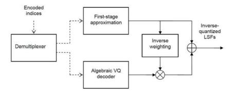
Figure 93: Overview high-rate LPC decoding
