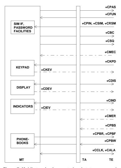
Figure 7: Mobile termination control and status commands
