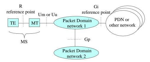
Figure 1: Packet Domain Access Interfaces and Reference Points
