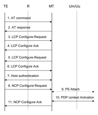
Figure 7a: IPv4 Over PPP Based Service
