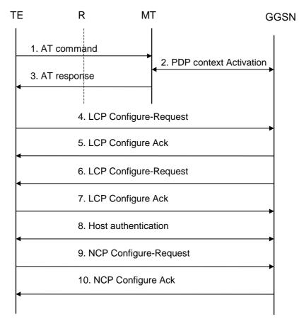
Figure 9a: PPP Based Service (transparent PPP negotiation)
