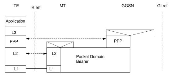
Figure 8a: PPP Based Services (transparent PPP negotiation)
