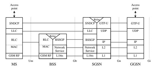
Figure 2: User Plane for Packet Domain services in GSM
