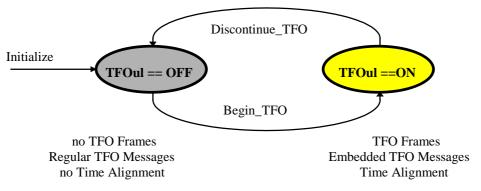
Figure D.3.3-1: States of the Tx\_TFO Process
