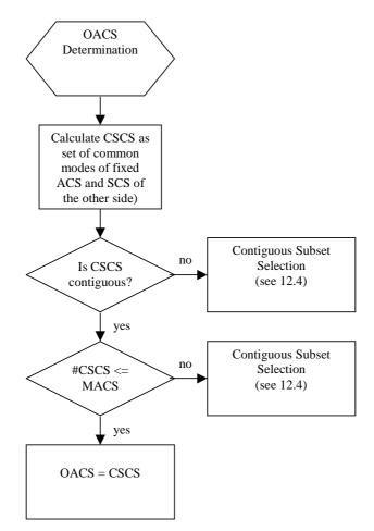
Figure 12.2.2-1: OACS Determination when only one side supports ACS Change
