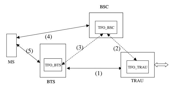
Figure C.2-1: Processes and Interfaces for TFO in GSM
