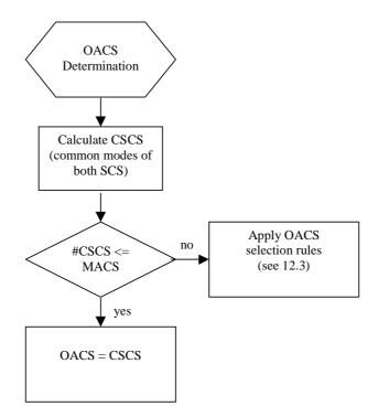
Figure 12.2.3-1: OACS Determination when both sides support ACS Change
