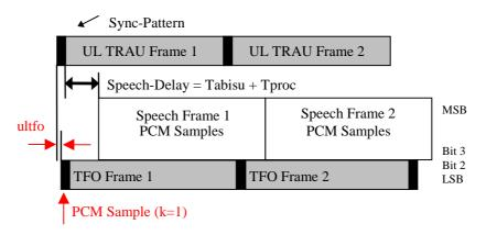
Figure 8.1.2-1: Uplink TFO Frame Time Alignment in GSM
