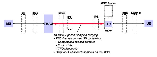
Figure 4.2.1-4: TFO Configuration between a GSM and a 3G Network
