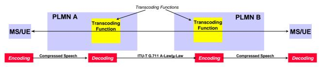
Figure 4.1-1: Typical Speech Codec Tandem Operation
