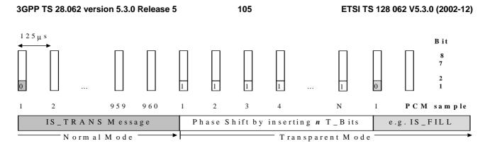
Figure A.4-1: Phase Shift of the 16\_PCM\_Sample\_Grid by inserting T\_Bits
