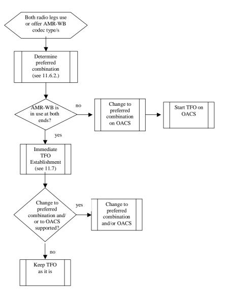
Figure 11.2.4-2: Flowchart for AMR-WB TFO Establishment at Call Set-Up
