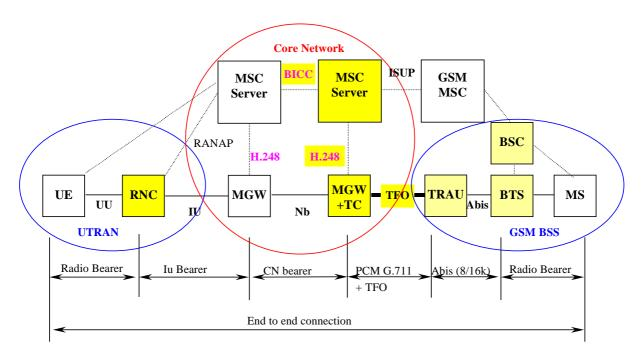
Figure D.2-1b: Nodes and Interfaces for TFO in UMTS-GSM Calls
