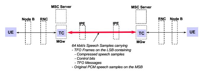
Figure 4.2.1-3: TFO Configuration between 3G Networks
