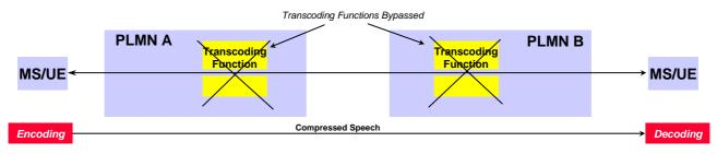
Figure 4.1-2: Tandem Free Operation of Speech Codec
