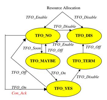
Figure C.4.1-1: Main TFO \_State Diagram within the BTS
