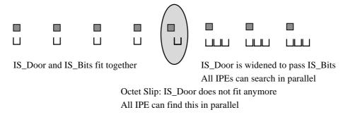
Figure B.3.3-1: Handling of octet slip for fast and parallel re-synchronization of all IPEs (optional)
