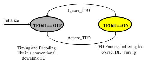
Figure D.3.2-1: States of the Tx\_IU Process
