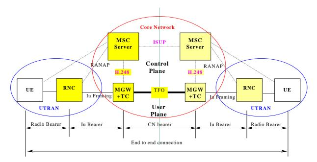
Figure D.2-1a: Nodes and Interfaces for TFO in UMTS-UMTS Calls
