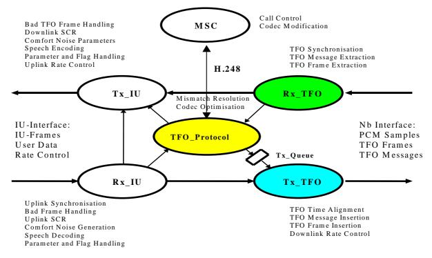
Figure D.3-1: The five TFO\_TC Processes and the TFO\_MSC Process
