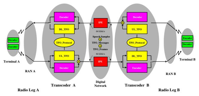
Figure 4.2.1-1: Functional Entities Handling Tandem Free Operation
