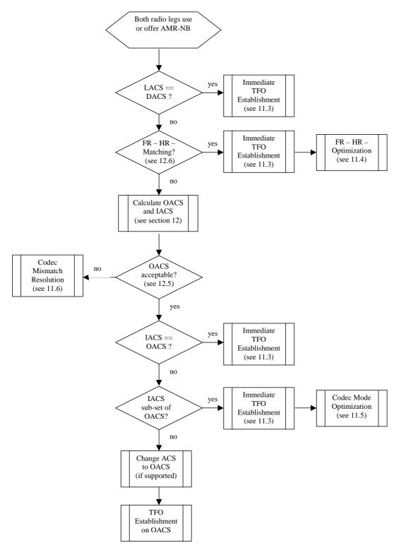
Figure 11.2.4-1: Flowchart for AMR-NB TFO Establishment at Call Set-Up
