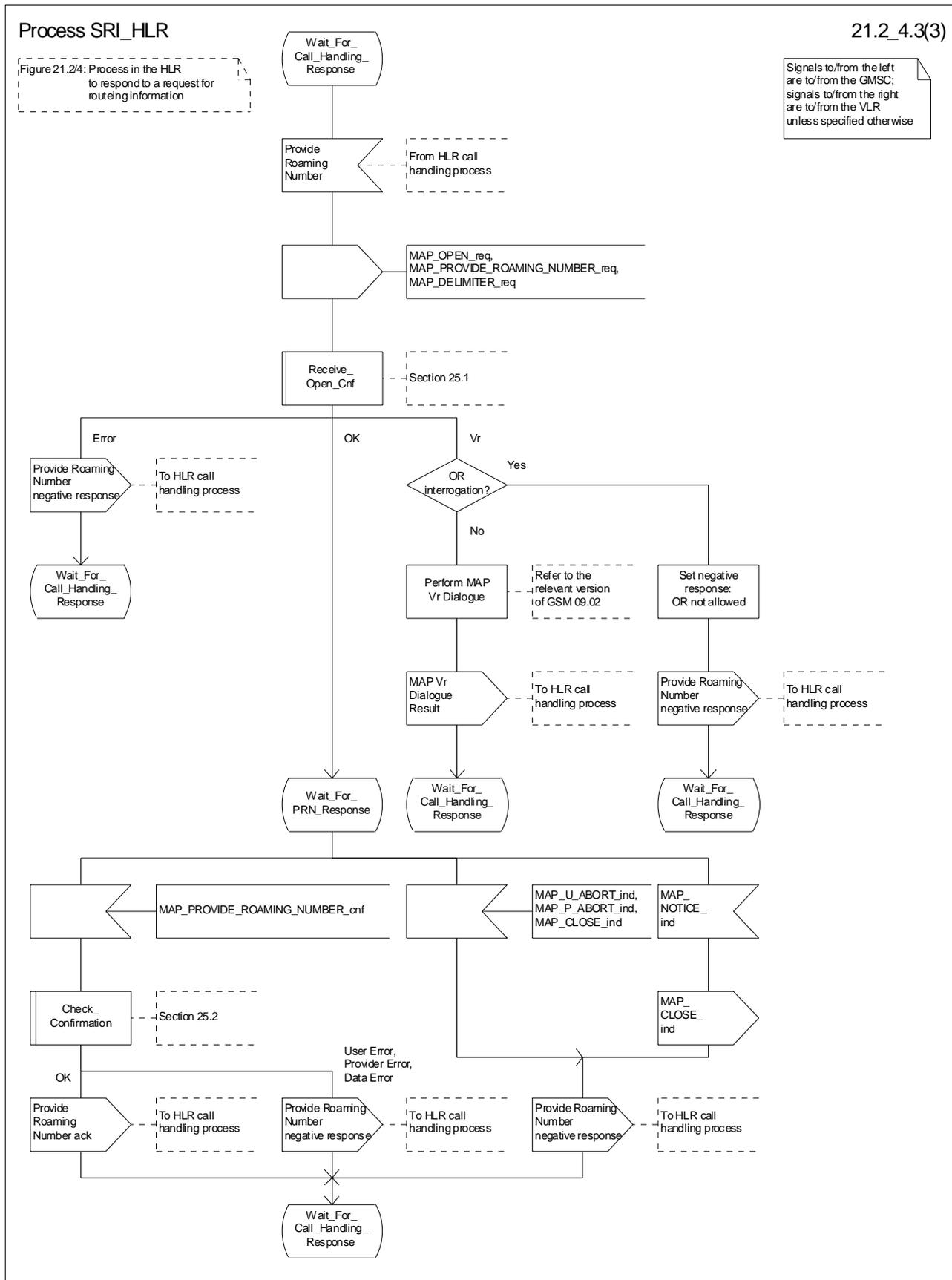
Figure 21.2/4 (sheet 3 of 3): Process SRI\_HLR
