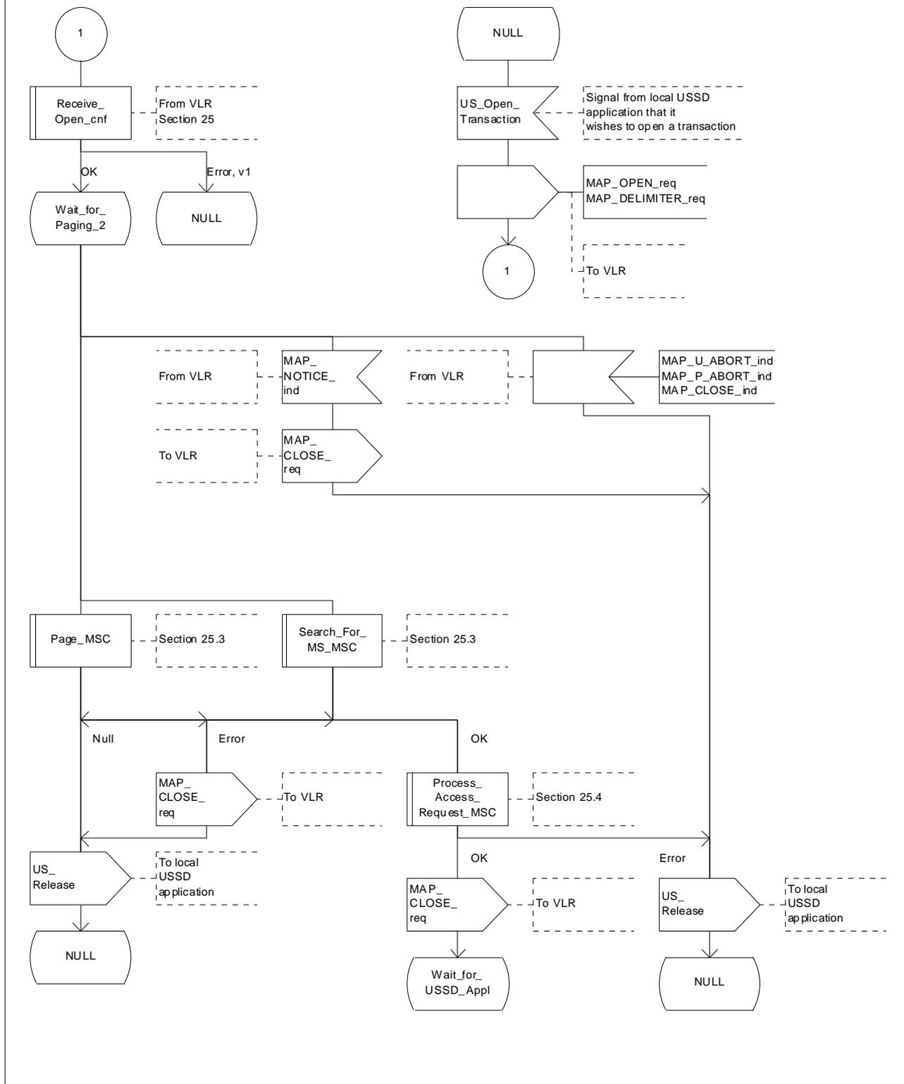
Figure 22.10.2/1 (sheet 3 of 4): Procedure NI\_USSD\_MSC
