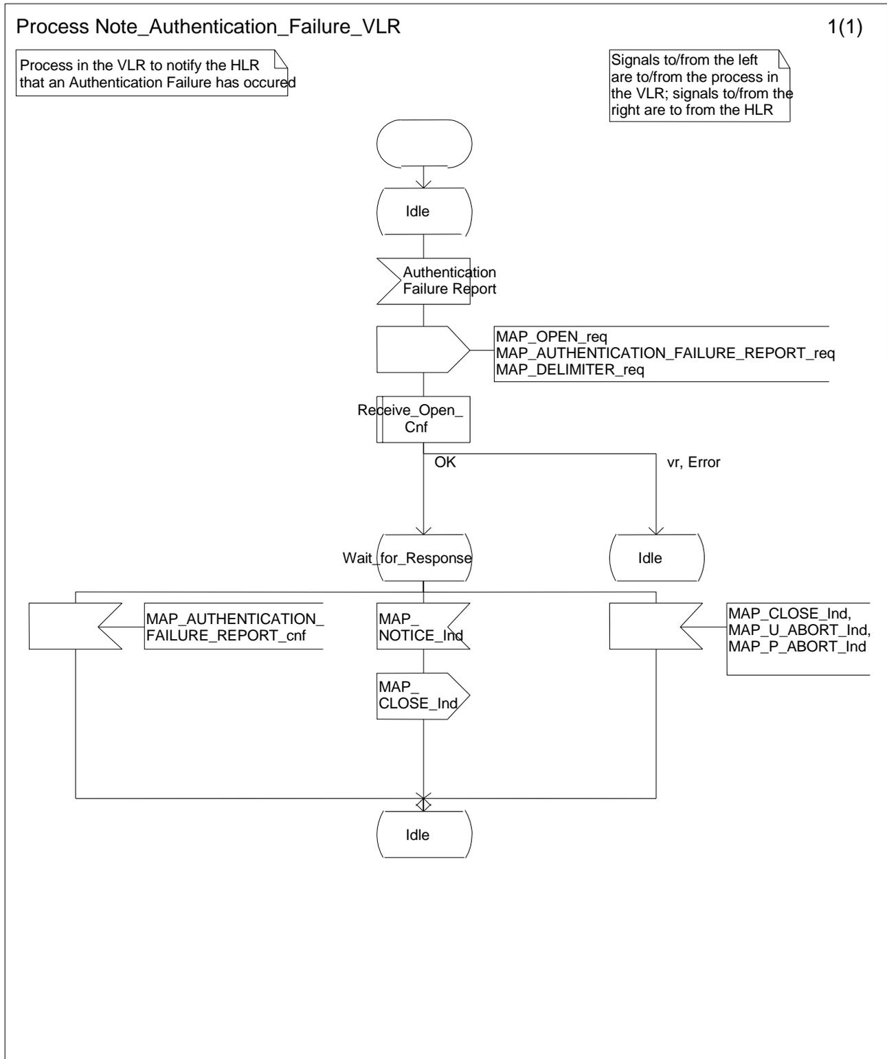
Figure 25.6/8: Process Note\_Authentication\_Failure\_VLR
