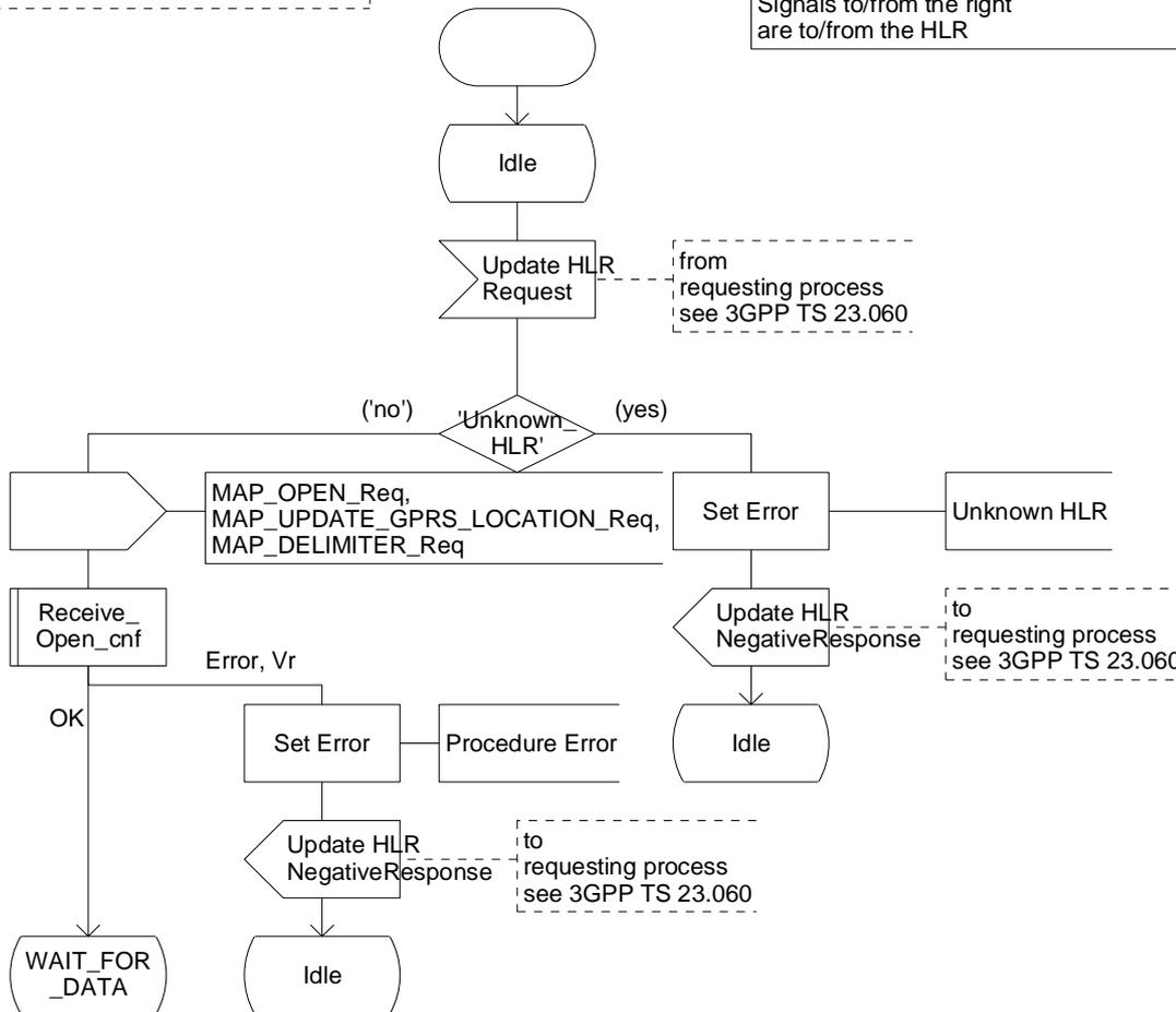
Figure 19.1.1/20 (sheet 1 of 2): Process SGSN\_Update\_HLR
