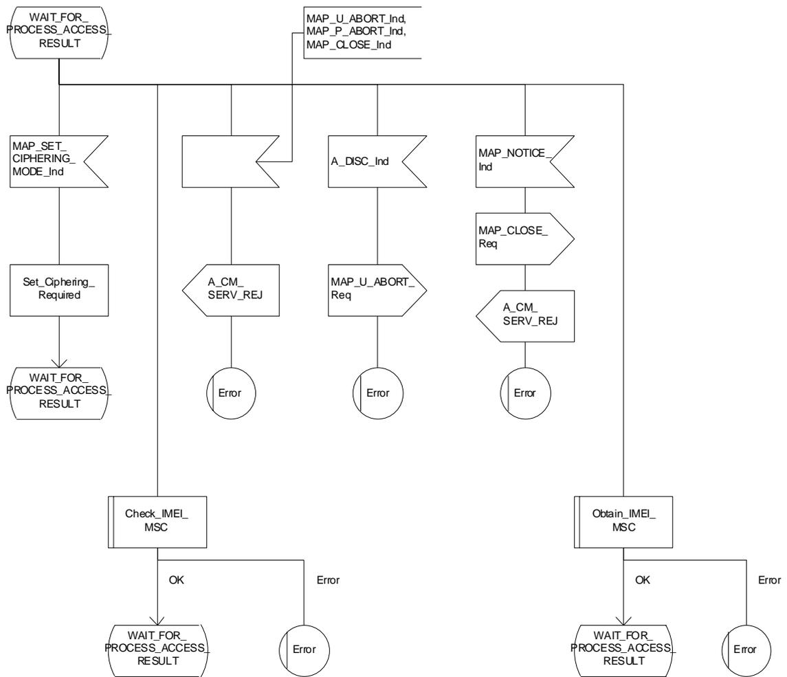
Figure 25.4/1 (sheet 2 of 3): Macro Process\_Access\_Request\_MSC
