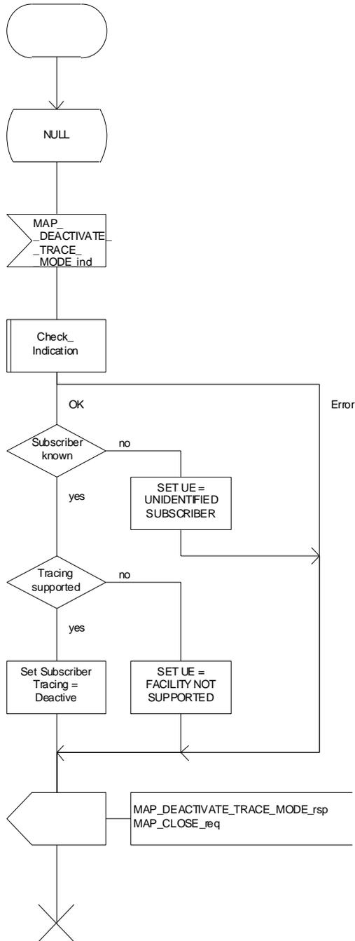
Figure 20.2/10: Process DTM\_VLR\_Standalone
