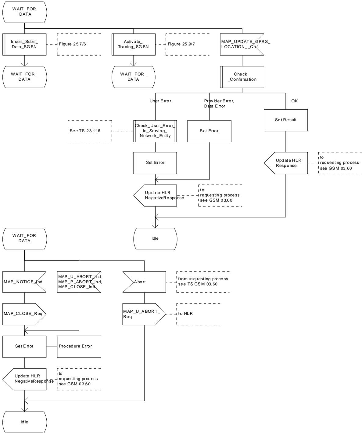
Figure 19.1.1/20 (sheet 2 of 2): Process SGSN\_Update\_HLR
