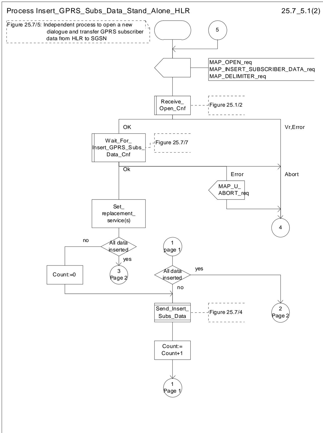
Figure 25.7/5 (sheet 1 of 2): Process Insert\_GPRS\_Subscriber\_Data\_Stand\_Alone\_HLR
