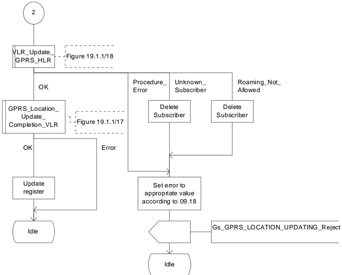
Figure 19.1.1/16 (sheet 2 of 2): Process GPRS\_Update\_Location\_Area\_VLR
