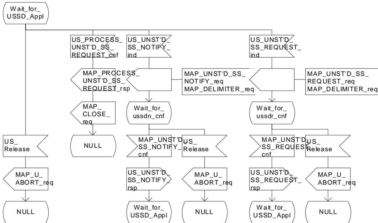
Figure 22.9.4/1 (sheet 2 of 4): Procedure MI\_USSD\_HLR
