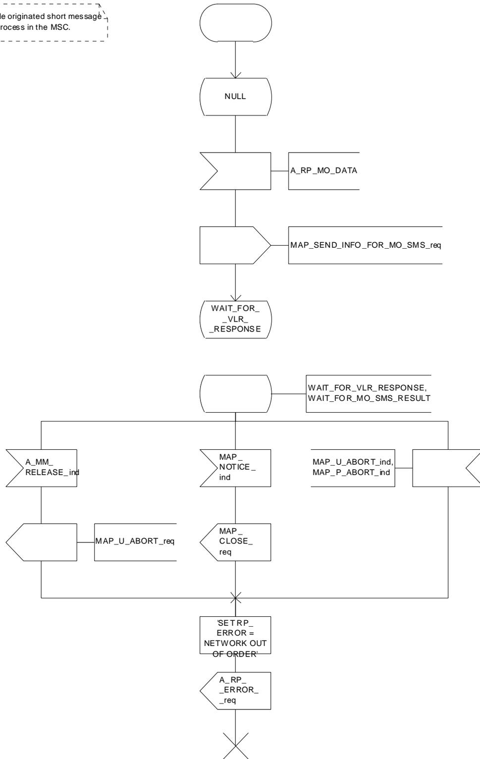
Figure 23.2/2 (sheet 1 of 4): Process MOSM\_MSC
