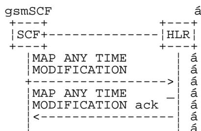
**Figure 24A.2/1: Message flow for any time modification**
