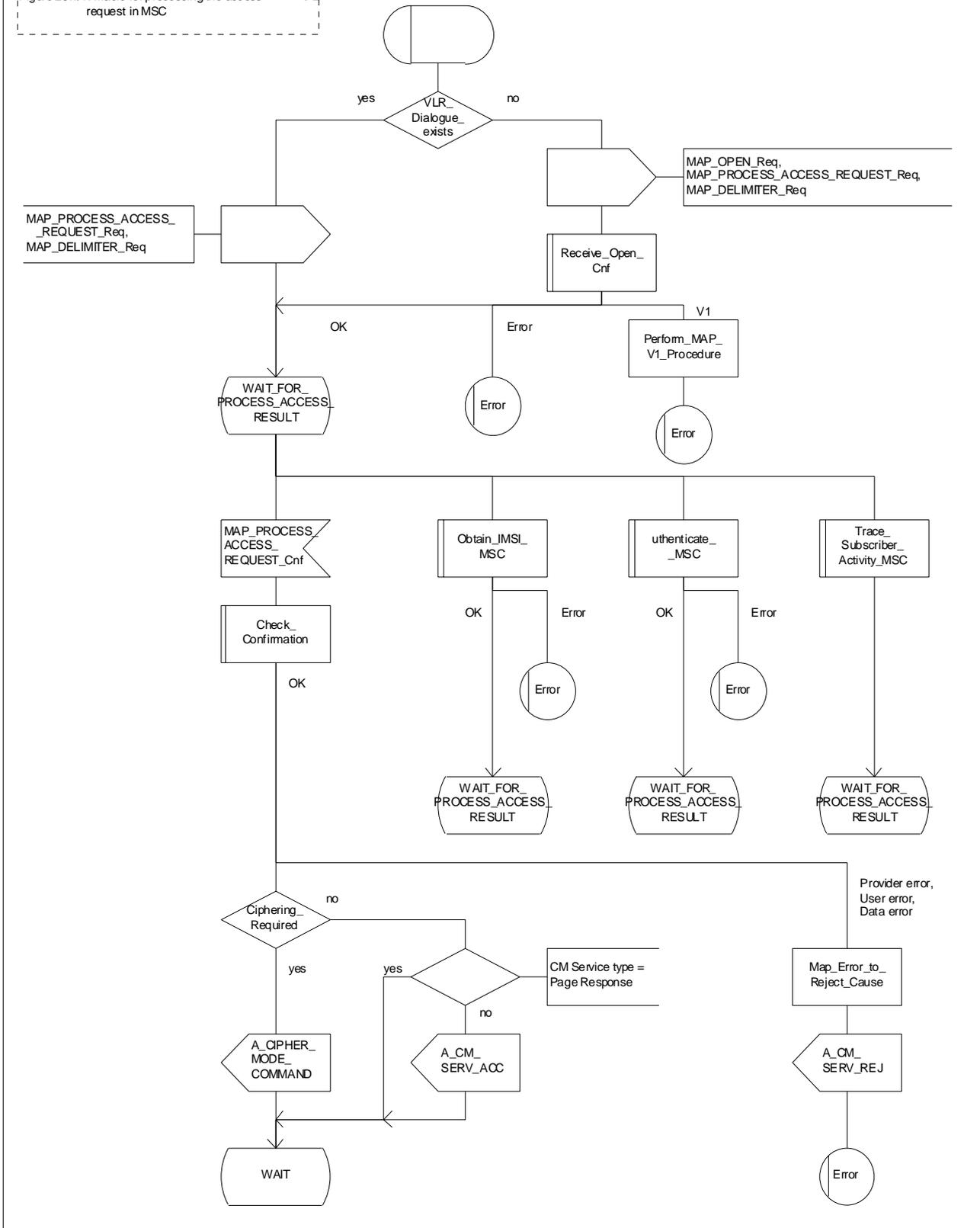
Figure 25.4/1 (sheet 1 of 3): Macro Process\_Access\_Request\_MSC
