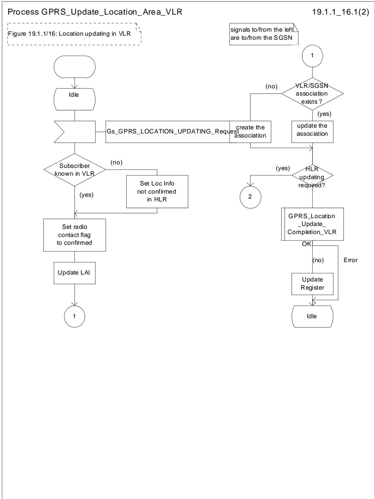
Figure 19.1.1/16 (sheet 1 of 2): Process GPRS\_Update\_Location\_Area\_VLR
