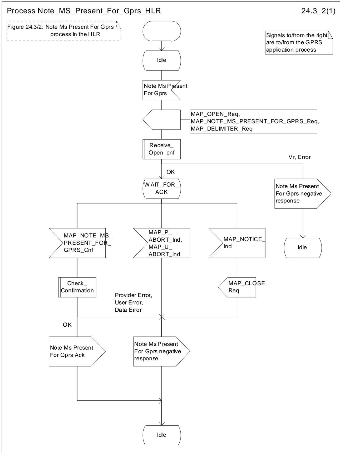
Figure 24.3/2: Process Note\_Ms\_Present\_For\_Gprs\_HLR
