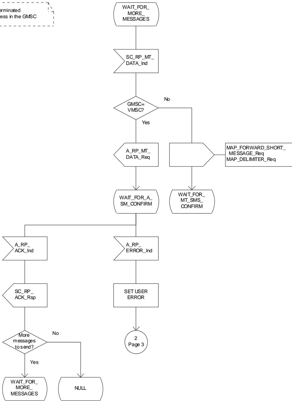
Figure 23.3/7 (sheet 4 of 6): Procedure\_MT\_SM\_GMSC
