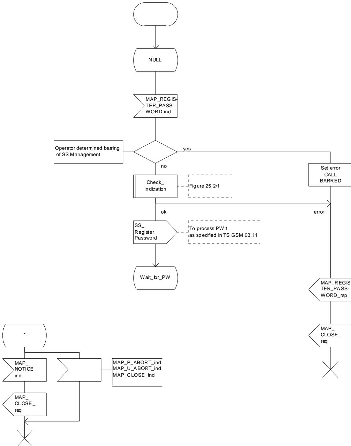
Figure 22.8.4/1 (sheet 1 of 2): Procedure Register\_PW\_HLR
