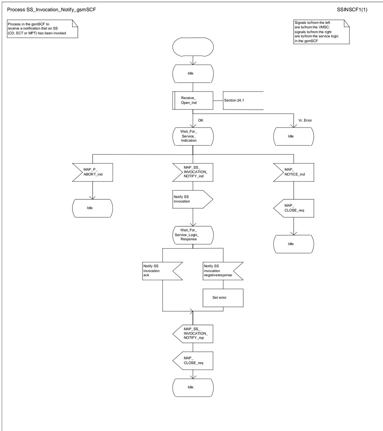
Figure 22.12.3/1: Process SS\_Invocation\_Notify\_gsmSCF (sheet 1 of 1)
