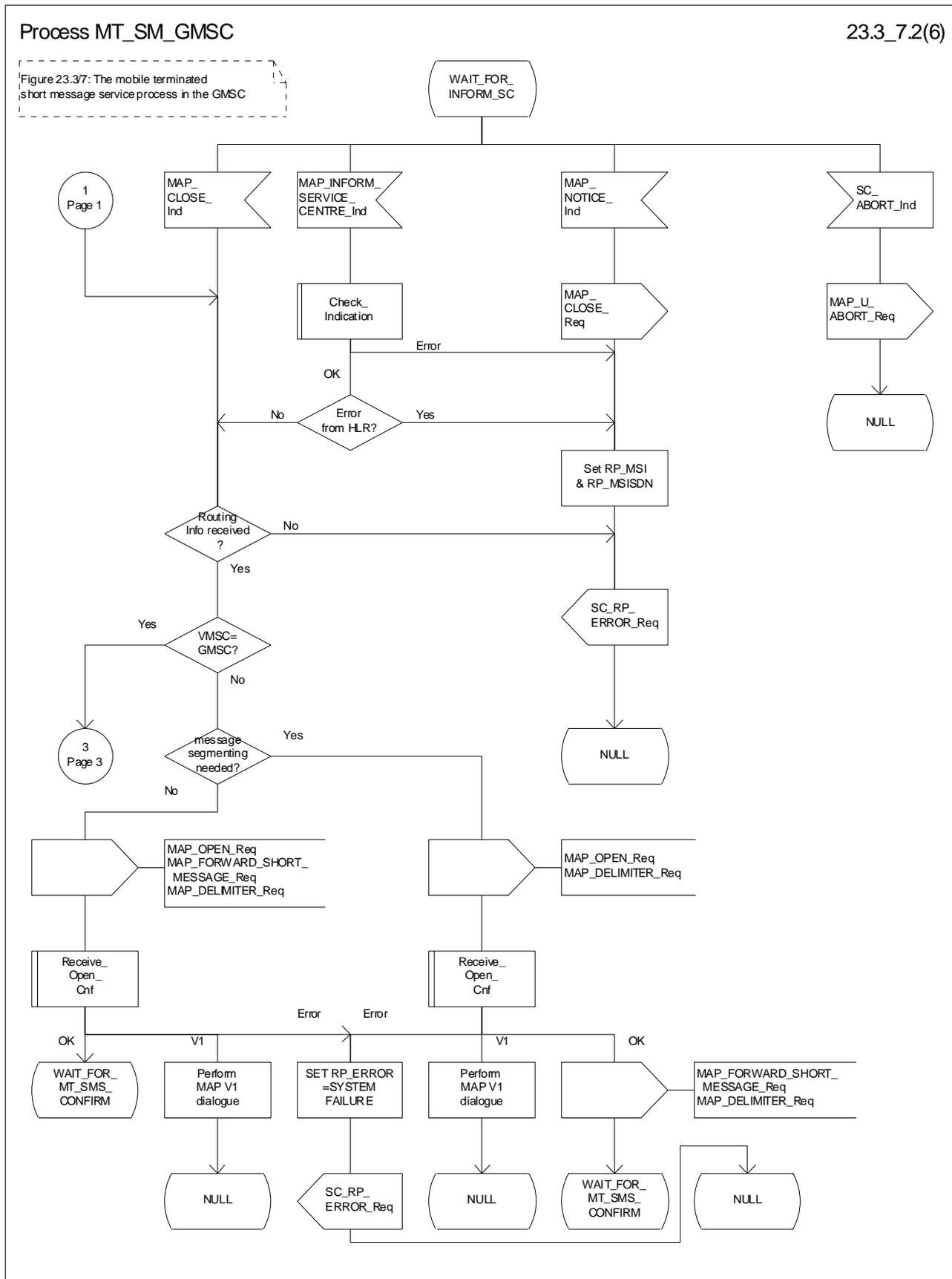
Figure 23.3/7 (sheet 2 to 6): Procedure MT\_SM\_GMSC
