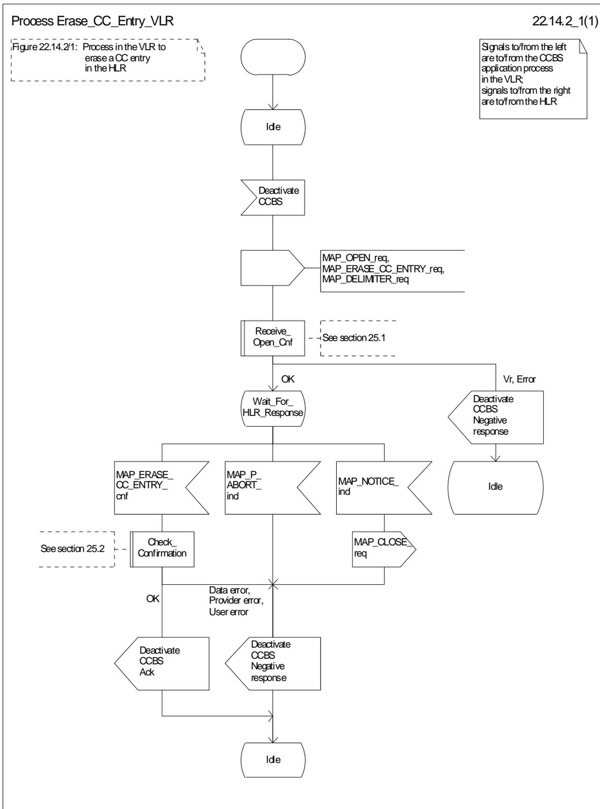
Figure 22.14.2/1: Process Erase\_CC\_Entry\_VLR
