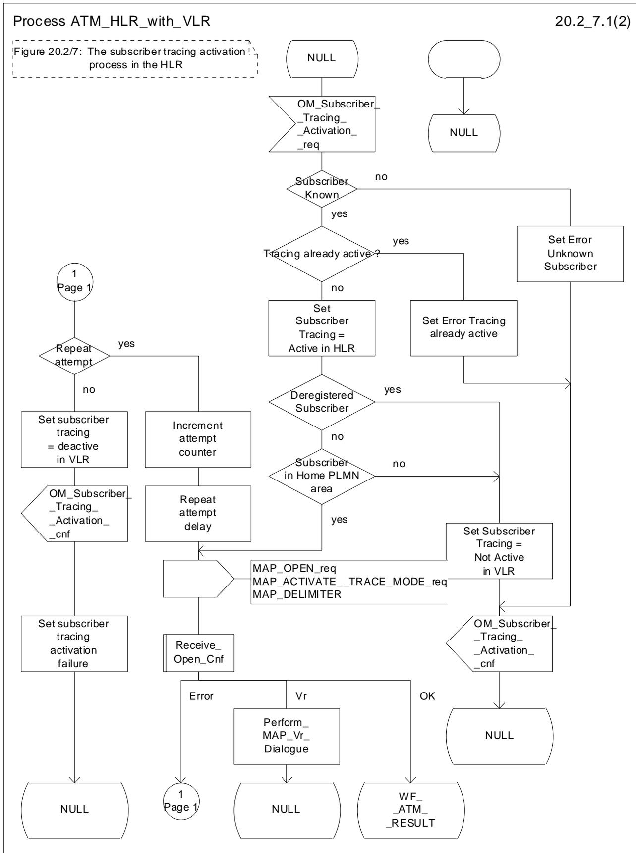
Figure 20.2/7 (sheet 1 of 2): Process ATM\_HLR\_with\_VLR
