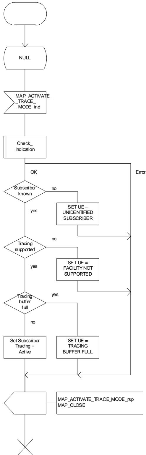
Figure 20.2/9: Process ATM\_VLR\_Standalone
