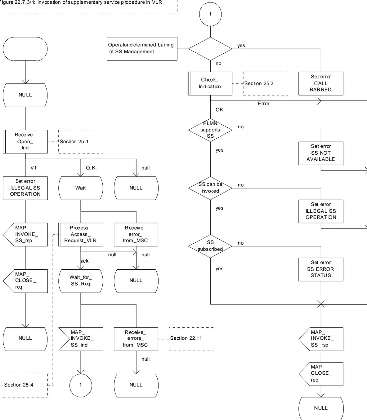
Figure 22.7.3/1: Procedure Invoke\_SS\_VLR
