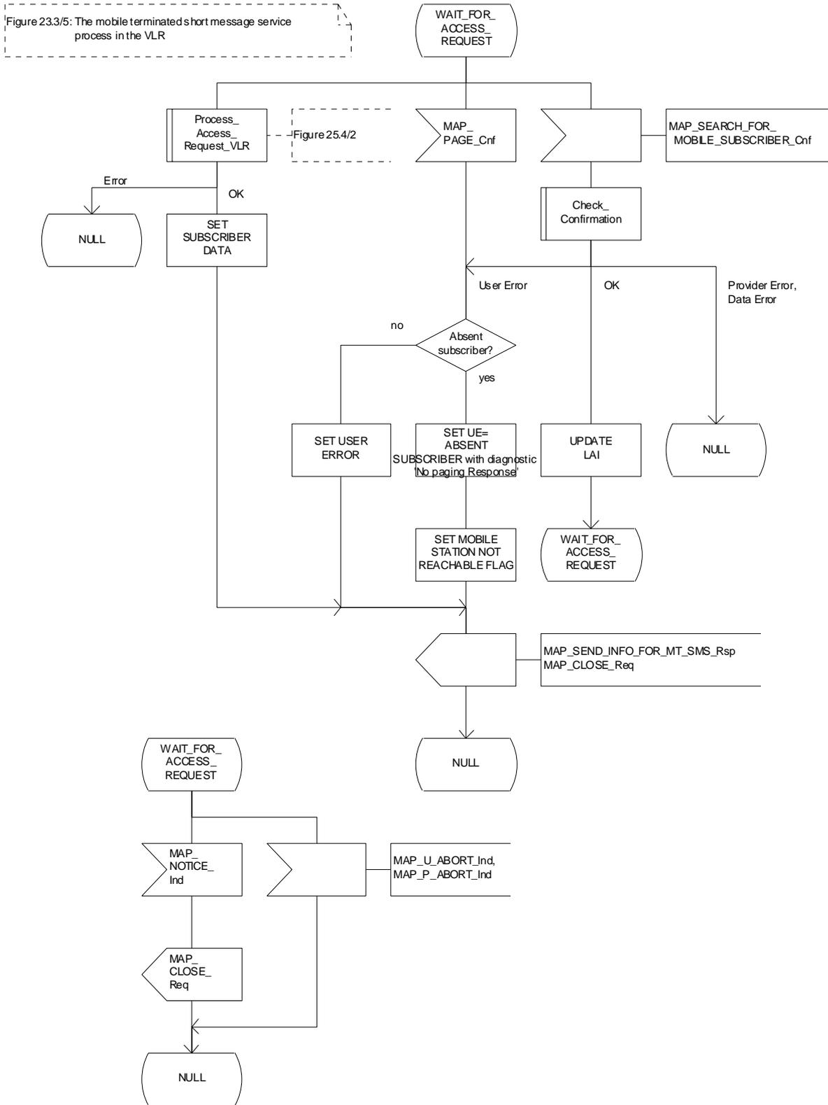
Figure 23.3/5 (sheet 3 to 3): Process MT\_SM\_VLR
