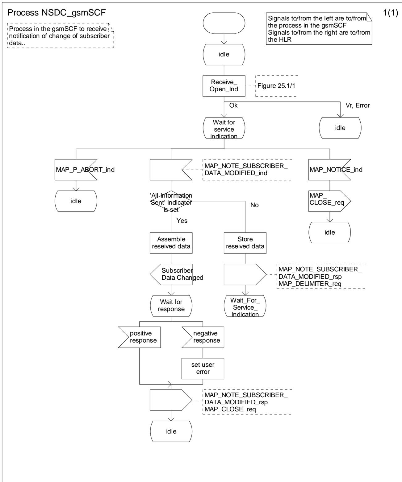
Figure 24A.3/3: Process Subscriber\_Data\_Modification\_Notification\_gsmSCF (sheet 1 of 1)
