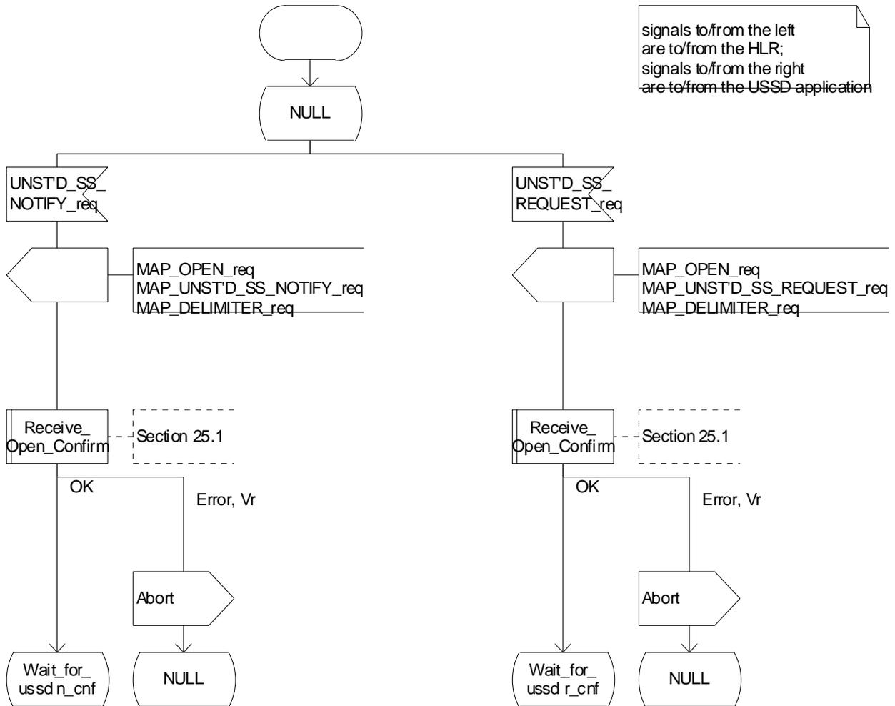
Figure 22.10.5/1 (sheet 1 of 2): Procedure NI\_USSD\_gsmSCF\_secondary\_HLR
