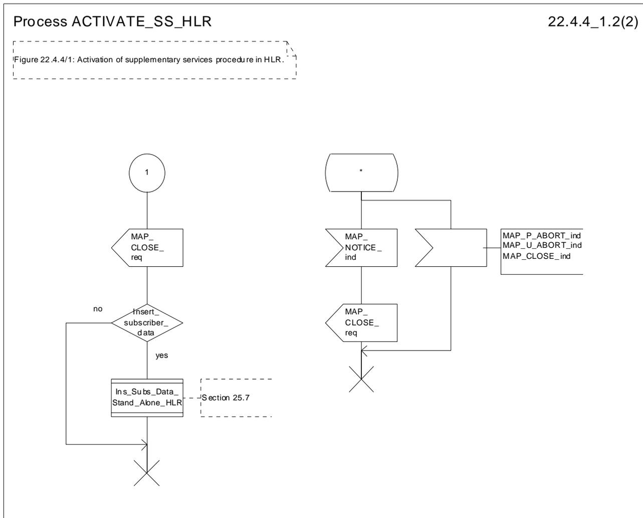
Figure 22.4.4/1 (sheet 2 of 2): Procedure Activate\_SS\_HLR
