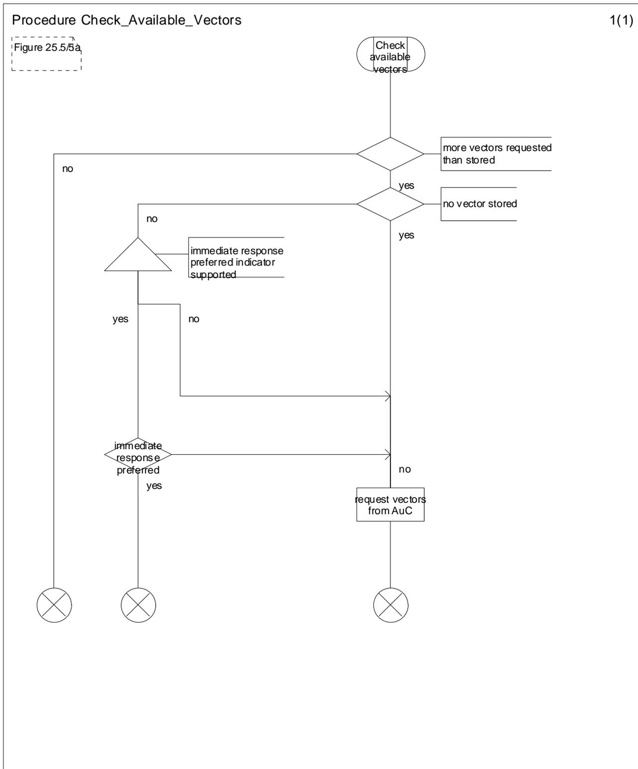
Figure 25.5/6: Procedure Check\_Available\_Vectors
