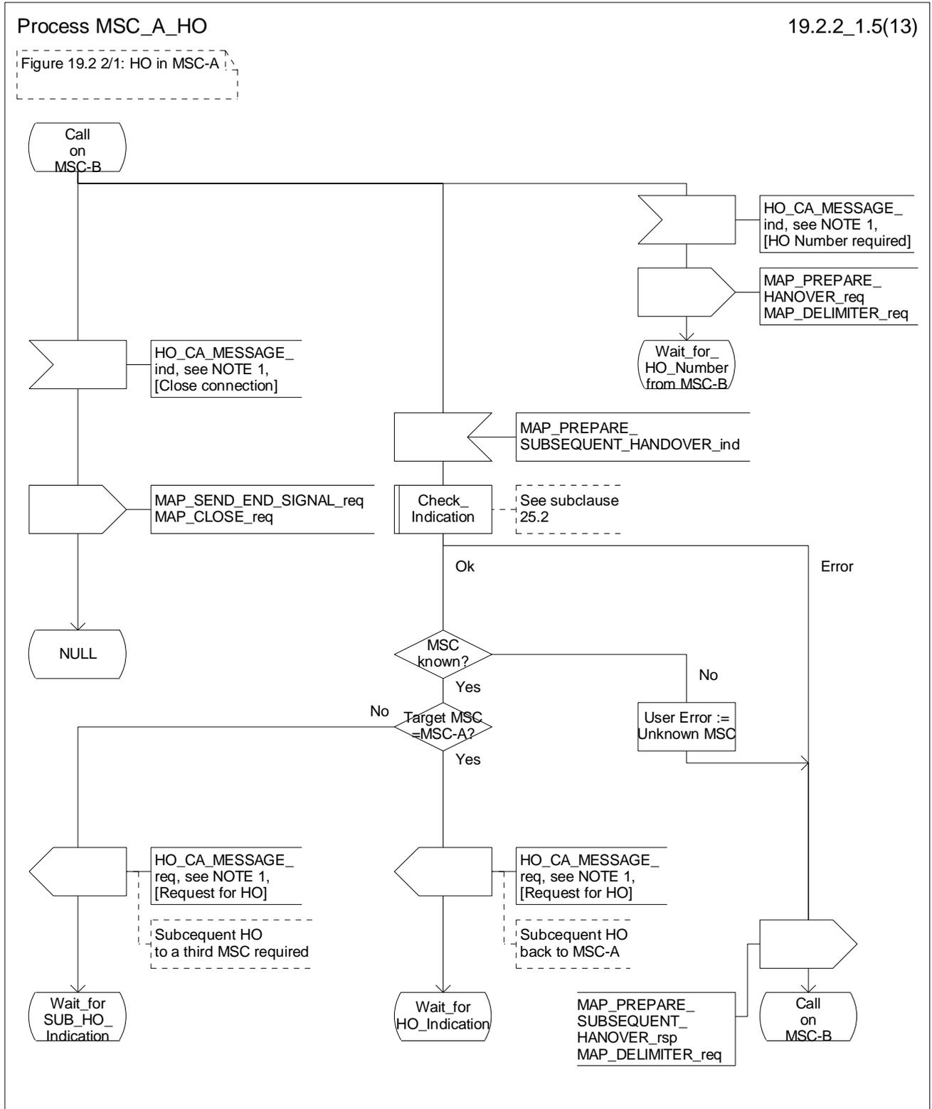
Figure 19.2.2/1 (sheet 5 of 13): Process MSC\_A\_HO
