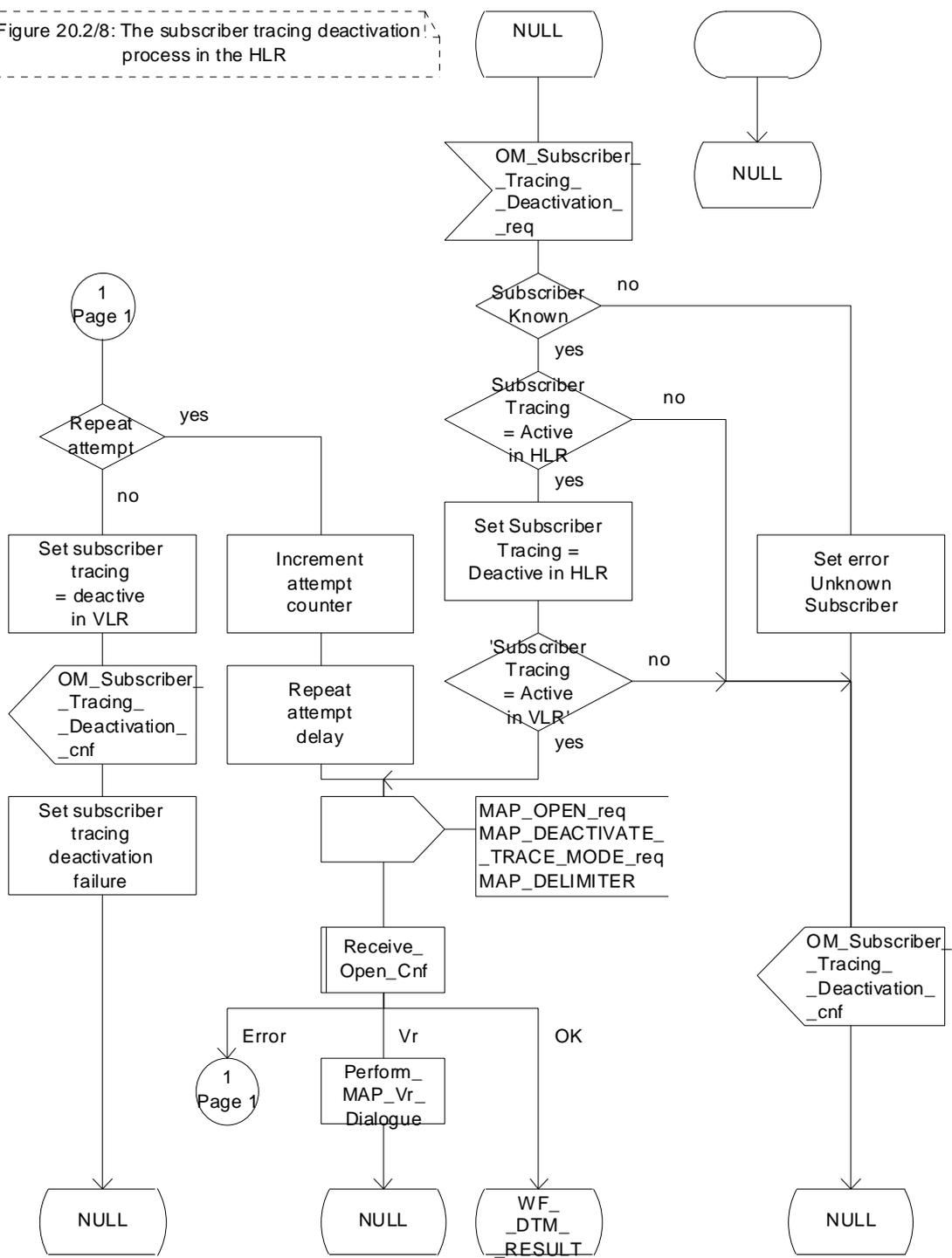
Figure 20.2/8 (sheet 1 of 2): Process DTM\_HLR\_with\_VLR
