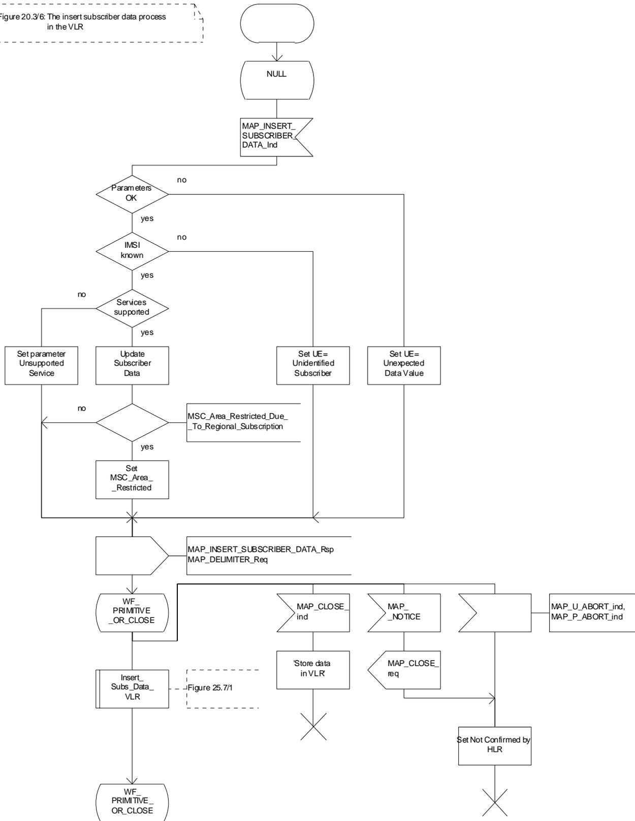
Figure 20.3/6: Process INS\_SUBS\_DATA\_VLR
