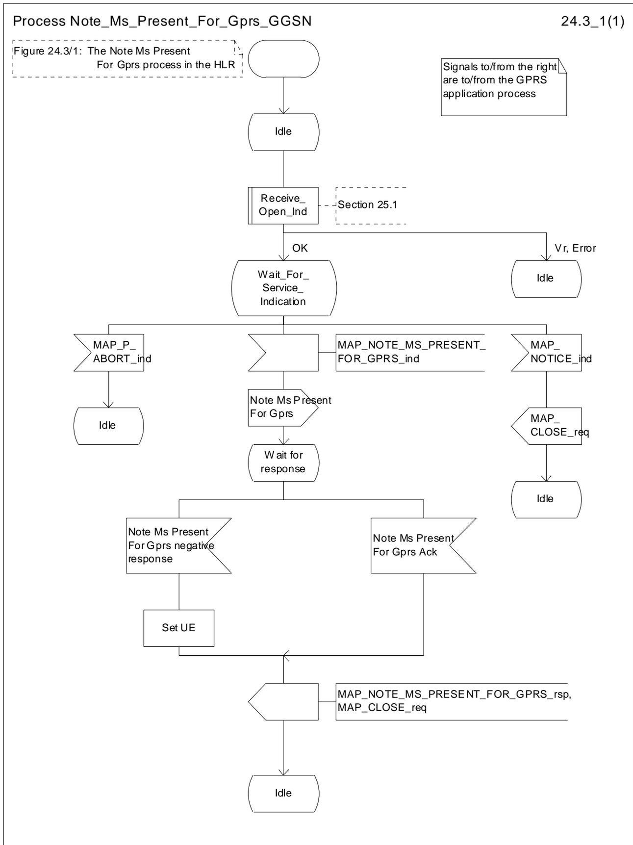
Figure 24.3/1: Process Note\_Ms\_Present\_For\_Gprs\_GGSN
