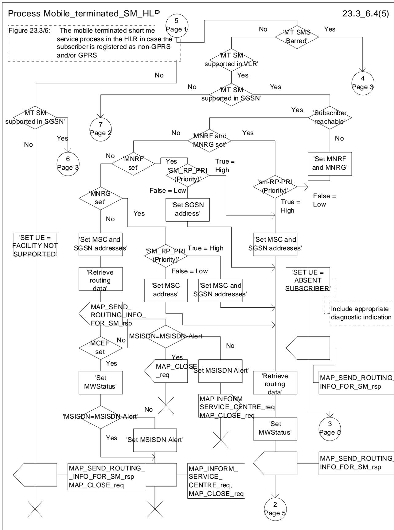
Figure 23.3/6 (sheet 4 of 5): Process Mobile\_terminated\_SM\_HLR
