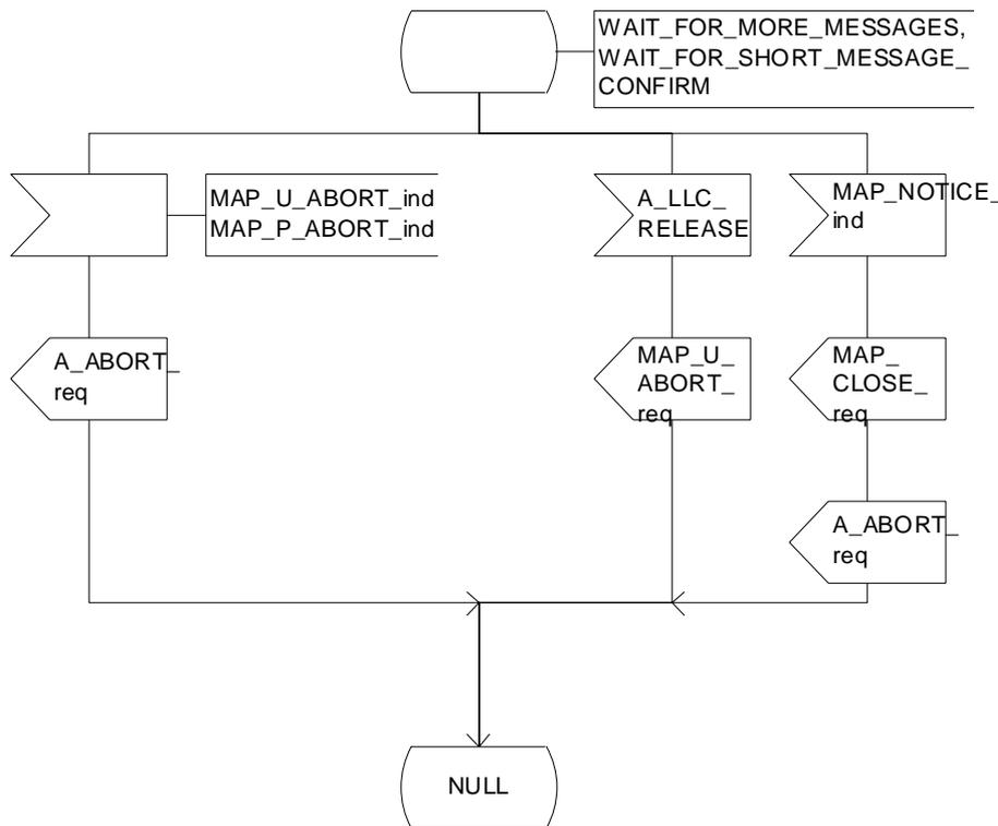
Figure 23.3/9 (sheet 3 of 3): Procedure MT\_SM\_Transfer\_SGSN
