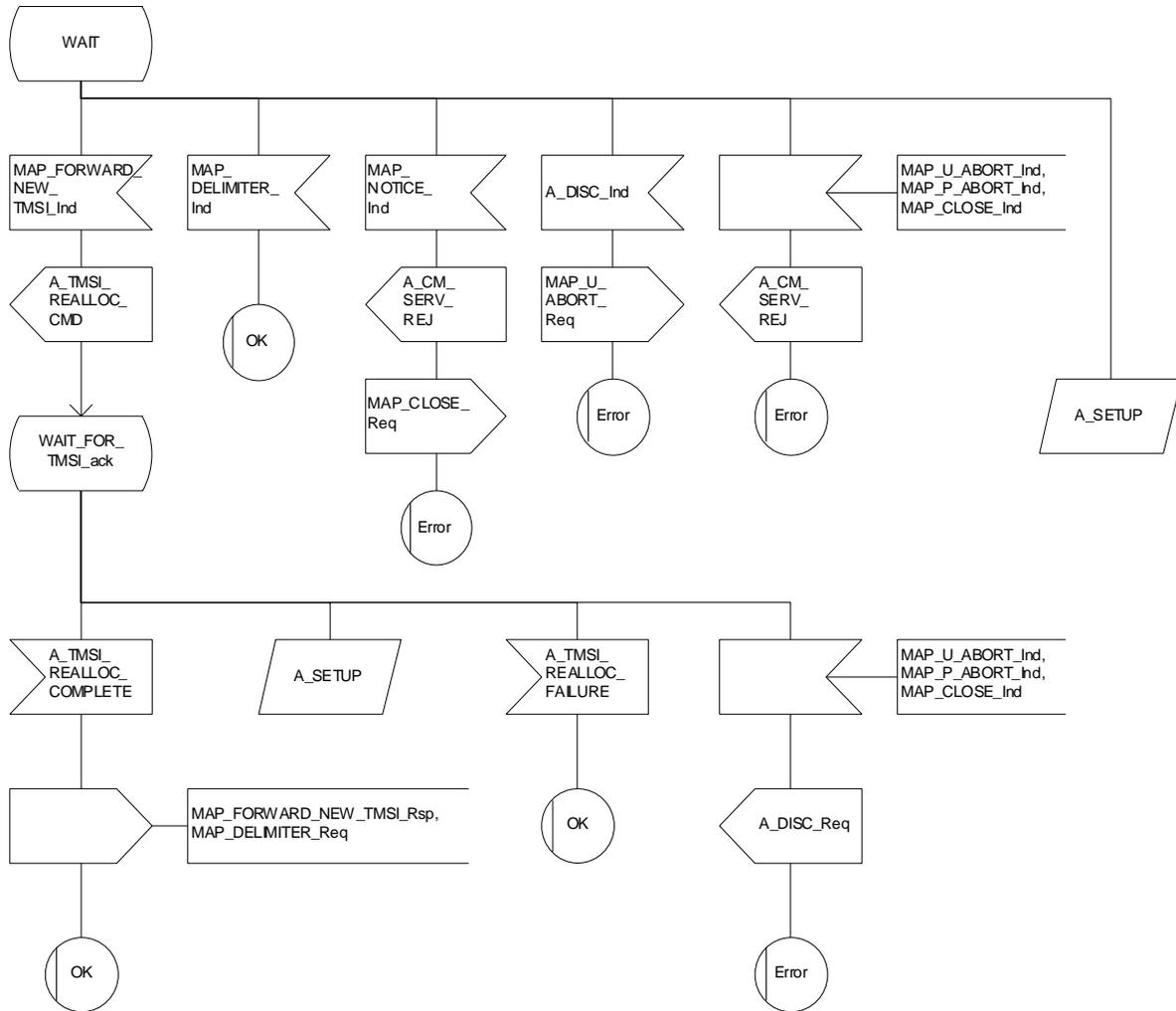
Figure 25.4/1 (sheet 3 of 3): Macro Process\_Access\_Request\_MSC
