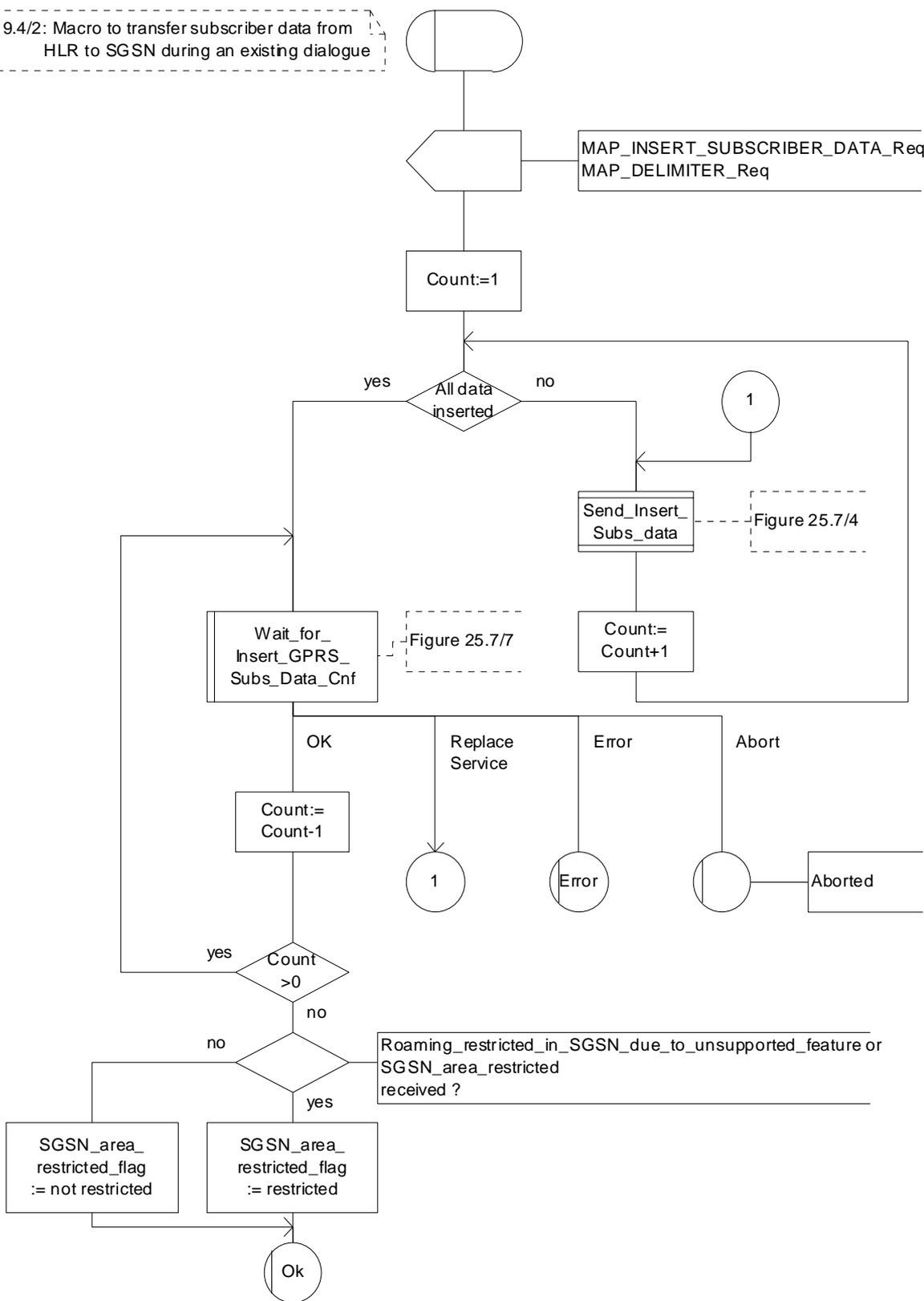
Figure 19.4/2: Macro Insert\_Subs\_Data\_In\_SGSN\_Framed\_HLR
