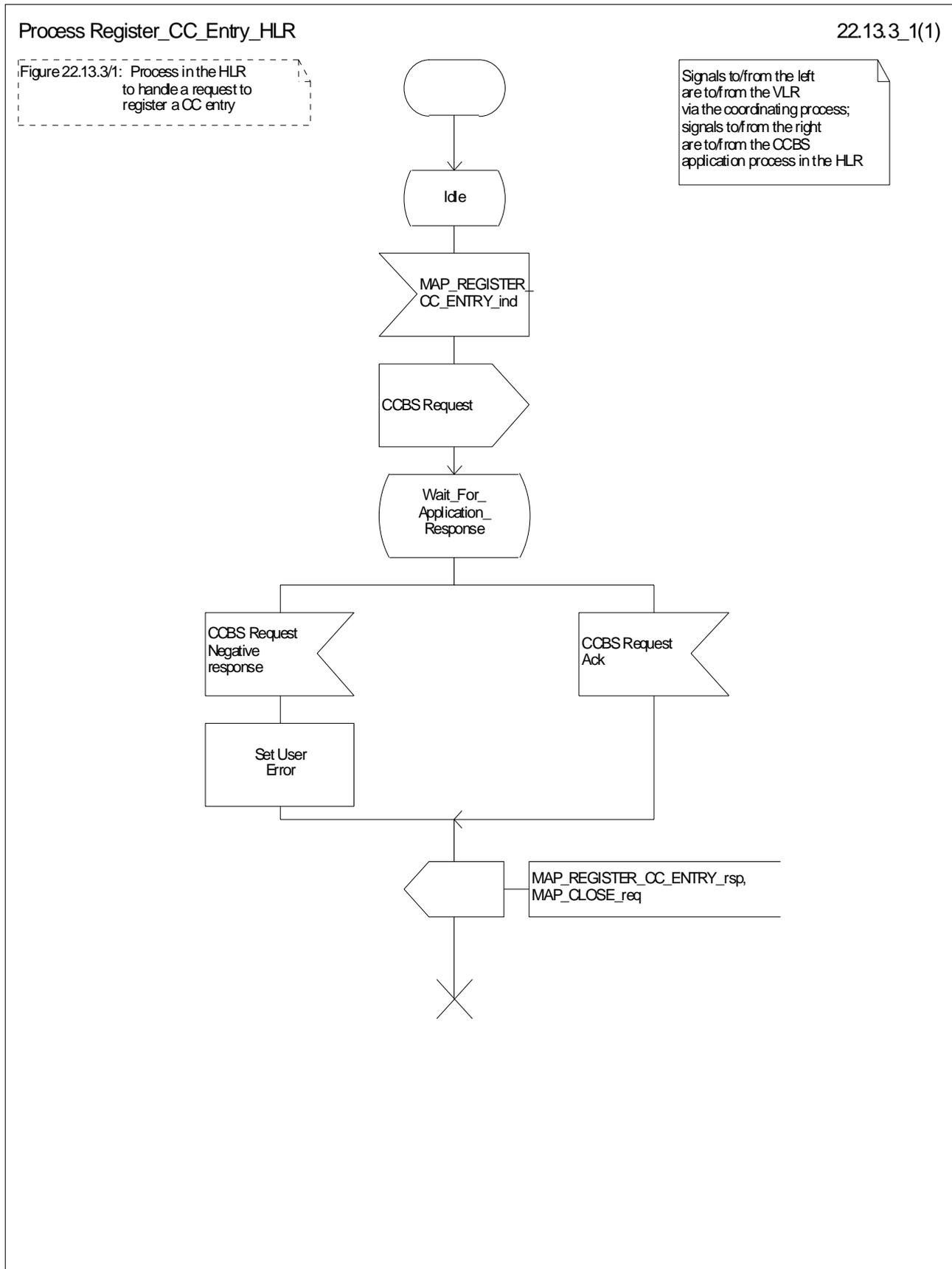
Figure 22.13.3/1: Process Register\_CC\_Entry\_HLR
