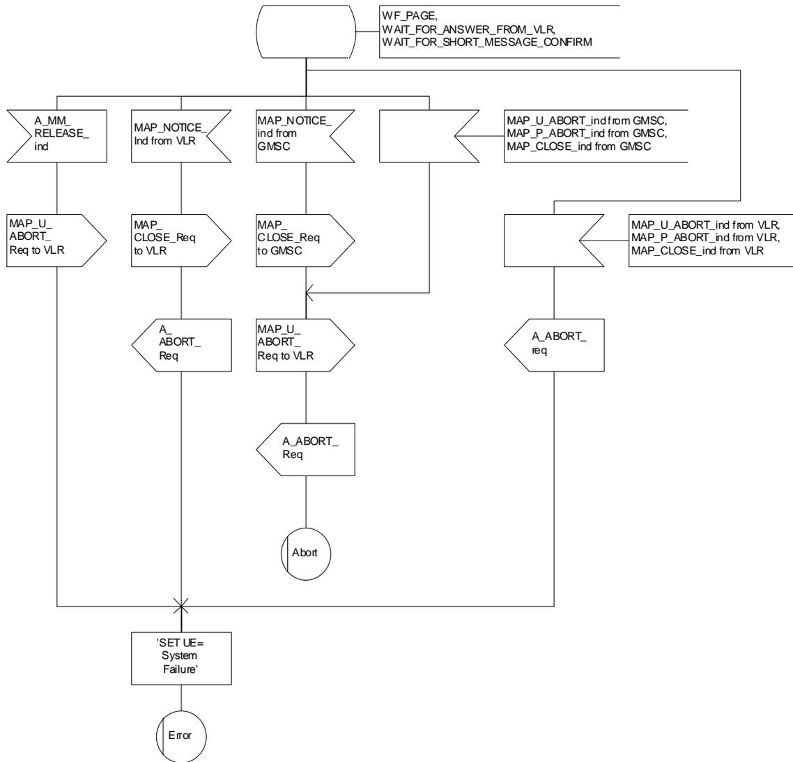
Figure 23.3/4 (sheet 3 of 3): Macro MT\_SM\_Transfer\_MSC
