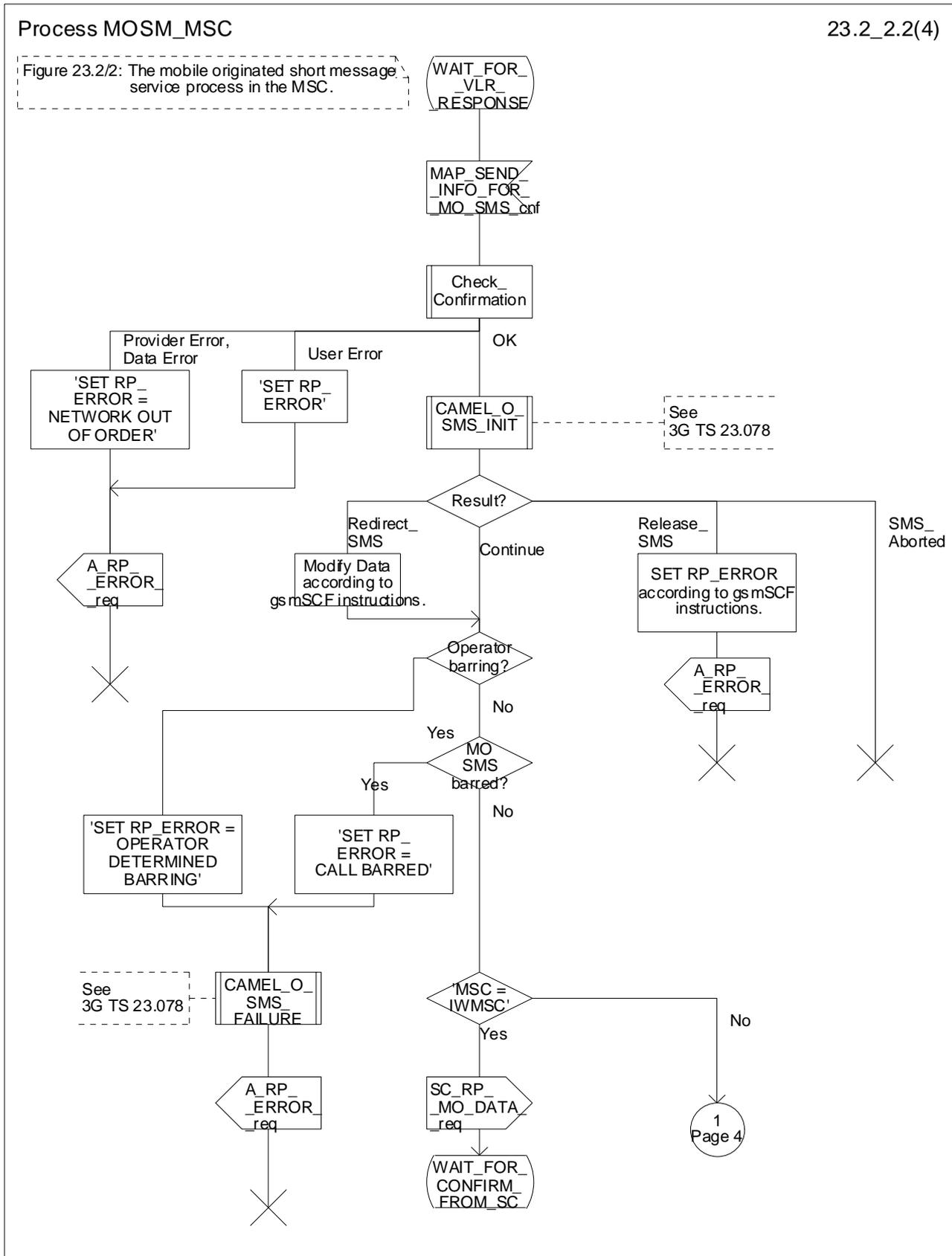
Figure 23.2/2 (sheet 2 of 4): Process MOSM\_MSC
