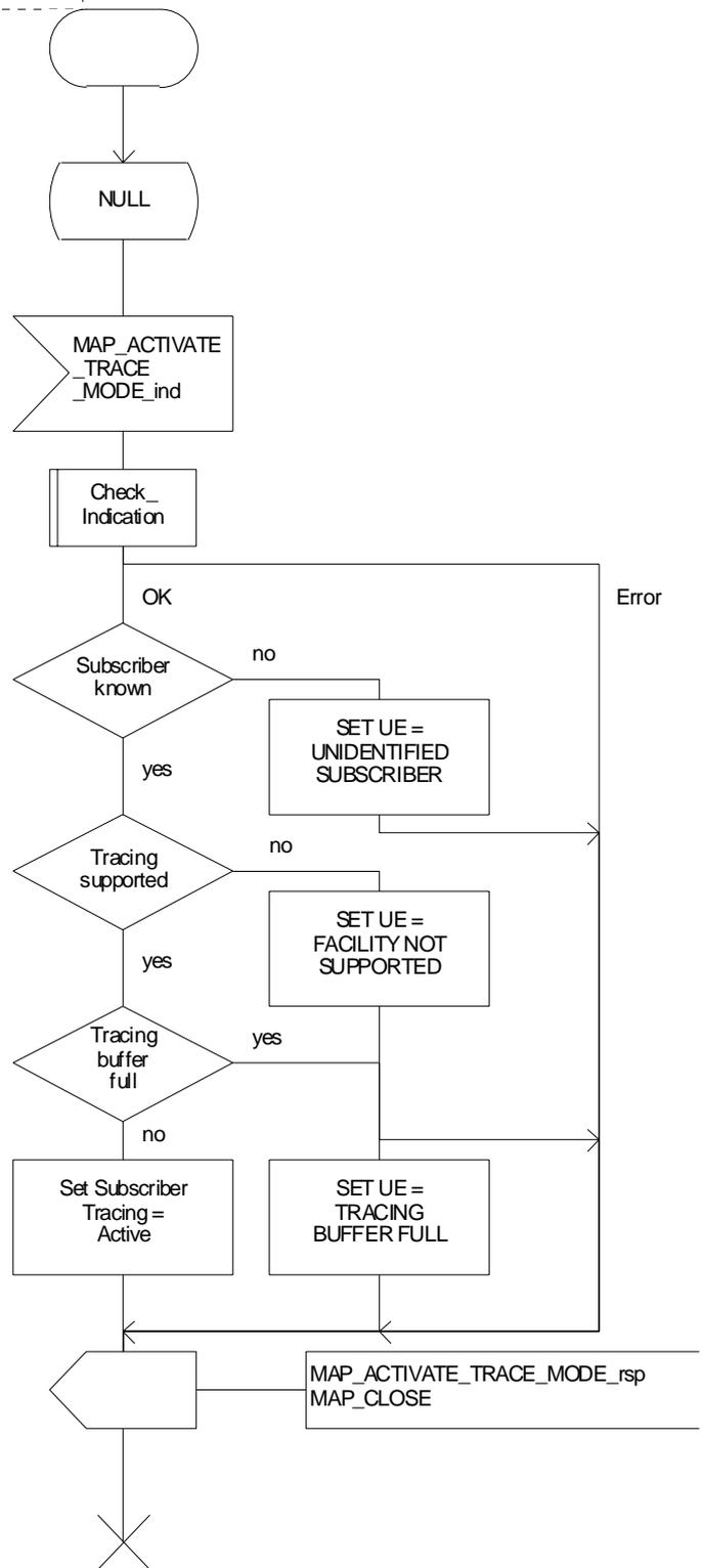
Figure 20.2/16: Process ATM\_SGSN\_Standalone
