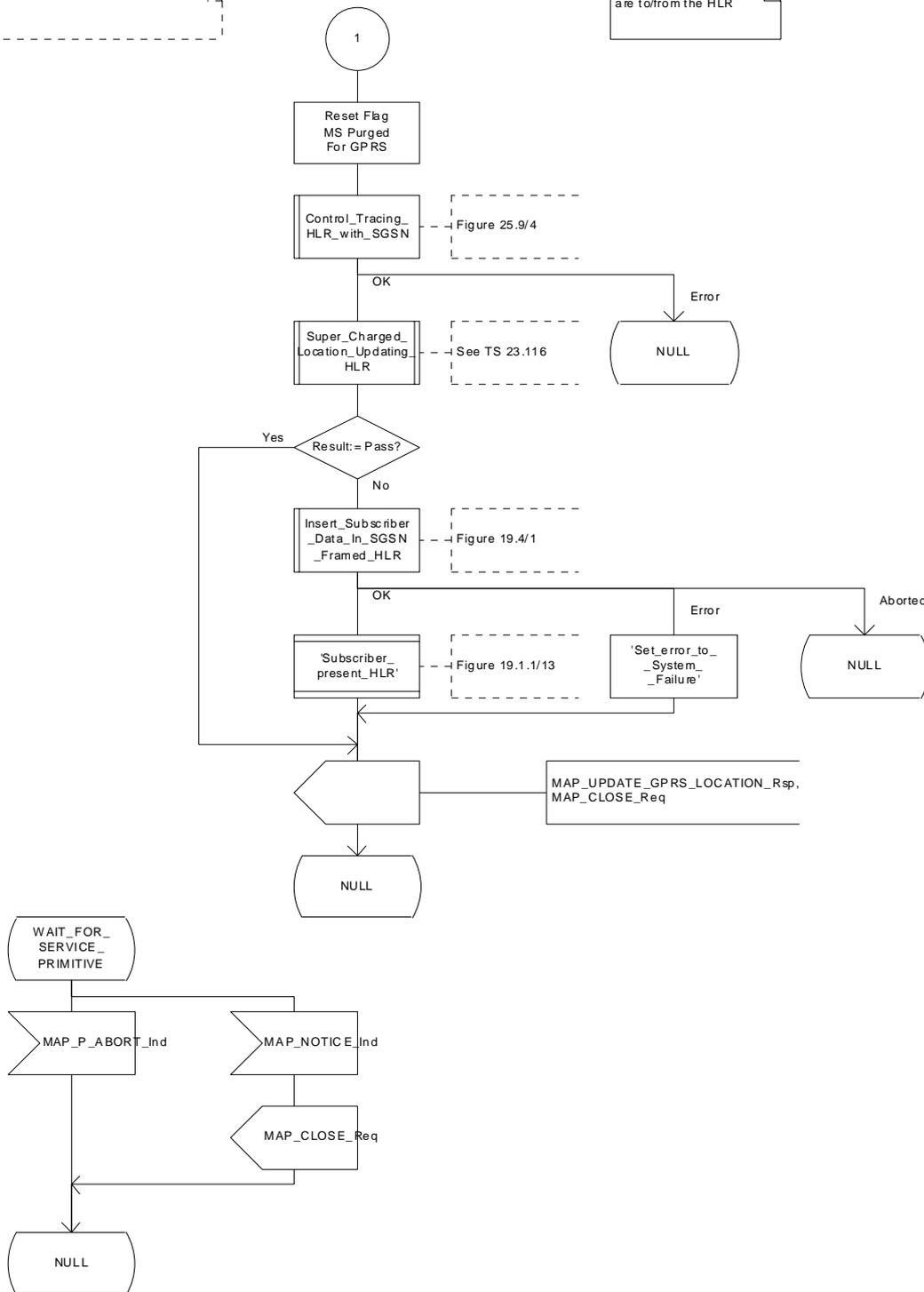
Figure 19.1.1/19 (sheet 2 of 2): Process Update\_GPRS\_Location\_HLR
