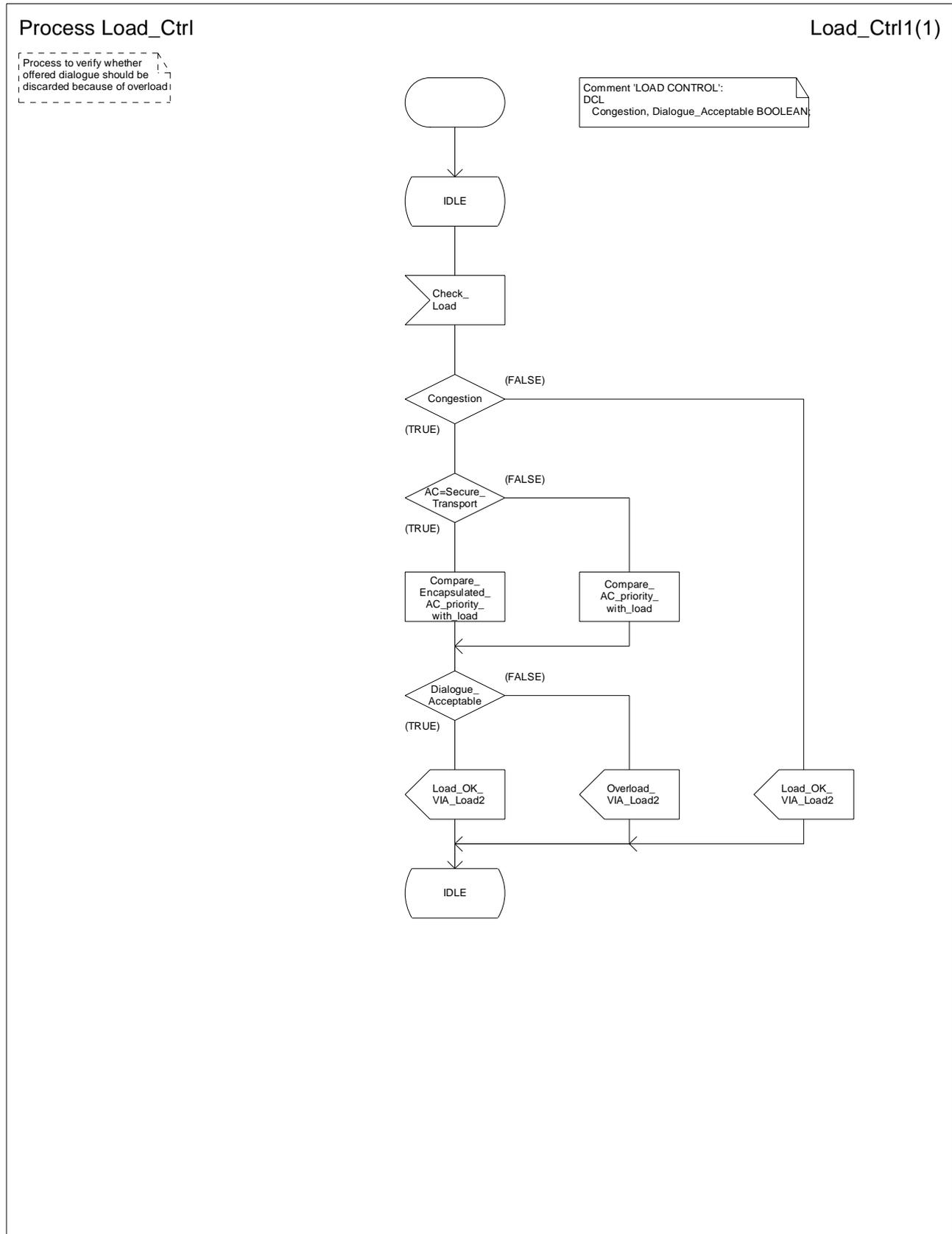
Figure 15.6/5: Process Load\_Ctrl
