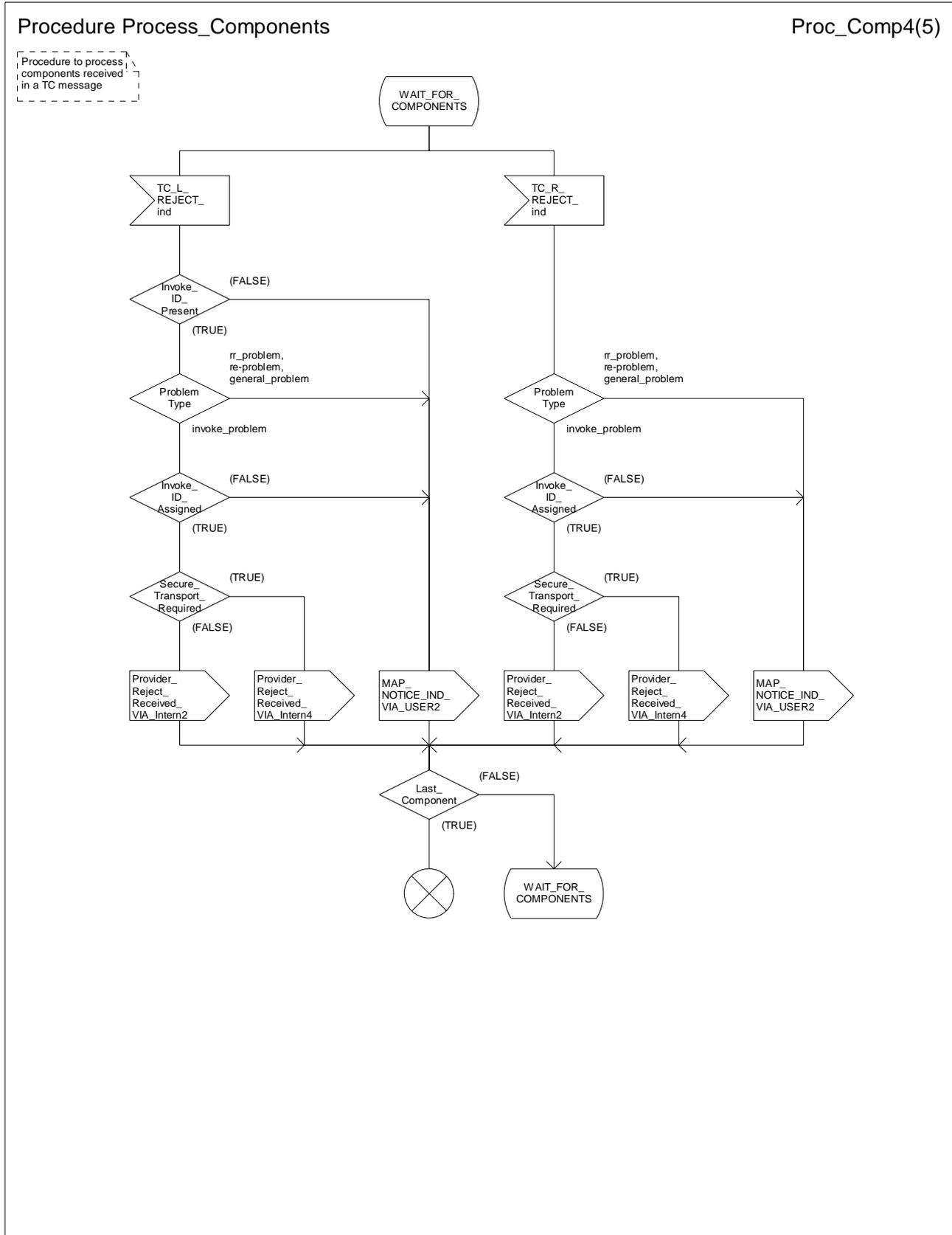
Figure 15.6/4d: Procedure Process\_Components (sheet 4)
