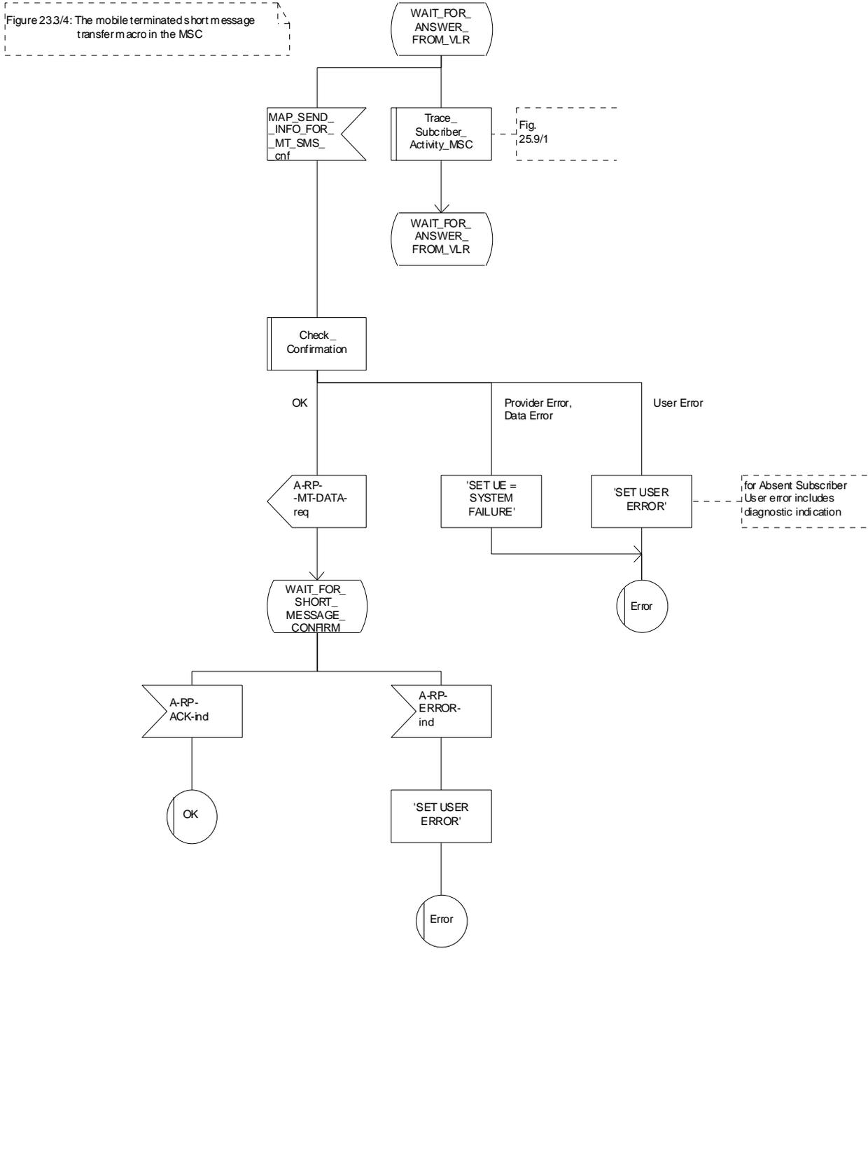
Figure 23.3/4 (sheet 2 of 3): Macro MT\_SM\_Transfer\_MSC
