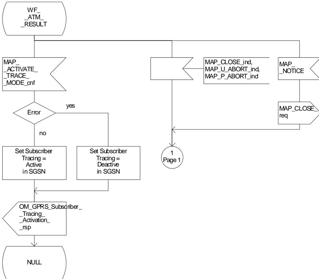
Figure 20.2/14 (sheet 2 of 2): Process ATM\_HLR\_with\_SGSN
