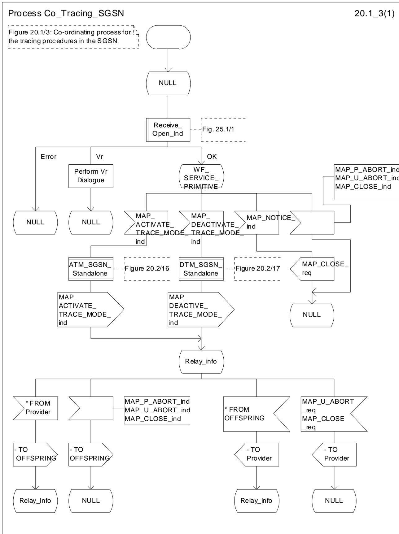
Figure 20.1/3: Process Co\_Tracing\_SGSN
