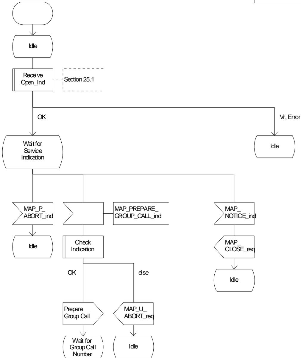
Figure 21.4/3 (sheet 1 of 3): Process ASCI\_Relay\_MSC
