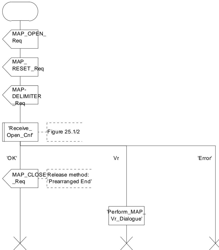
Figure 19.3/7: Process SEND\_RESET\_TO\_SGSN
