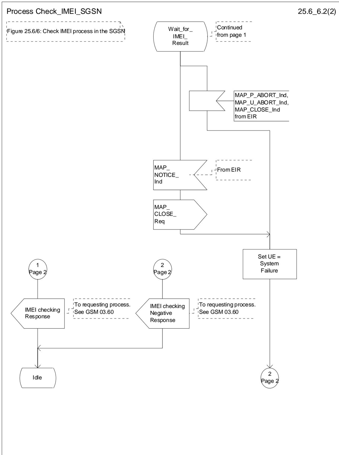
Figure 25.6/6 (sheet 2 of 2): Process Check\_IMEI\_SGSN
