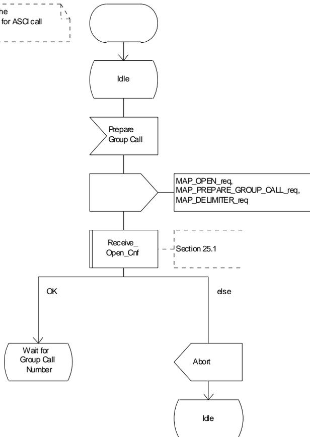
Figure 21.4/2 (sheet 1 of 4): Process ASCI\_Anchor\_MSC
