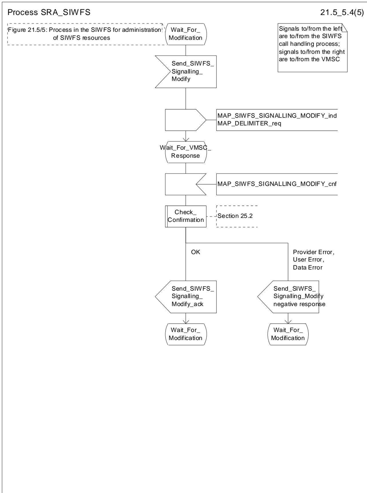
Figure 21.5/5 (sheet 4 of 5): Process SRA\_SIWFS
