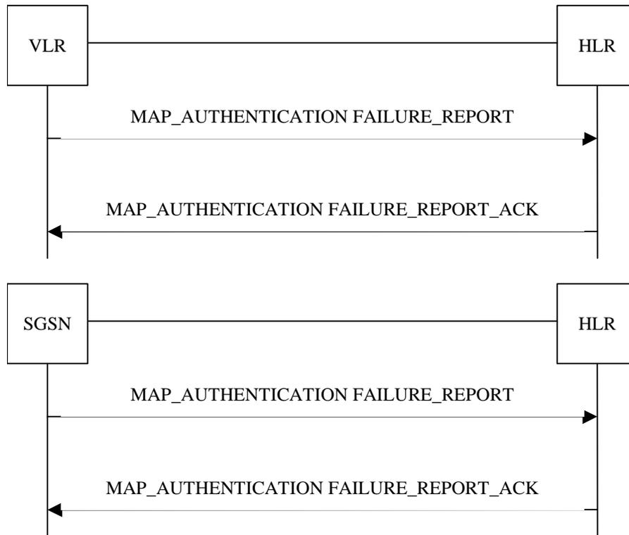
**Figure 25.6/7: Message Flows to Authentication Failure Report**
