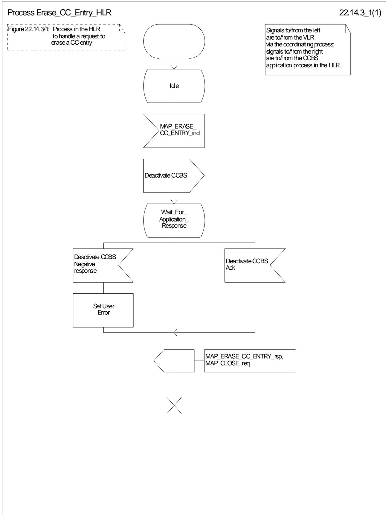
Figure 22.14.3/1: Process Erase\_CC\_Entry\_HLR
