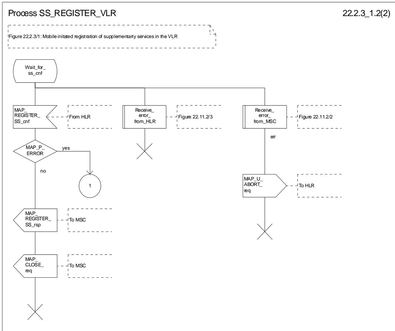
Figure 22.2.3/1 (sheet 2 of 2): Procedure SS\_Register\_VLR
