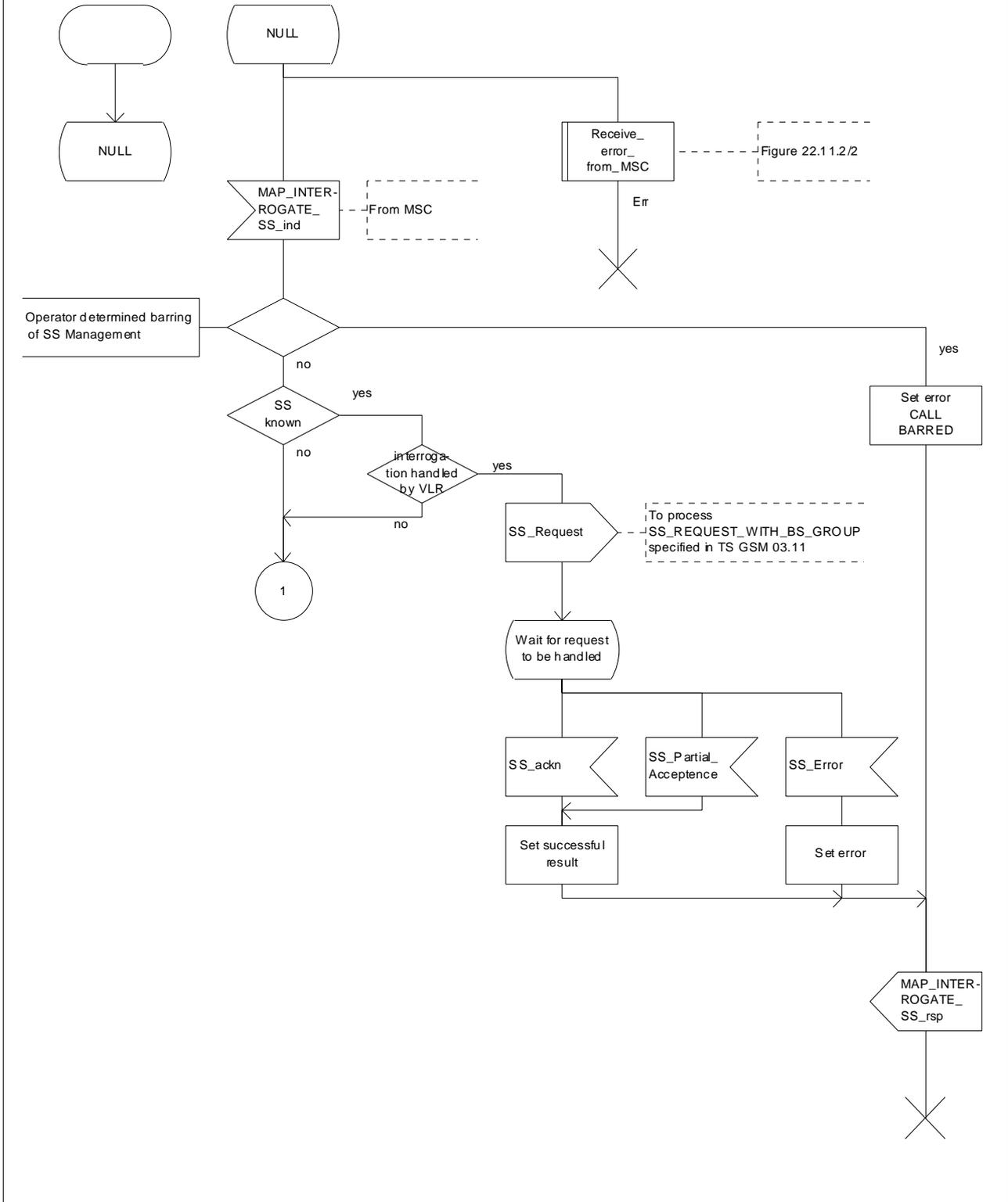
Figure 22.6.3/1 (sheet 1 of 3): Procedure Interrogate\_SS\_VLR
