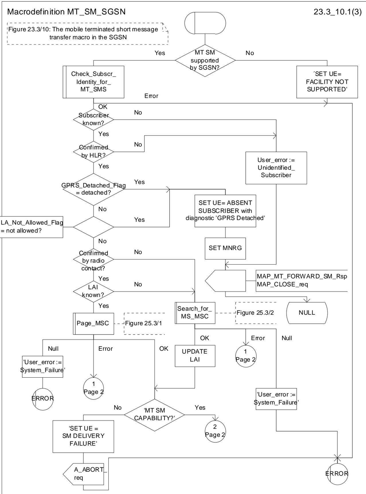
Figure 23.3/10 (sheet 1 of 3): Macro MT\_SM\_SGSN
