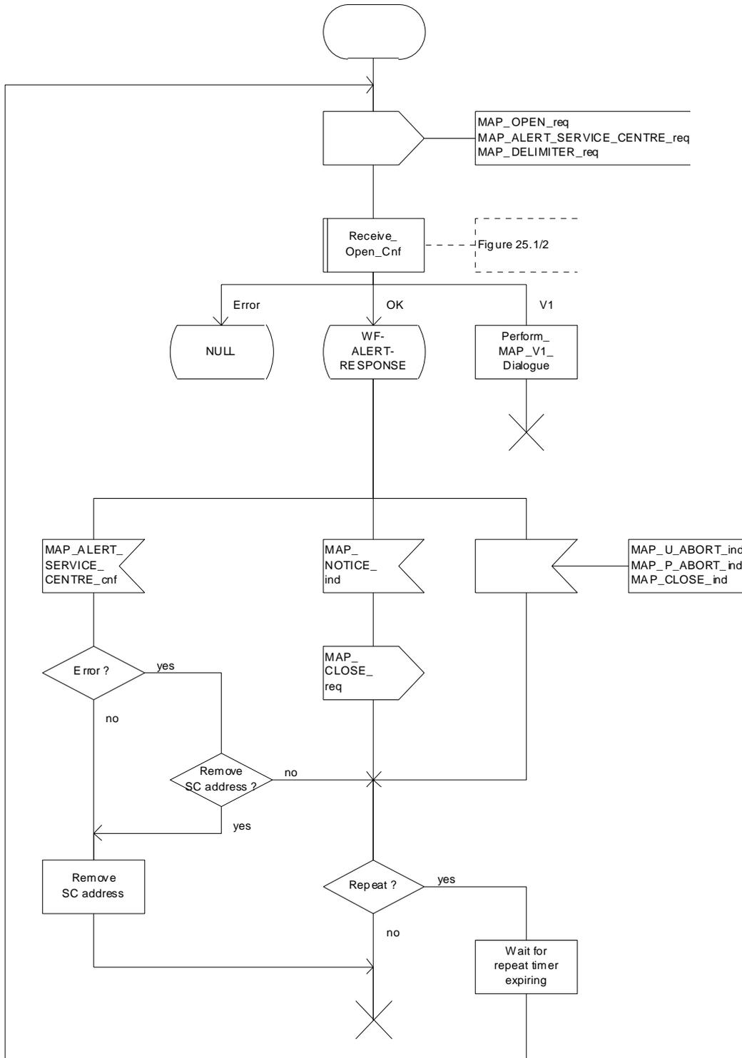
Figure 25.10/3: Process Alert\_Service\_Centre\_HLR
