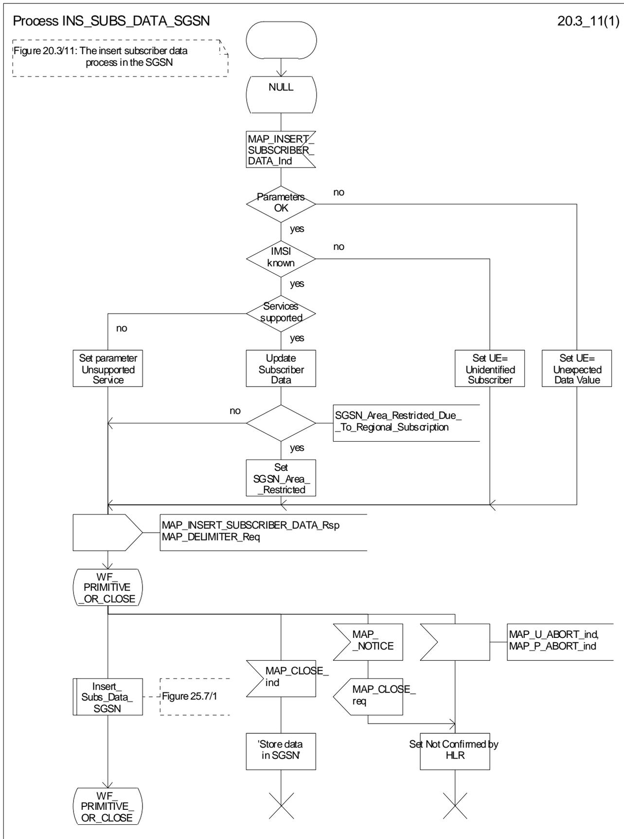
Figure 20.3/11: Process INS\_SUBS\_DATA\_SGSN
