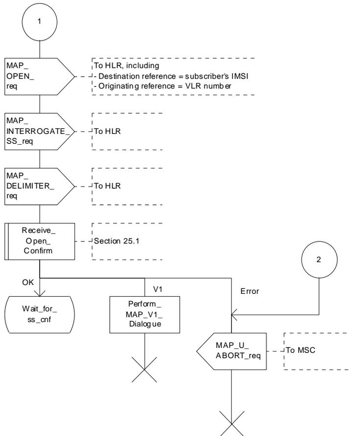
Figure 22.6.3/1 (sheet 2 of 3): Procedure Interrogate\_SS\_VLR
