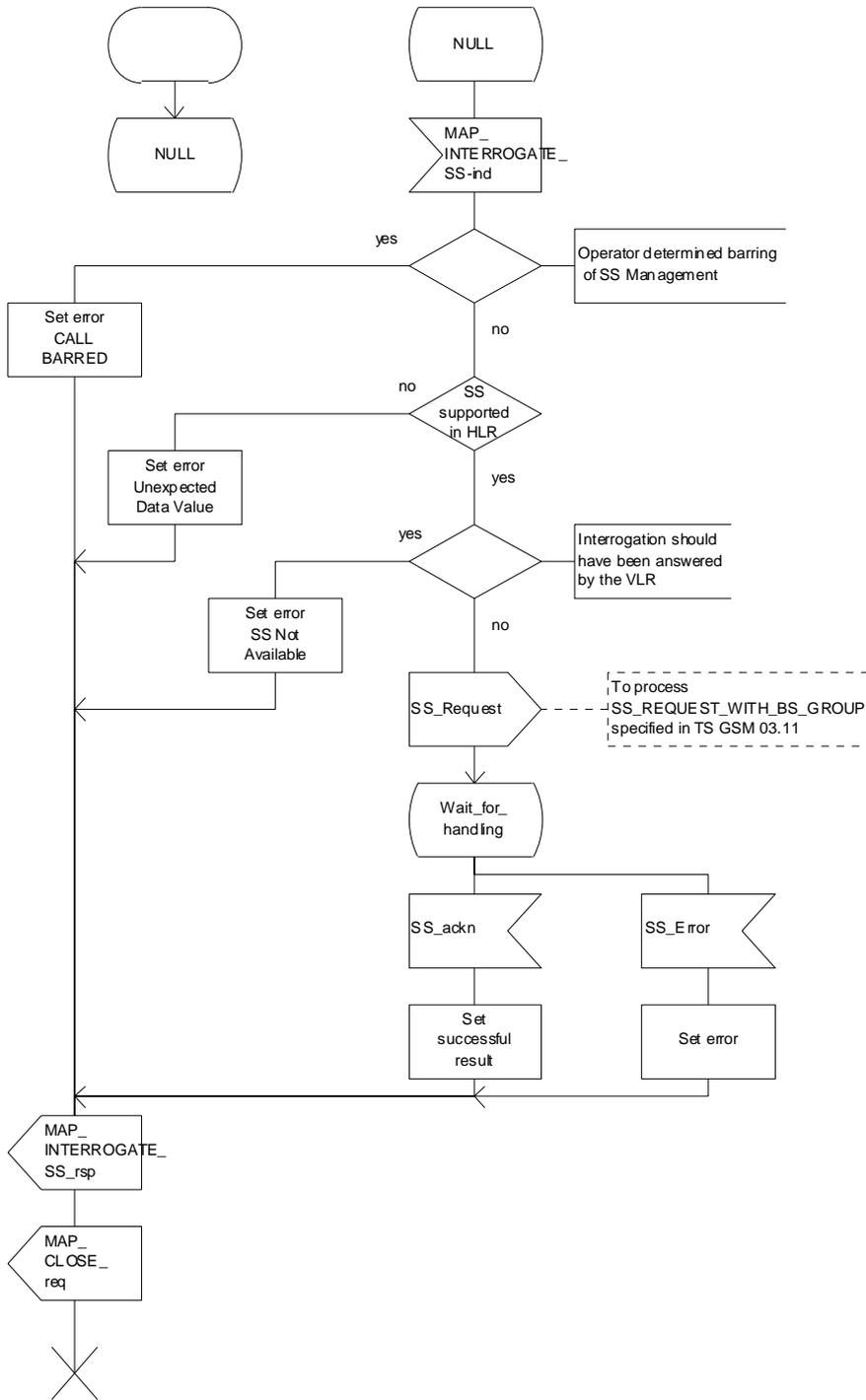
Figure 22.6.4/1: Procedure Interrogate\_SS\_HLR
