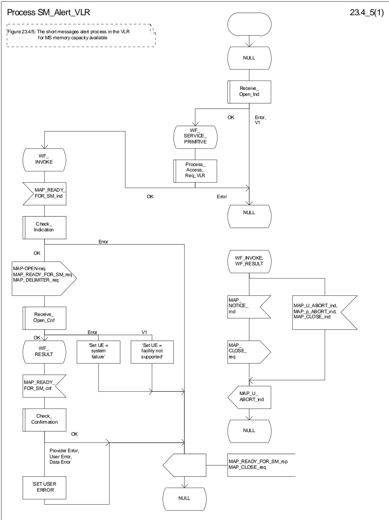
Figure 23.4/5: Procedure SM\_Alert\_VLR
