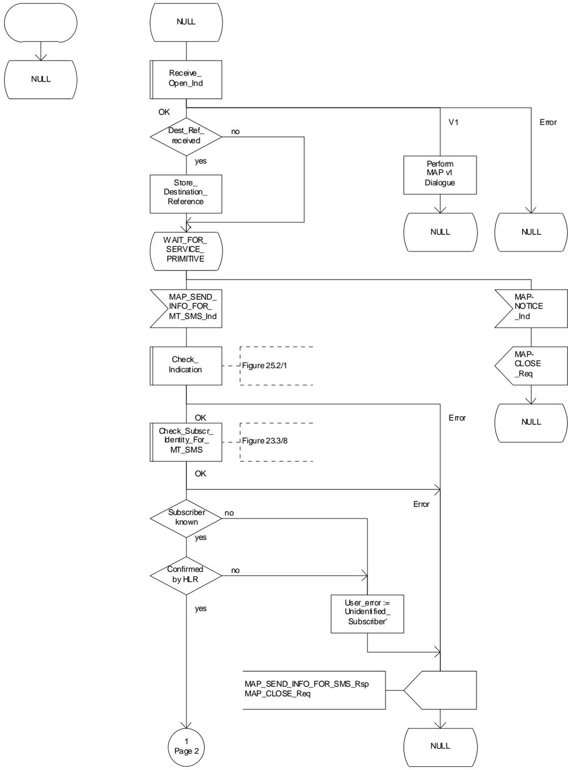
Figure 23.3/5 (sheet 1 of 3): Process MT\_SM\_VLR
