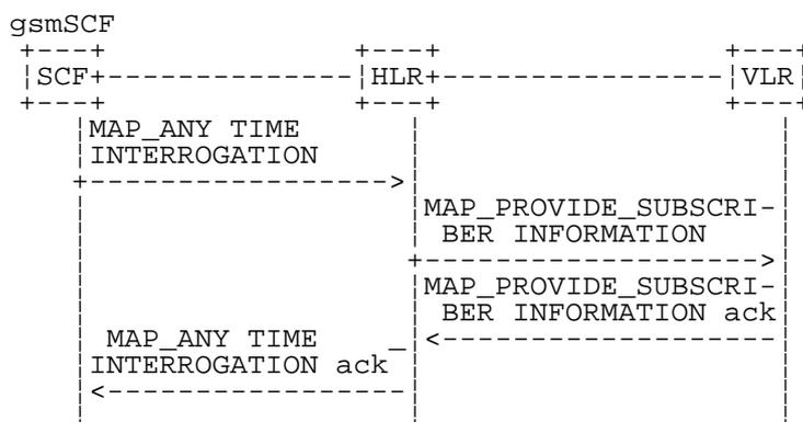
**Figure 21.2/8: Message flow for any time interrogation**
