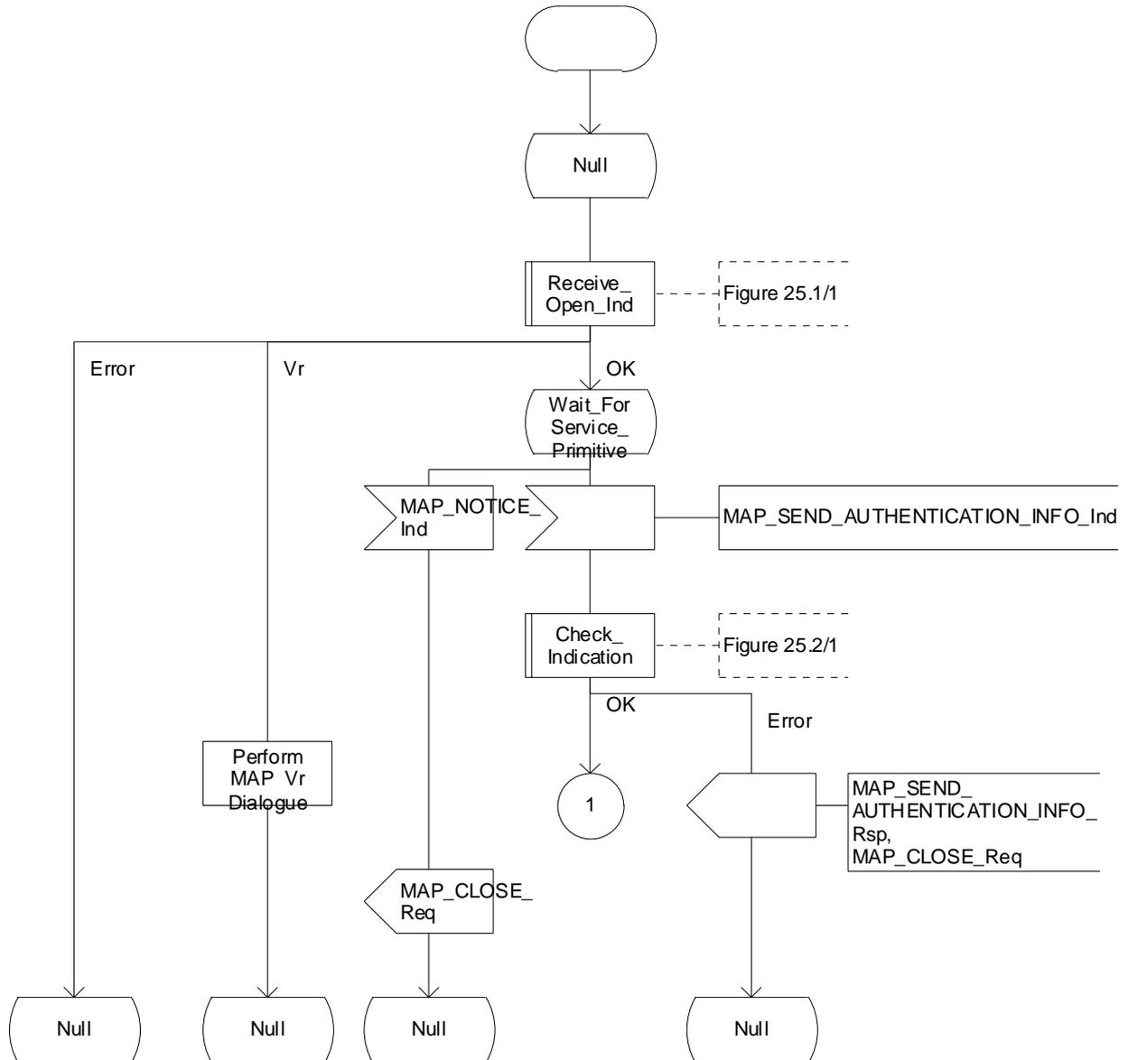
Figure 25.5/5 (sheet 1 of 2): Process Obtain\_Auth\_Sets\_HLR
