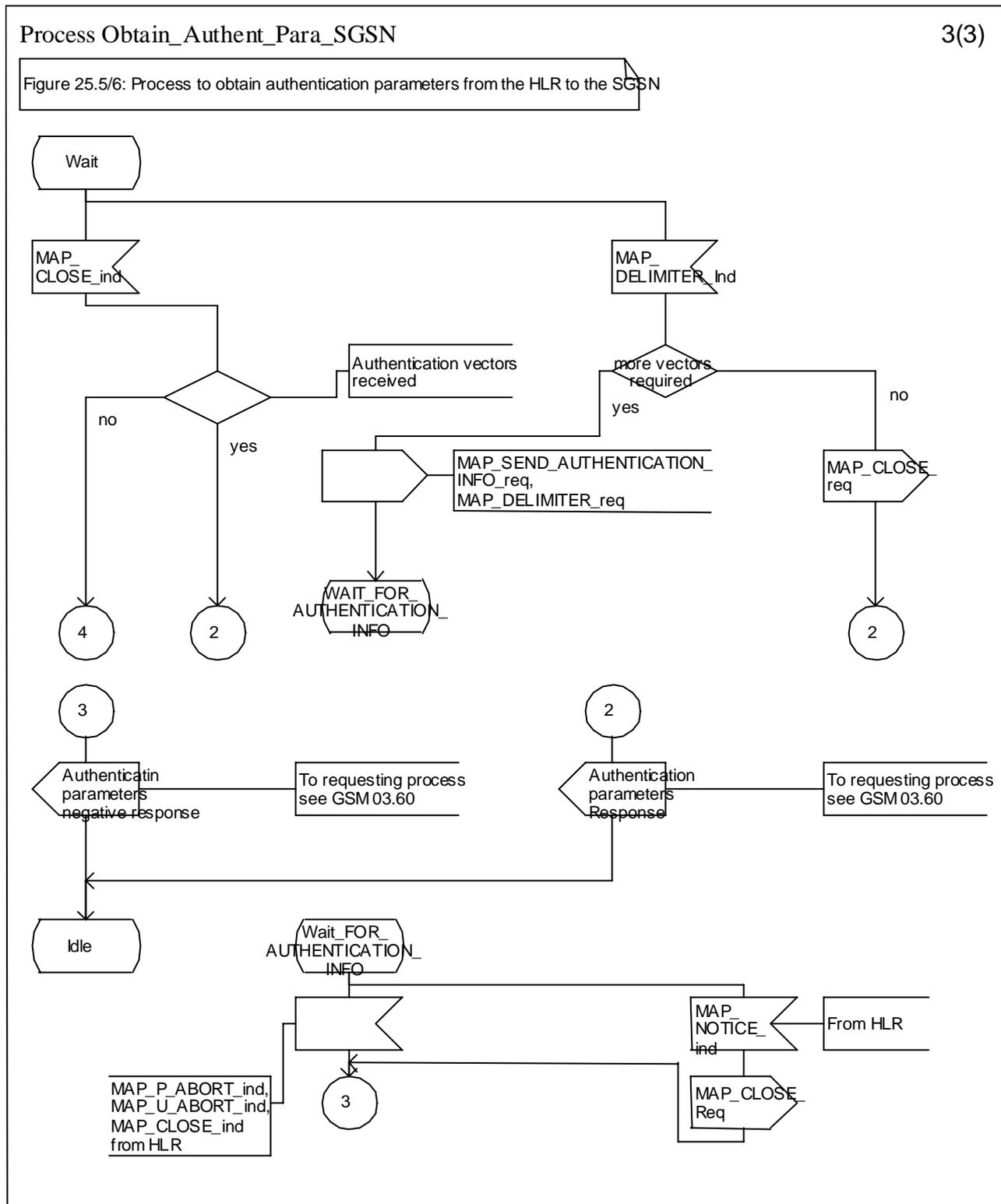
Figure 25.5/6 (sheet 3 of 3): Process Obtain\_Authent\_Para\_SGSN
