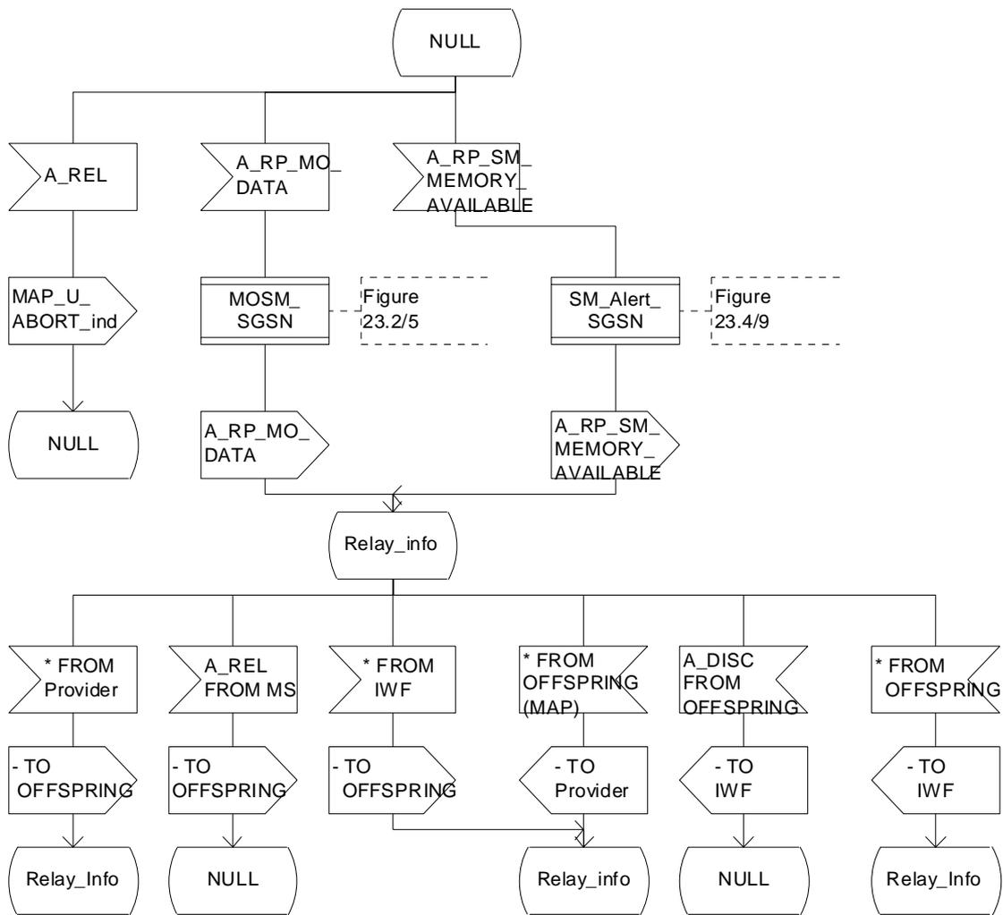
Figure 23.1/3: Process Co\_SMS\_SGSN
