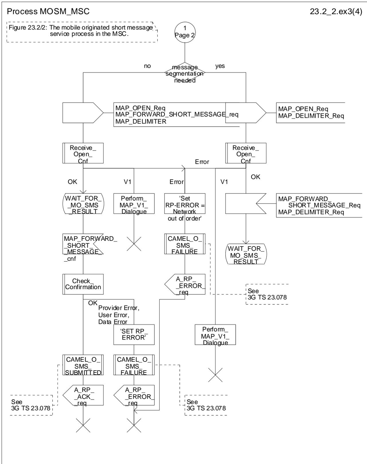
Figure 23.2/2 (sheet 4 of 4): Process MOSM\_MSC
