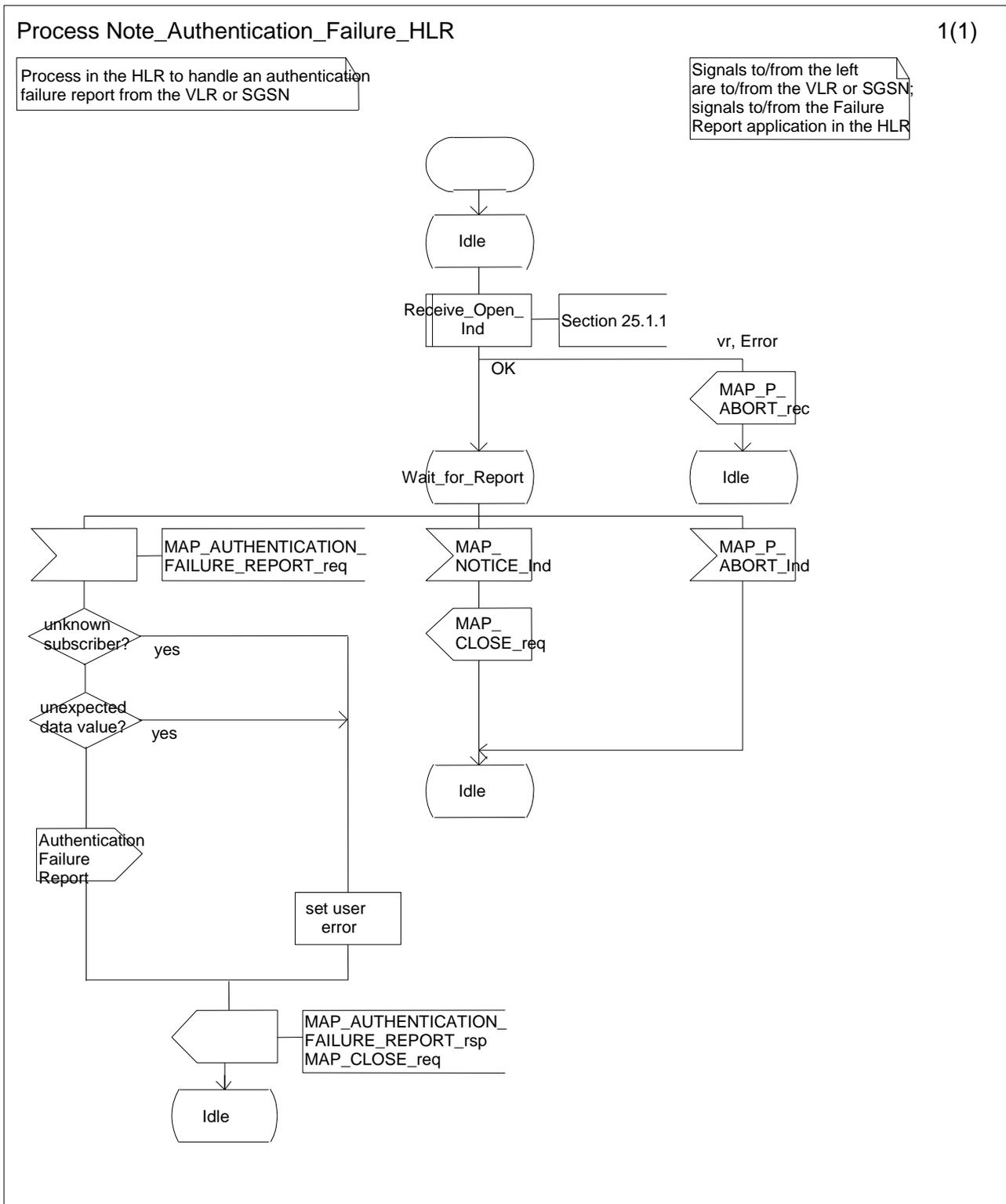
Figure 25.6/10: Process Note\_Authentication\_Failure\_HLR
