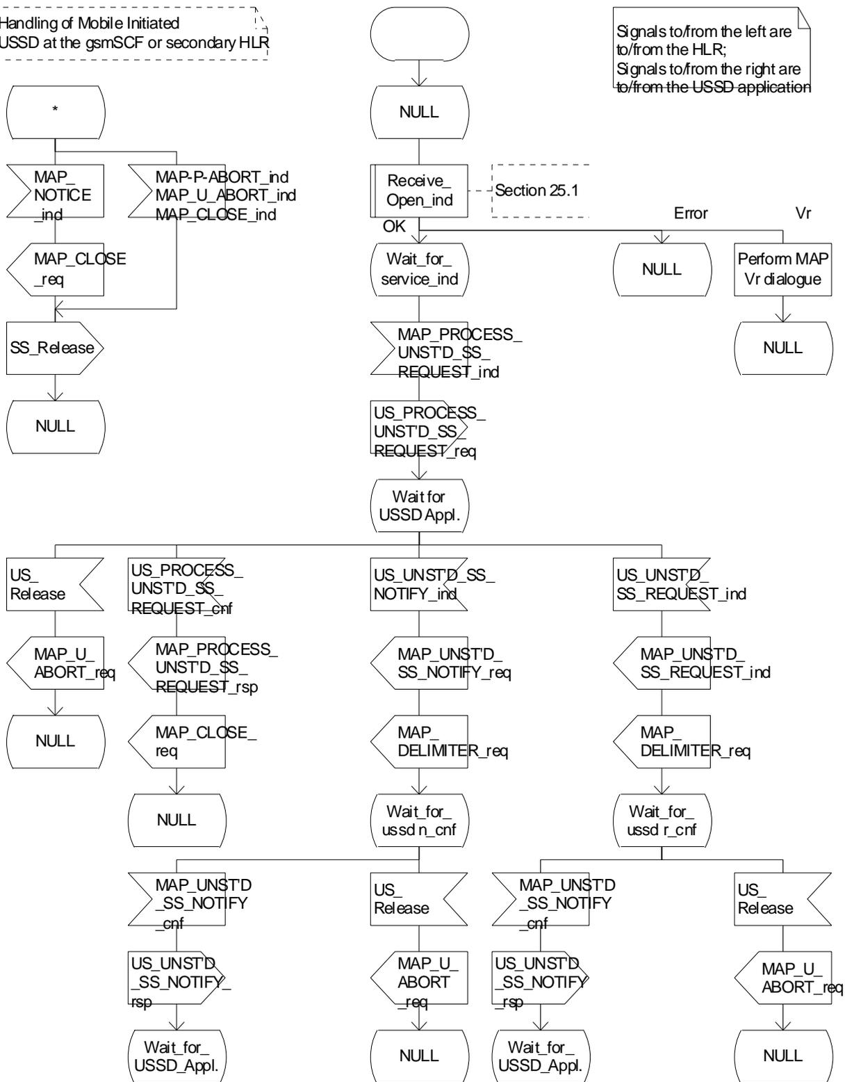
**Figure 22.9.5/1 Process MS\_INIT\_USSD\_gsmSCF\_secondary\_HLR**
