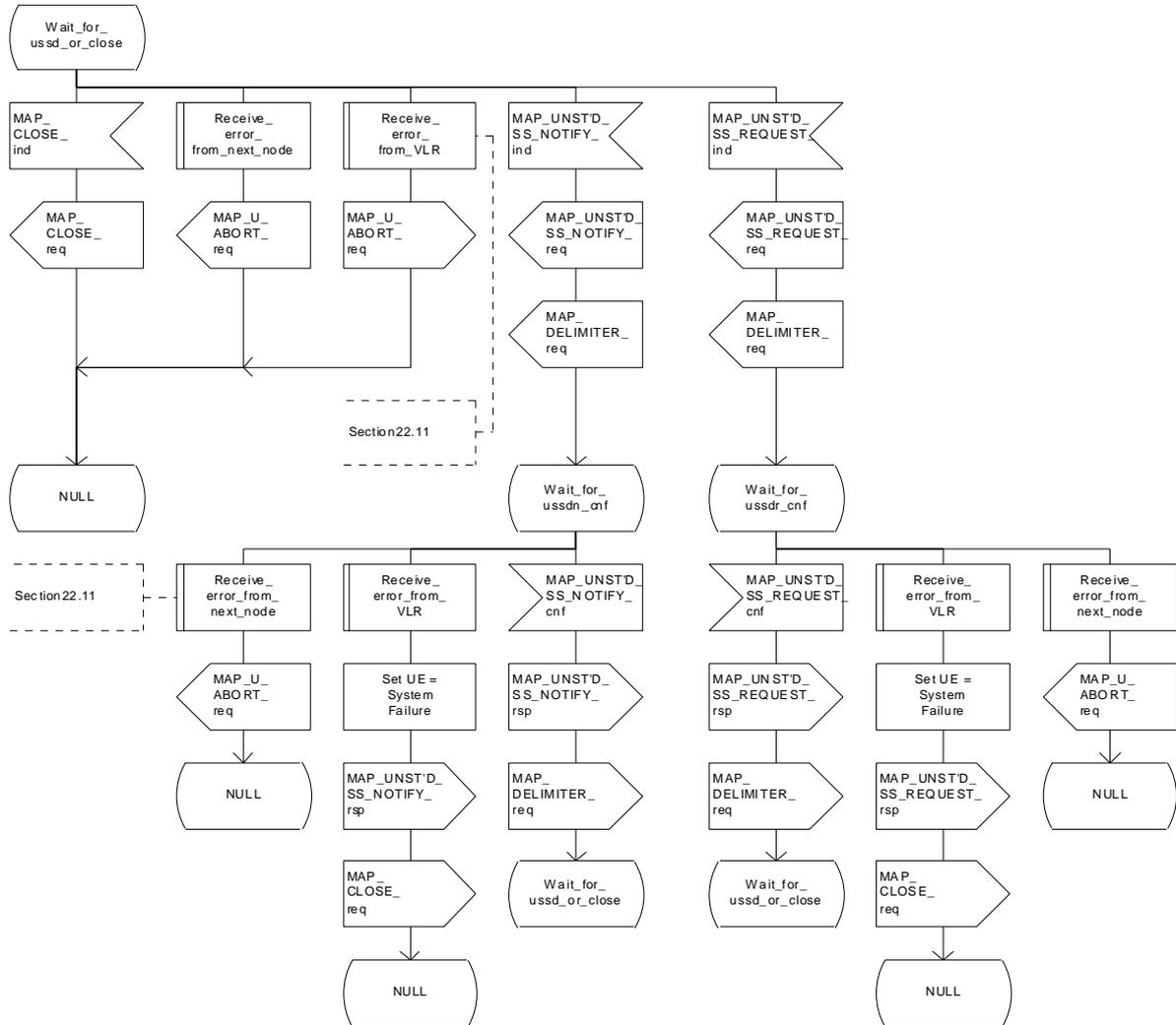
Figure 22.10.4/1 (sheet 3 of 5): Procedure NI\_USSD\_HLR
