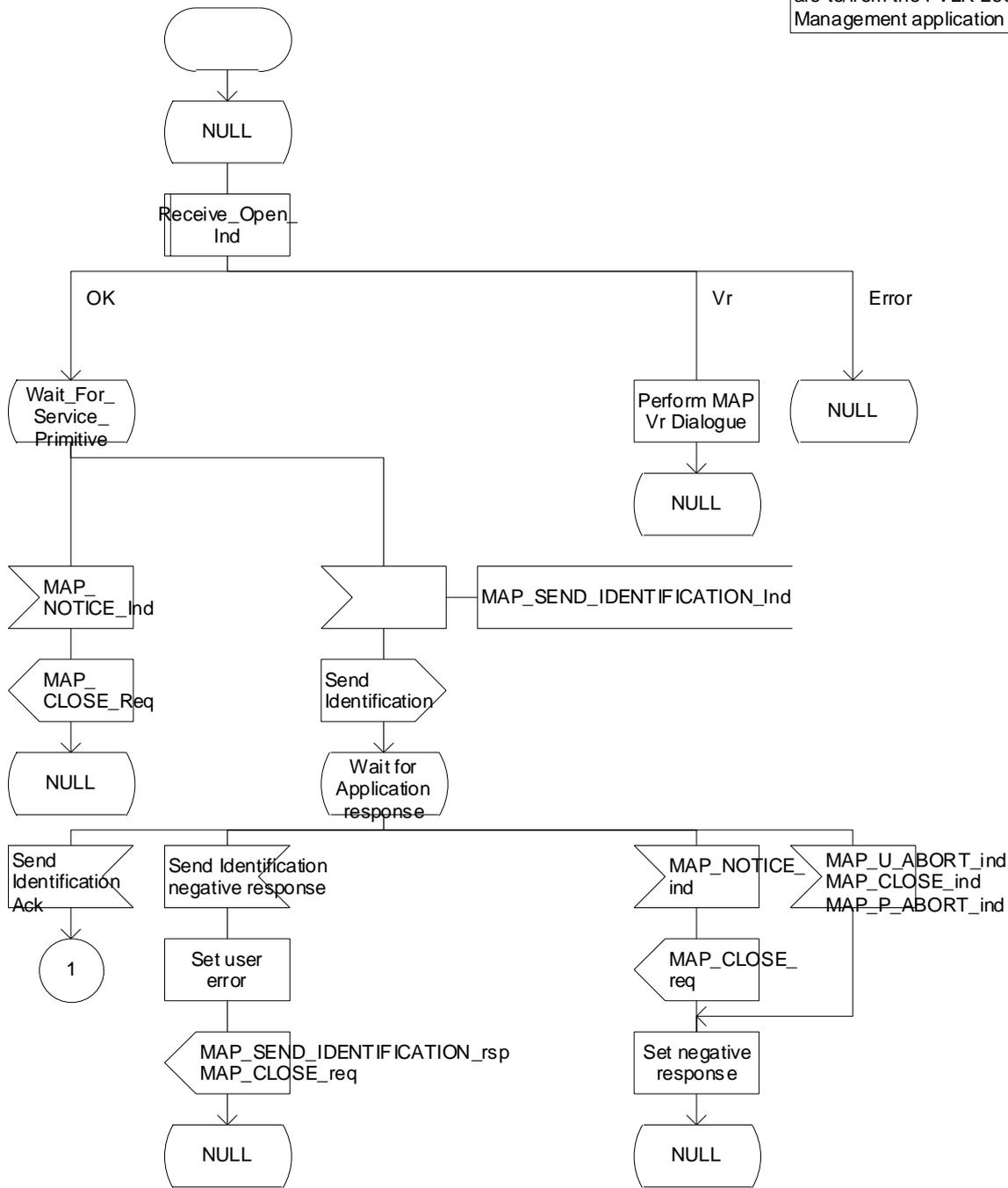
Figure 19.1.1/XX (sheet 1 of 2): Process Send\_Identification\_PVLR
