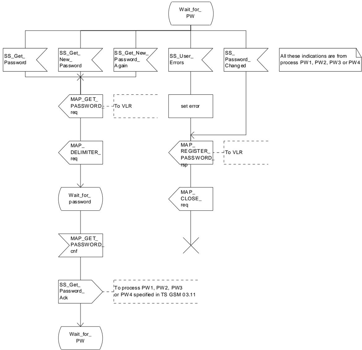
Figure 22.8.4/1 (sheet 2 of 2): Procedure Register\_PW\_HLR
