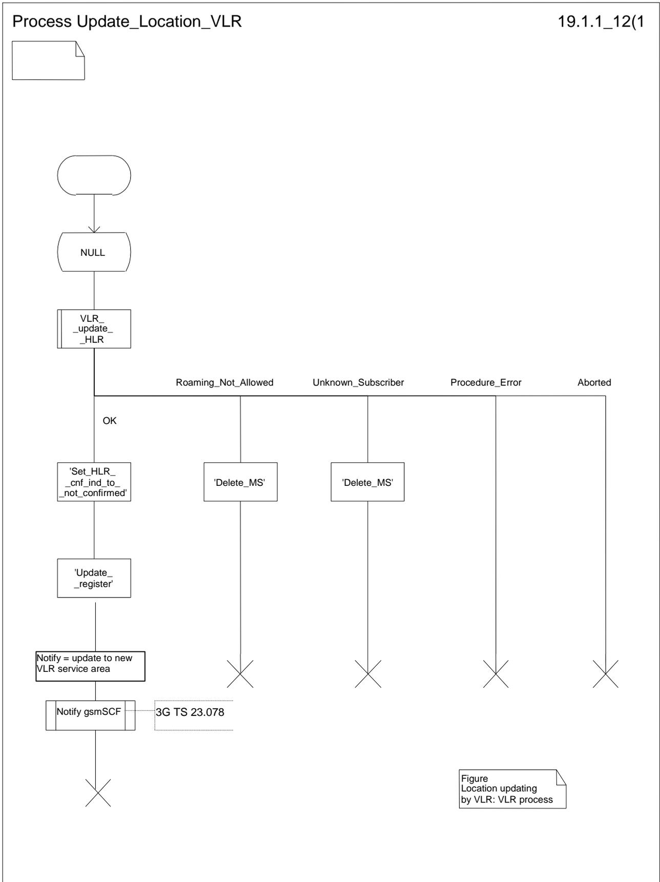
Figure 19.1.1/12: Process UL\_VLR
