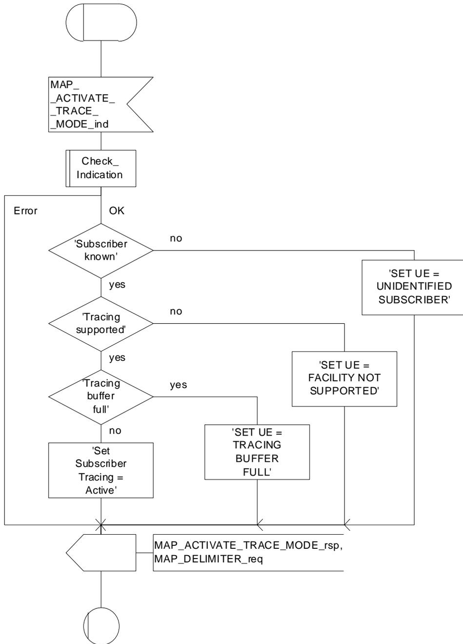
Figure 25.9/7: Macro Activate\_Tracing\_SGSN
