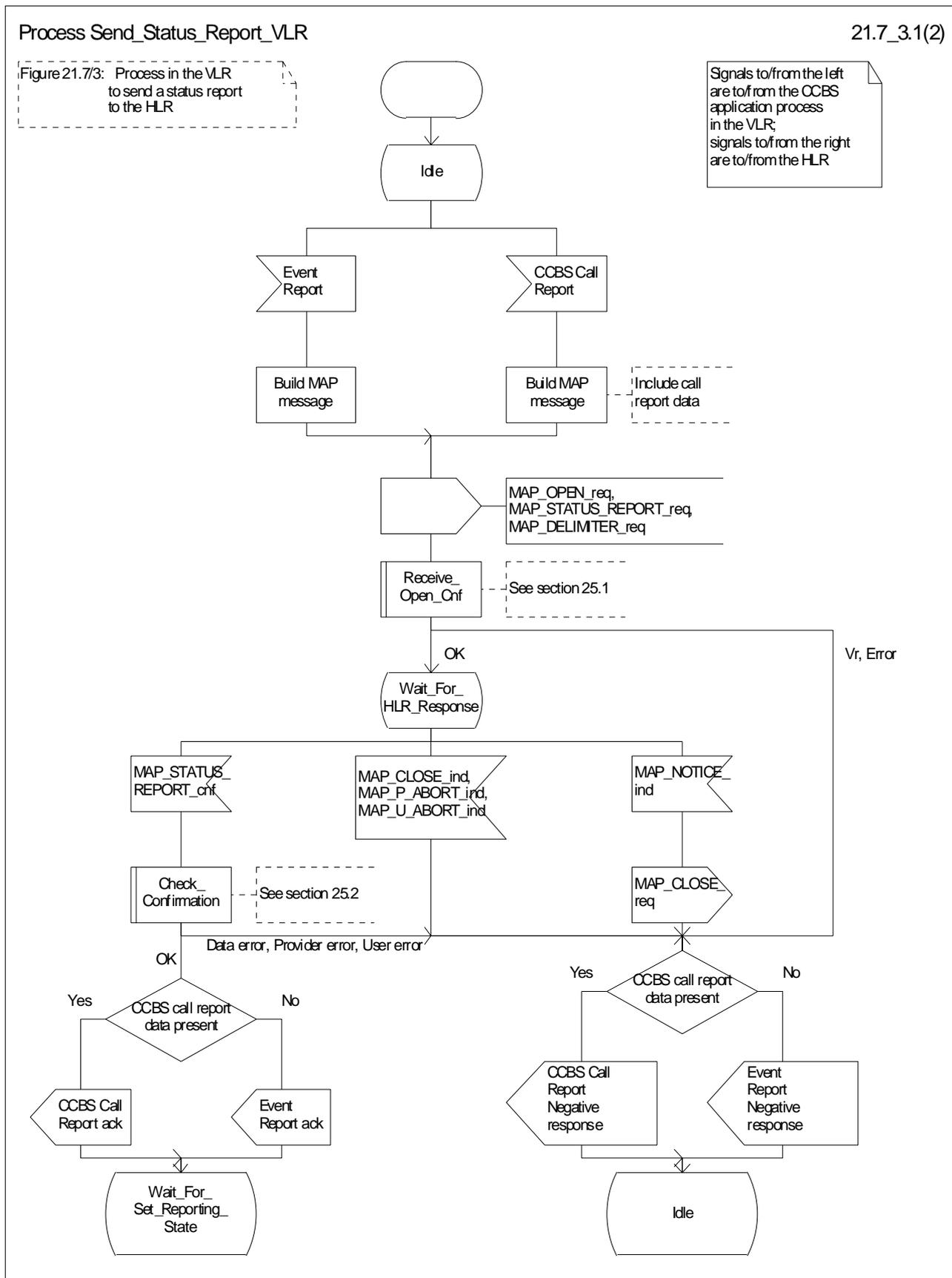
Figure 21.7/3 (sheet 1 of 2): Process Send\_Status\_Report\_VLR
