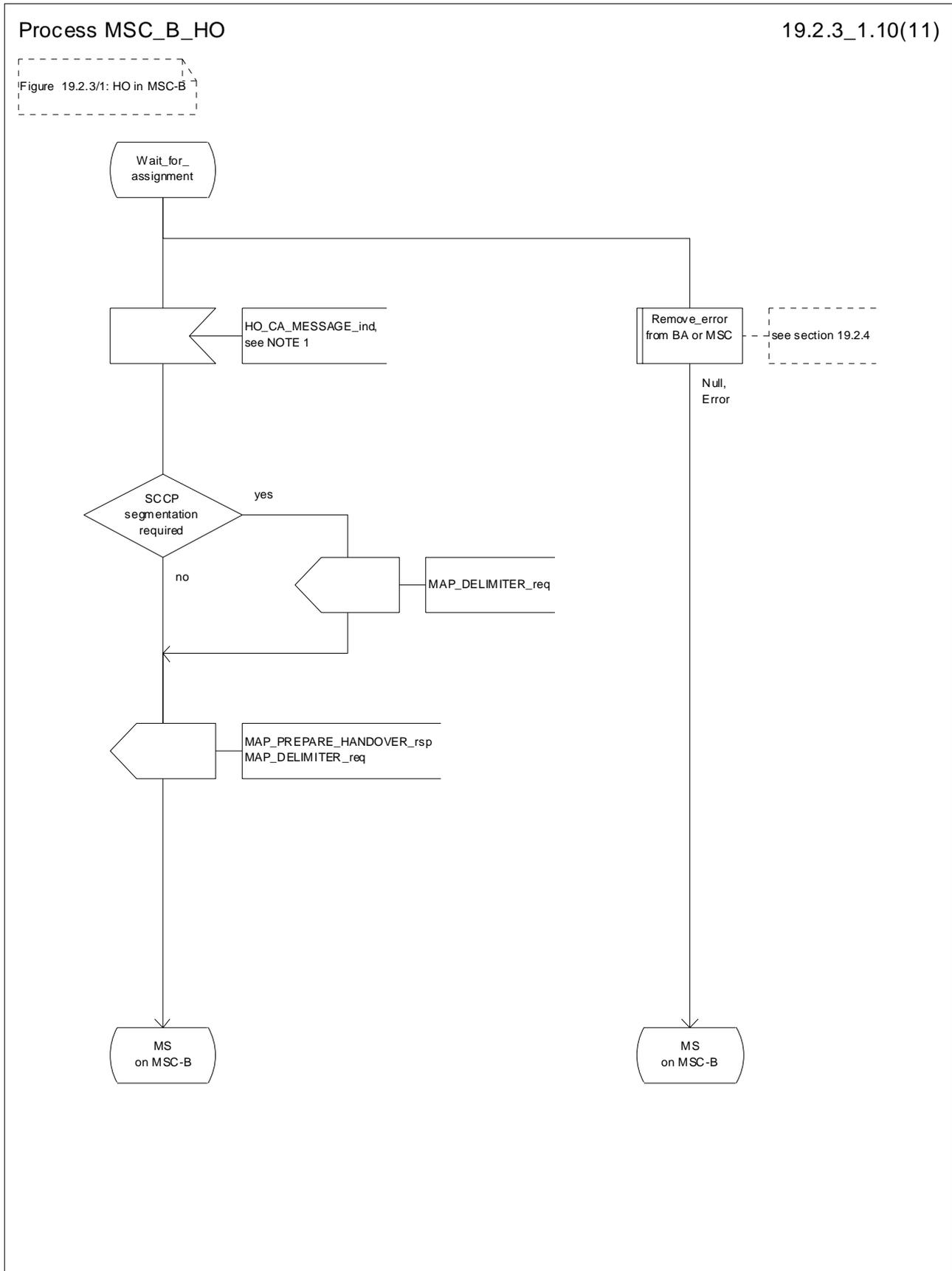
Figure 19.2.3/1 (sheet 10 of 11): Process MSC\_B\_HO
