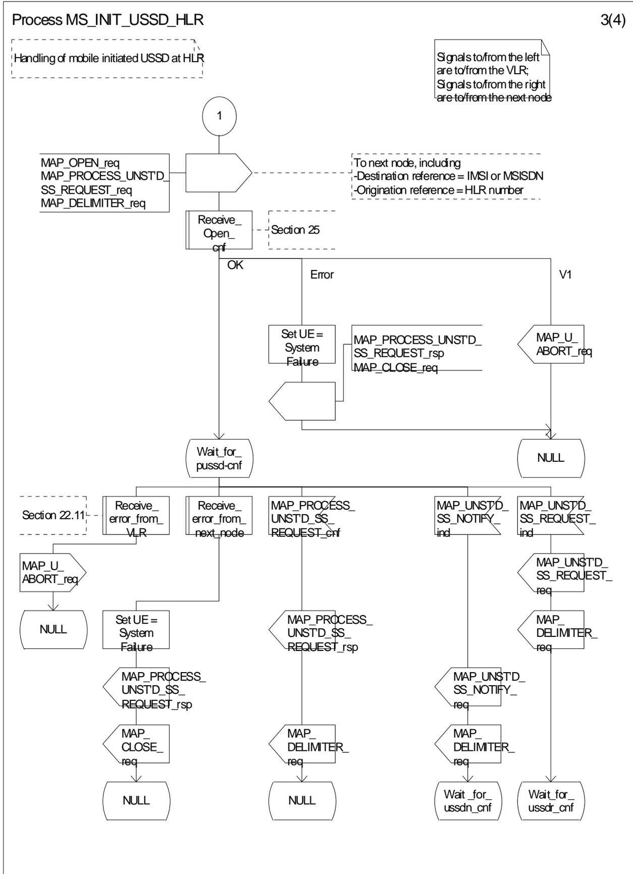
Figure 22.9.4/1 (sheet 3 of 4): Procedure MI\_USSD\_HLR
