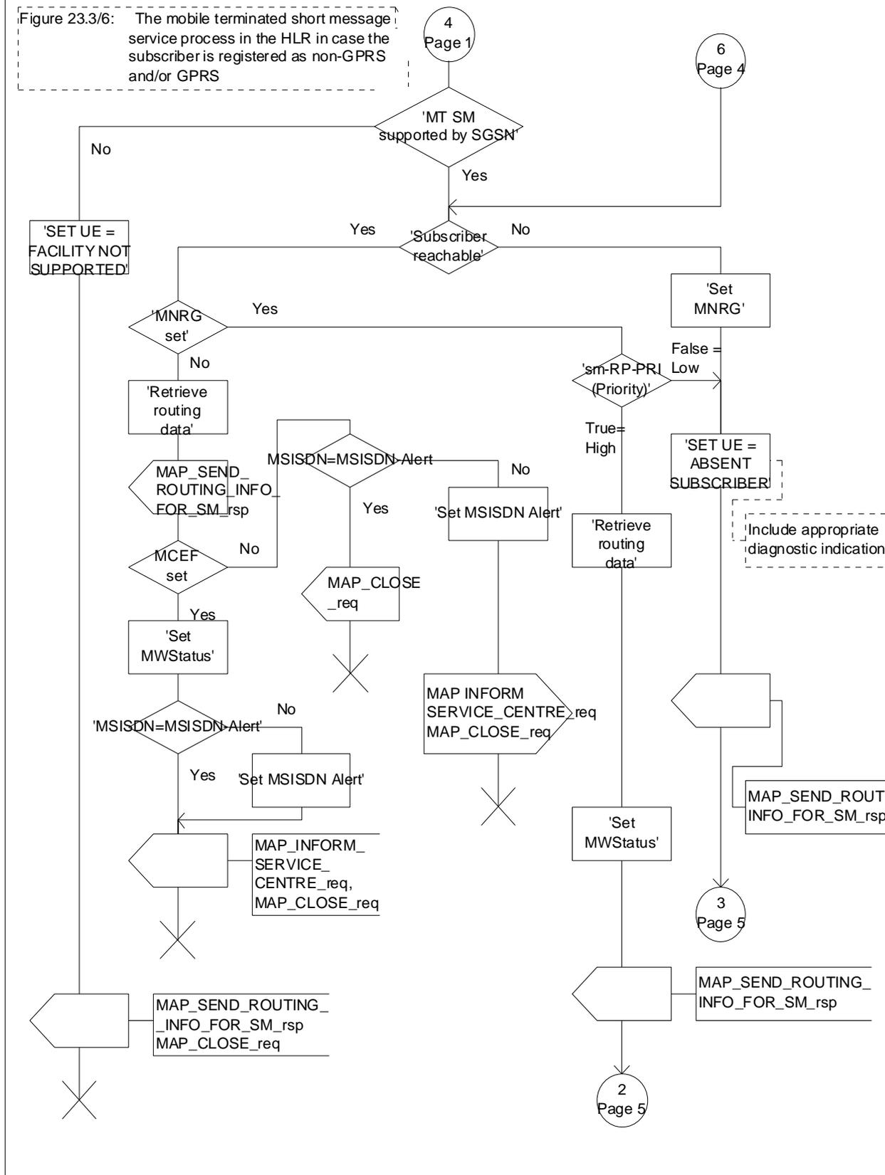
Figure 23.3/6 (sheet 3 of 5): Process Mobile\_terminated\_SM\_HLR
