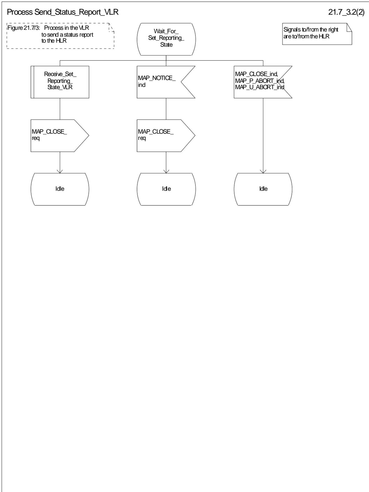
Figure 21.7/3 (sheet 2 of 2): Process Send\_Status\_Report\_VLR
