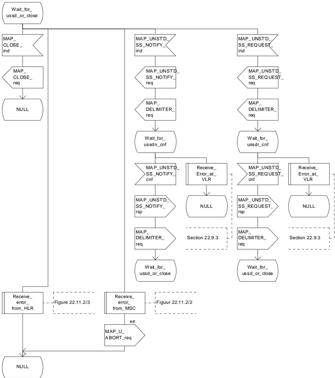
Figure 22.10.3/1 (sheet 2 of 4): Procedure NI\_USSD\_VLR
