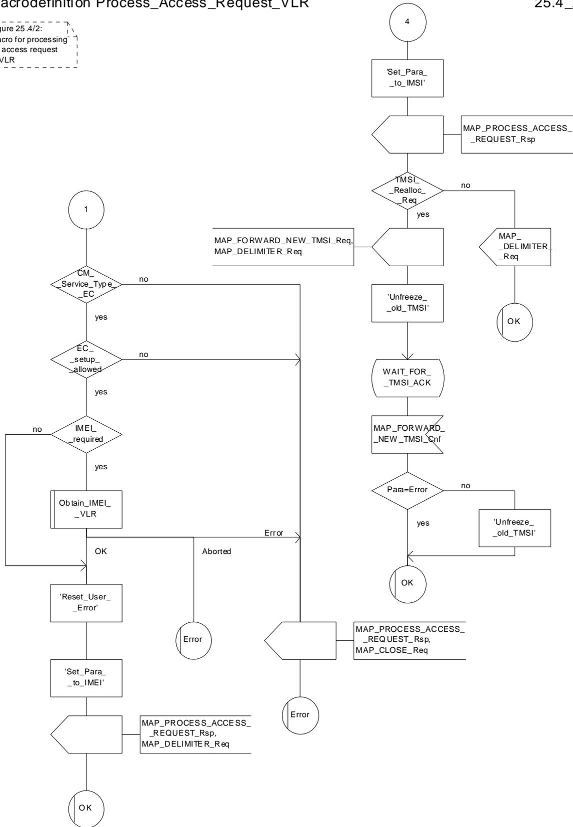
Figure 25.4/2 (sheet 3 of 3): Macro Process\_Access\_Request\_VLR
