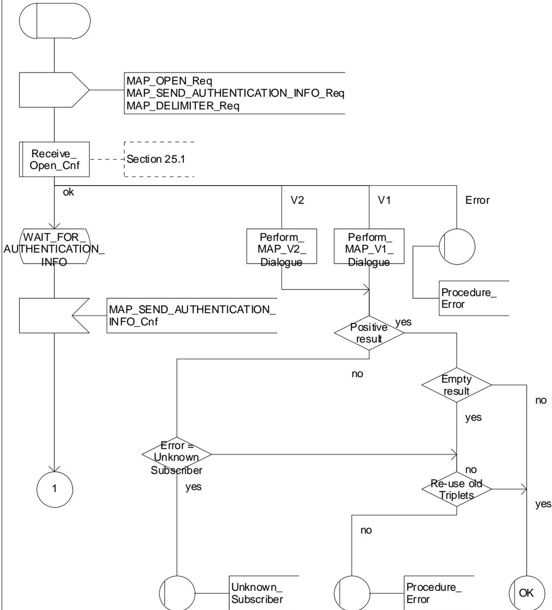
Figure 25.5/4 (sheet 1 of 3): Macro Obtain\_Authent\_Para\_VLR
