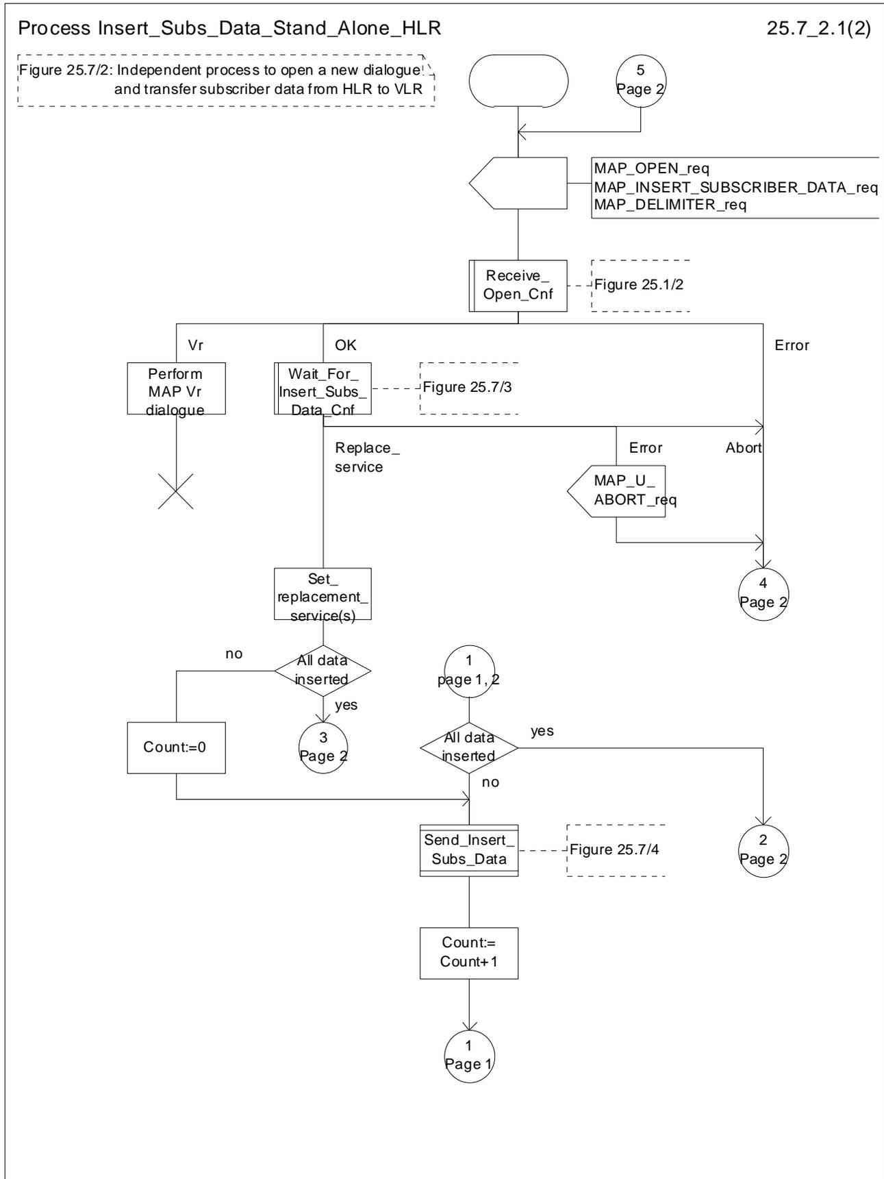
Figure 25.7/2 (sheet 1 of 2): Process Insert\_Subs\_Data\_Stand\_Alone\_HLR
