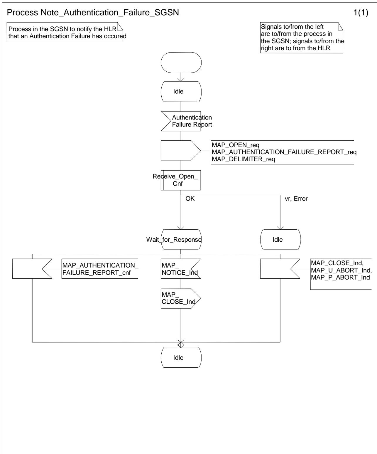
Figure 25.6/9: Process Note\_Authentication\_Failure\_SGSN
