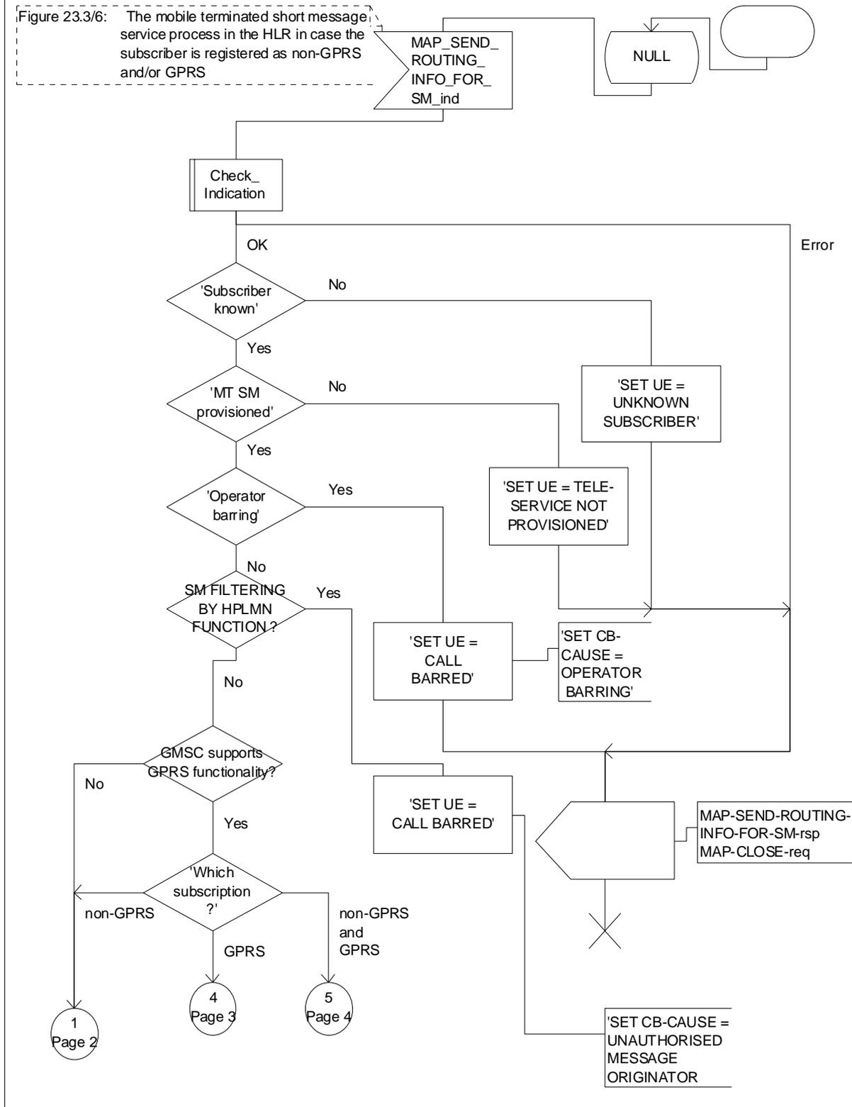
Figure 23.3/6 (sheet 1 of 5): Process Mobile\_terminated\_SM\_HLR
