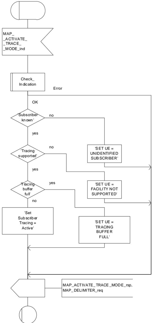
Figure 25.9/3: Macro Activate\_Tracing\_VLR
