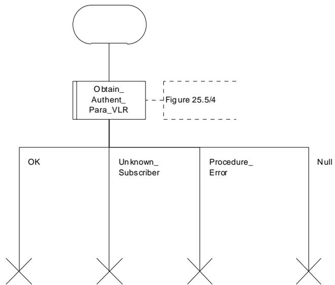
Figure 25.5/3: Process Obtain\_Authentication\_Sets\_VLR
