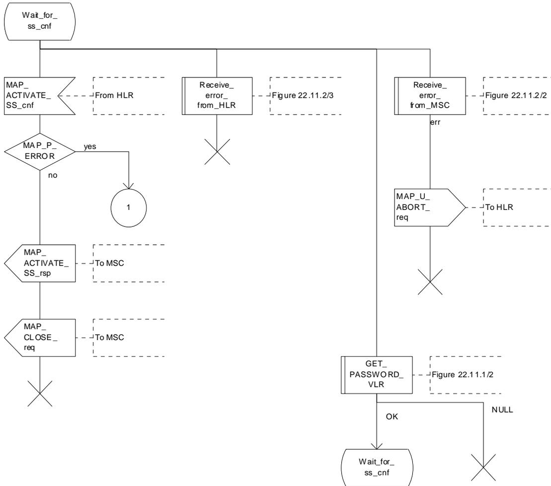
Figure 22.4.3/1 (sheet 2 of 2): Procedure SS\_Activate\_VLR
