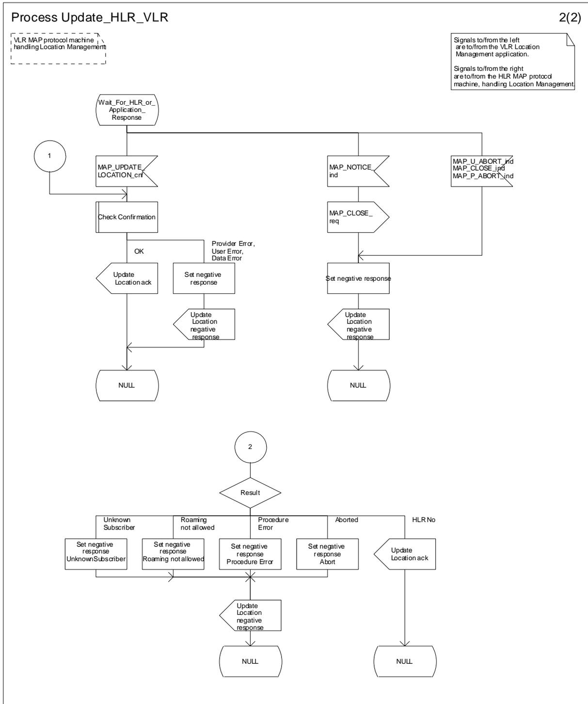
Figure 19.1.1/6 (sheet 2 of 2): Process Update\_HLR\_VLR
