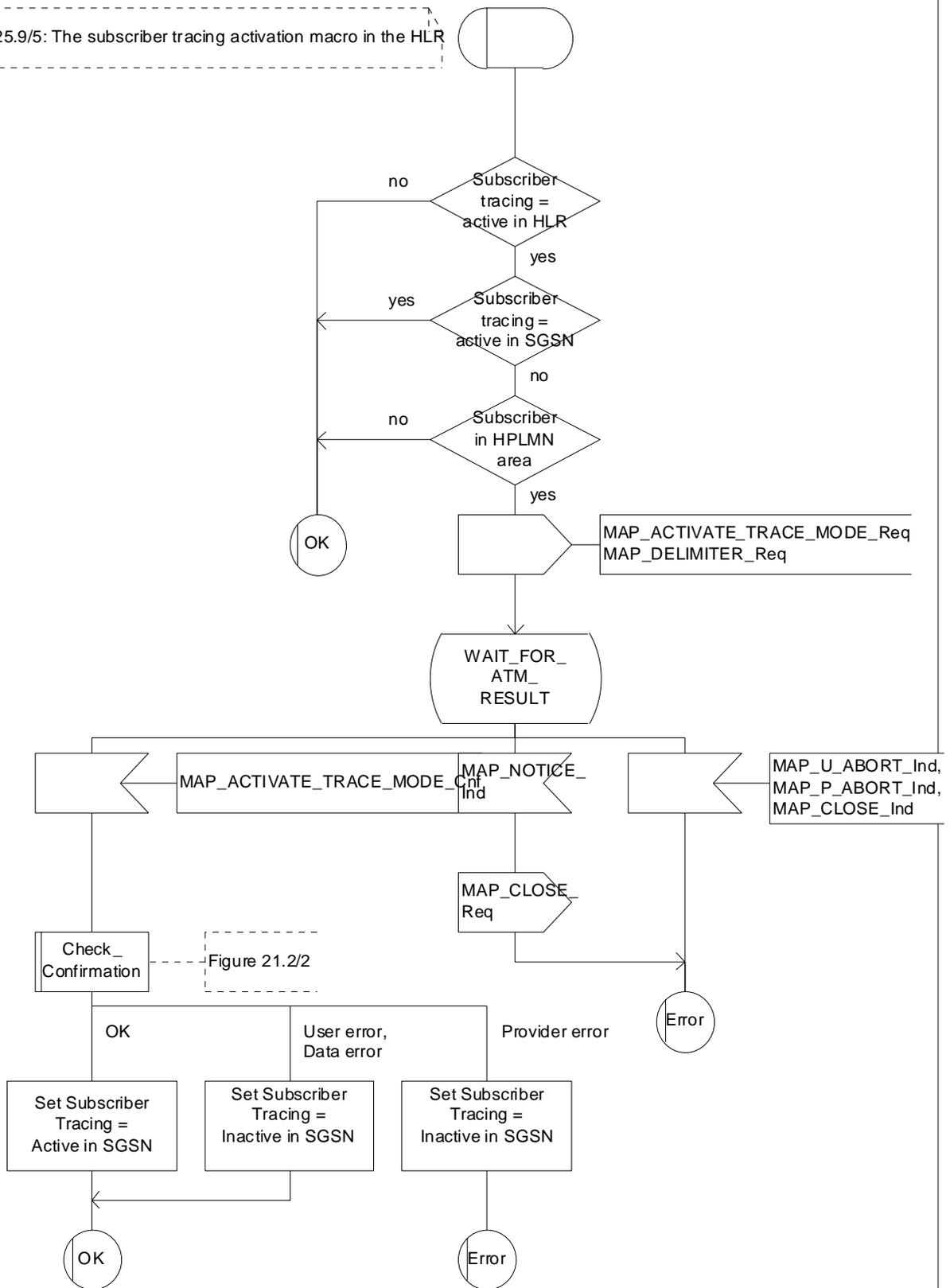
Figure 25.9/5: Macro Control\_Tracing\_HLR\_with\_SGSN
