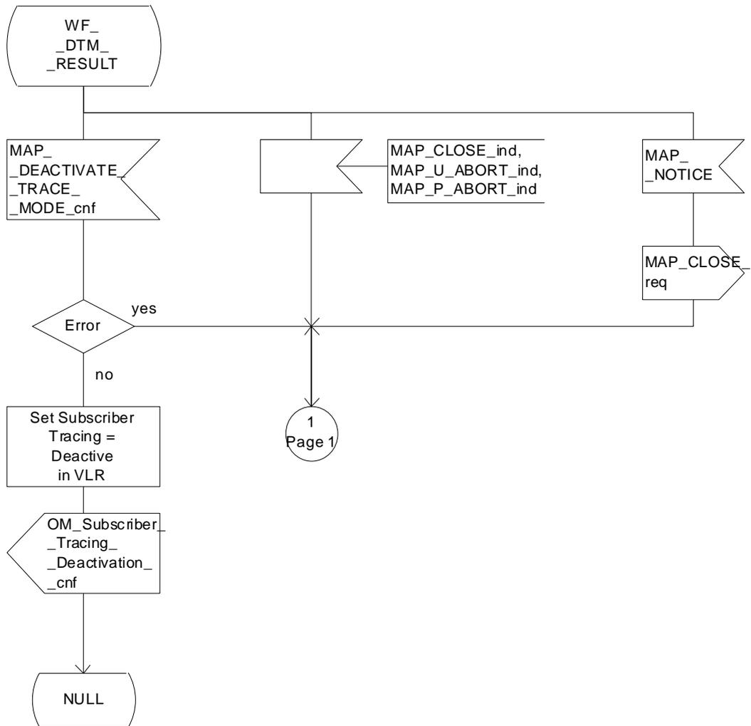
Figure 20.2/8 (sheet 2 of 2): Process DTM\_HLR\_with\_VLR
