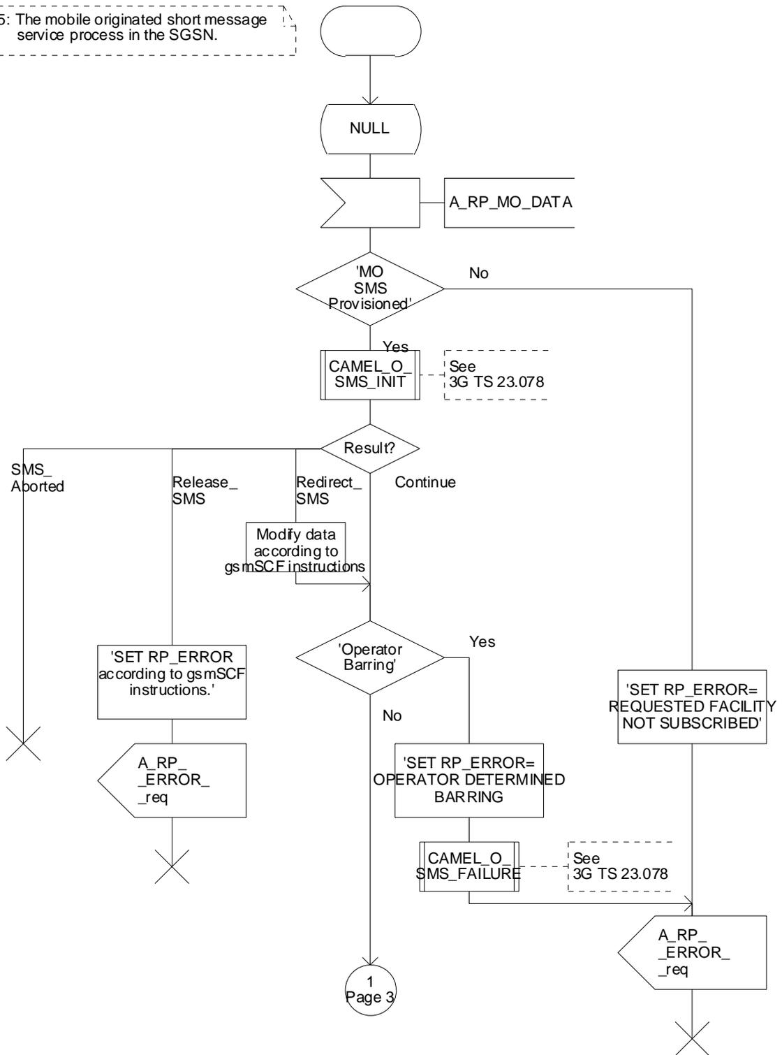
Figure 23.2/5 (sheet 1 of 3): Process MOSM\_SGSN
