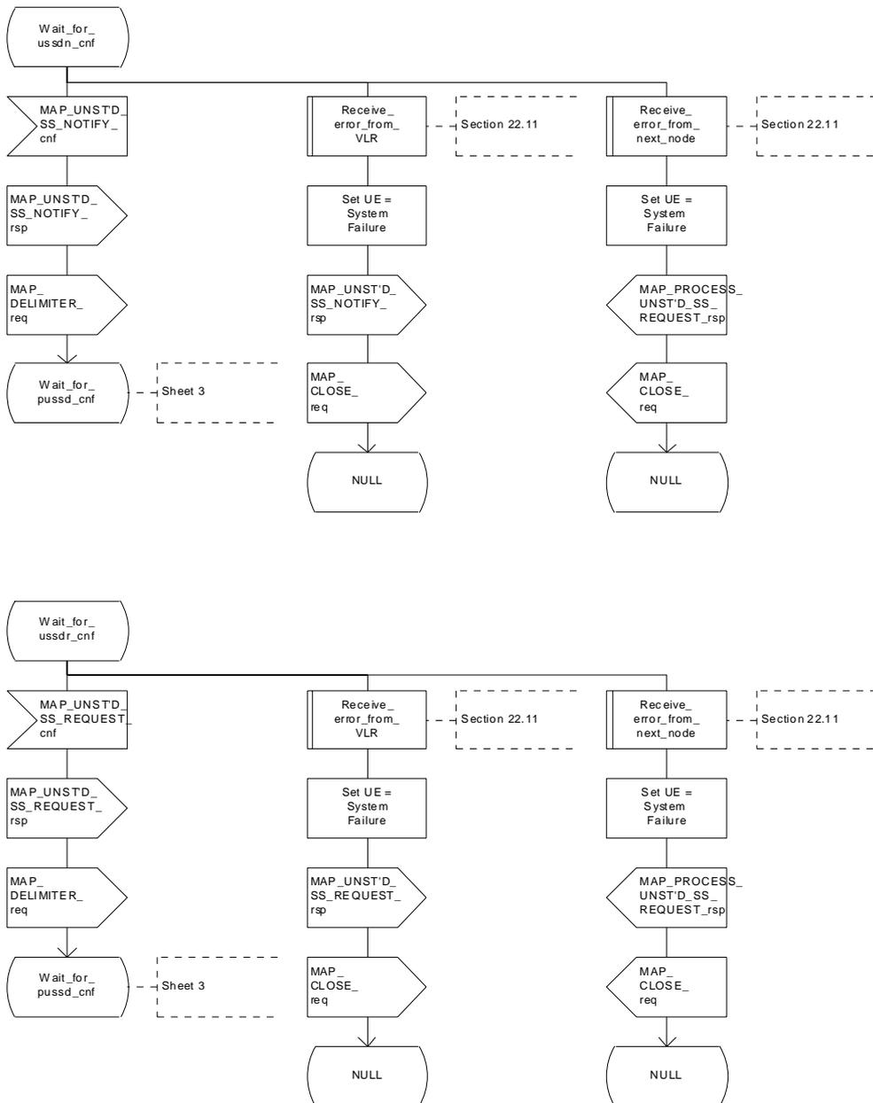
Figure 22.9.4/1 (sheet 4 of 4): Procedure MI\_USSD\_HLR
