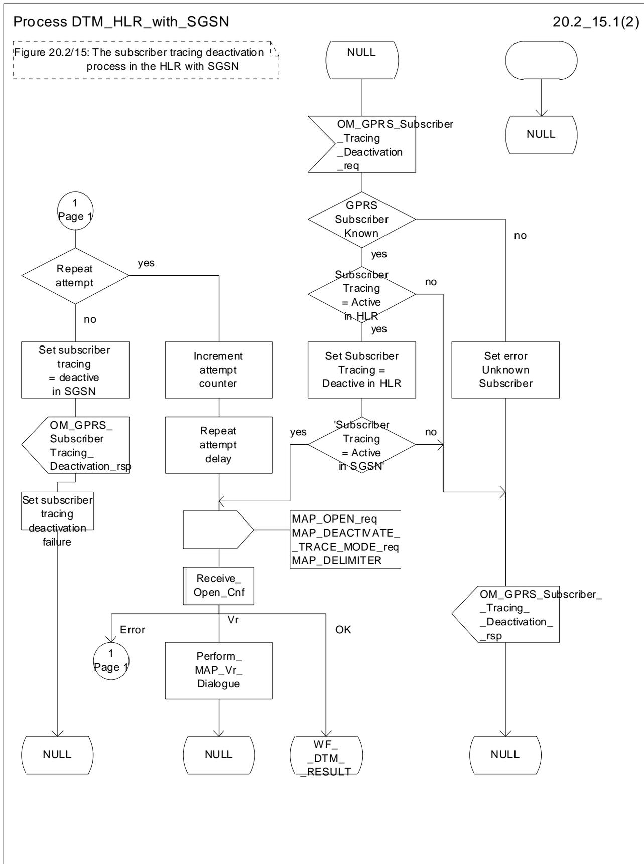
Figure 20.2/15 (sheet 1 of 2): Process DTM\_HLR\_with\_SGSN
