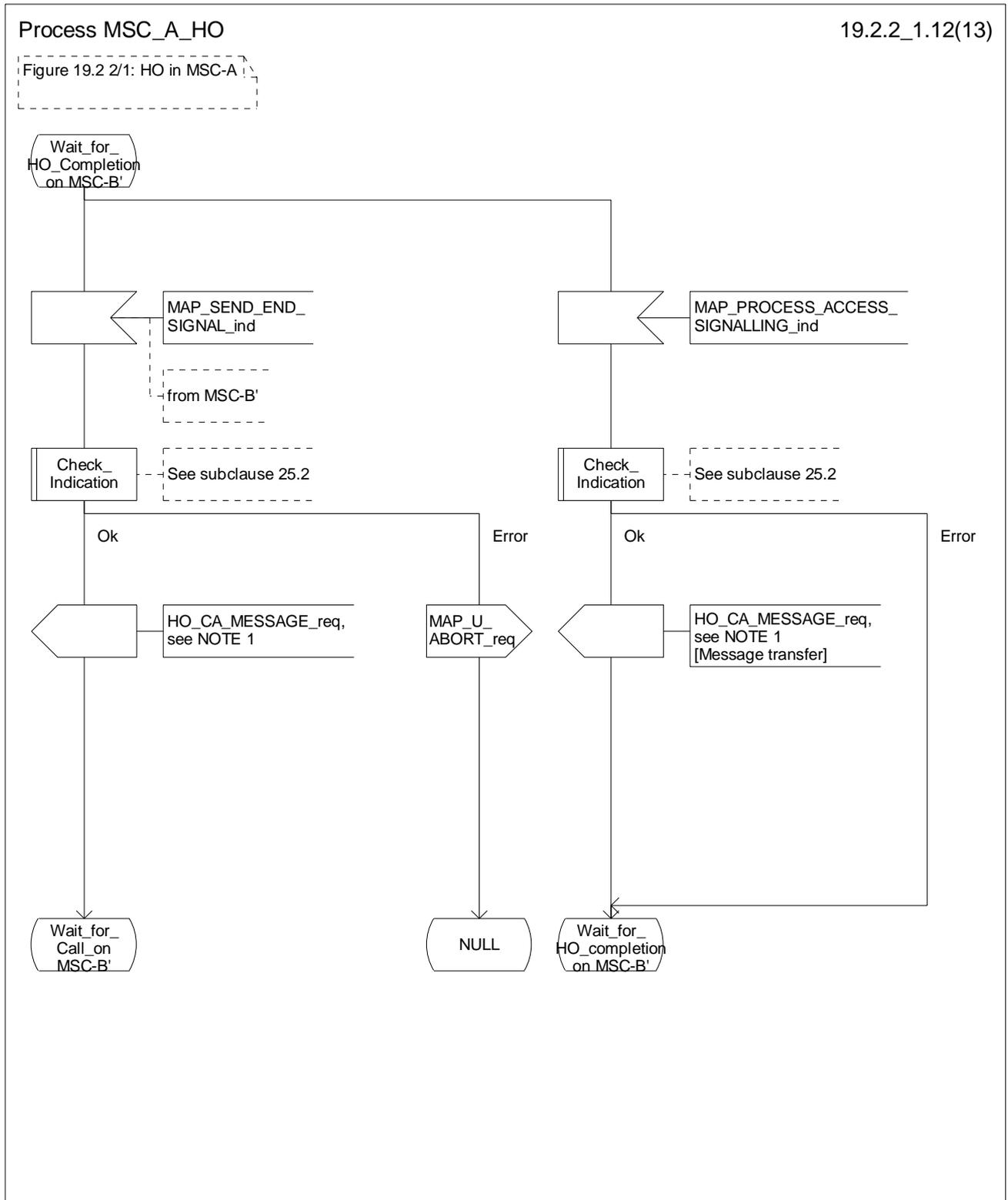
Figure 19.2.2/1 (sheet 12 of 13): Process MSC\_A\_HO
