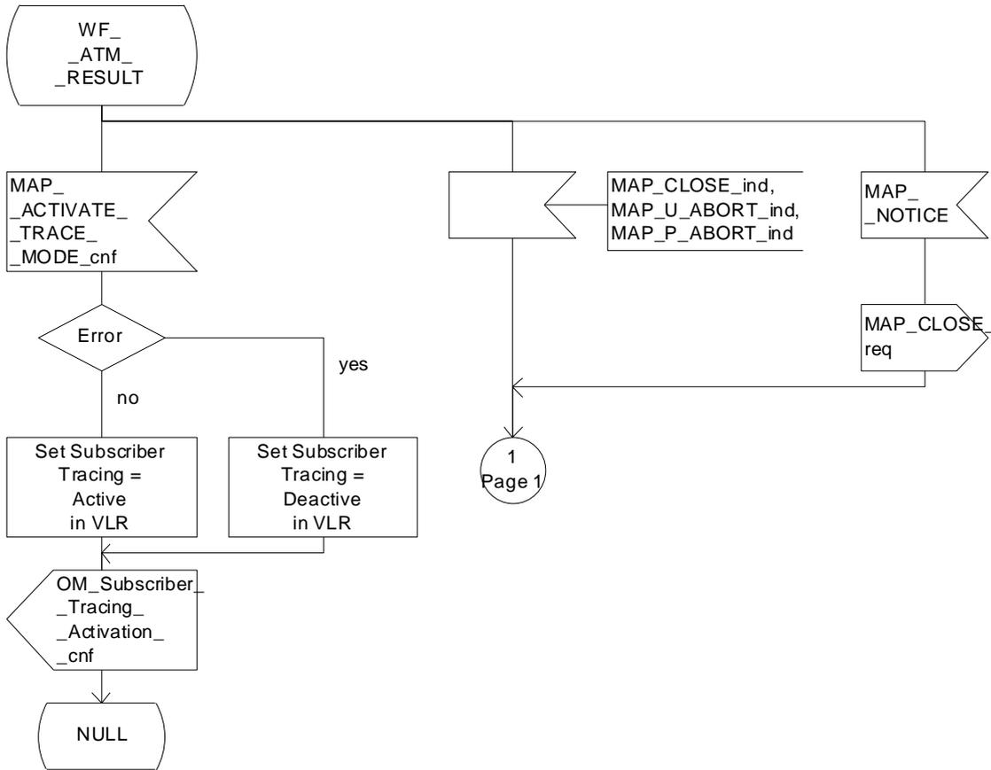
Figure 20.2/7 (sheet 2 of 2): Process ATM\_HLR\_with\_VLR
