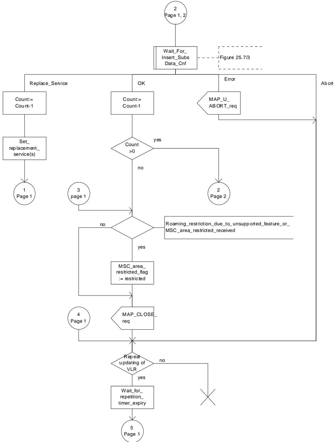
Figure 25.7/2 (sheet 2 of 2): Process Insert\_Subs\_Data\_Stand\_Alone\_HLR
