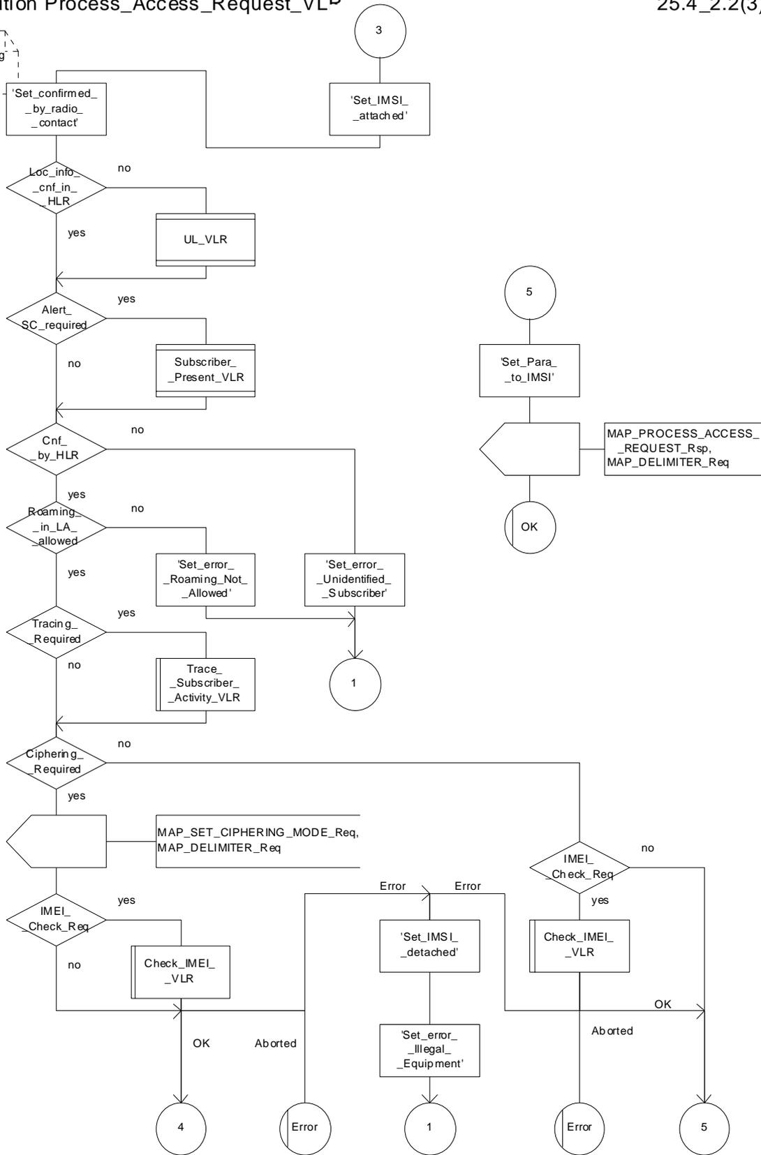
Figure 25.4/2 (sheet 2 of 3): Macro Process\_Access\_Request\_VLR
