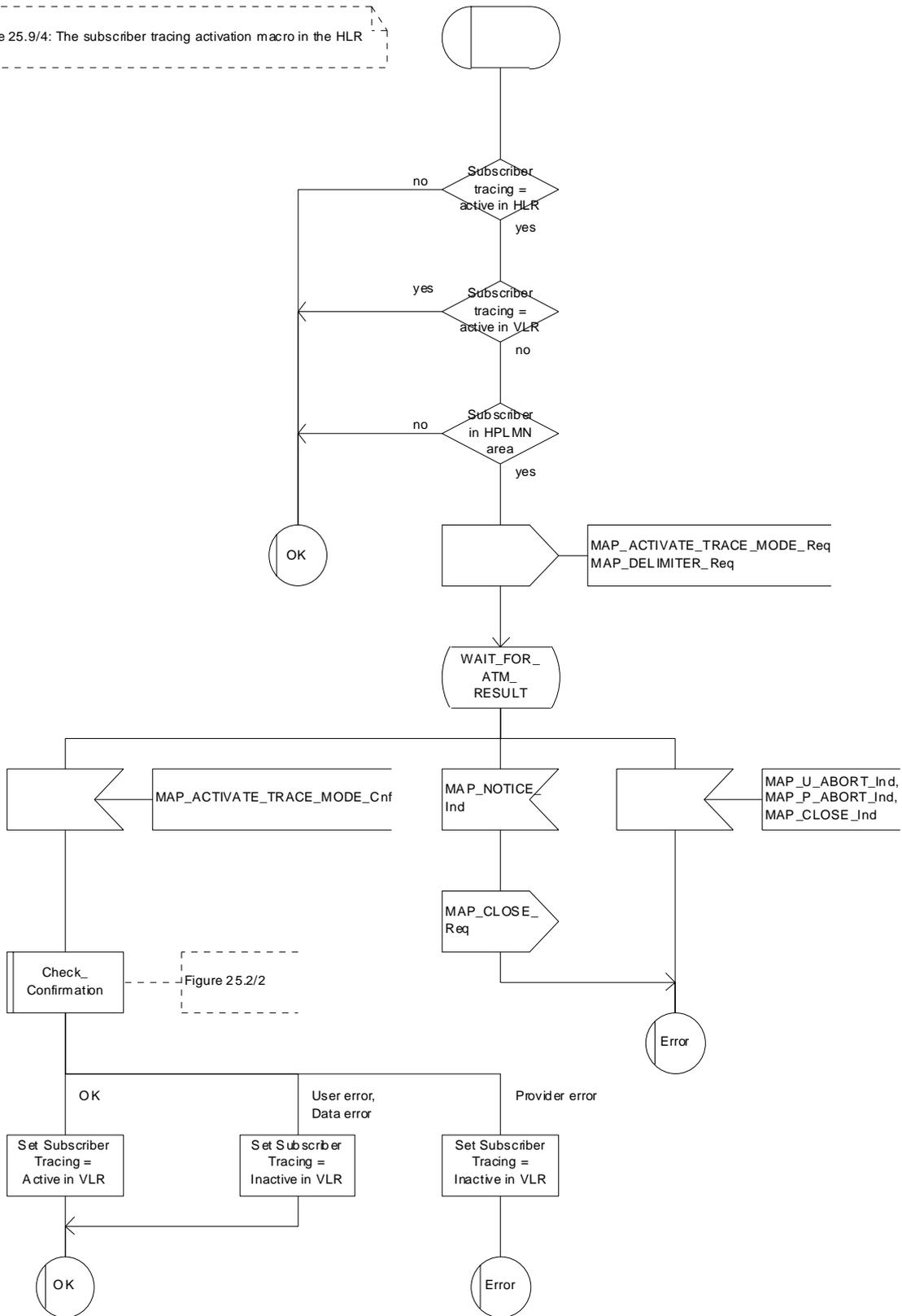
Figure 25.9/4: Macro Control\_Tracing\_HLR
