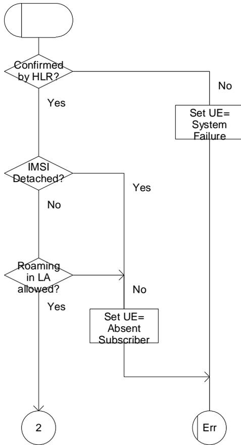
Figure 22.10.3/2 (sheet 1 of 2): Macro Start\_USSD\_VLR
