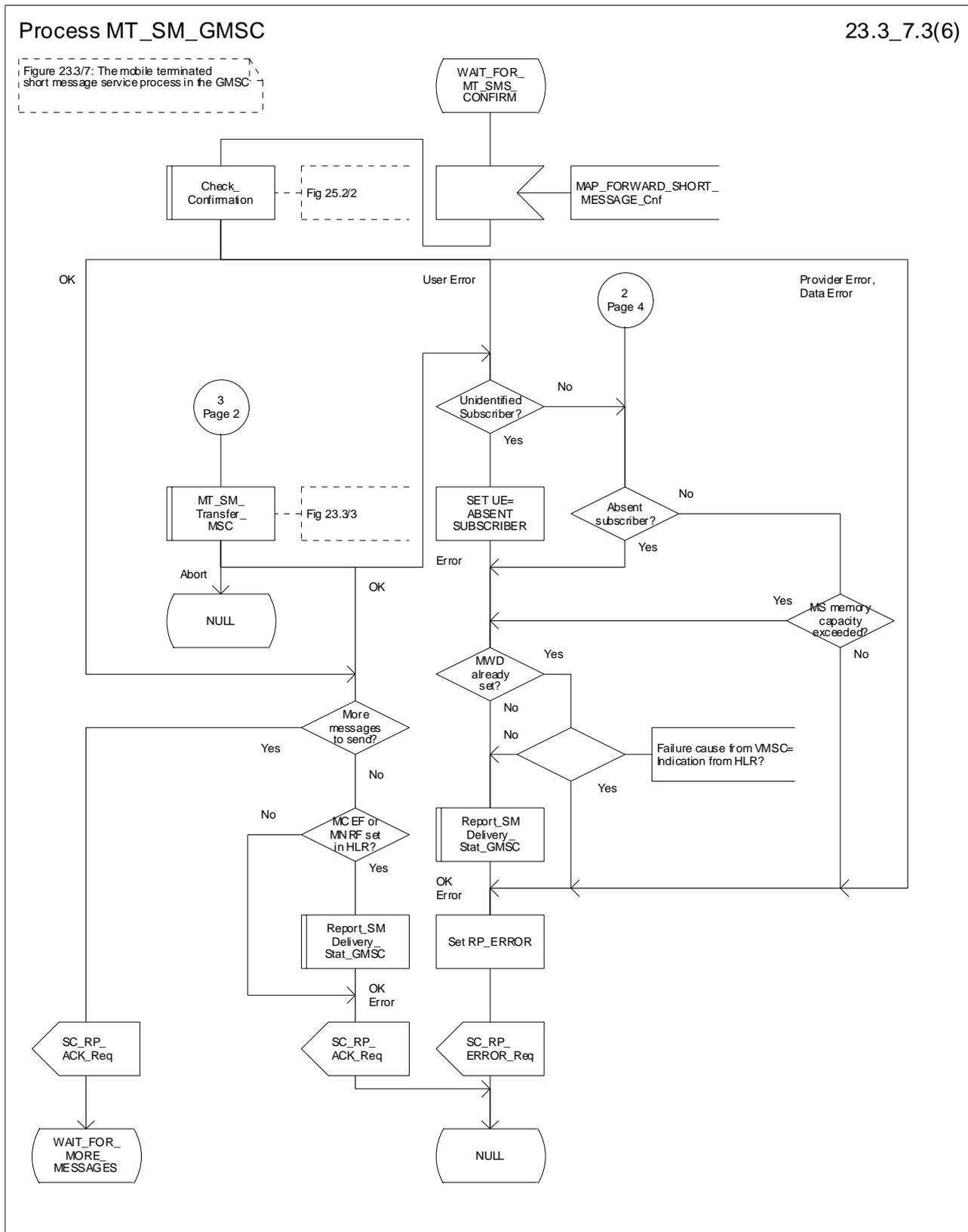
Figure 23.3/7 (sheet 3 of 6): Procedure MT\_SM\_GMSC
