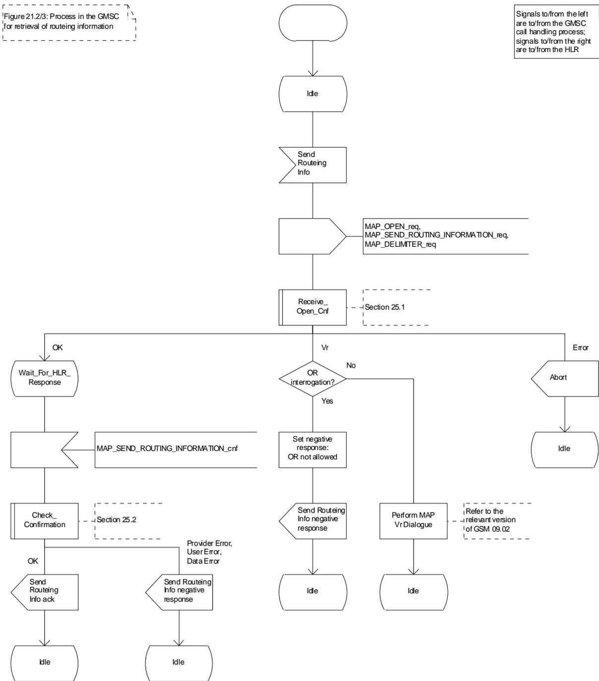
Figure 21.2/3 (sheet 1 of 2): Process SRI\_GMSC
