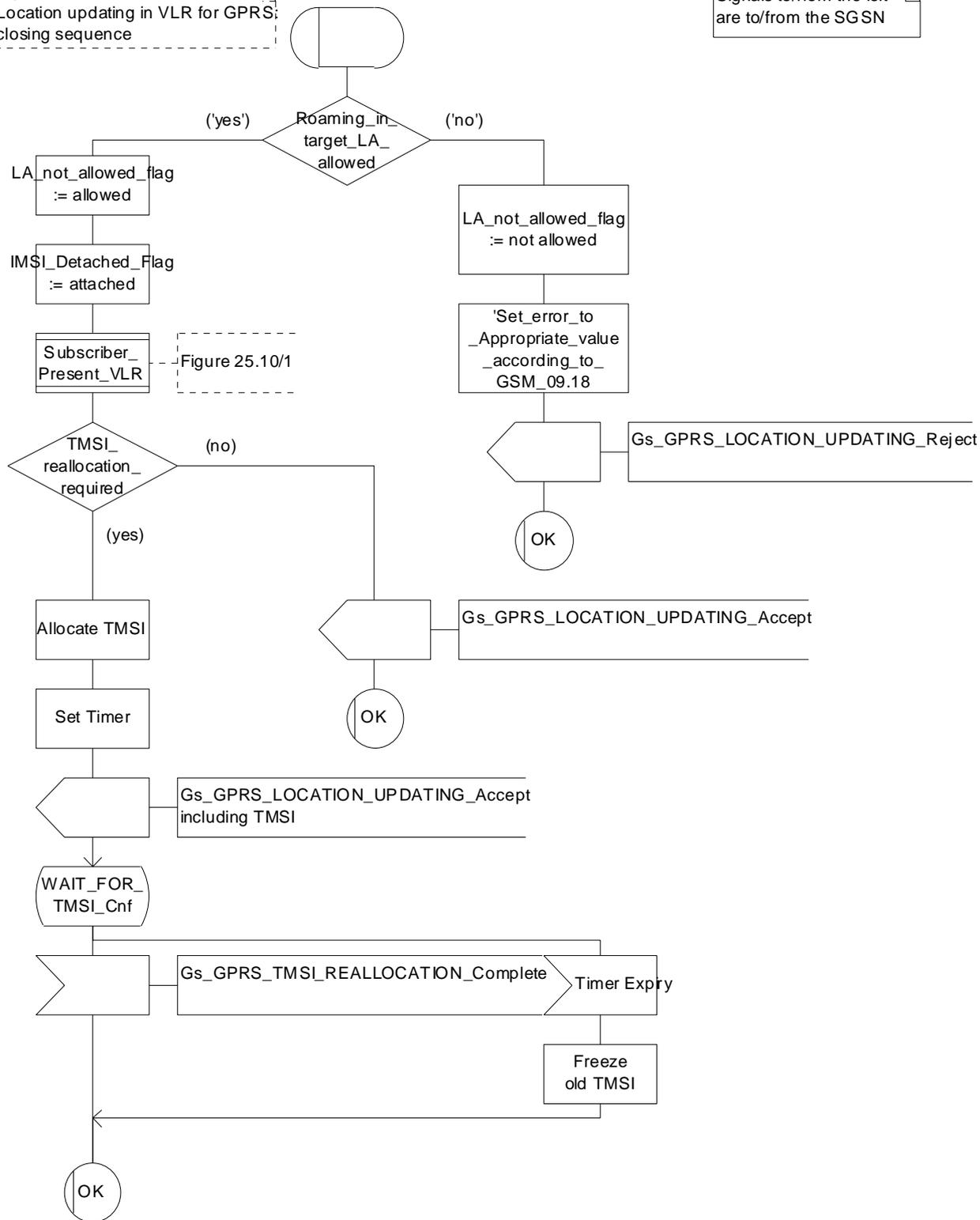
Figure 19.1.1/17: Macro GPRS\_Location\_Update\_Completion\_VLR
