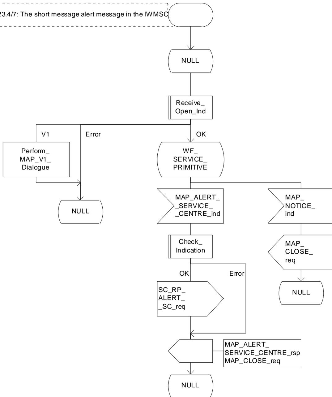
Figure 23.4/7: Process Alert\_SC\_IWMSC
