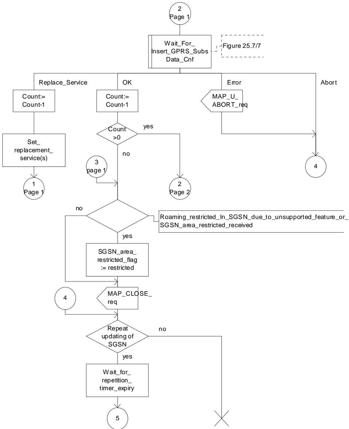
Figure 25.7/5 (sheet 2 of 2): Process Insert\_GPRS\_Subscriber\_Data\_Stand\_Alone\_HLR
