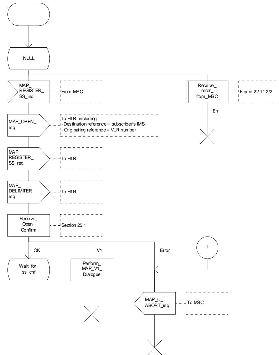
Figure 22.2.3/1 (sheet 1 of 2): Procedure SS\_Register\_VLR
