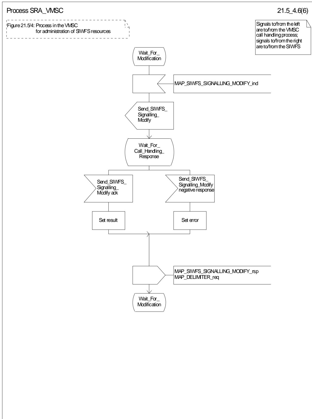
Figure 21.5/4 (sheet 6 of 6): Process SRA\_VMSC
