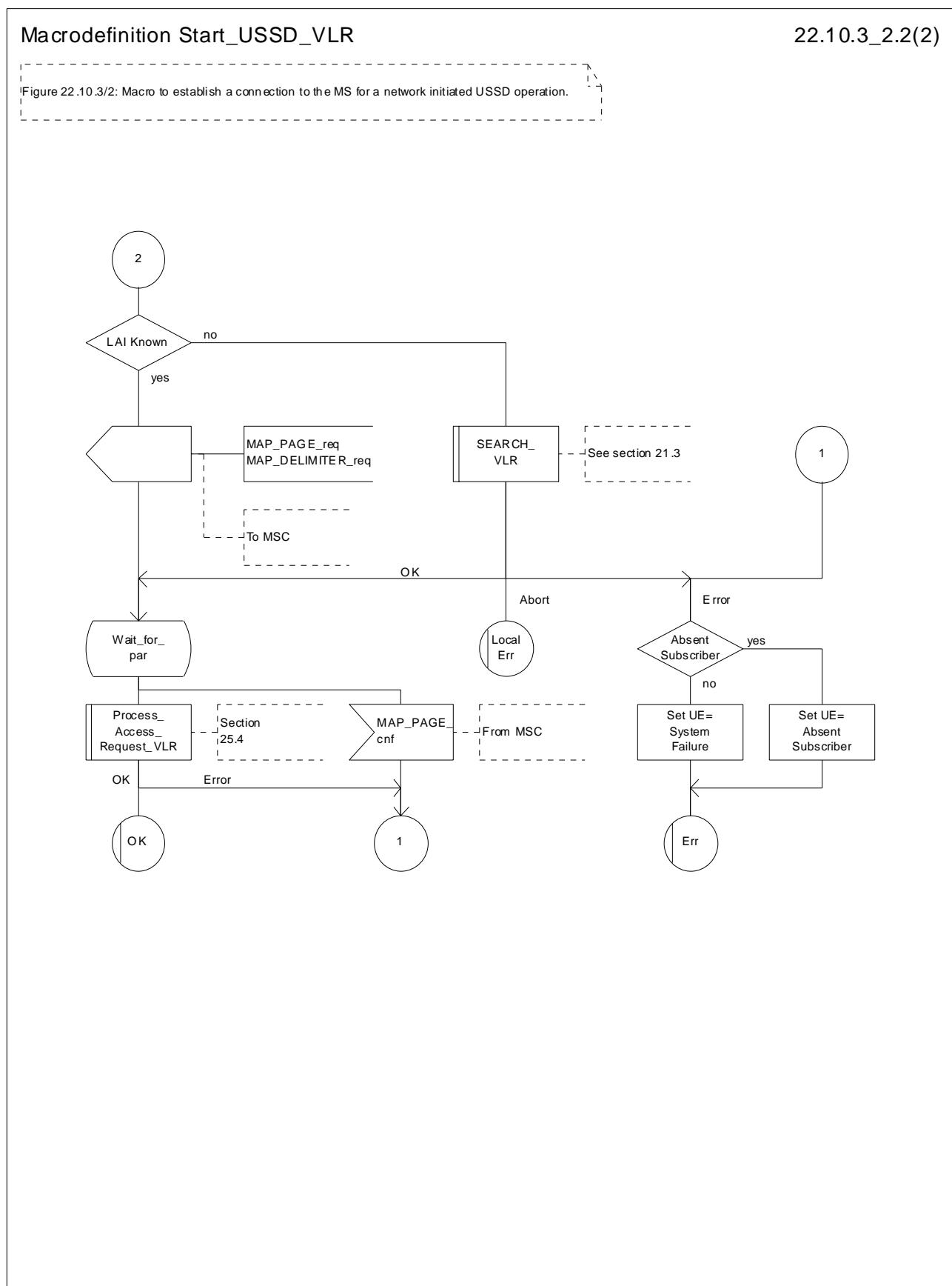
Figure 22.10.3/2 (sheet 2 of 2): Macro Start\_USSD\_VLR
