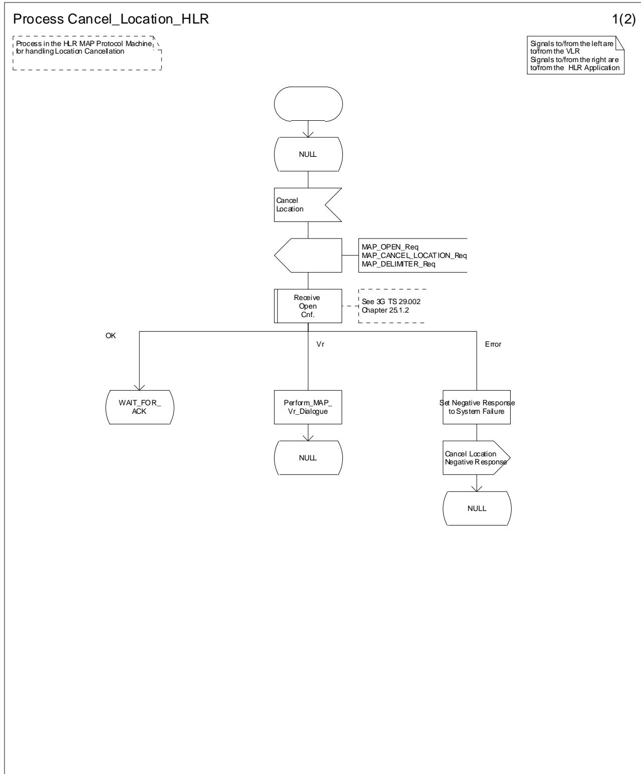
Figure 19.1.2/2 (Sheet 1 of 2): Process Cancel\_Location\_HLR
