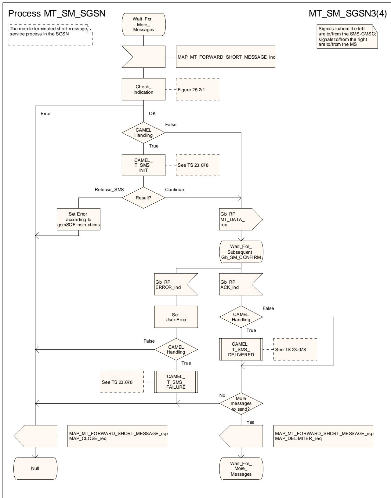
Figure 23.3/10 (sheet 3 of 4): Process MT\_SM\_SGSN
