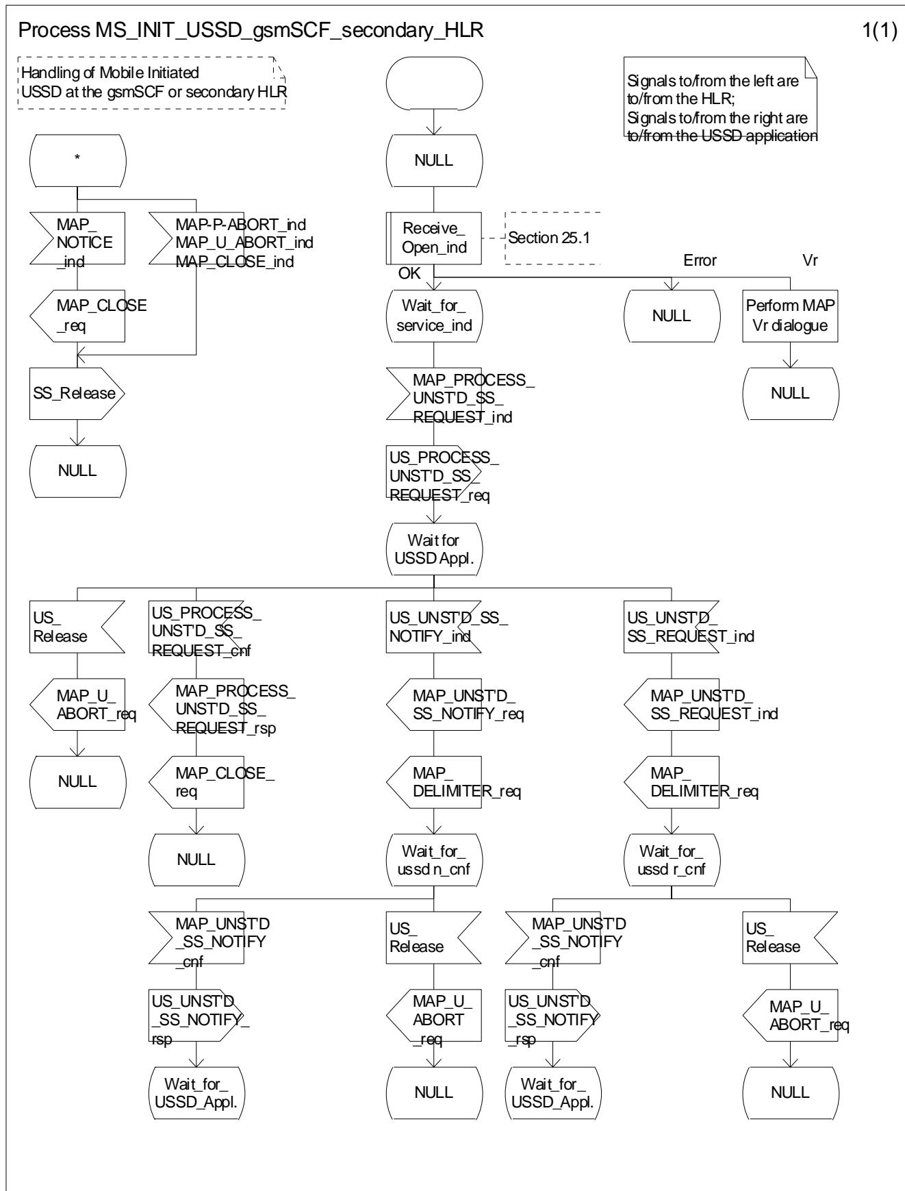
Figure 22.9.5/1 Process MS\_INIT\_USSD\_gsmSCF\_secondary\_HLR
