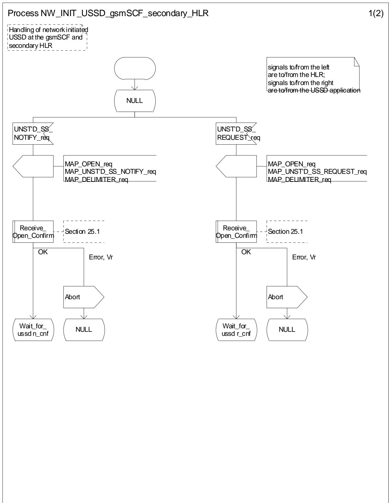
Figure 22.10.5/1 (sheet 1 of 2): Procedure NI\_USSD\_gsmSCF\_secondary\_HLR
