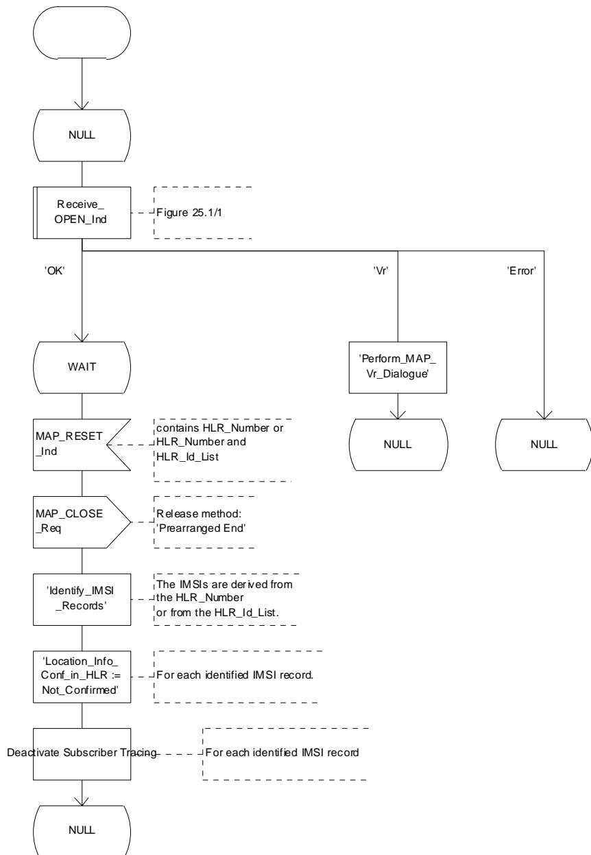
Figure 19.3/5: Process REC\_RESET\_IN\_VLR
