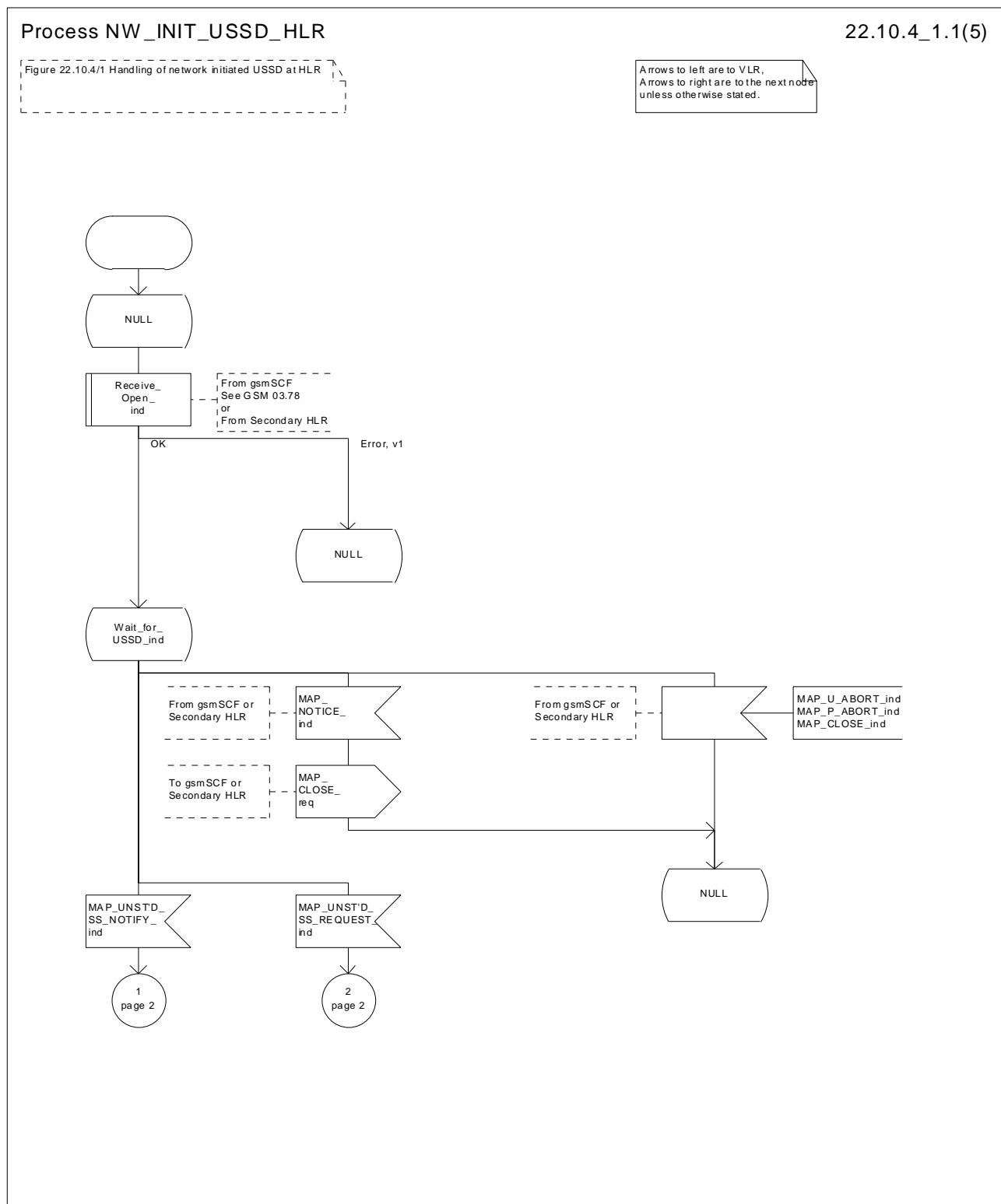
Figure 22.10.4/1 (sheet 1 of 5): Procedure NI\_USSD\_HLR
