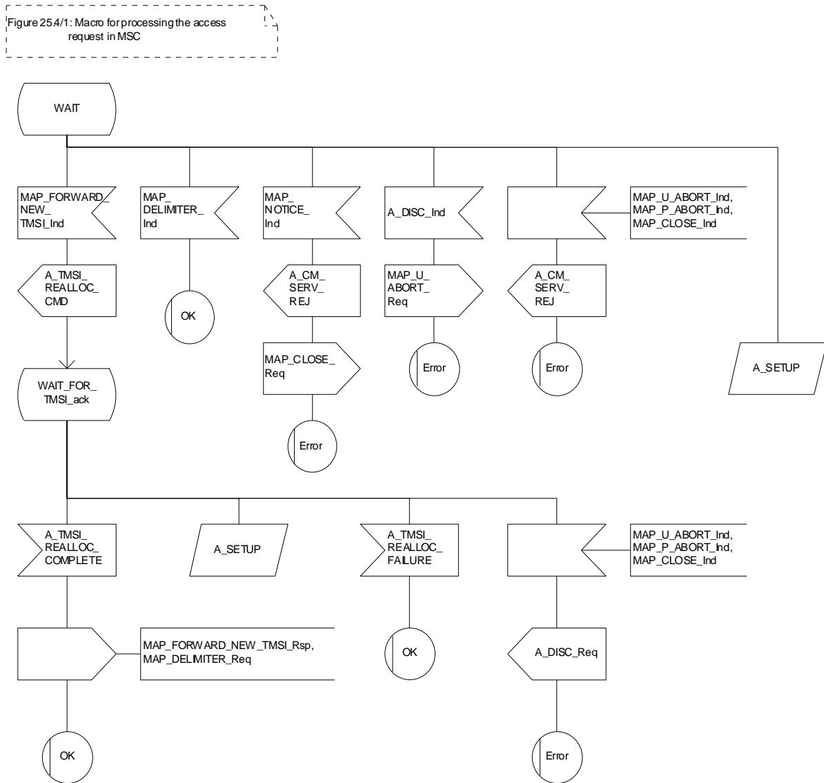
Figure 25.4/1 (sheet 3 of 3): Macro Process\_Access\_Request\_MSC
