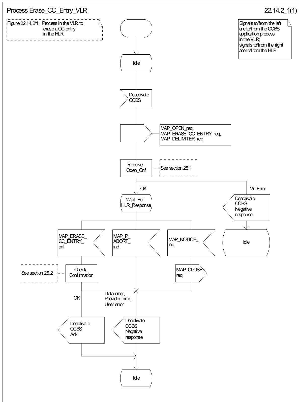
Figure 22.14.2/1: Process Erase\_CC\_Entry\_VLR
