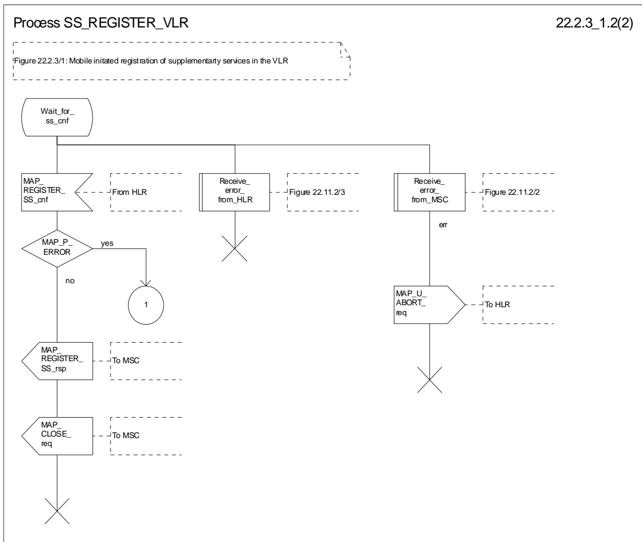
**Figure 22.2.3/1 (sheet 2 of 2): Procedure SS\_Register\_VLR**
