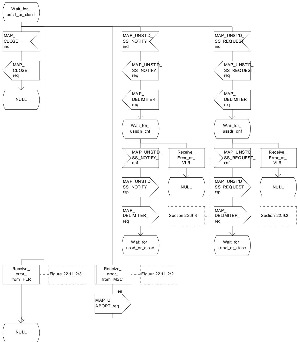
**Figure 22.10.3/1 (sheet 2 of 4): Procedure NI\_USSD\_VLR**
