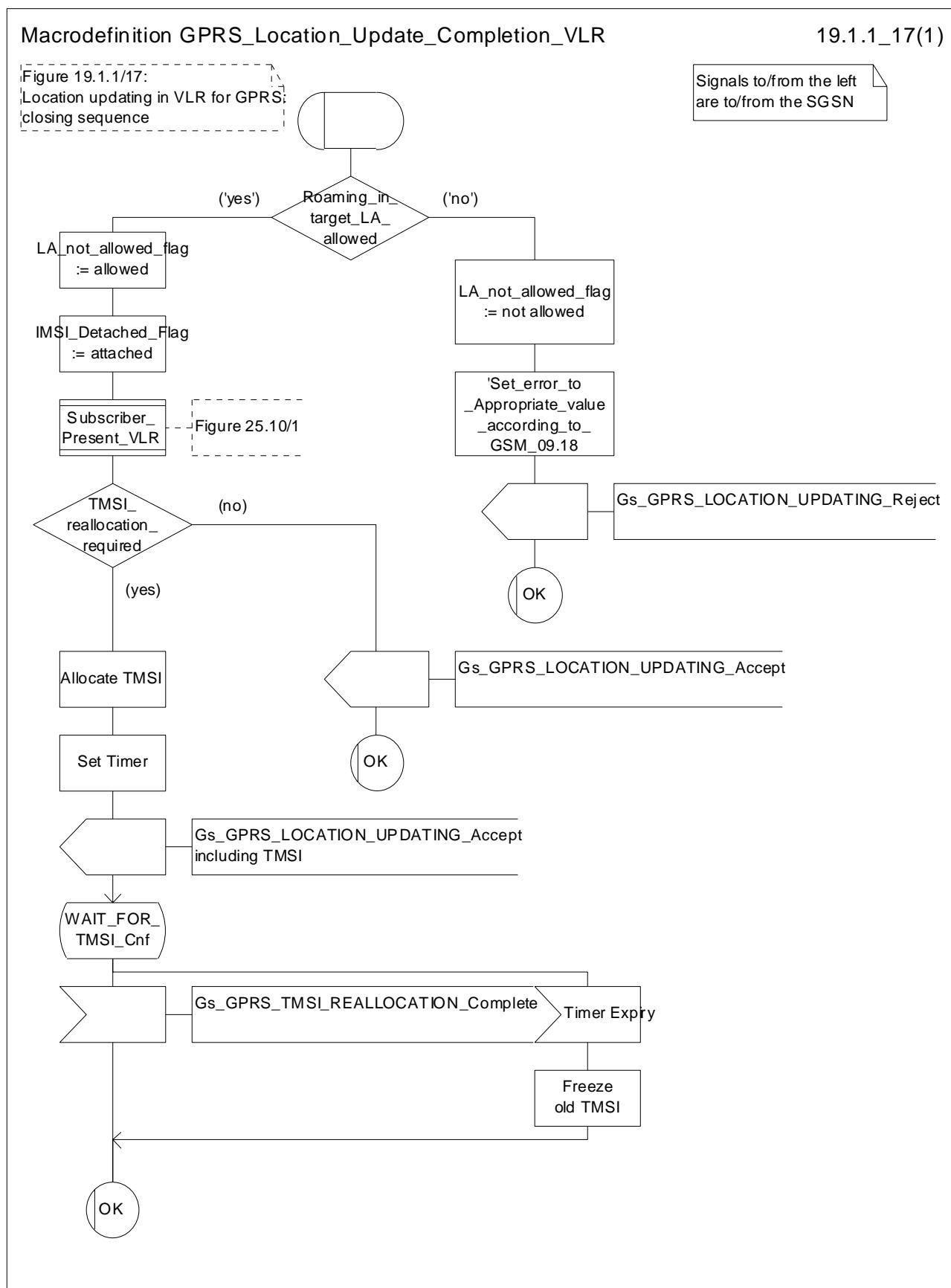
**Figure 19.1.1/17: Macro GPRS\_Location\_Update\_Completion\_VLR**
