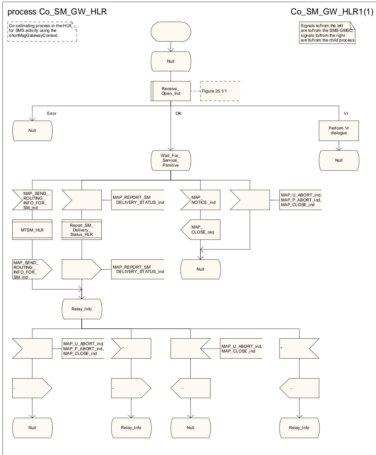
**Figure 23.1/2: Process Co\_SM\_Gateway\_HLR**
