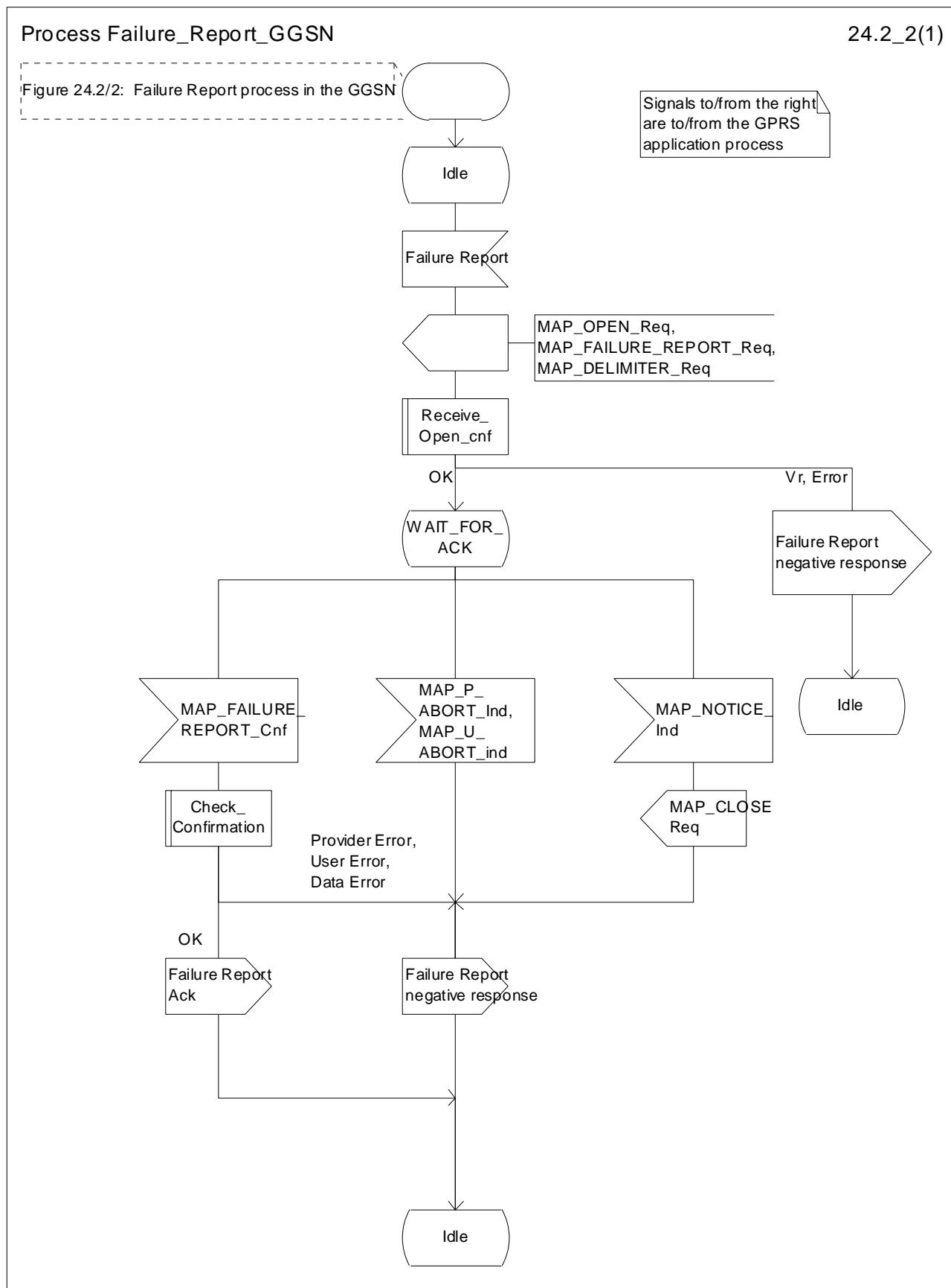
Figure 24.2/2: Process Failure\_Report\_GGSN
