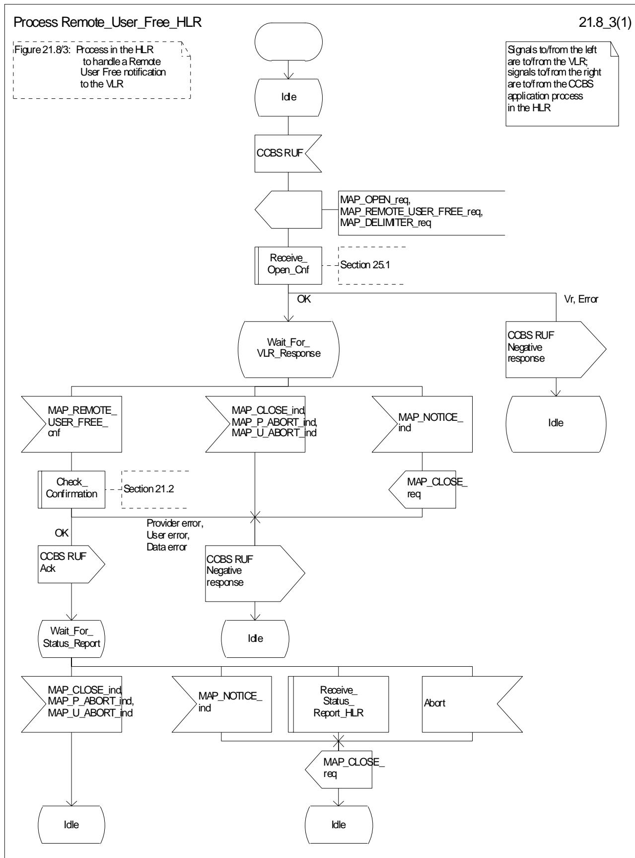
Figure 21.8/3: Process Remote\_User\_Free\_HLR
