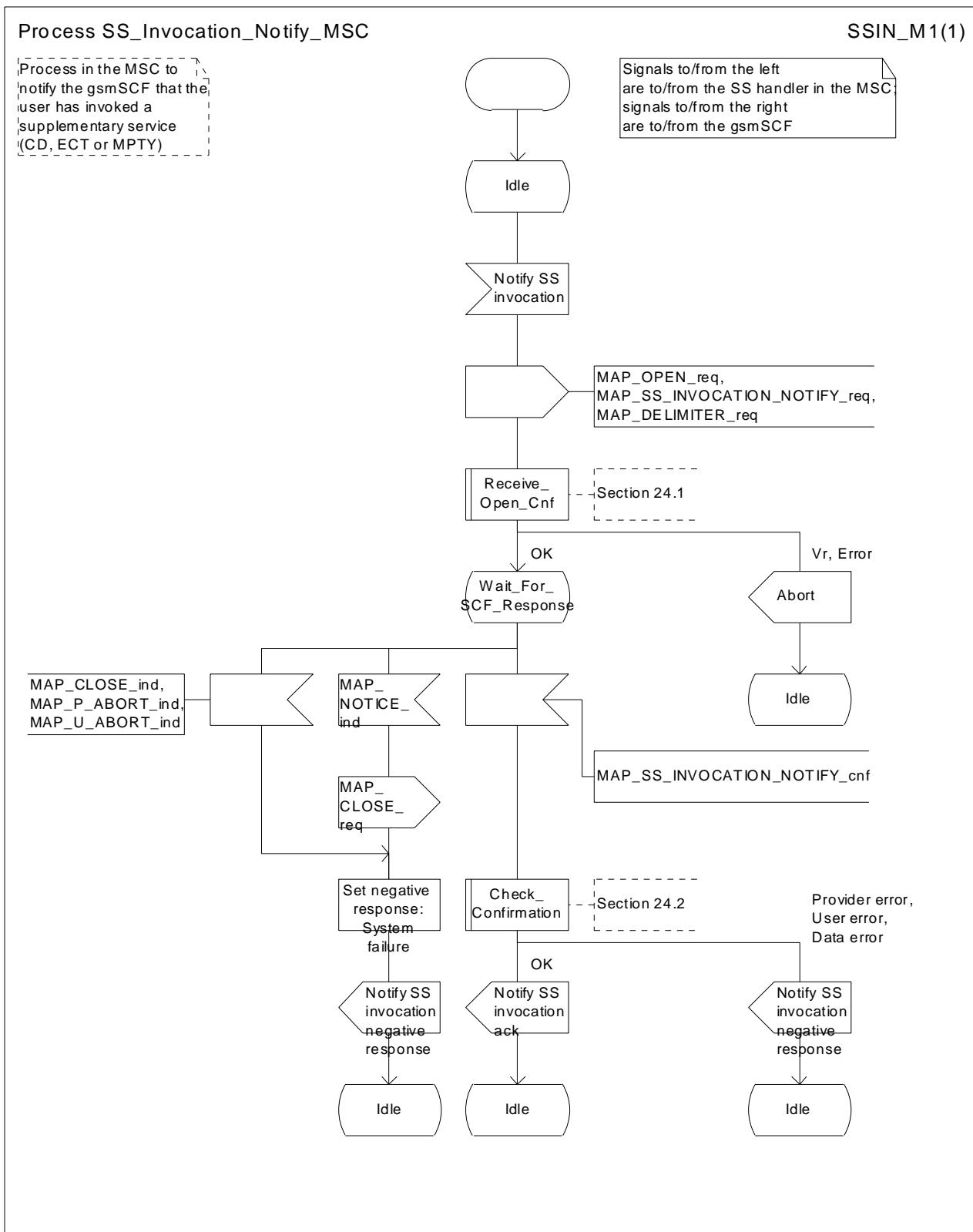
Figure 22.12.2/1: Process SS\_Invocation\_Notify\_MSC (sheet 1 of 1)
