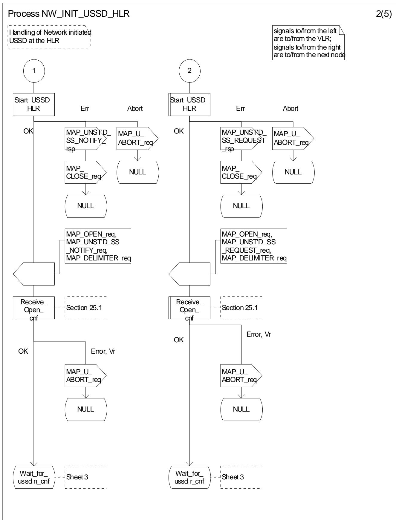
Figure 22.10.4/1 (sheet 2 of 5): Procedure NI\_USSD\_HLR
