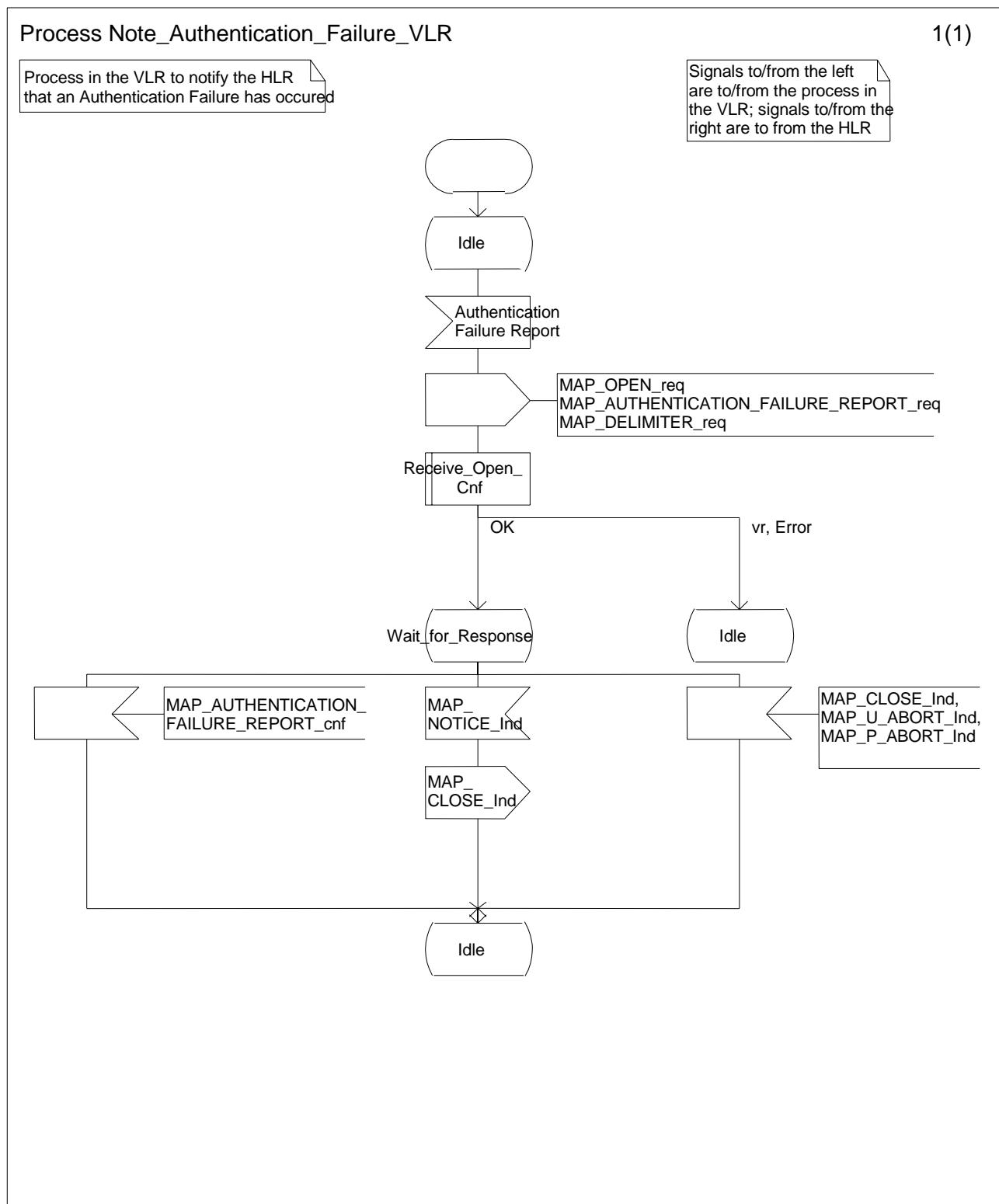
Figure 25.6/8: Process Note\_Authentication\_Failure\_VLR
