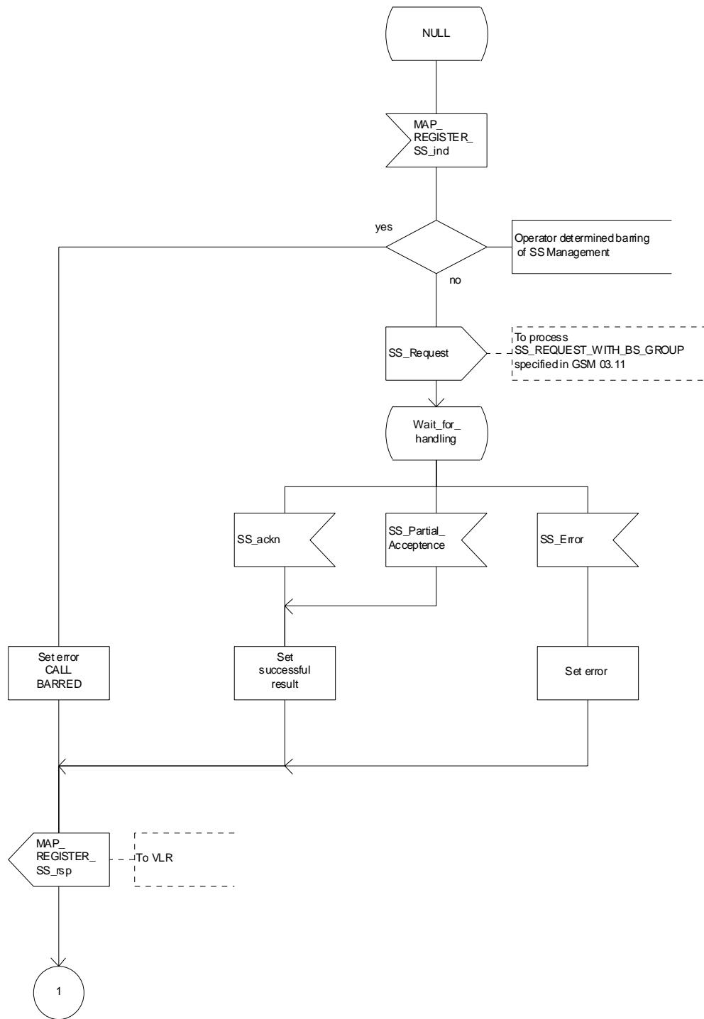
Figure 22.2.4/1 (sheet 1 of 2): Procedure SS\_Register\_HLR
