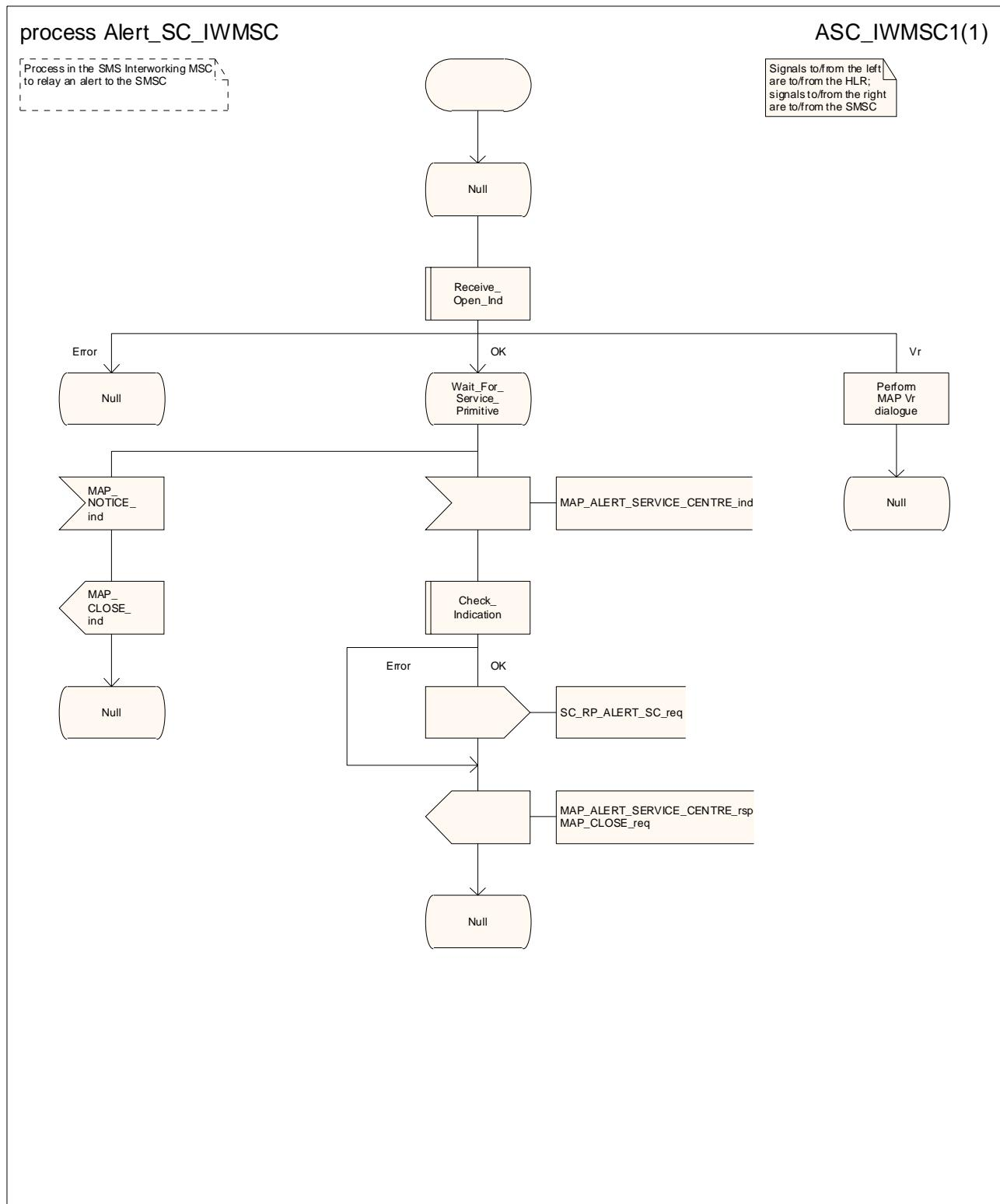
**Figure 23.4/7: Process Alert\_SC\_IWMSC**
