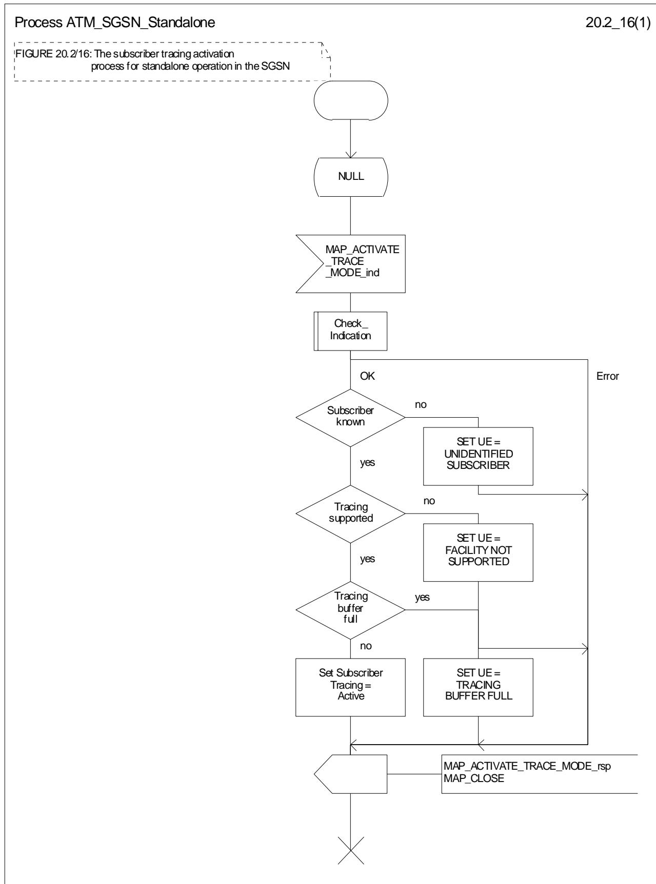
Figure 20.2/16: Process ATM\_SGSN\_Standalone
