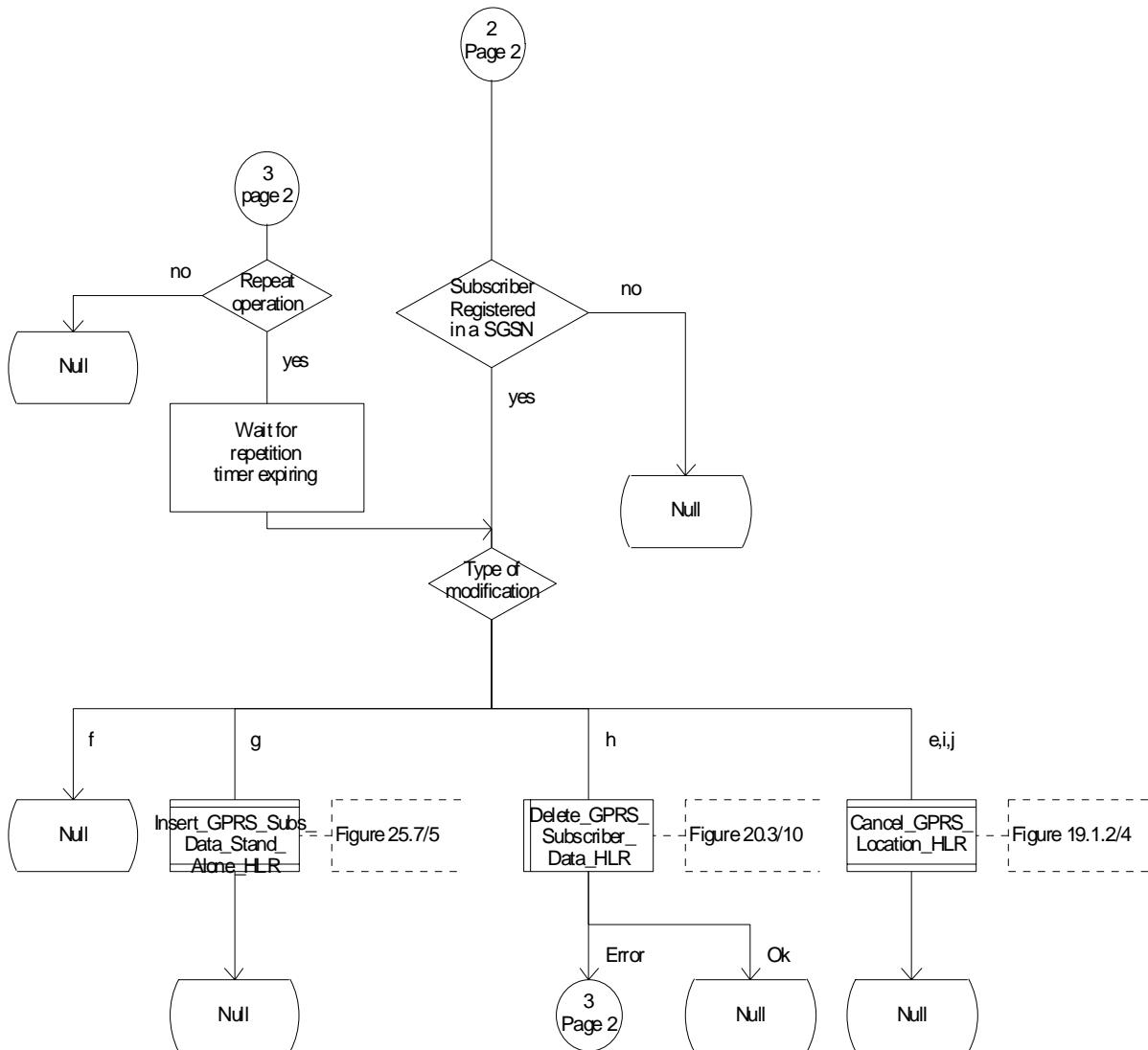
Figure 20.3/4 (sheet 2 of 2): Process Modify\_Data\_HLR
