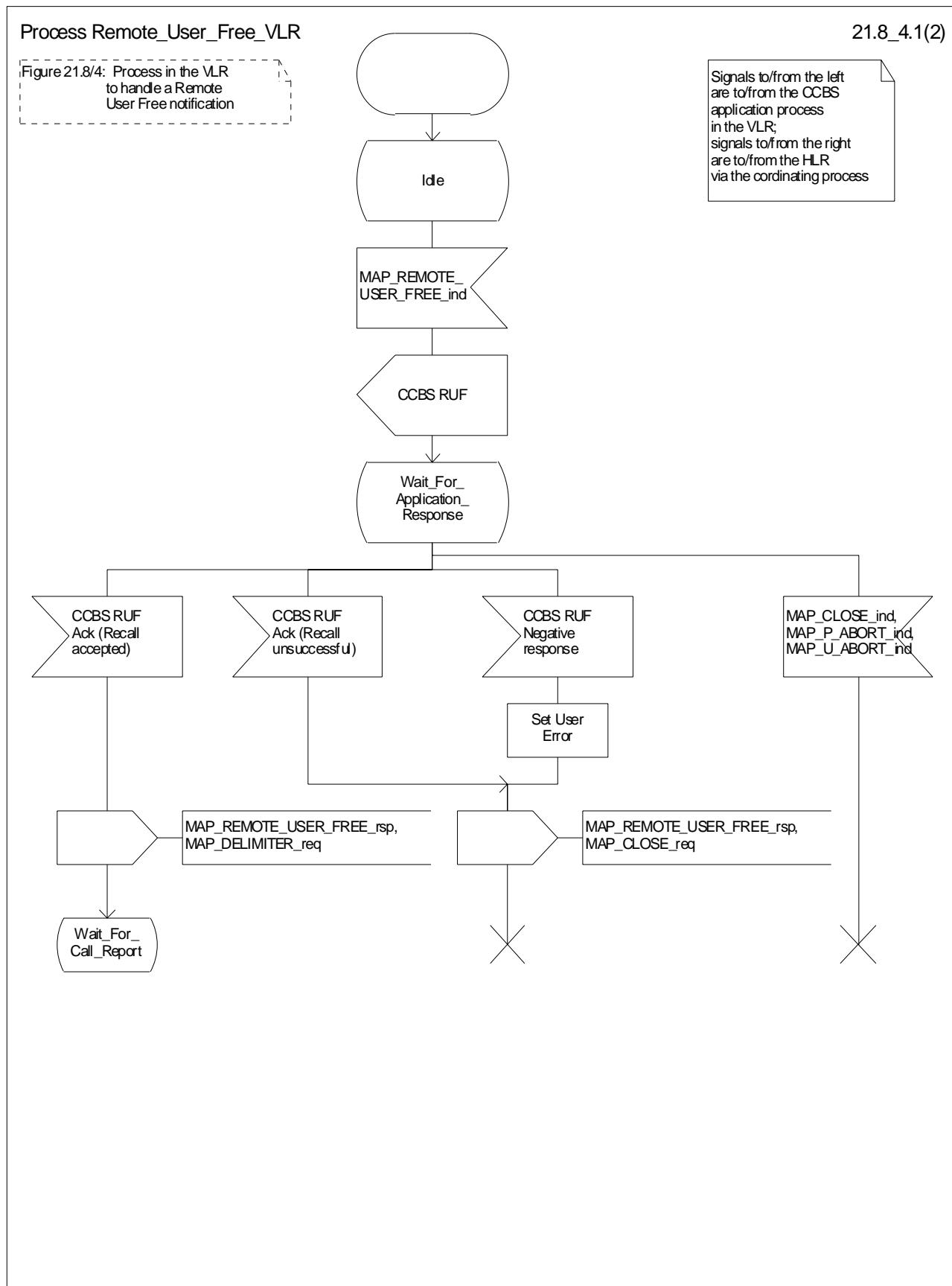
Figure 21.8/4 (sheet 1 of 2): Process Remote\_User\_Free\_VLR
