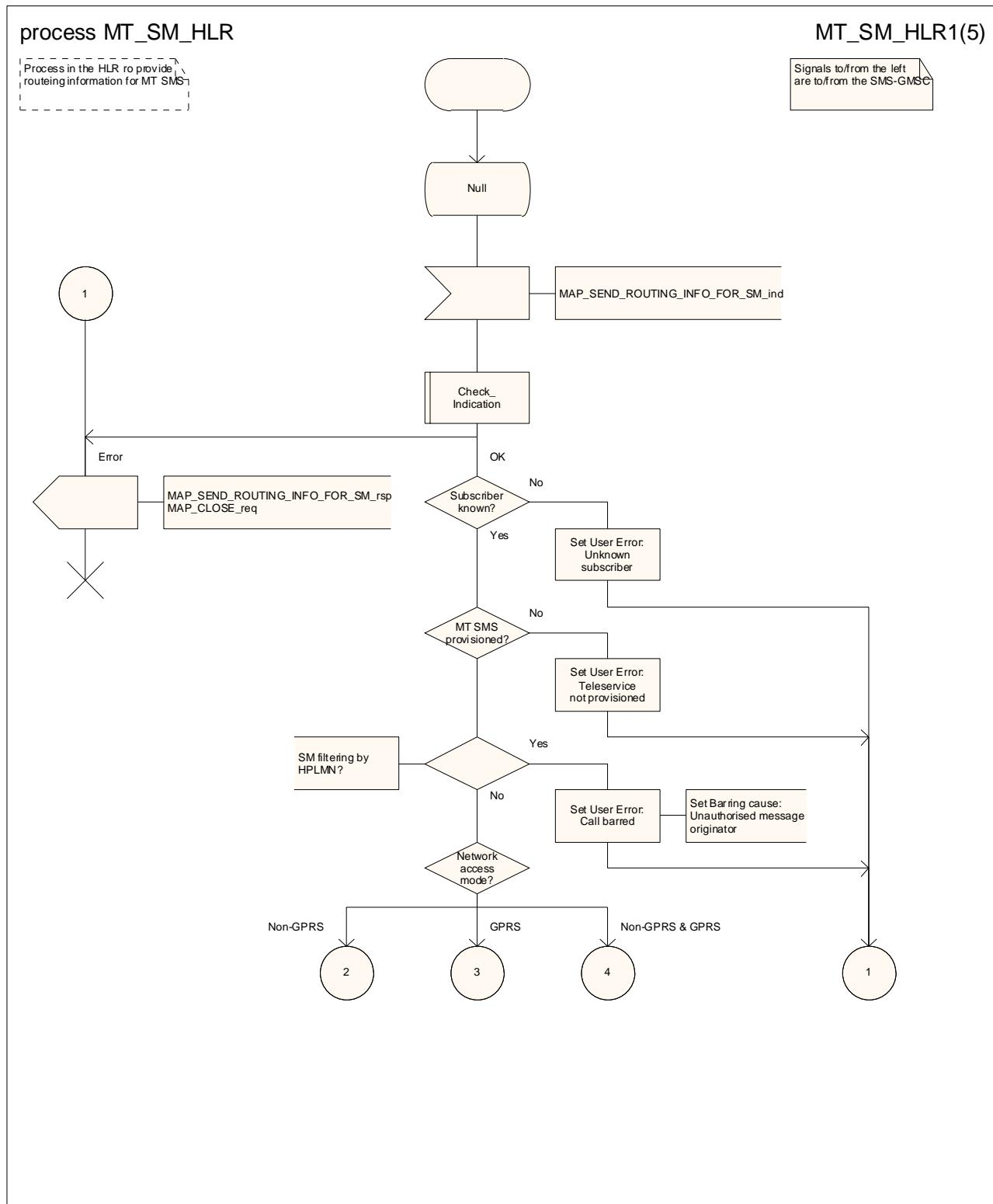
**Figure 23.3/5 (sheet 1 of 5): Process MT\_SM\_HLR**
