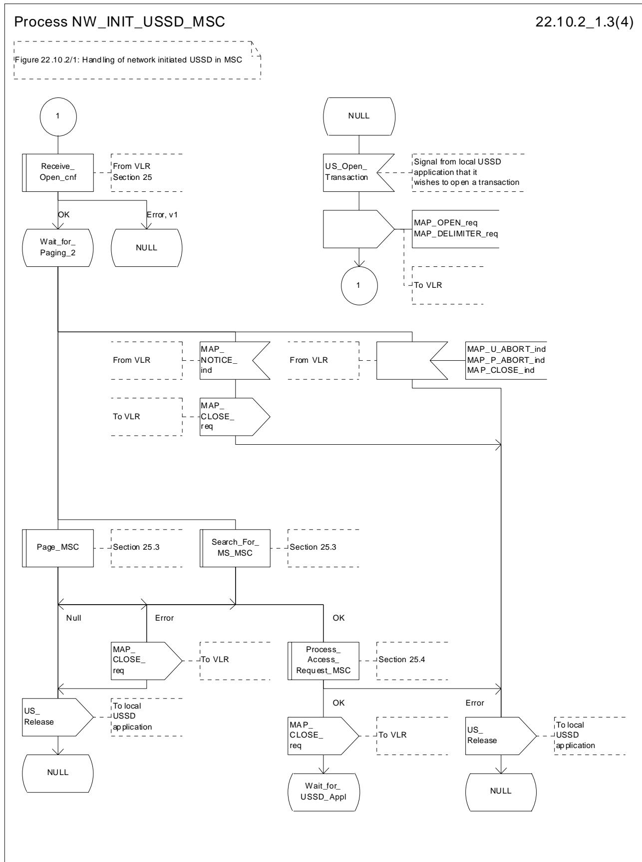
Figure 22.10.2/1 (sheet 3 of 4): Procedure NI\_USSD\_MSC
