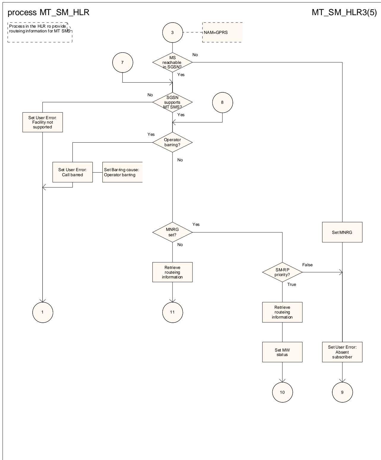
Figure 23.3/5 (sheet 3 of 5): Process MT\_SM\_HLR
