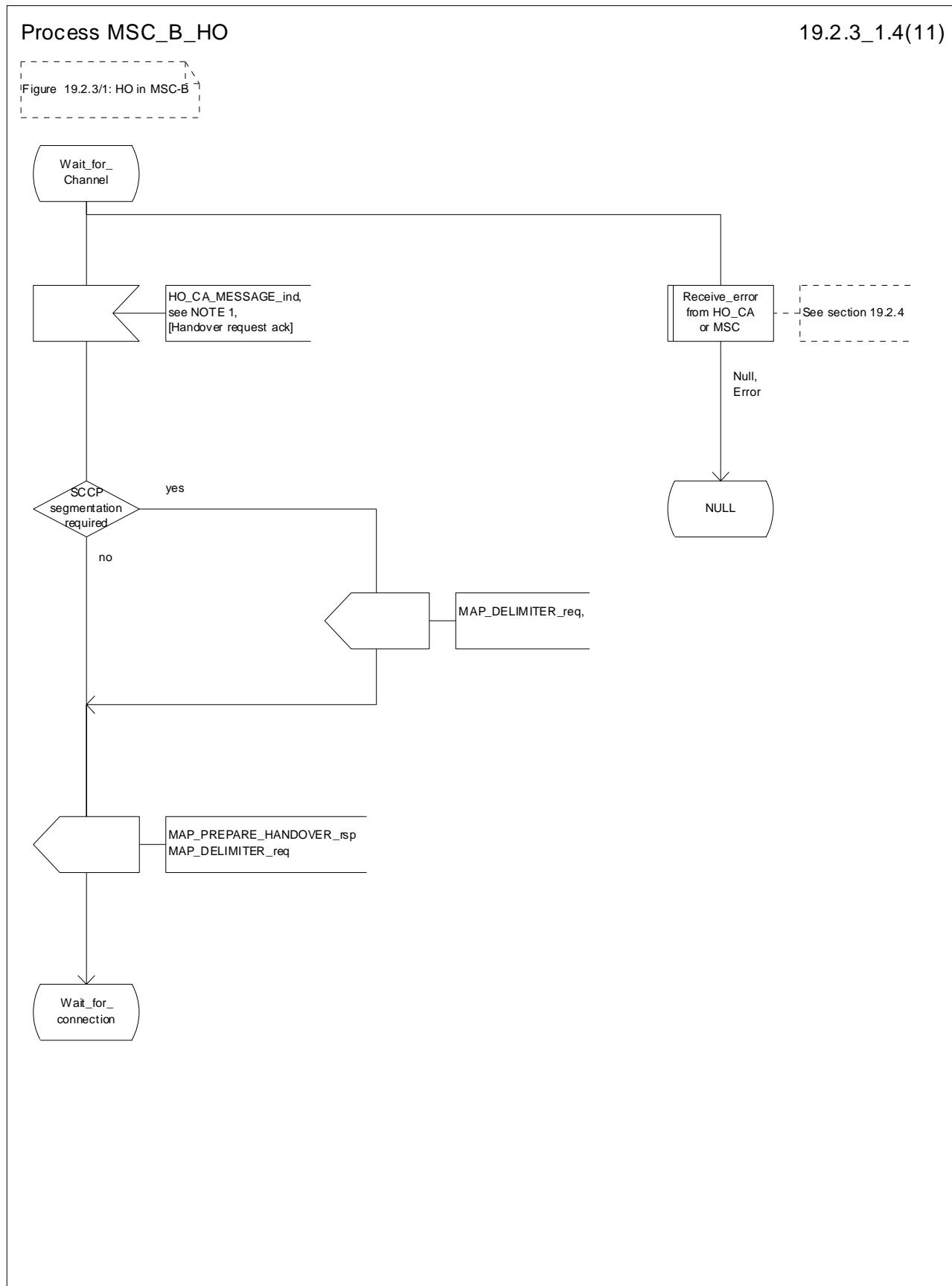
Figure 19.2.3/1 (sheet 4 of 11): Process MSC\_B\_HO
