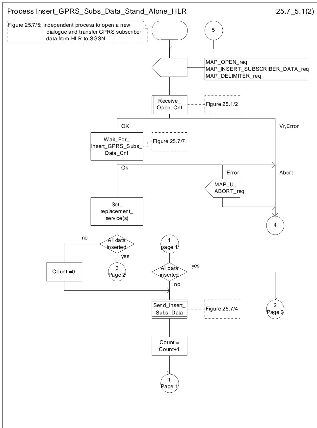
Figure 25.7/5 (sheet 1 of 2): Process Insert\_GPRS\_Subs\_Data\_Stand\_Alone\_HLR
