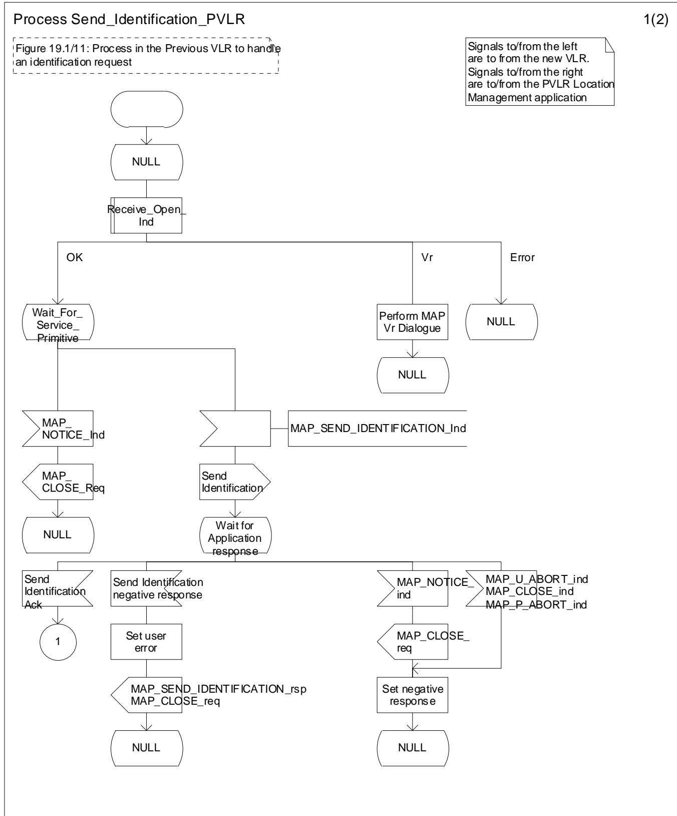
Figure 19.1.1/XX (sheet 1 of 2): Process Send\_Identification\_PVLR
