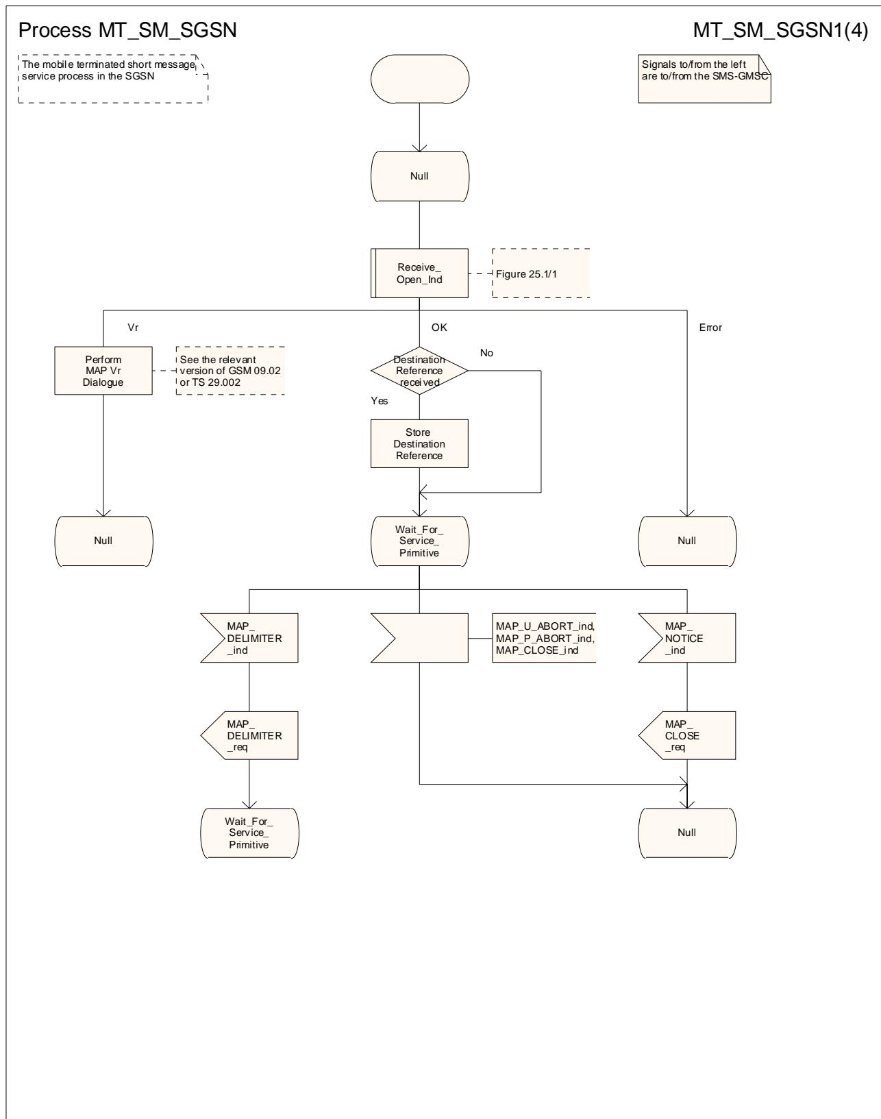
Figure 23.3/10 (sheet 1 of 4): Process MT\_SM\_SGSN
