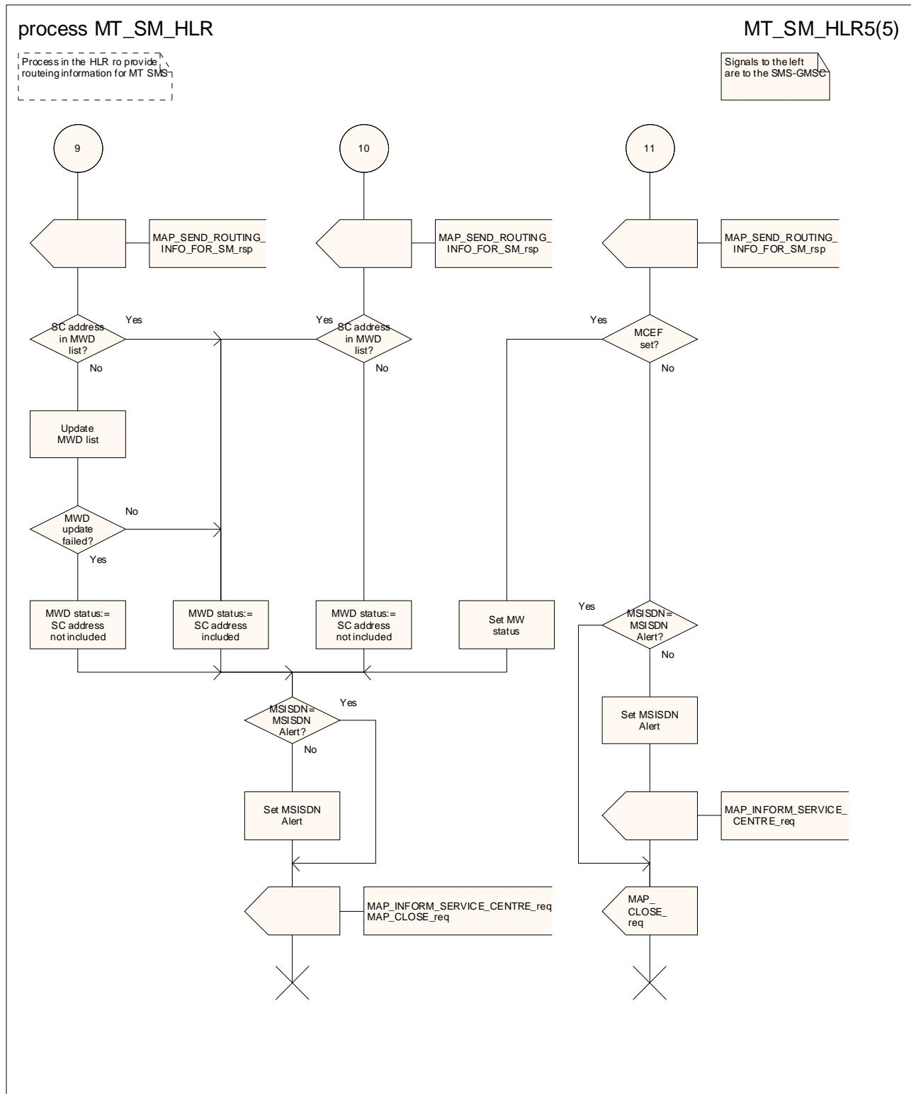
Figure 23.3/5 (sheet 5 of 5): Process MT\_SM\_HLR
