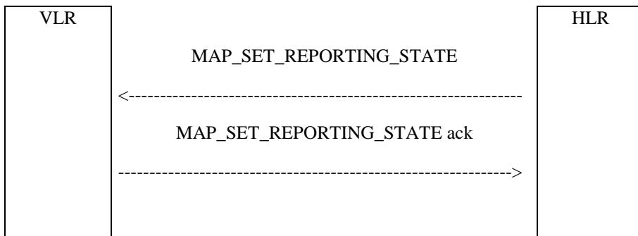
**Figure 21.6/1: Message Flow for Setting the Reporting State**
