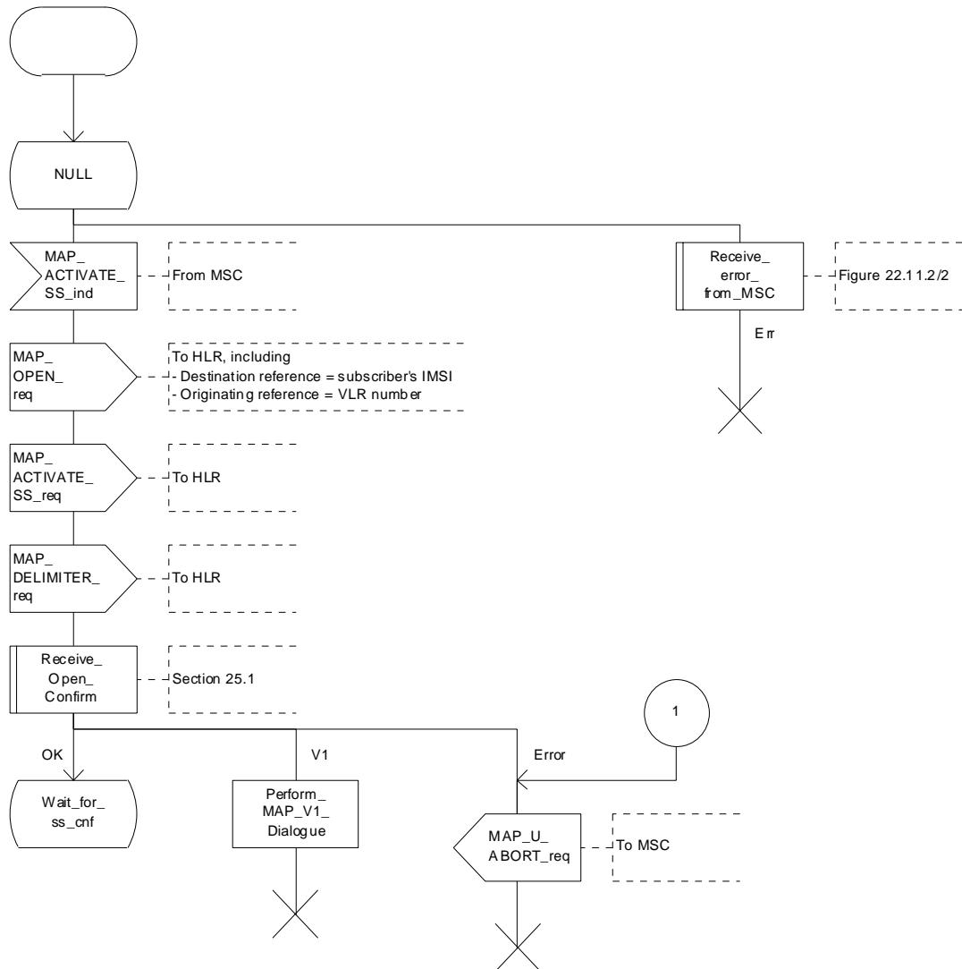
Figure 22.4.3/1 (sheet 1 of 2): Procedure Activate\_SS\_VLR
