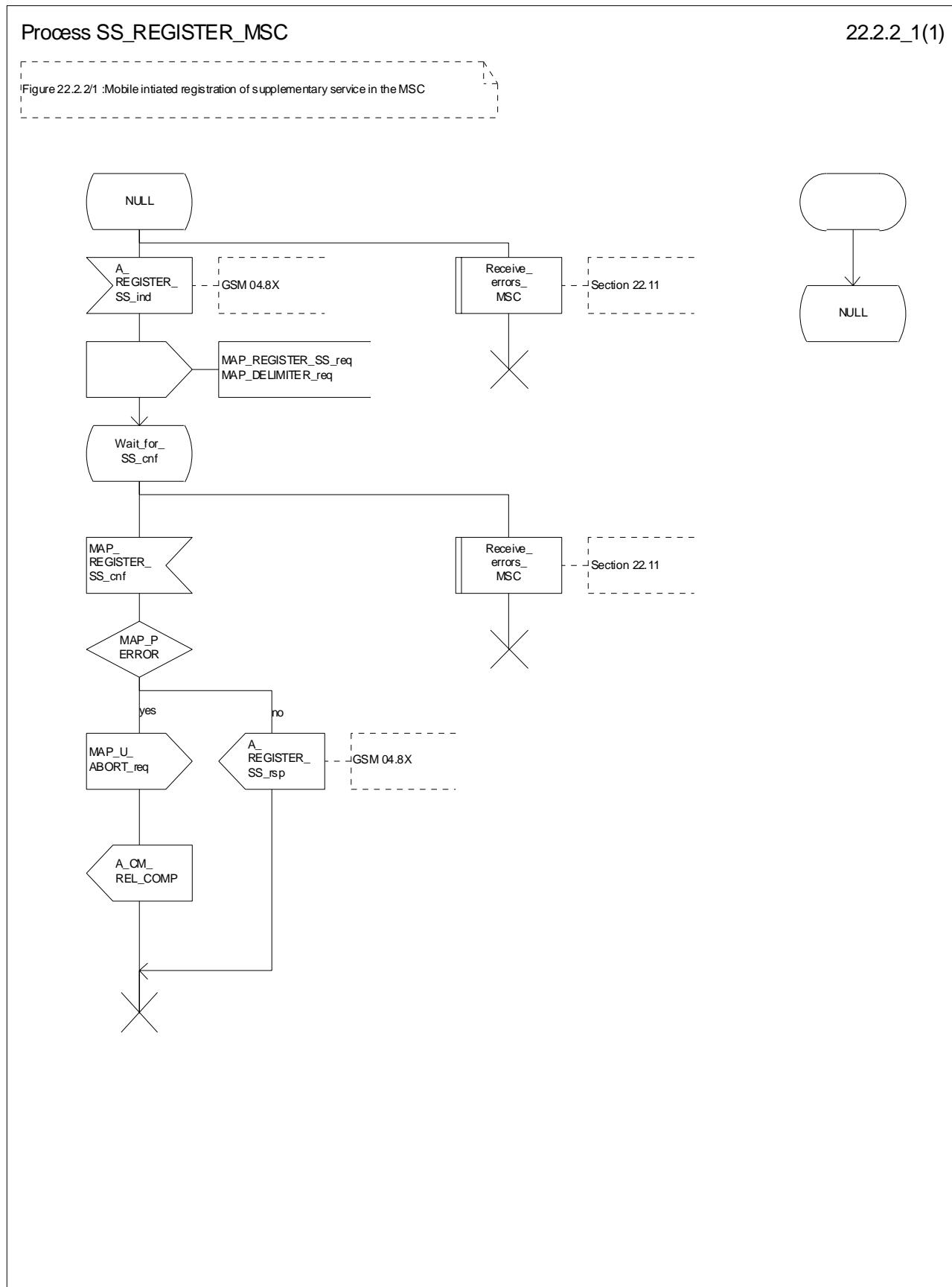
**Figure 22.2.2/1: Procedure SS\_Register\_MSC**
