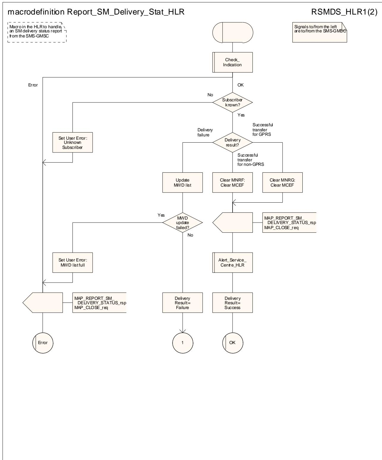
Figure 23.6/1 (sheet 1 of 2): Macro Report\_SM\_Delivery\_Stat\_HLR
