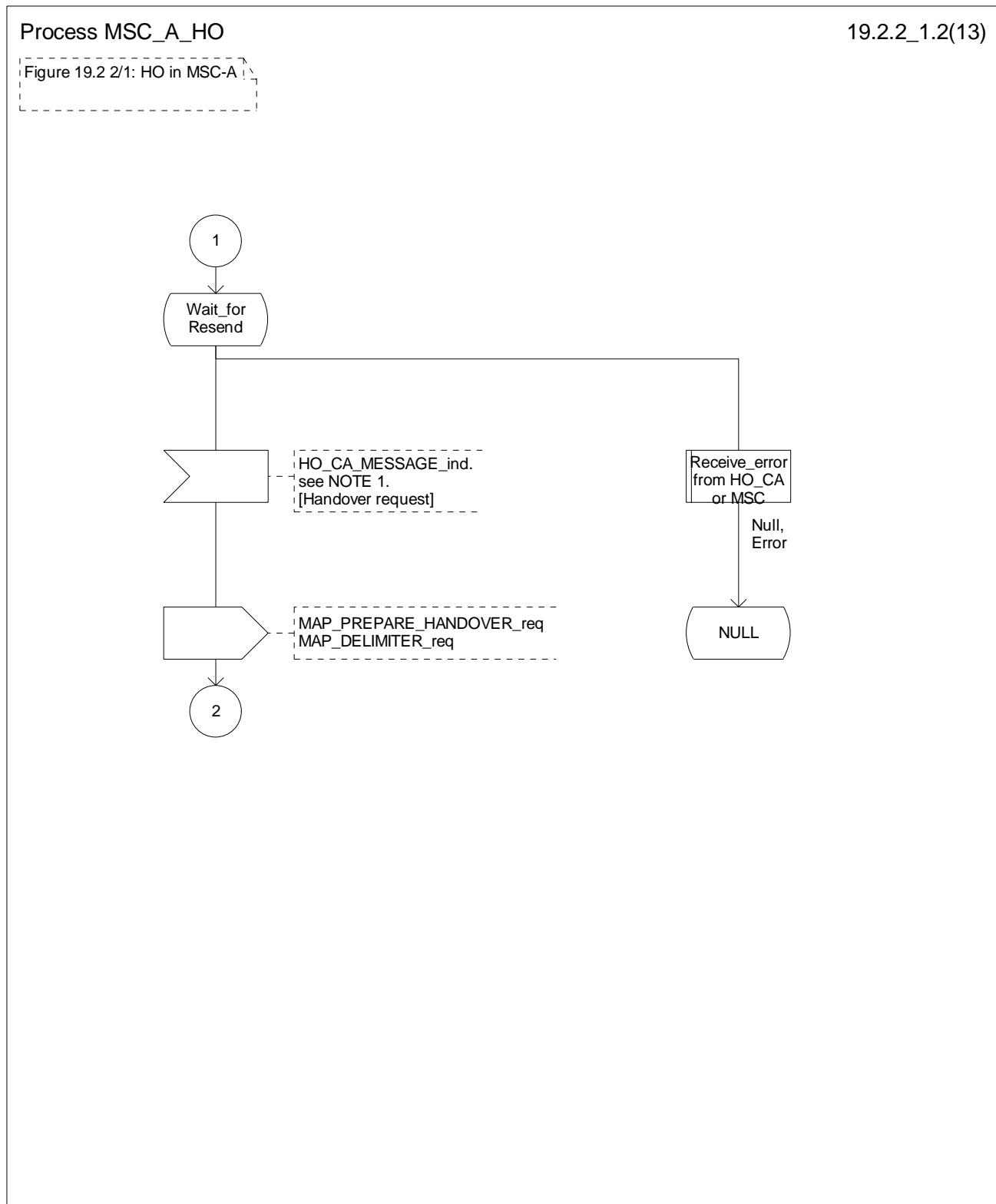
Figure 19.2.2/1 (sheet 2 of 13): Process MSC\_A\_HO
