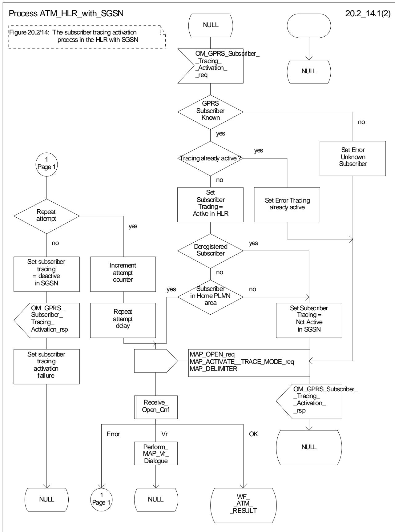
**Figure 20.2/14 (sheet 1 of 2): Process ATM\_HLR\_with\_SGSN**
