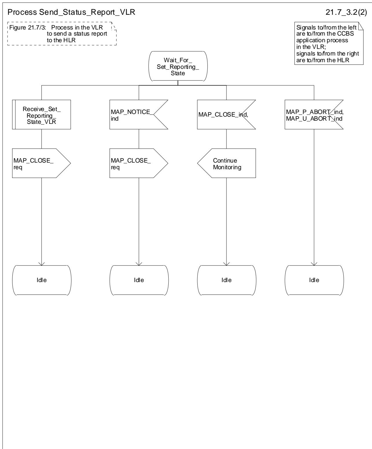
Figure 21.7/3 (sheet 2 of 2): Process Send\_Status\_Report\_VLR
