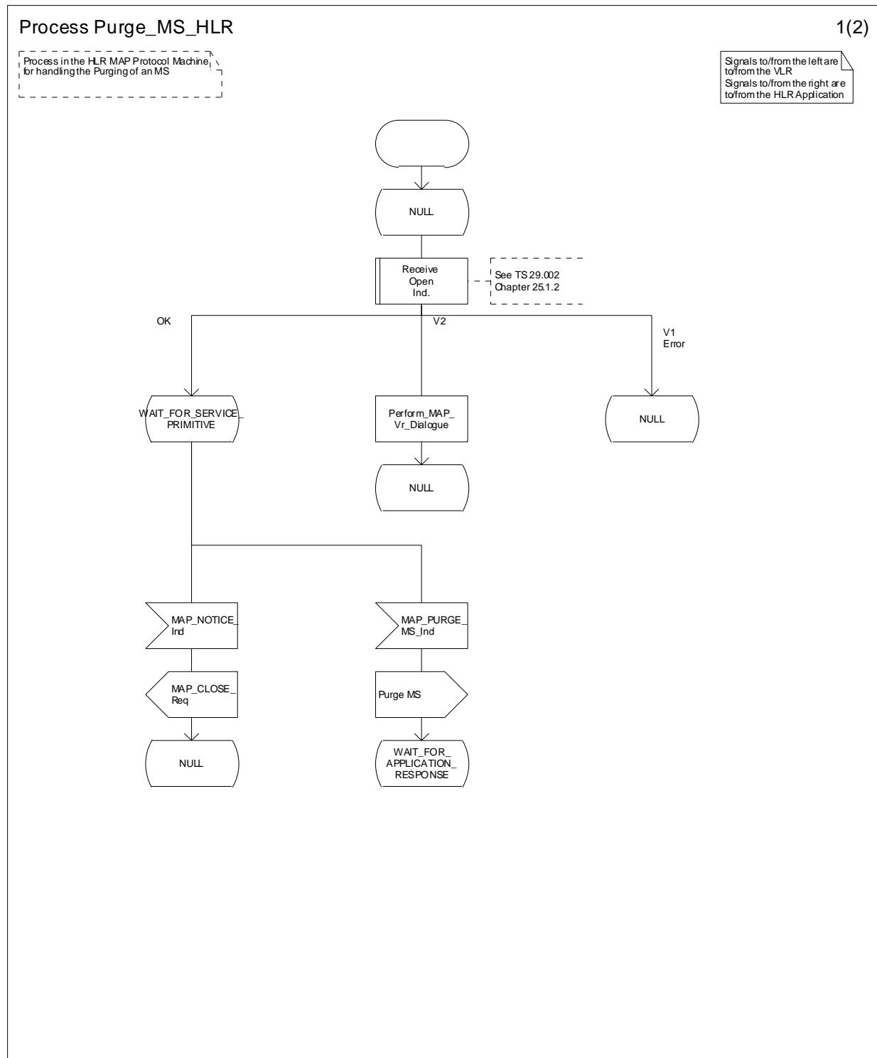
Figure 19.1.4/3 (Sheet 1 of 2): Process Purge\_MS\_HLR
