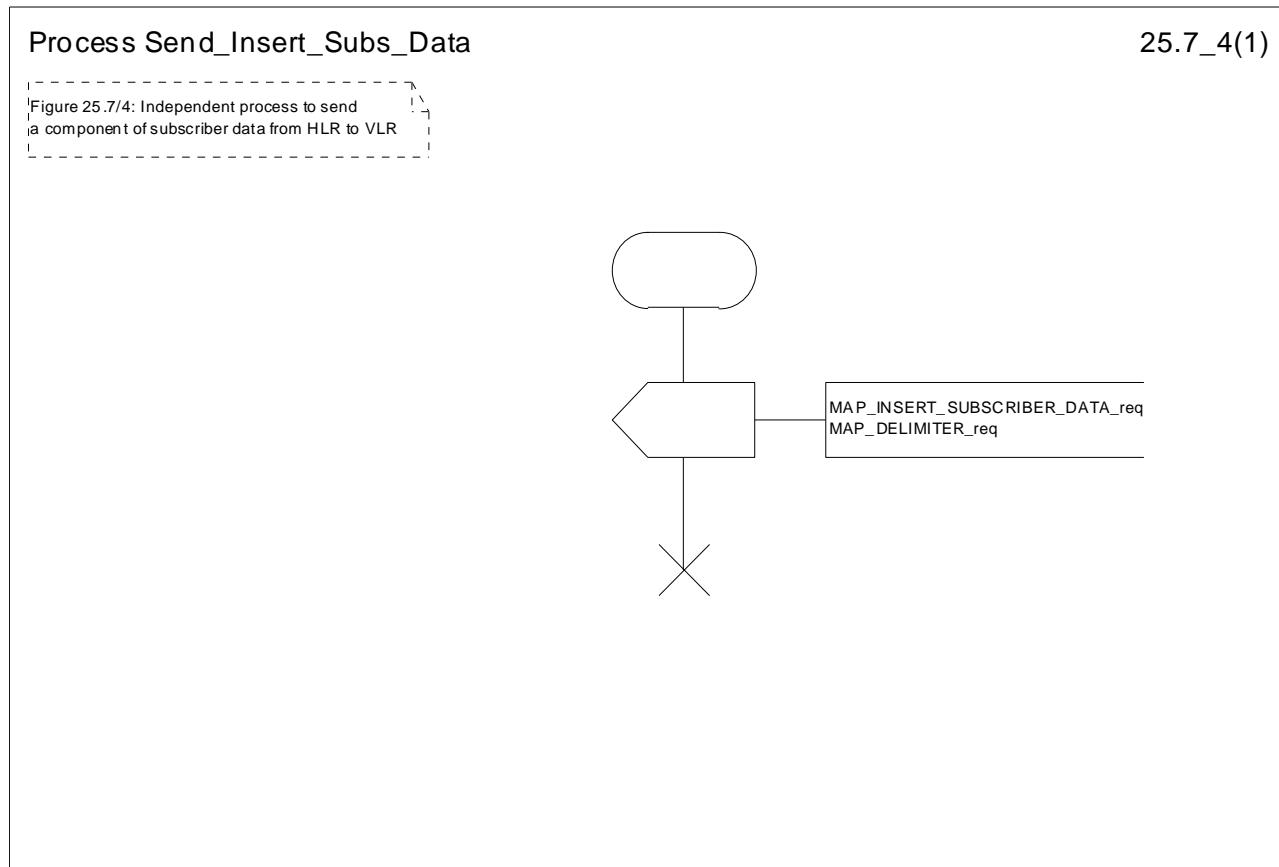
**Figure 25.7/4: Process Send\_Insert\_Subs\_Data**
