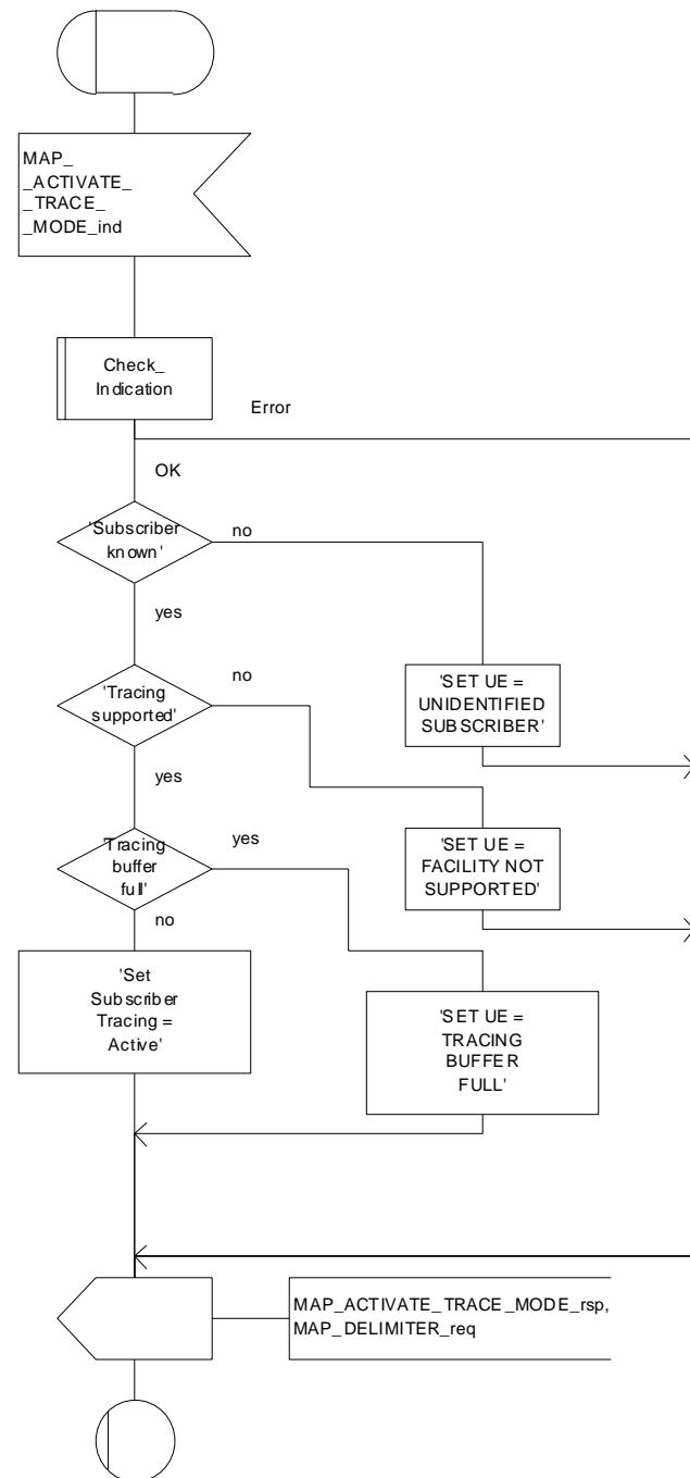
Figure 25.9/3: Macro Activate\_Tracing\_VLR
