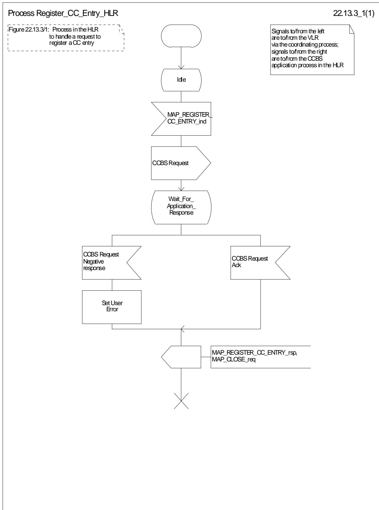
Figure 22.13.3/1: Process Register\_CC\_Entry\_HLR
