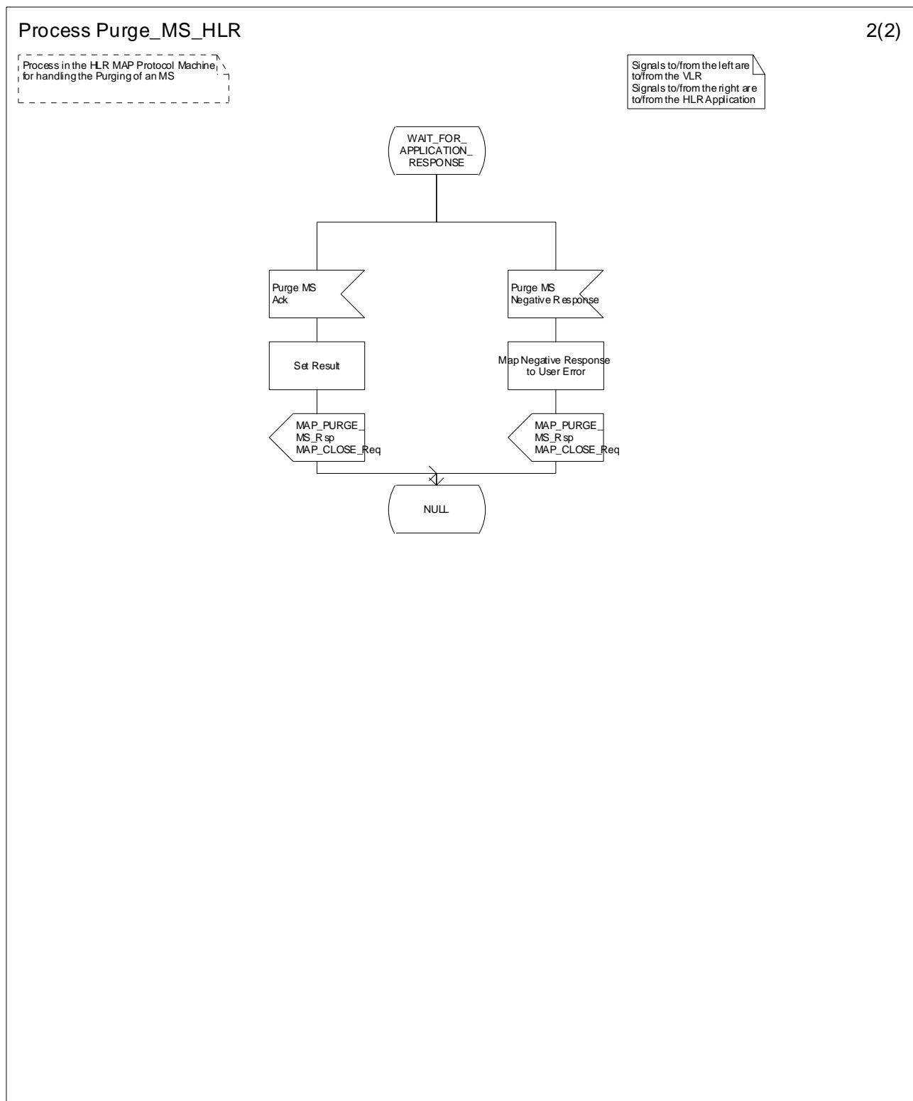
**Figure 19.1.4/3 (Sheet 2 of 2): Process Purge\_MS\_HLR**
