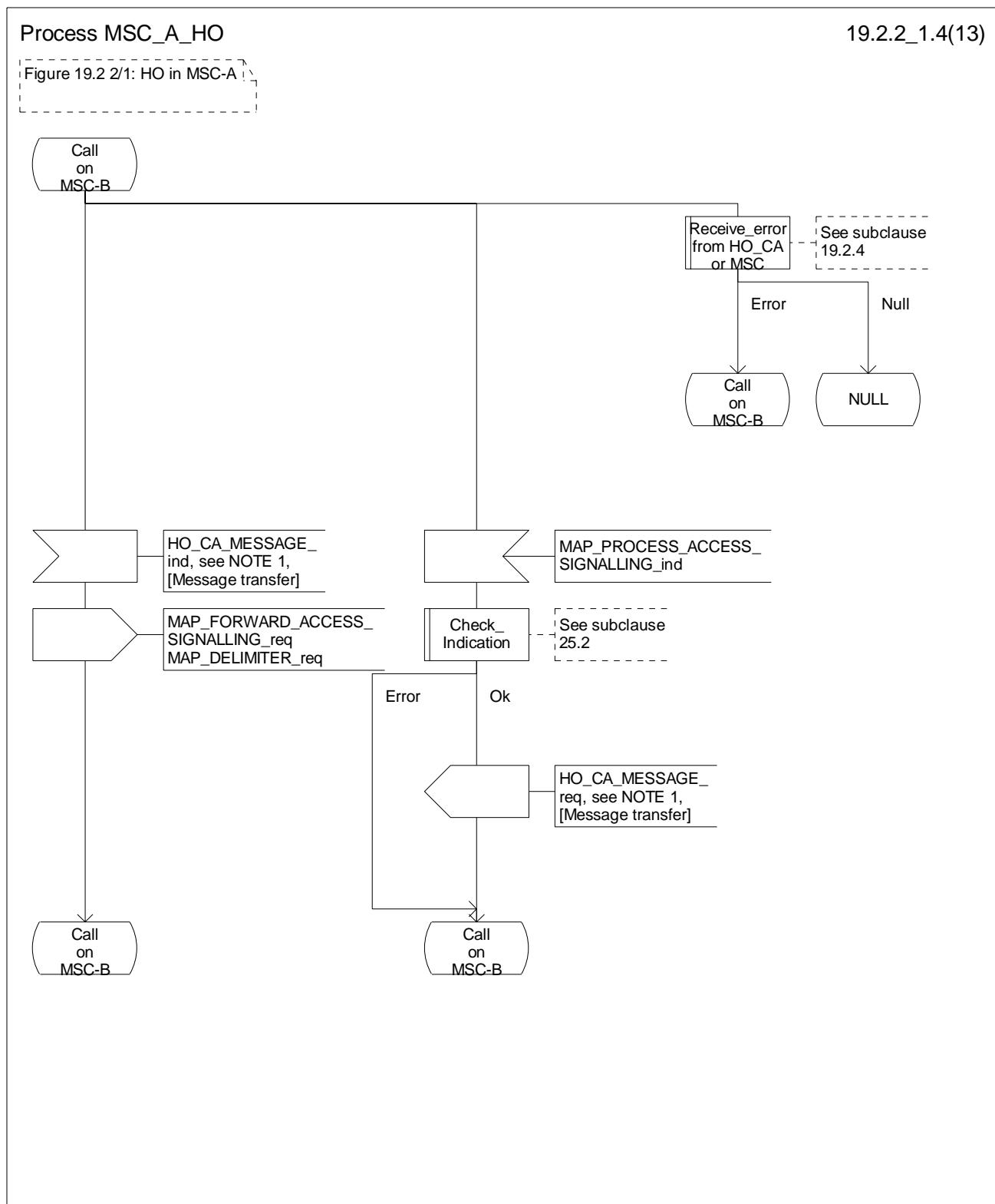
Figure 19.2.2/1 (sheet 4 of 13): Process MSC\_A\_HO
