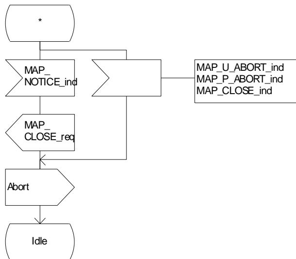
Figure 21.4/3 (sheet 2 of 3): Process ASCI\_Relay\_MSC
