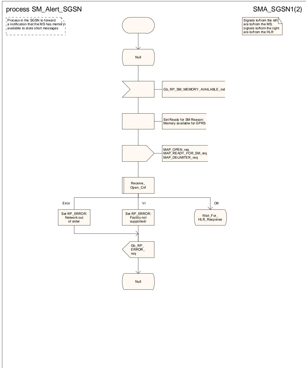
Figure 23.4/8 (sheet 1 of 2): SM\_Alert\_SGSN
