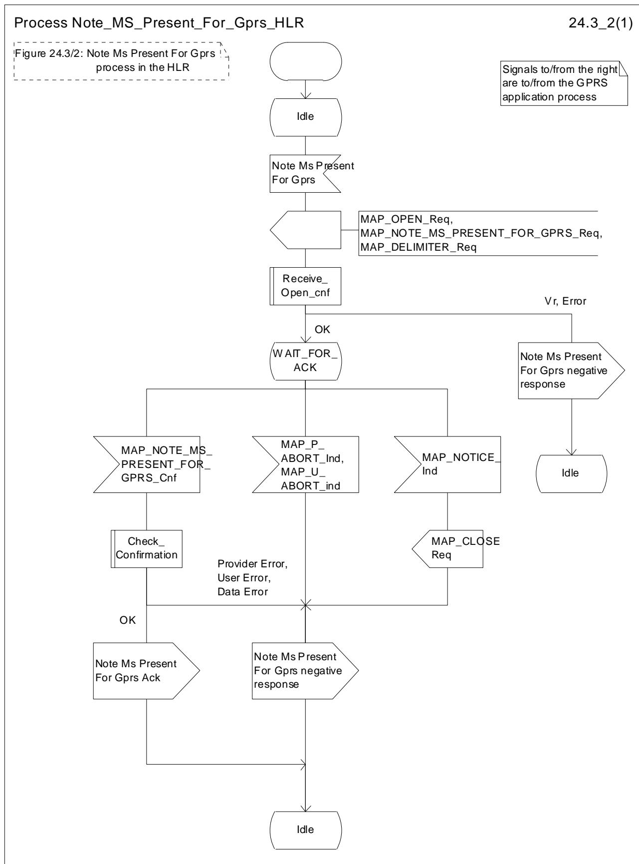
**Figure 24.3/2: Process Note\_MS\_Present\_For\_Gprs\_HLR**
