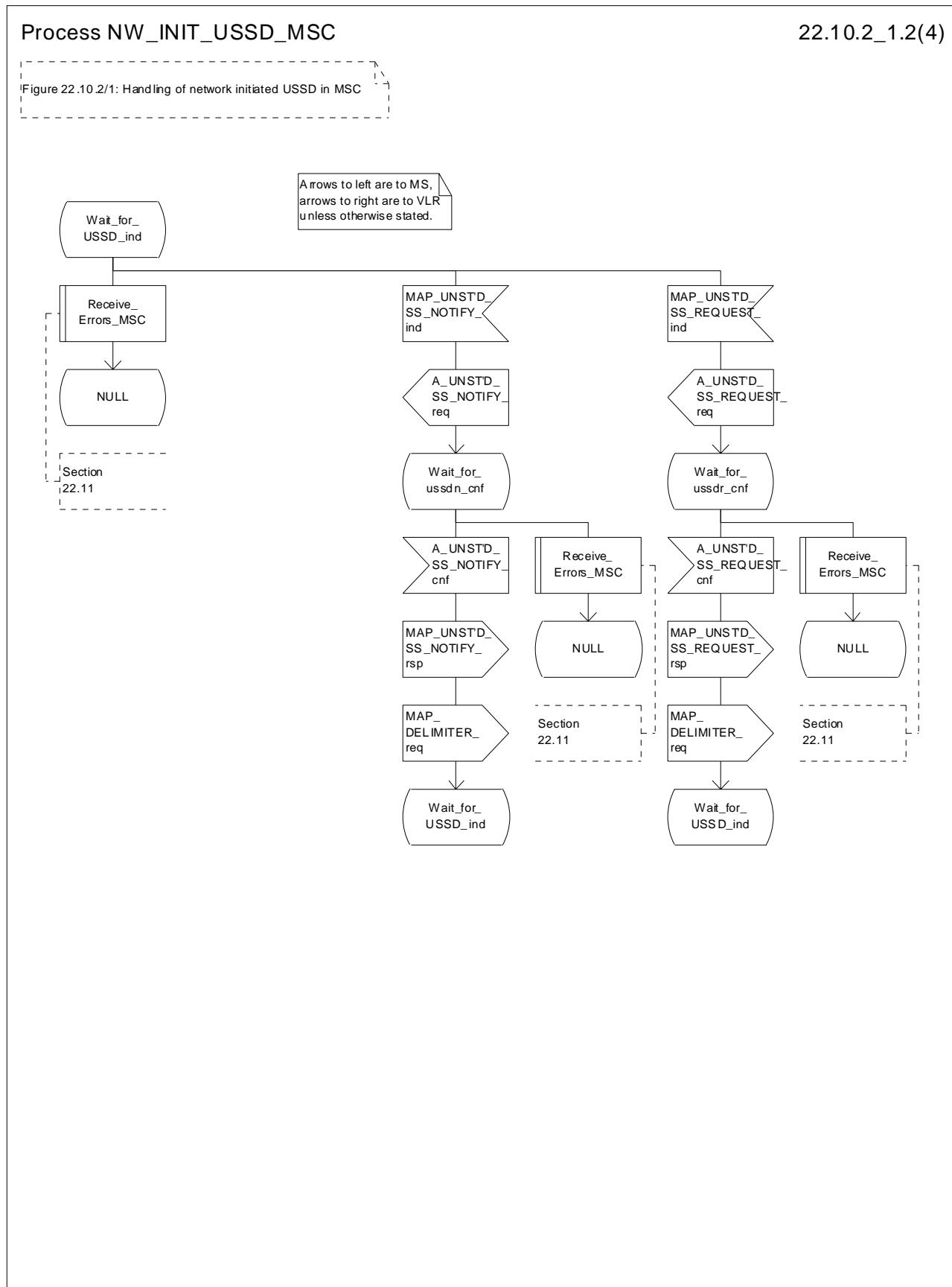
Figure 22.10.2/1 (sheet 2 of 4): Procedure NI\_USSD\_MSC
