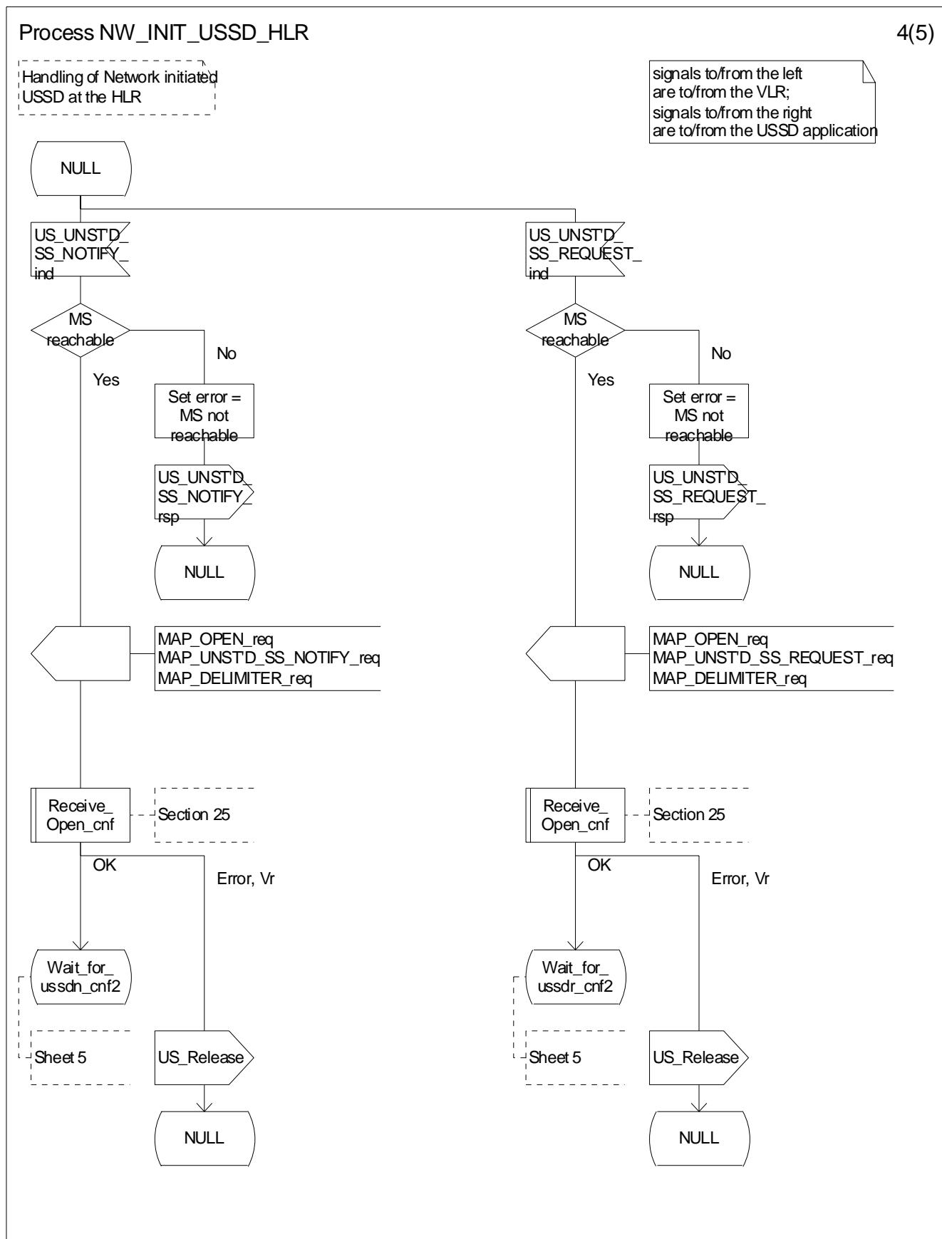
Figure 22.10.4/1 (sheet 4 of 5): Procedure NI\_USSD\_HLR
