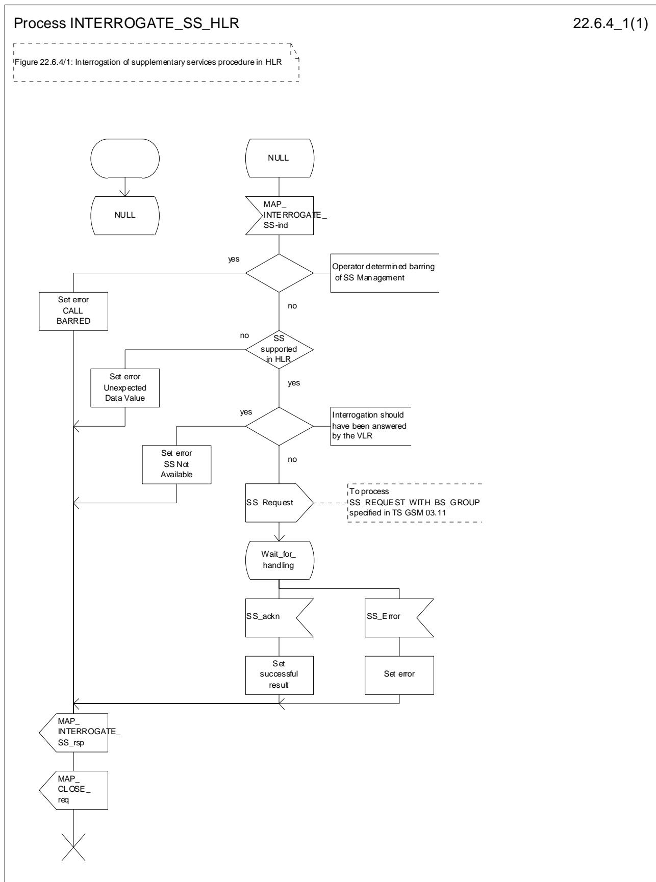
Figure 22.6.4/1: Procedure Interrogate\_SS\_HLR
