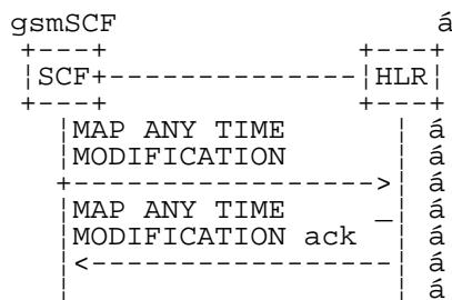
**Figure 24A.2/1: Message flow for any time modification**
