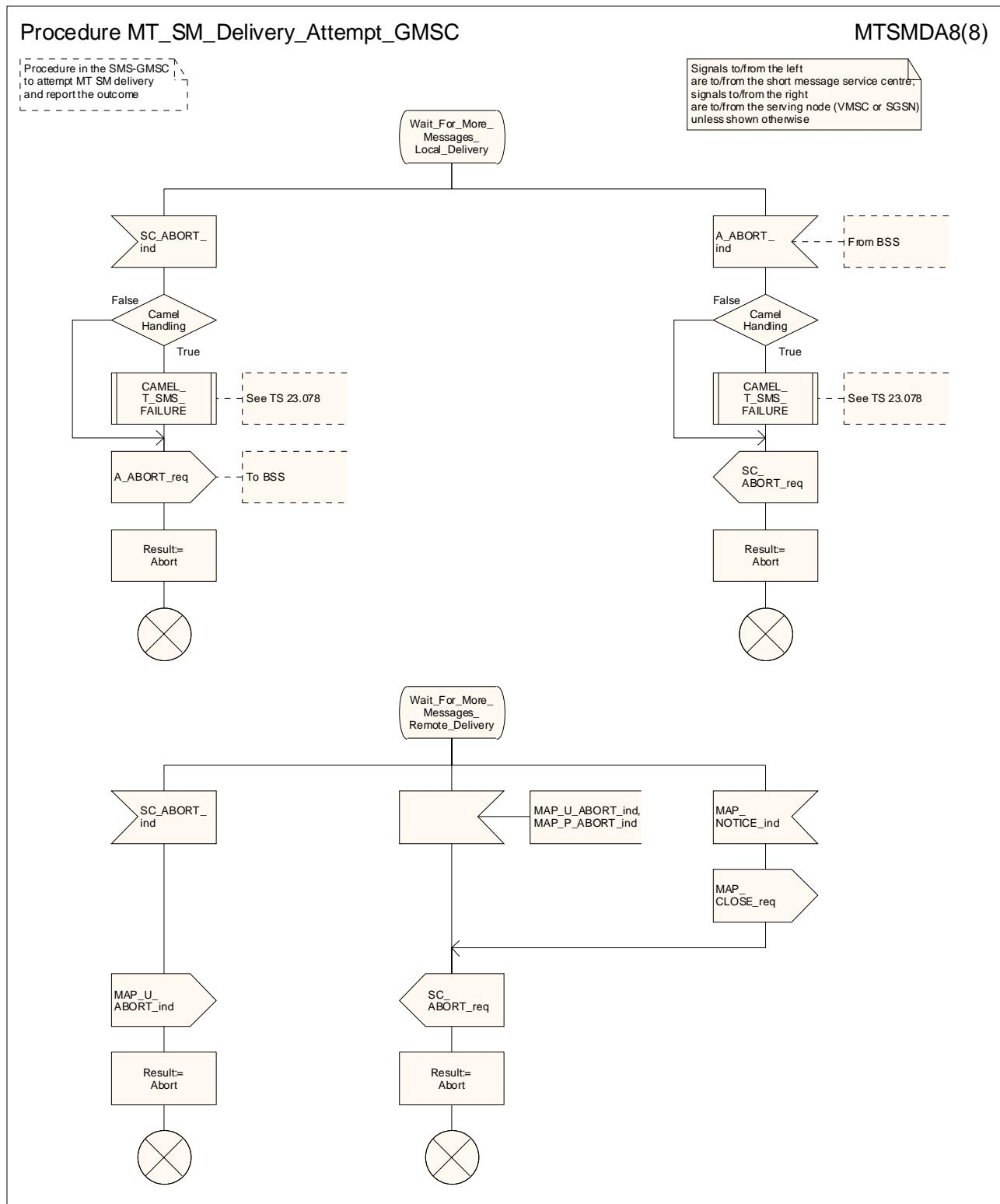
**Figure 23.3/4 (sheet 8 of 8): Procedure MT\_SM\_Delivery\_Attempt\_GMSC**
