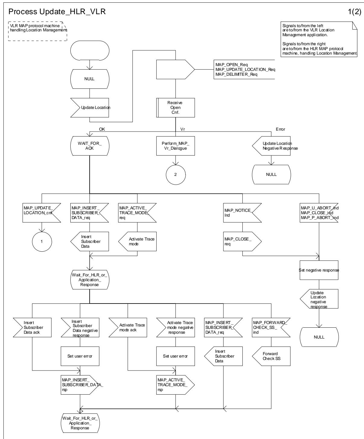
Figure 19.1.1/6 (sheet 1 of 2): Process Update\_HLR\_VLR
