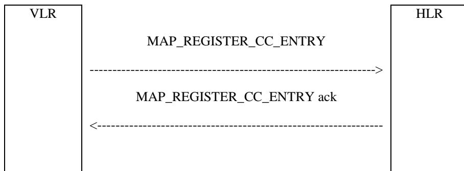
**Figure 22.13.1/1: Message flow to activate a CCBS request**
