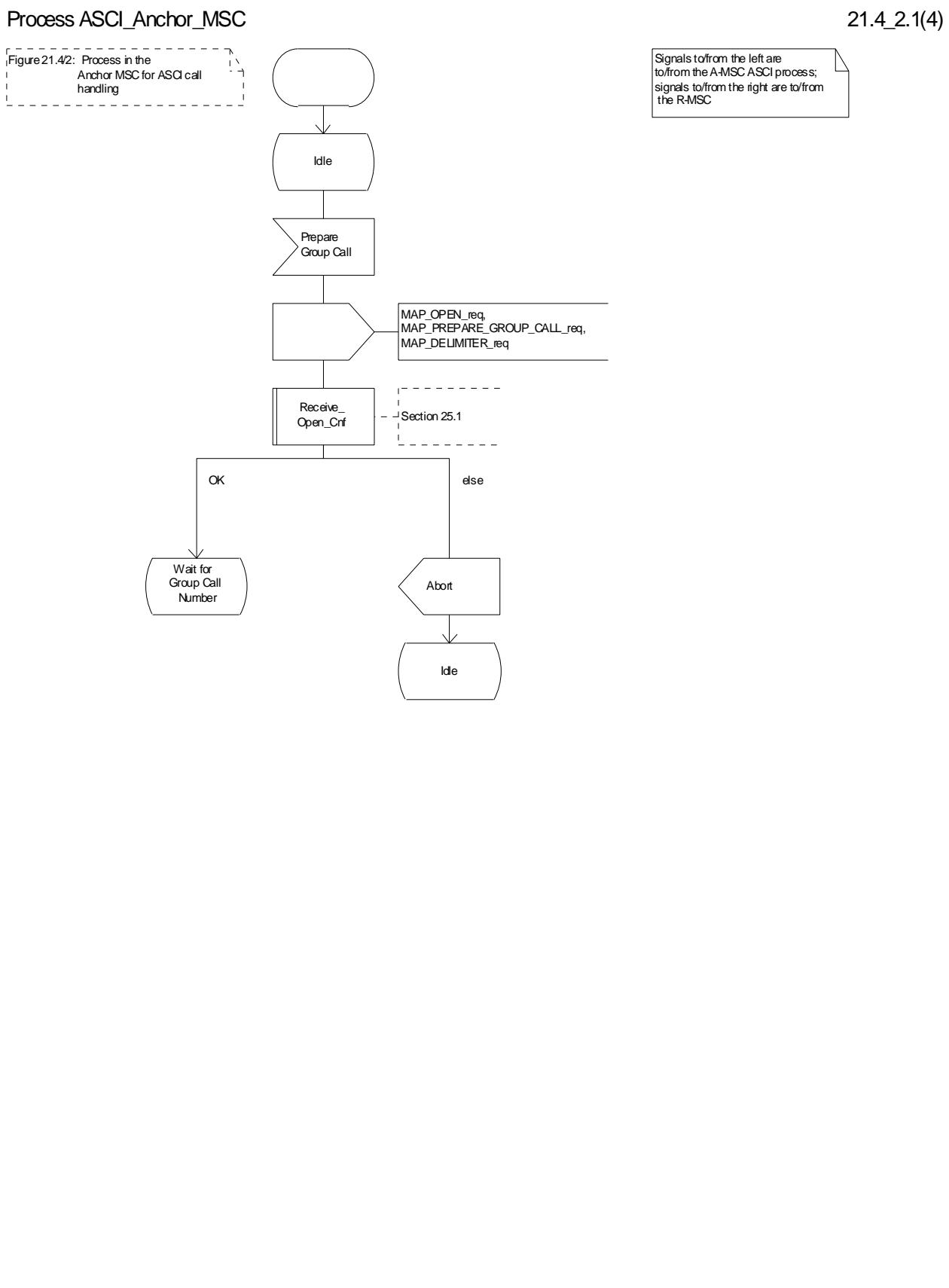
Figure 21.4/2 (sheet 1 of 4): Process ASCI\_Anchor\_MSC
