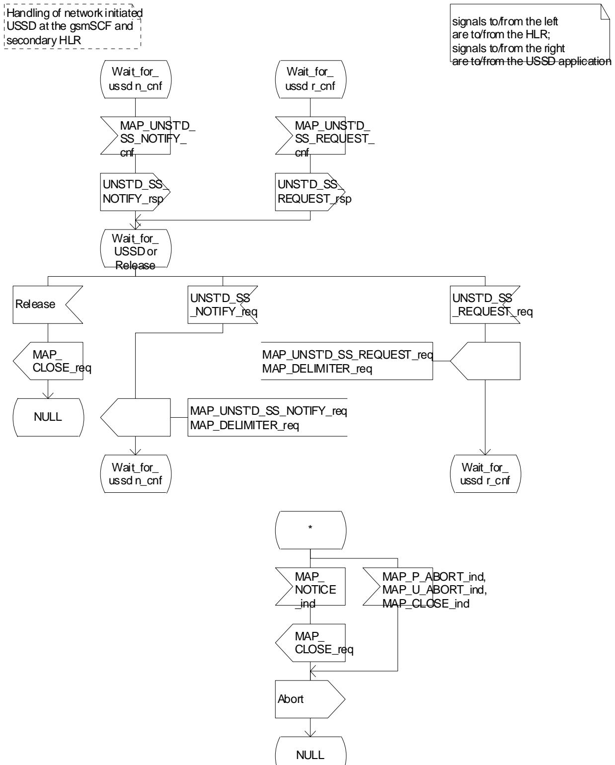
Figure 22.10.5/1 (sheet 2 of 2): Procedure NI\_USSD\_gsmSCF\_secondary\_HLR
