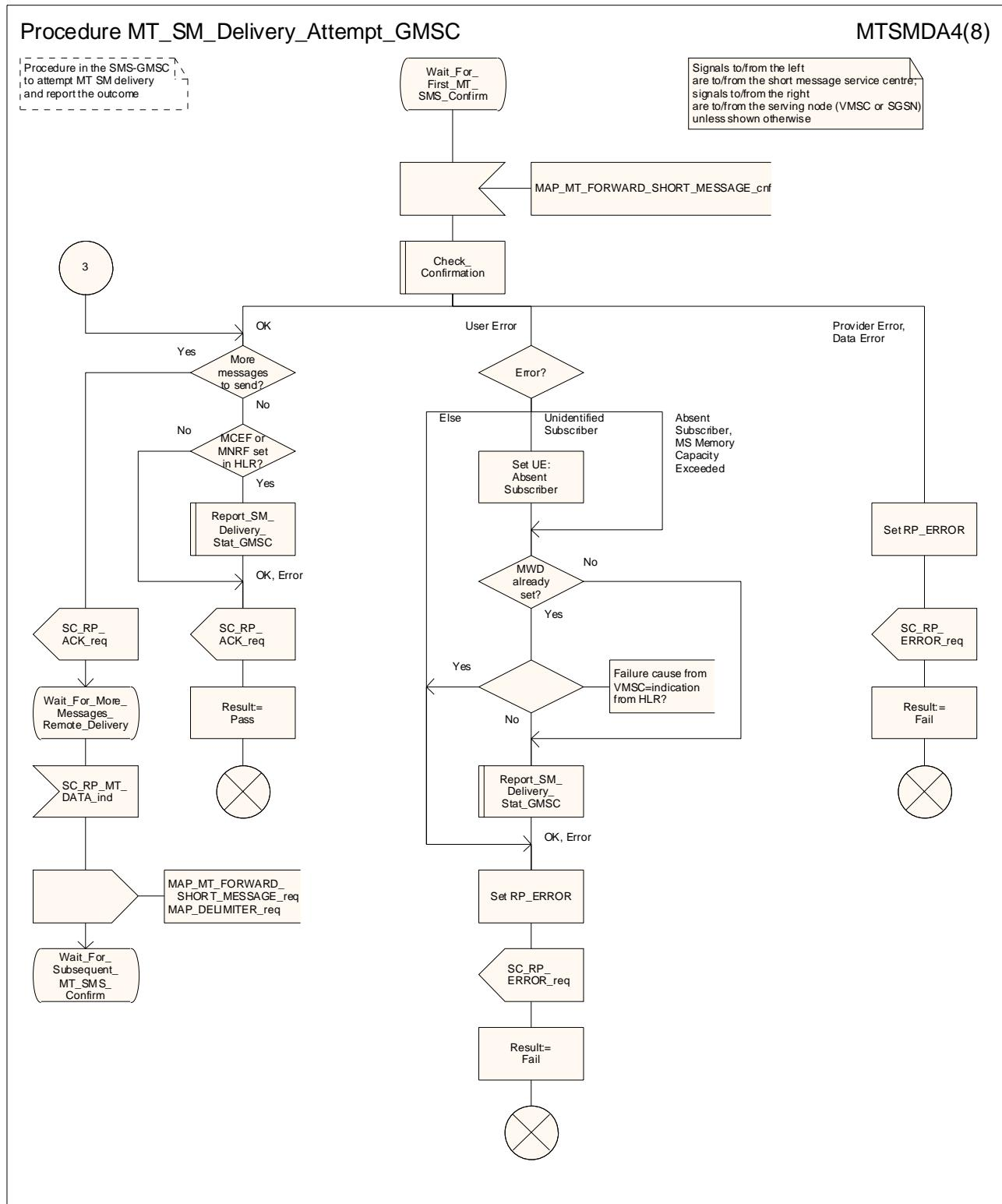
Figure 23.3/4 (sheet 4 of 8): Procedure MT\_SM\_Delivery\_Attempt\_GMSC
