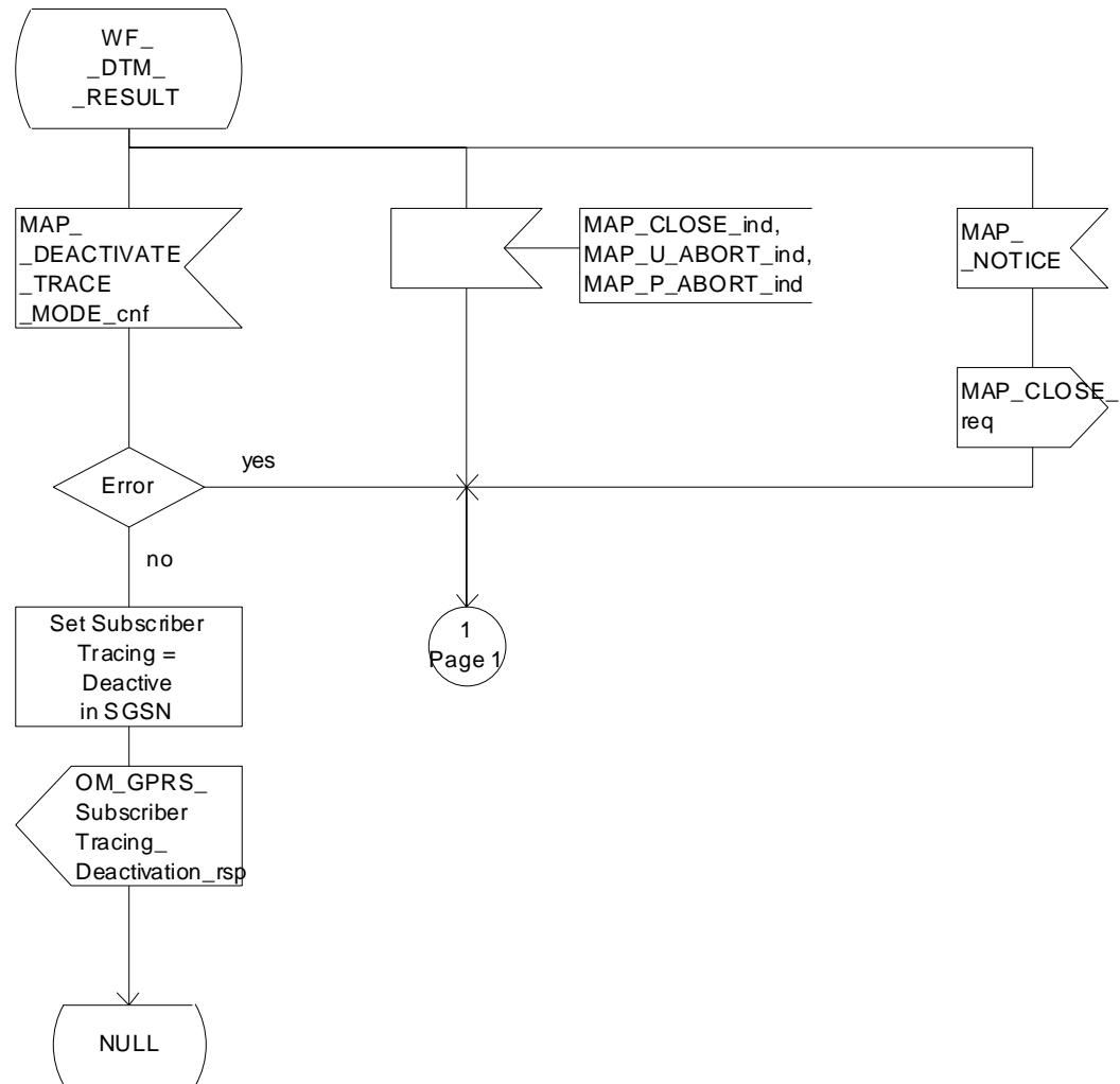
Figure 20.2/15 (sheet 2 of 2): Process DTM\_HLR\_with\_SGSN
