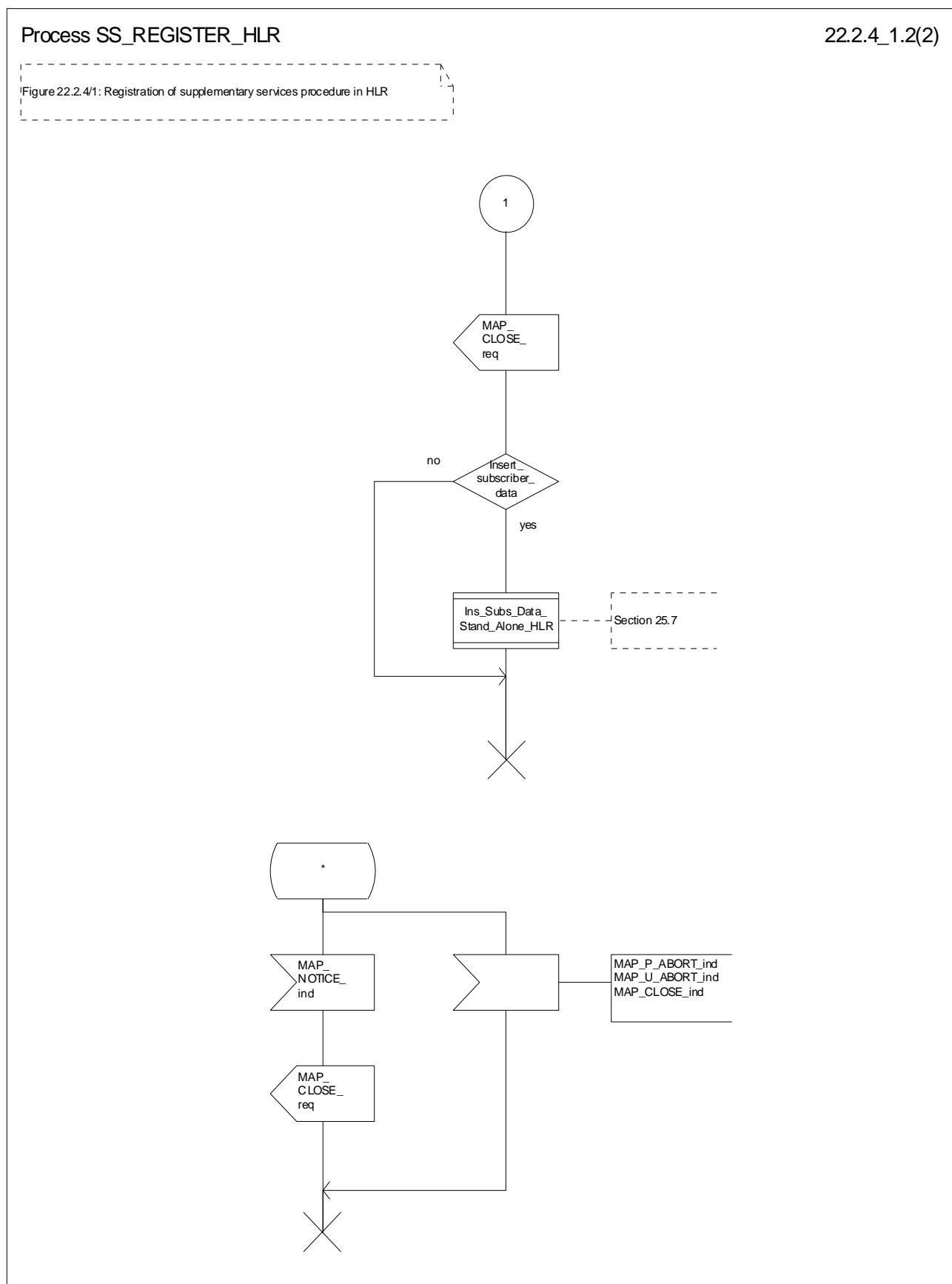
Figure 22.2.4/1 (sheet 2 of 2): Procedure SS\_Register\_HLR
