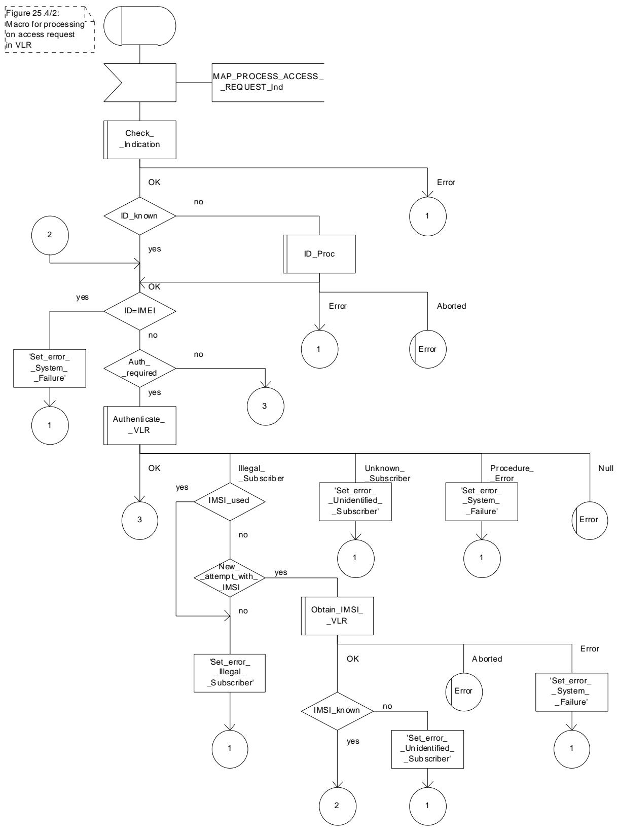
**Figure 25.4/2 (sheet 1 of 3): Macro Process Access Request VLR**
