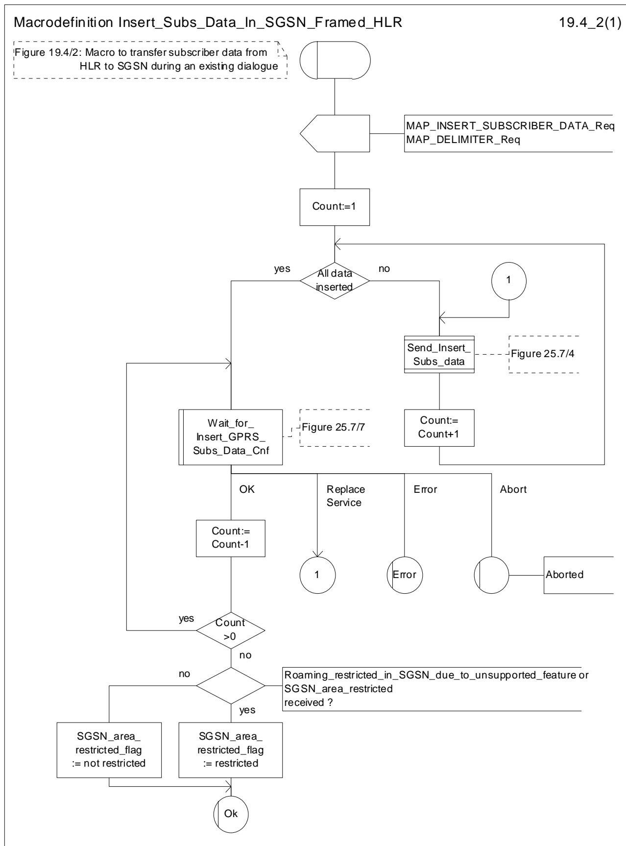
Figure 19.4/2: Macro Insert\_Subs\_Data\_In\_SGSN\_Framed\_HLR
