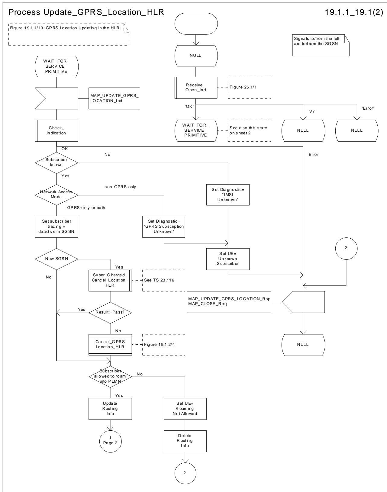
Figure 19.1.1/19 (sheet 1 of 2): Process Update\_GPRS\_Location\_HLR
