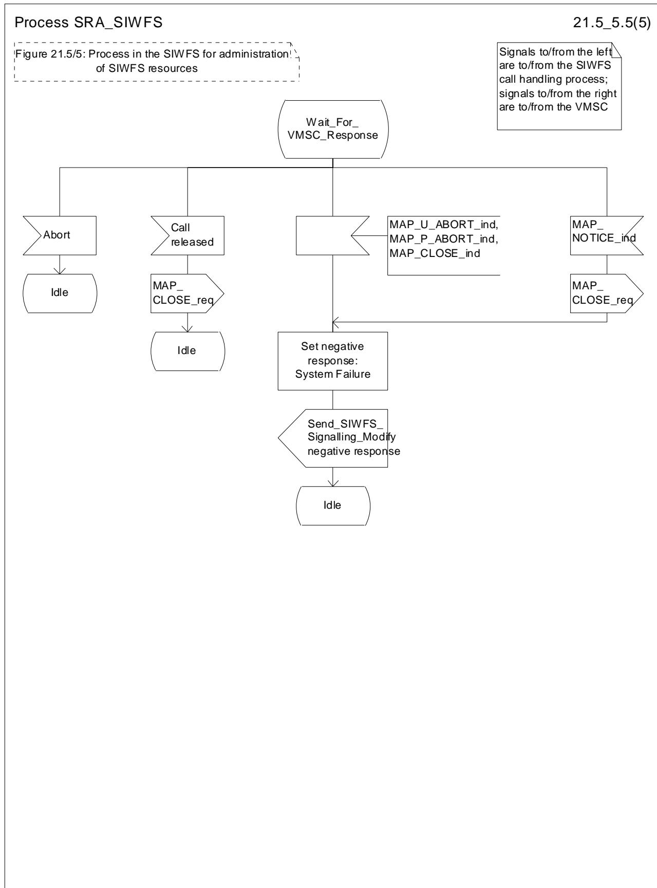
Figure 21.5/5 (sheet 5 of 5): Process SRA\_SIWFs
