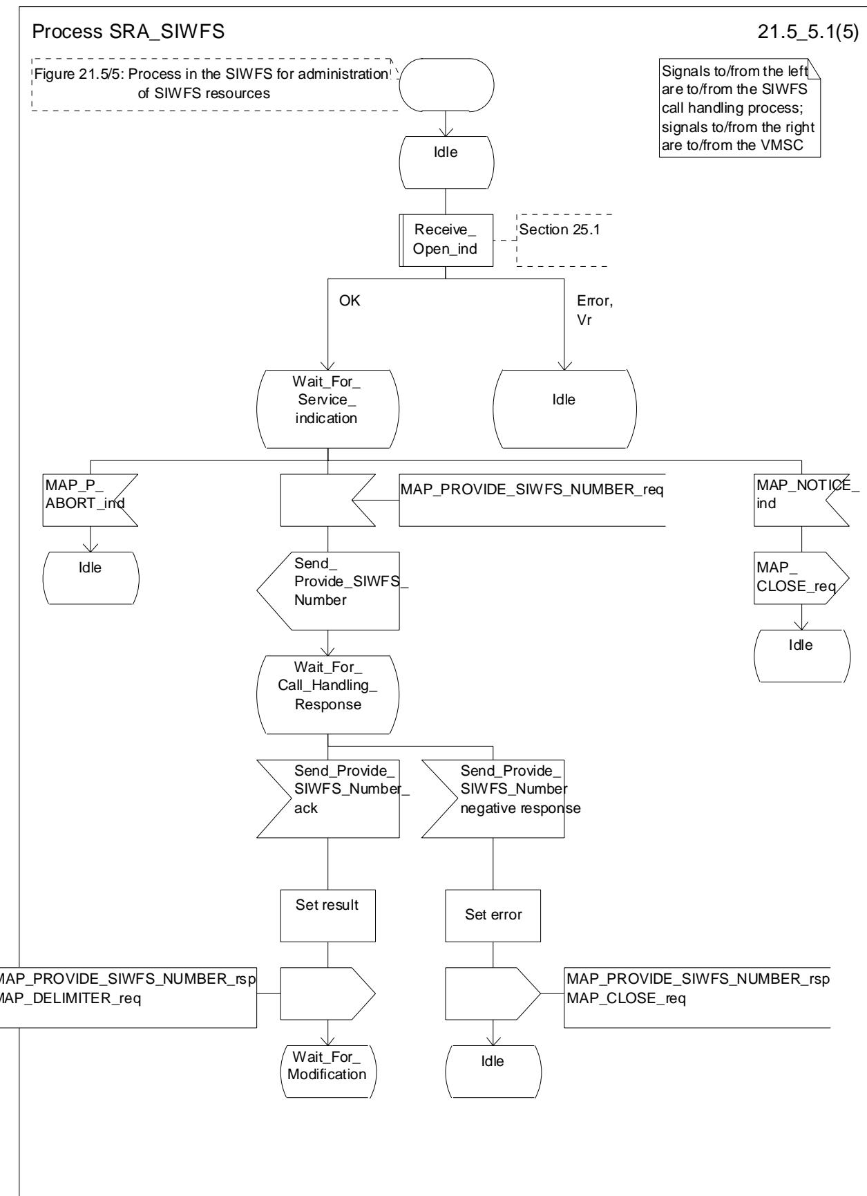
Figure 21.5/5 (sheet 1 of 5): Process SRA\_SIWFs
