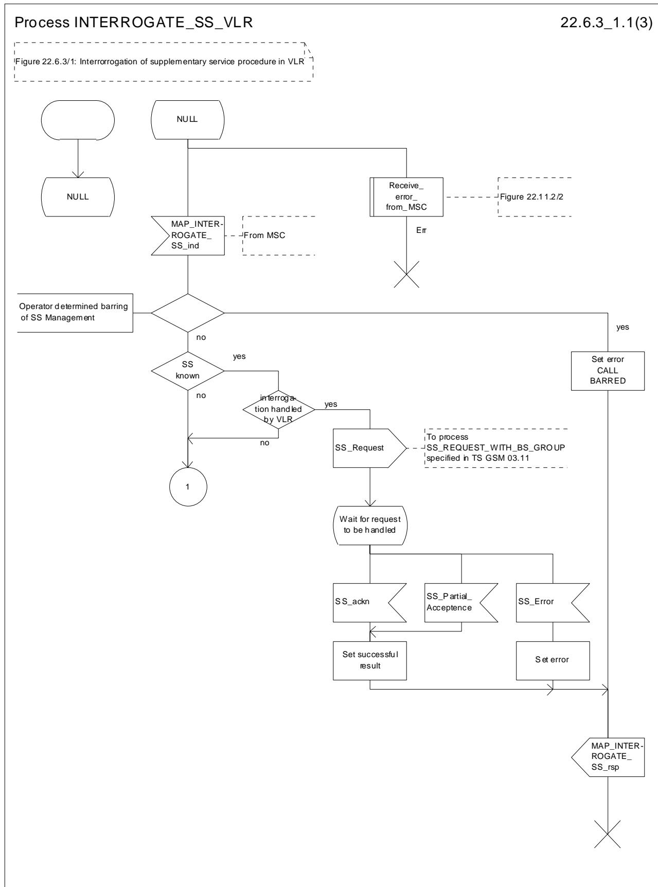
Figure 22.6.3/1 (sheet 1 of 3): Procedure Interrogate\_SS\_VLR
