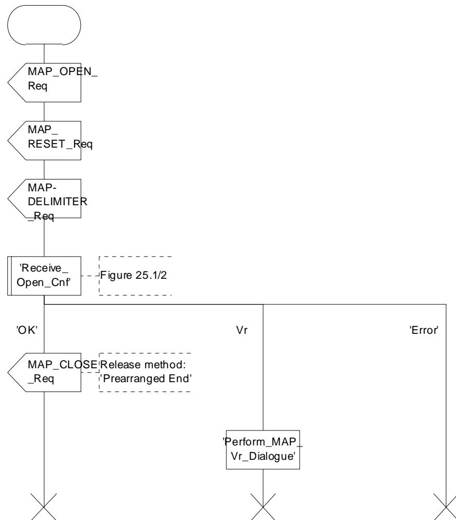
Figure 19.3/7: Process SEND\_RESET\_TO\_SGSN
