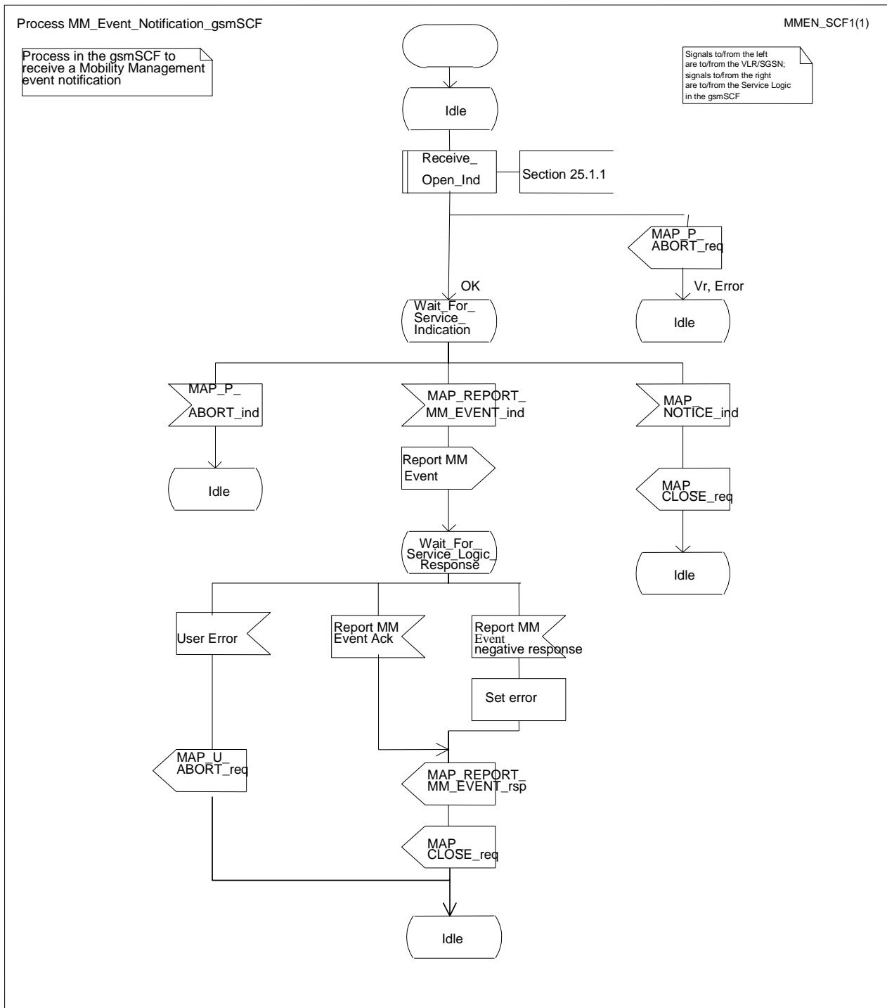
Figure 19.5/3: Process MM\_Event\_Notification\_gsmSCF (sheet 1 of 1)
