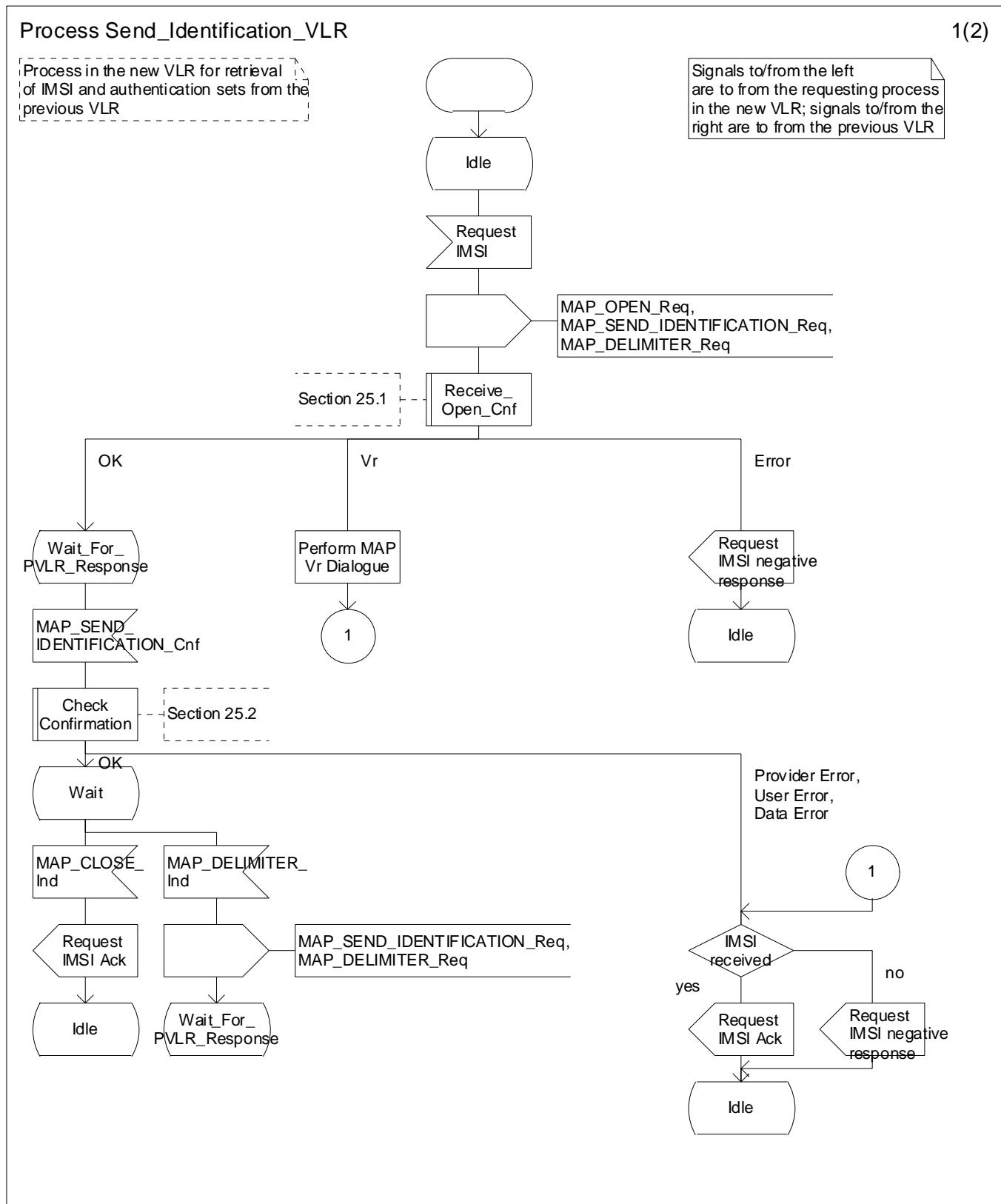
Figure 19.1.1/XX (sheet 1 of 2): Process Send\_Identification\_VLR
