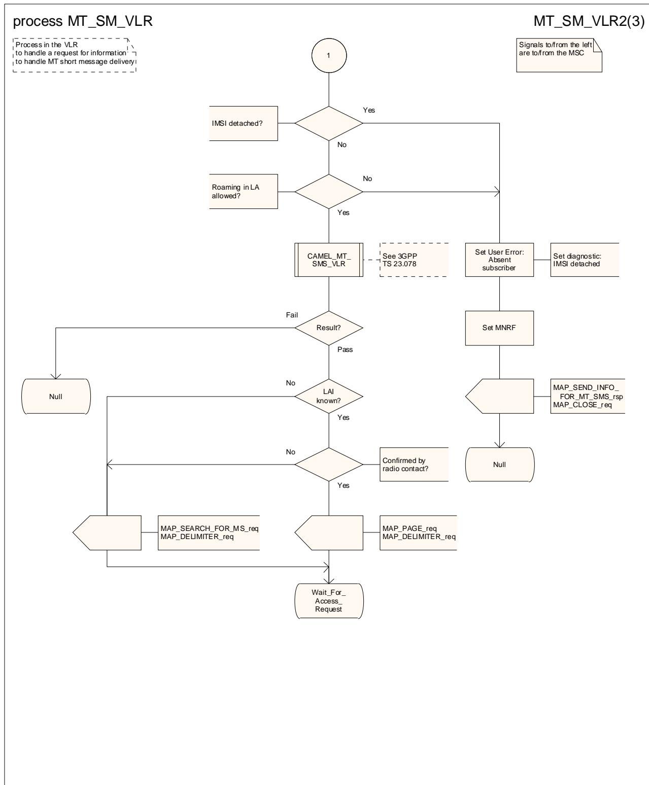
**Figure 23.3/9 (sheet 2 of 3): Process MT\_SM\_VLR**
