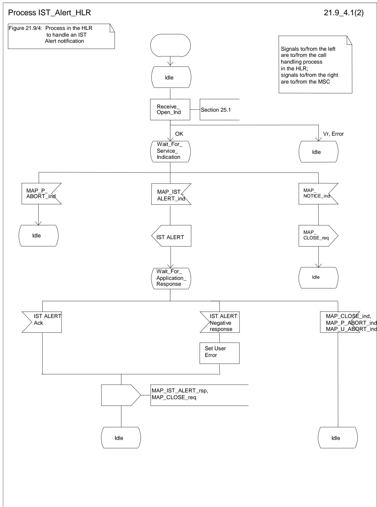
Figure 21.9/3: Process IST\_Alert\_HLR
