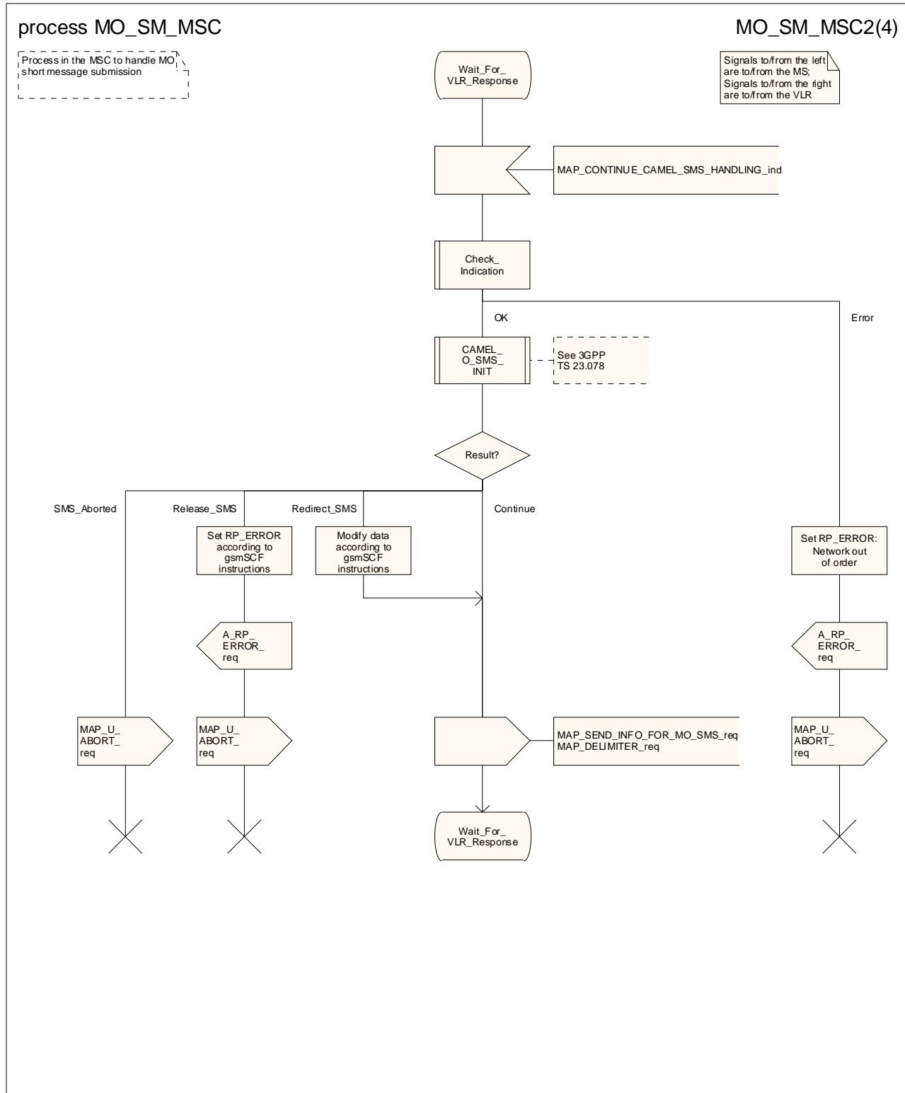
Figure 23.2/2 (sheet 2 of 4): Process MO\_SM\_MSC
