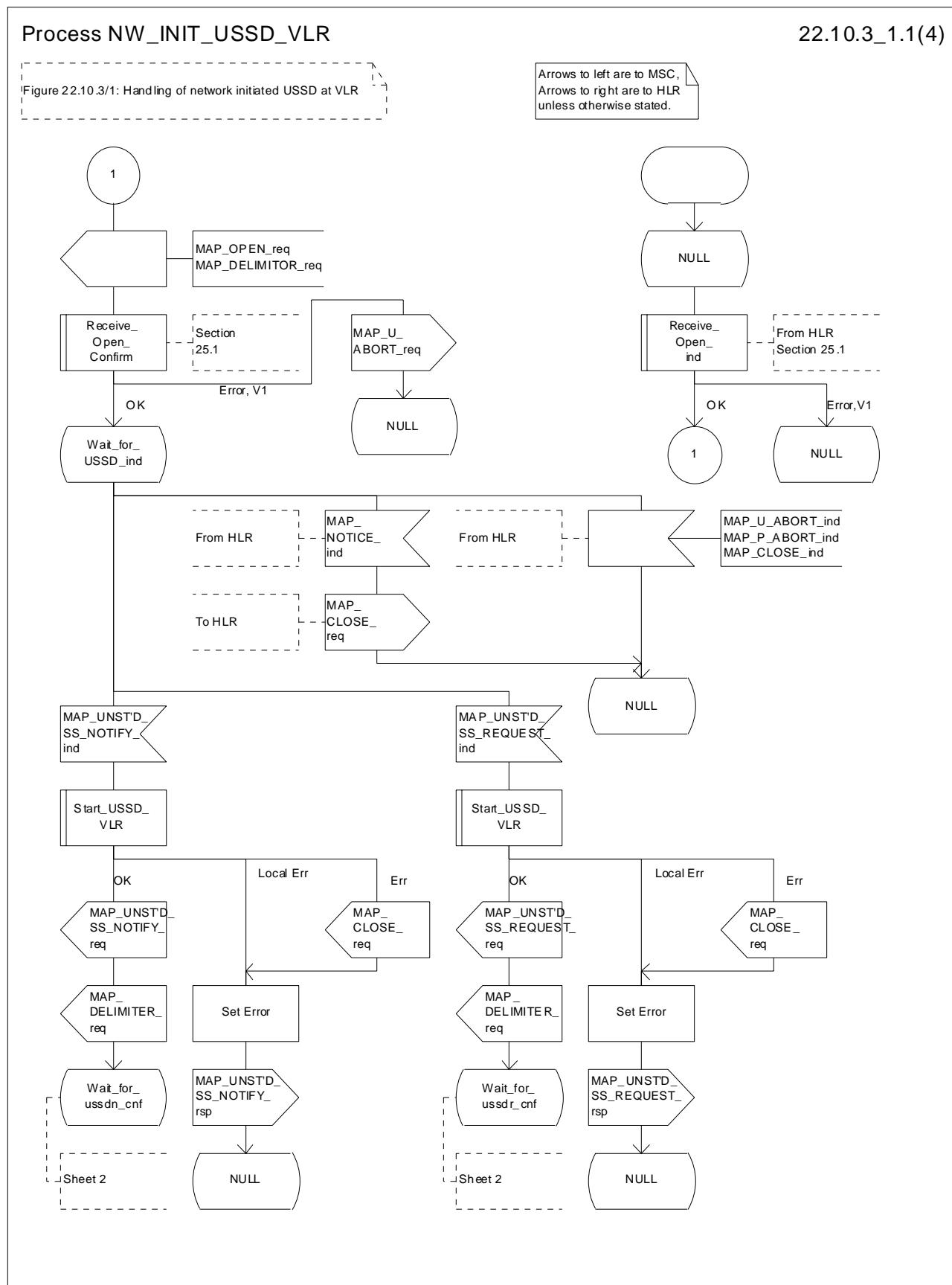
**Figure 22.10.3/1 (sheet 1 of 4): Procedure NI USSD VLR**
