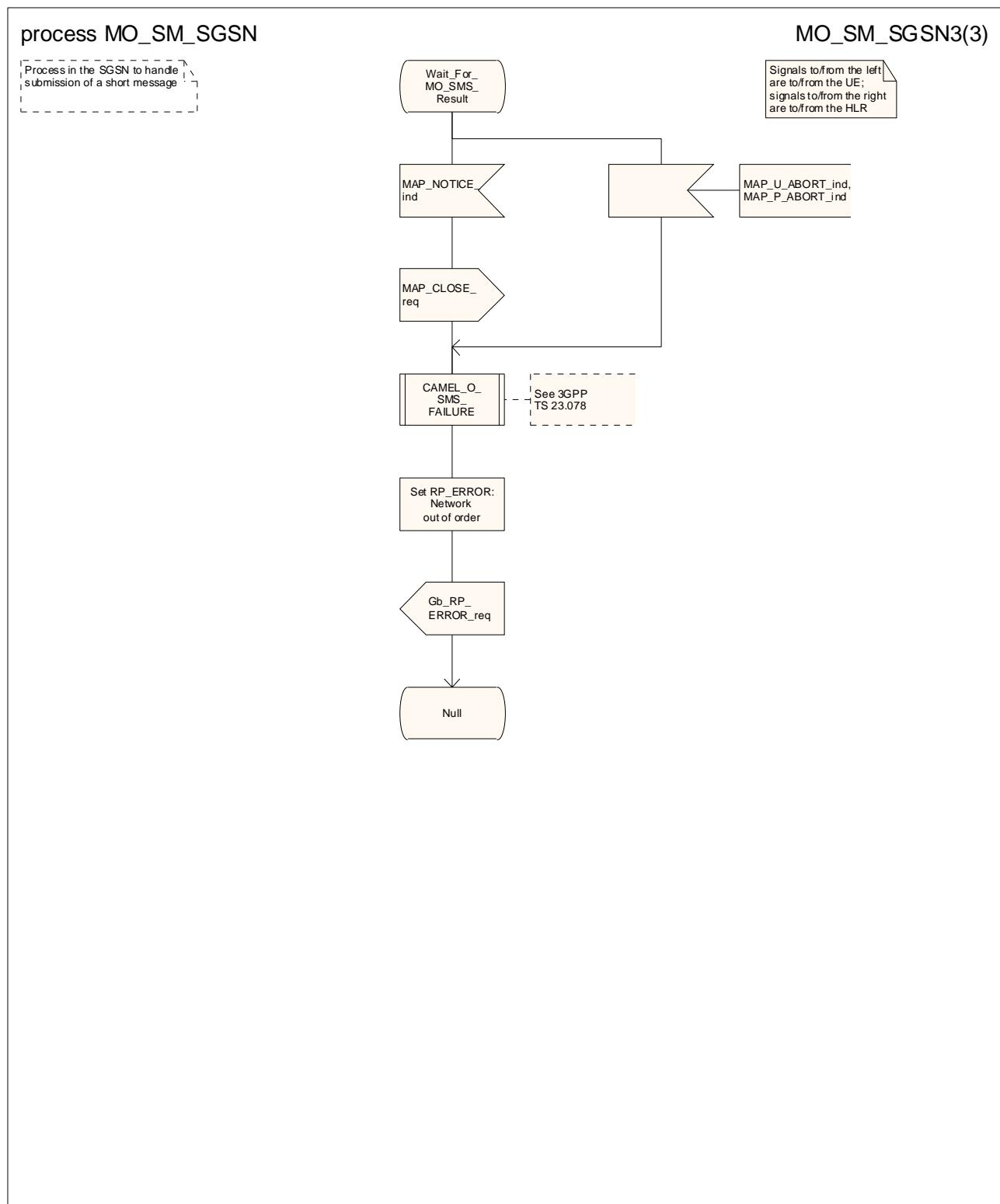
Figure 23.2/5 (sheet 3 of 3): Process MO\_SM\_SGSN
