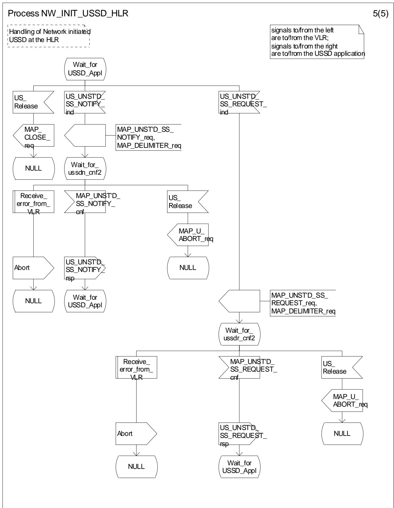
Figure 22.10.4/1 (sheet 5 of 5): Procedure NI\_USSD\_HLR
