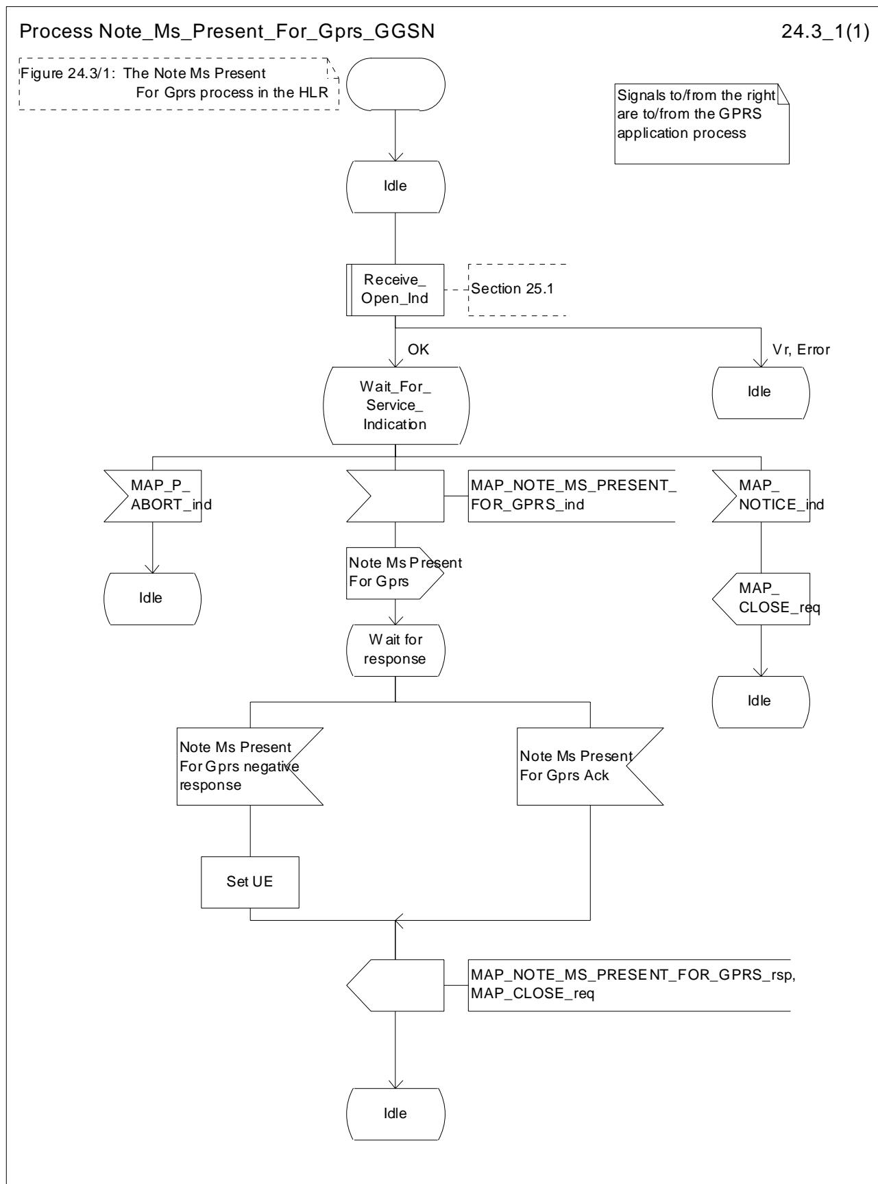
Figure 24.3/1: Process Note\_Ms\_Present\_For\_Gprs\_GGSN
