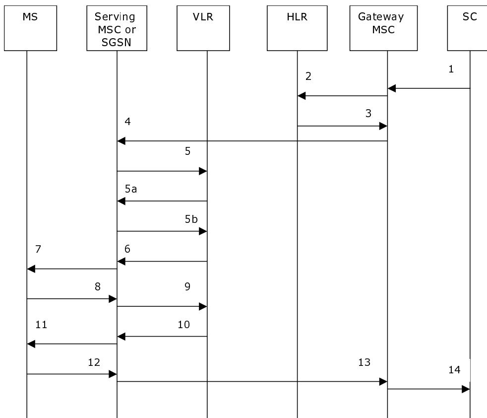
**Figure 23.3/1: Mobile terminated short message service procedures**
