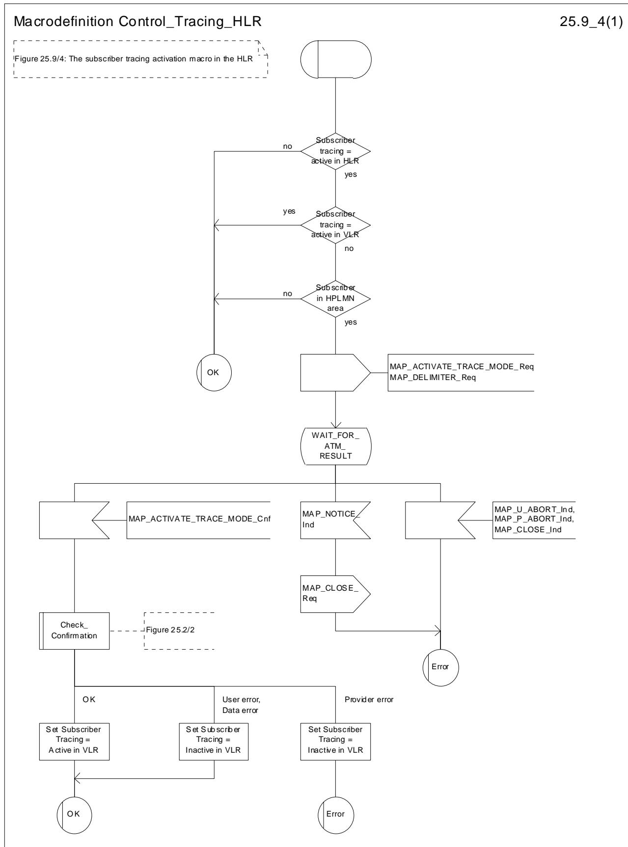
Figure 25.9/4: Macro Control\_Tracing\_HLR
