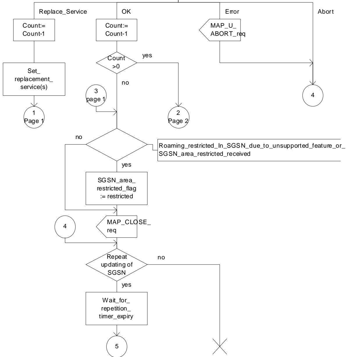
Figure 25.7/5 (sheet 2 of 2): Process Insert\_GPRS\_Subs\_Data\_Stand\_Alone\_HLR
