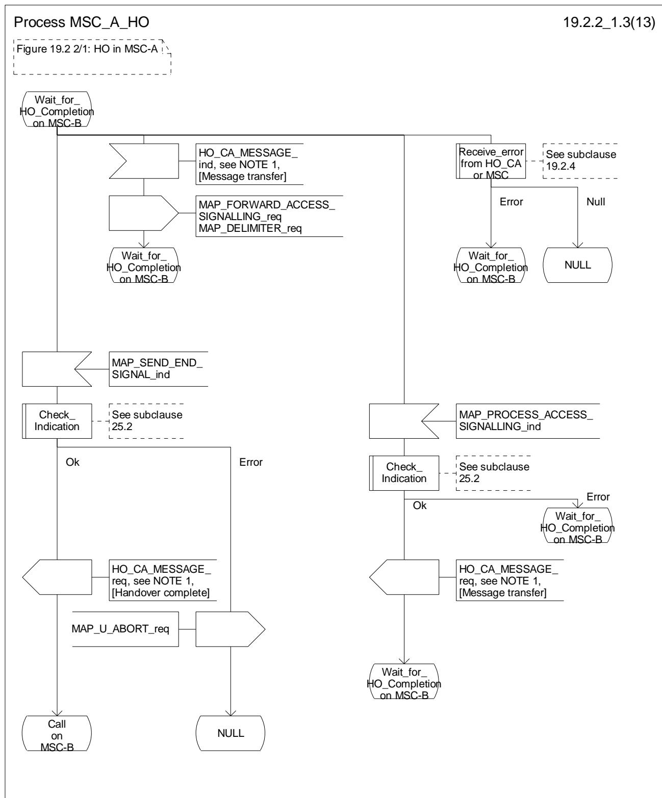
Figure 19.2.2/1 (sheet 3 of 13): Process MSC\_A\_HO
