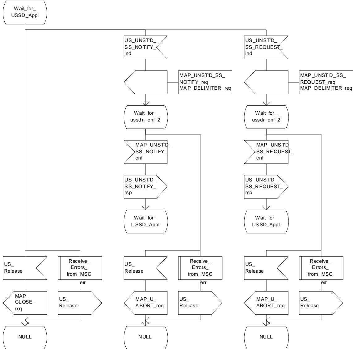
Figure 22.10.3/1 (sheet 4 of 4): Procedure NI\_USSD\_VLR
