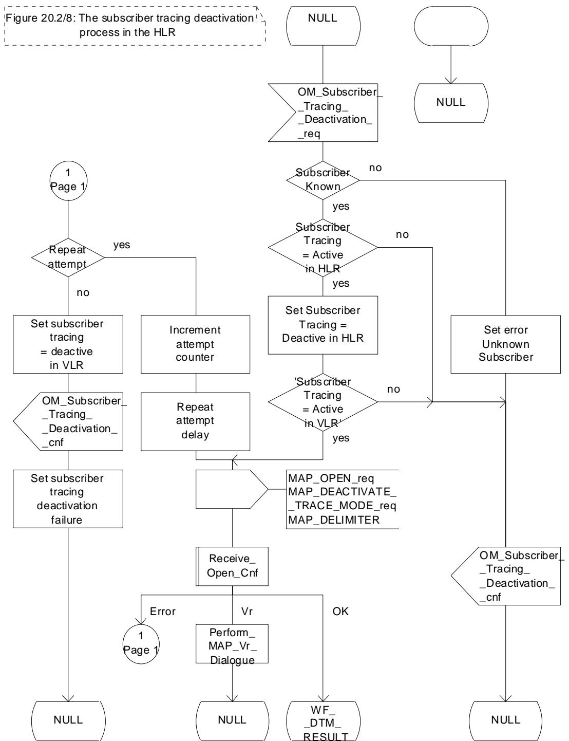
Figure 20.2/8 (sheet 1 of 2): Process DTM\_HLR\_with\_VLR
