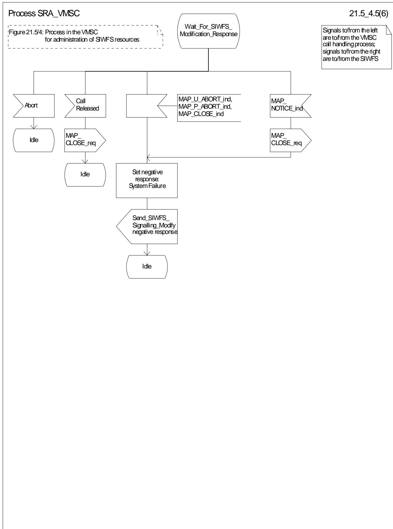
Figure 21.5/4 (sheet 5 of 6): Process SRA\_VMSC
