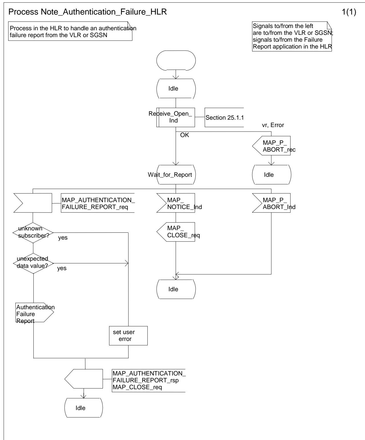
Figure 25.6/10: Process Note\_Authentication\_Failure\_HLR
