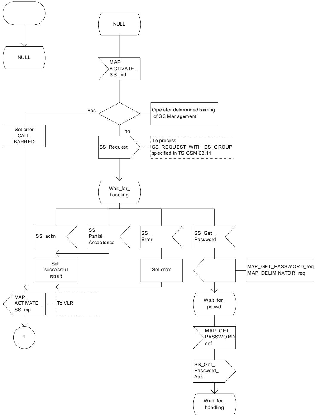
Figure 22.4.4/1 (sheet 1 of 2): Procedure Activate\_SS\_HLR
