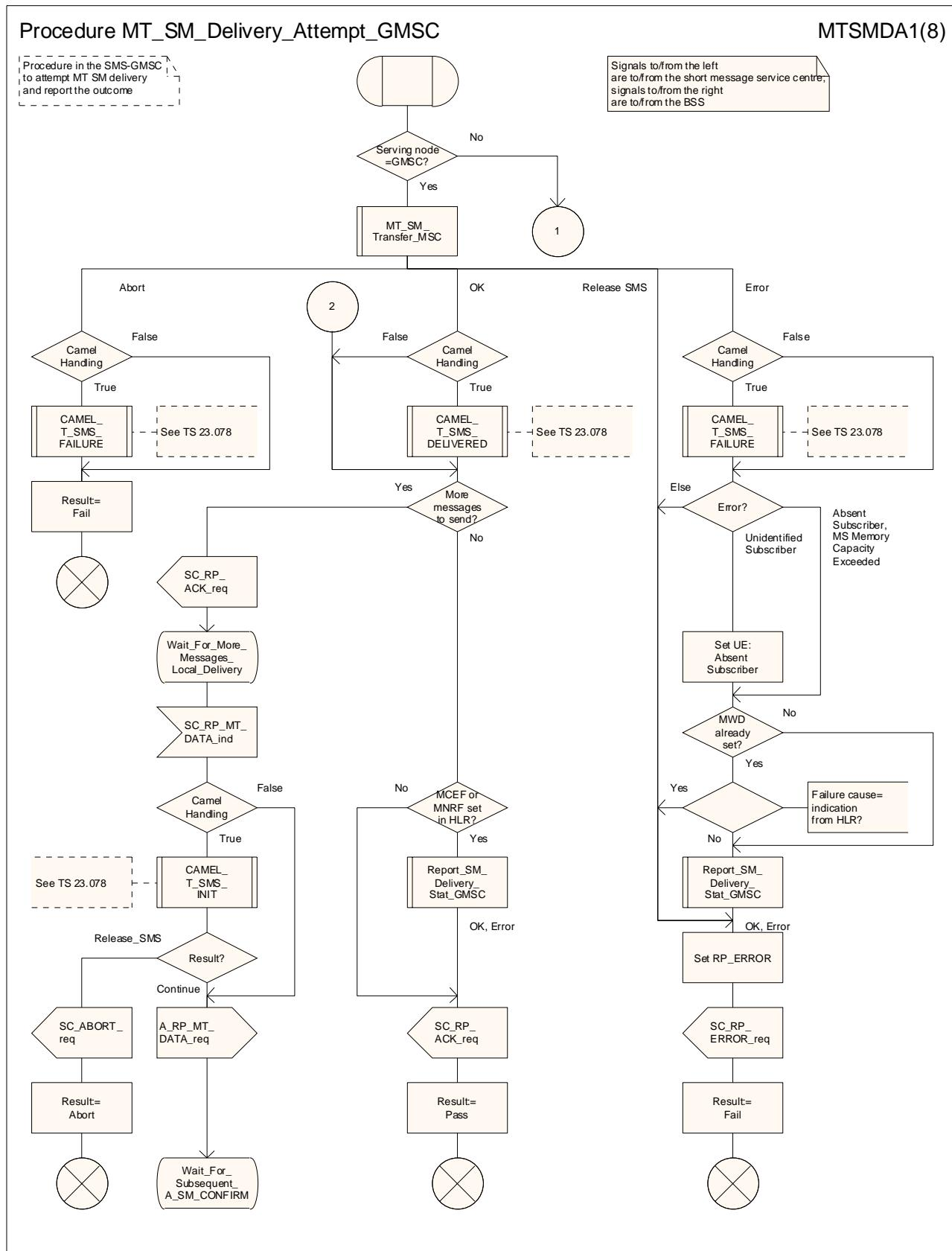
Figure 23.3/4 (sheet 1 of 8): Procedure MT\_SM\_Delivery\_Attempt\_GMSC
