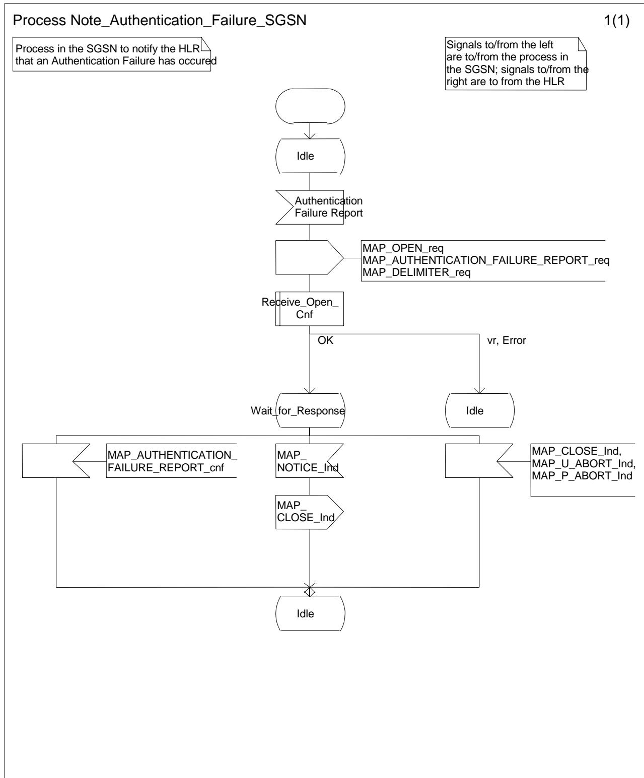
Figure 25.6/9: Process Note\_Authentication\_Failure\_SGSN
