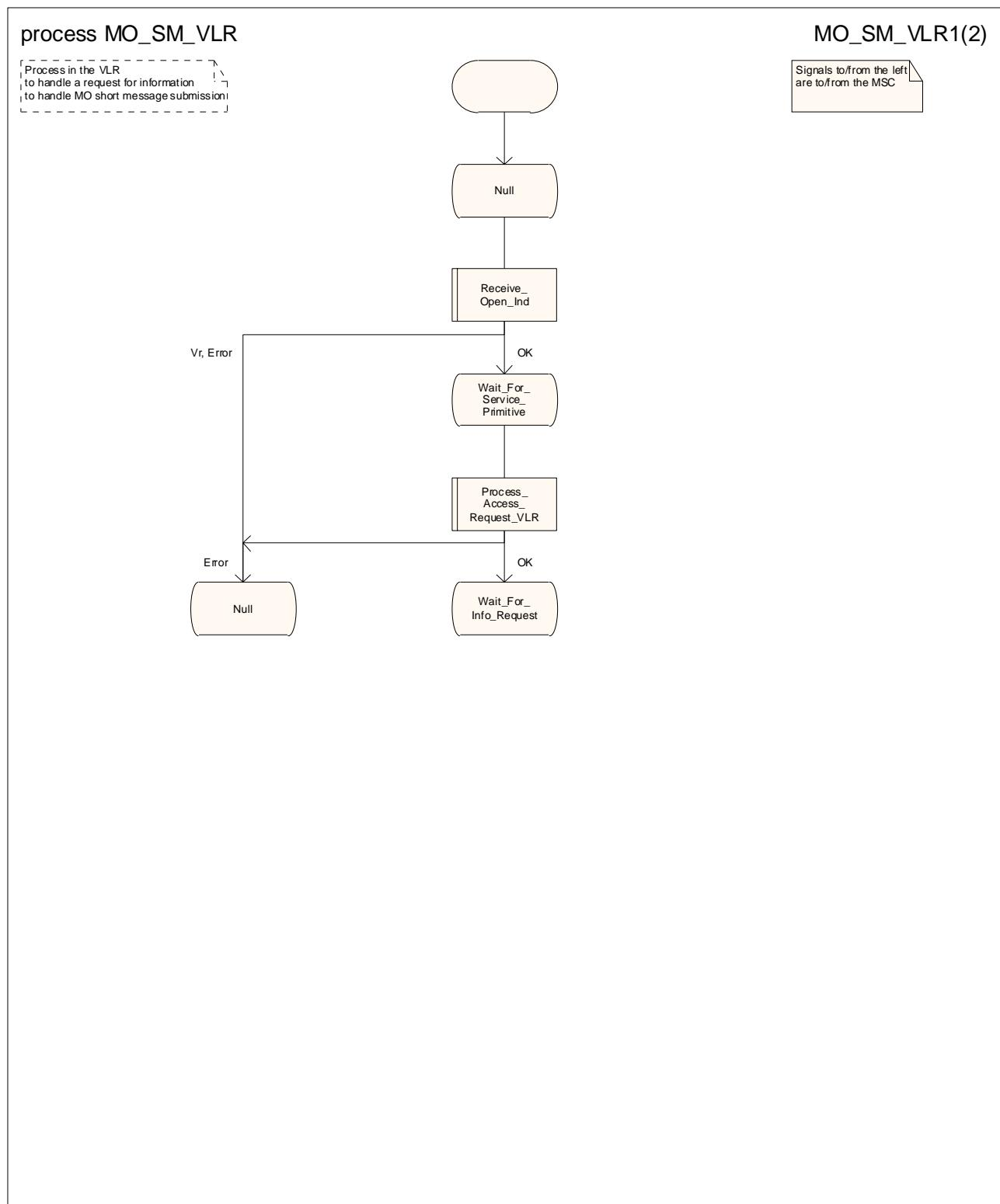
Figure 23.2/3 (sheet 1 of 2): Process MO\_SM\_VLR
