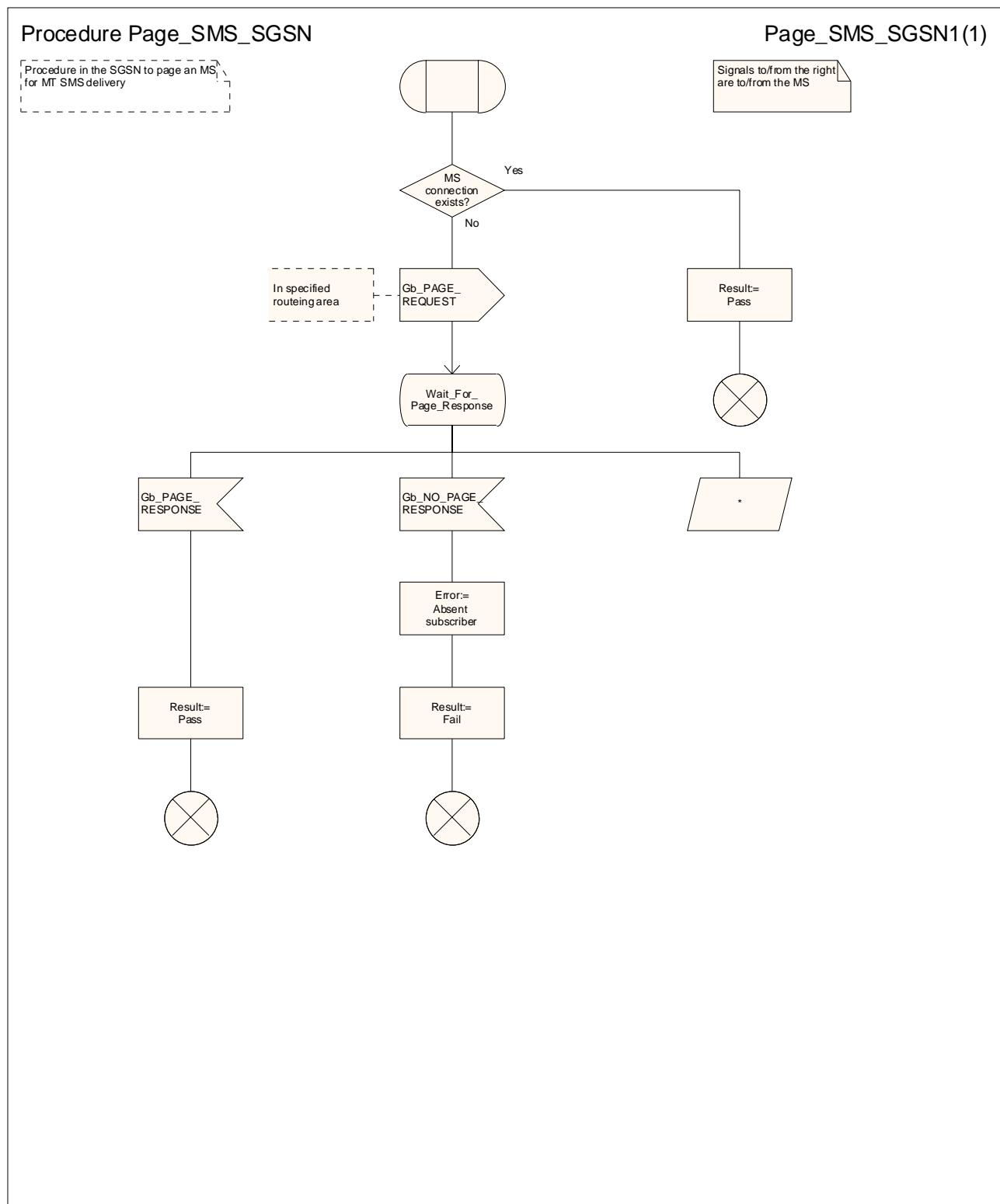
Figure 23.3/12 (sheet 1 of 1): Procedure Page\_SMS\_SGSN
