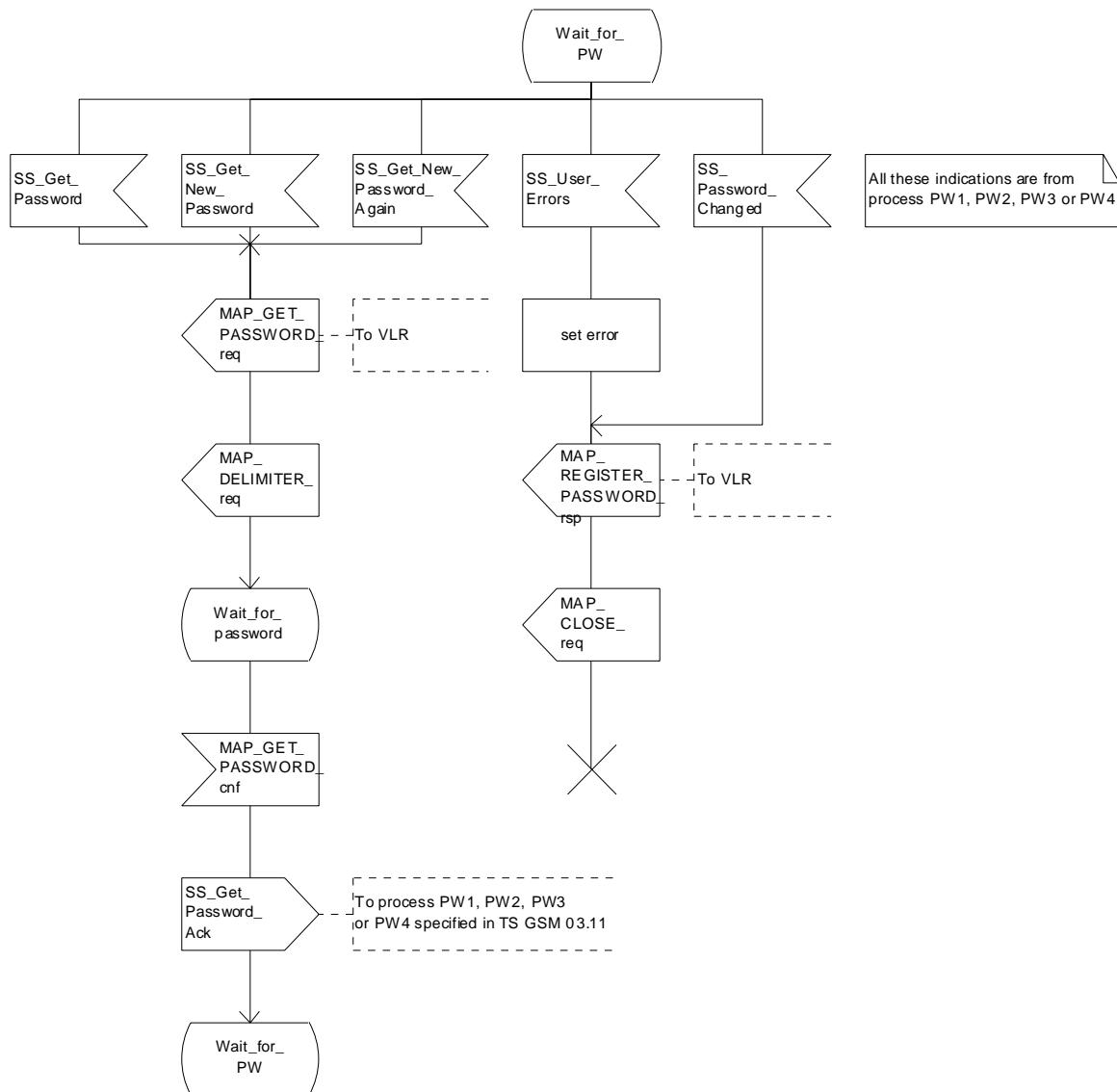
**Figure 22.8.4/1 (sheet 2 of 2): Procedure Register\_PW\_HLR**
