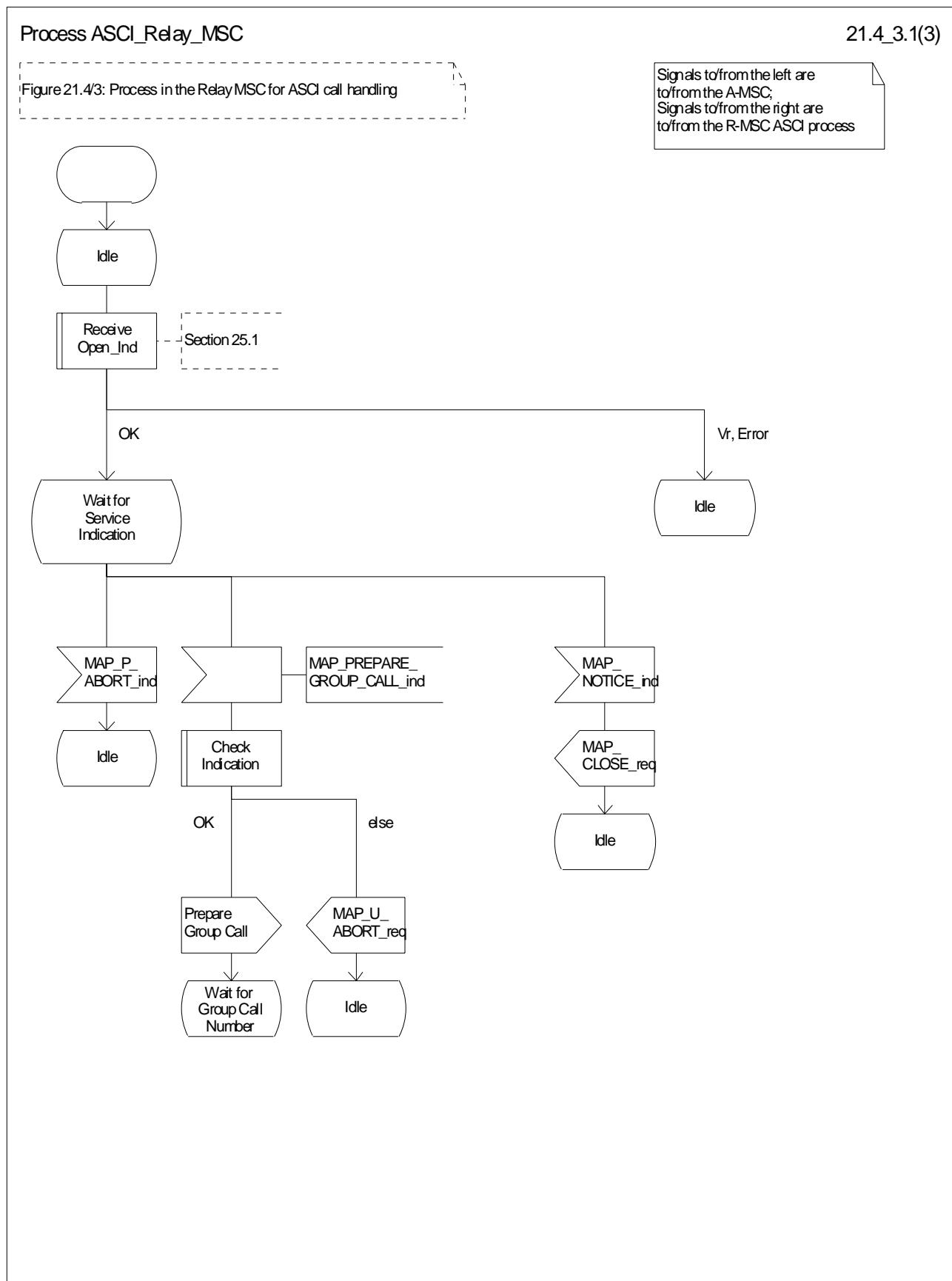
Figure 21.4/3 (sheet 1 of 3): Process ASCI\_Relay\_MSC
