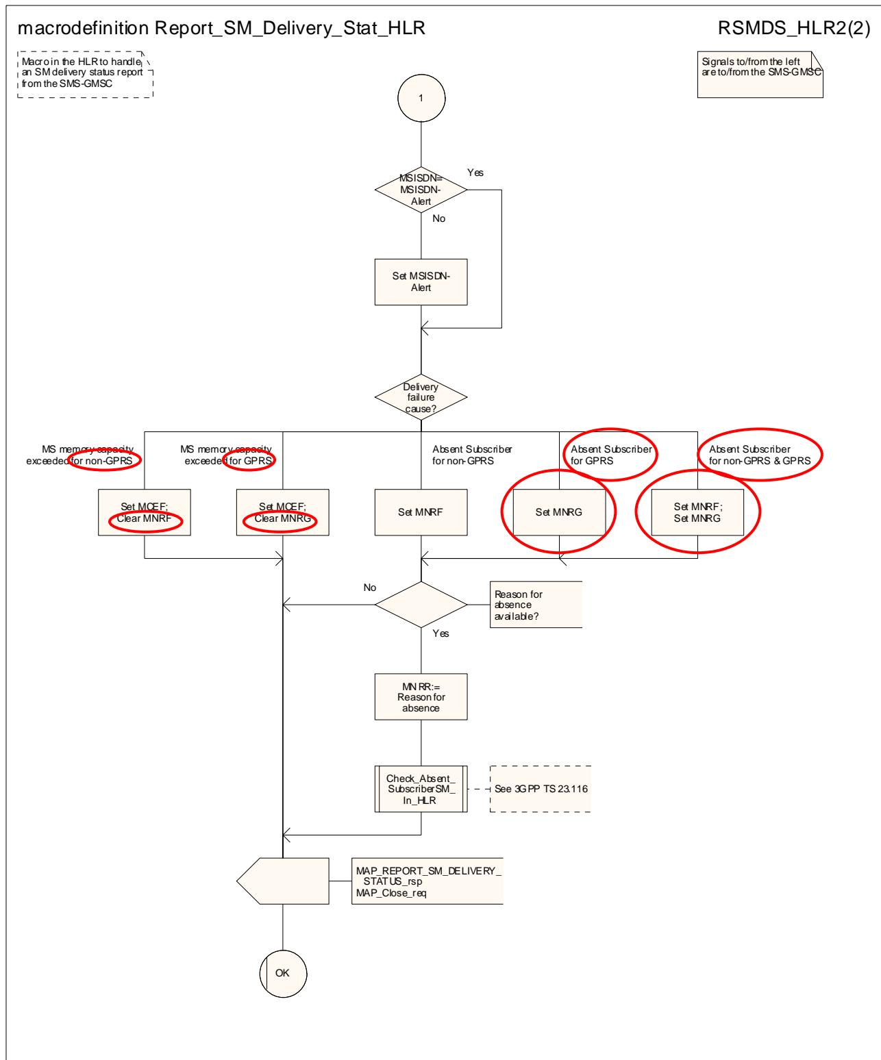
Figure 23.6/1 (sheet 2 of 2): Macro Report\_SM\_Delivery\_Stat\_HLR
