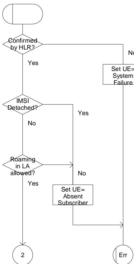
Figure 22.10.3/2 (sheet 1 of 2): Macro Start\_USSD\_VLR
