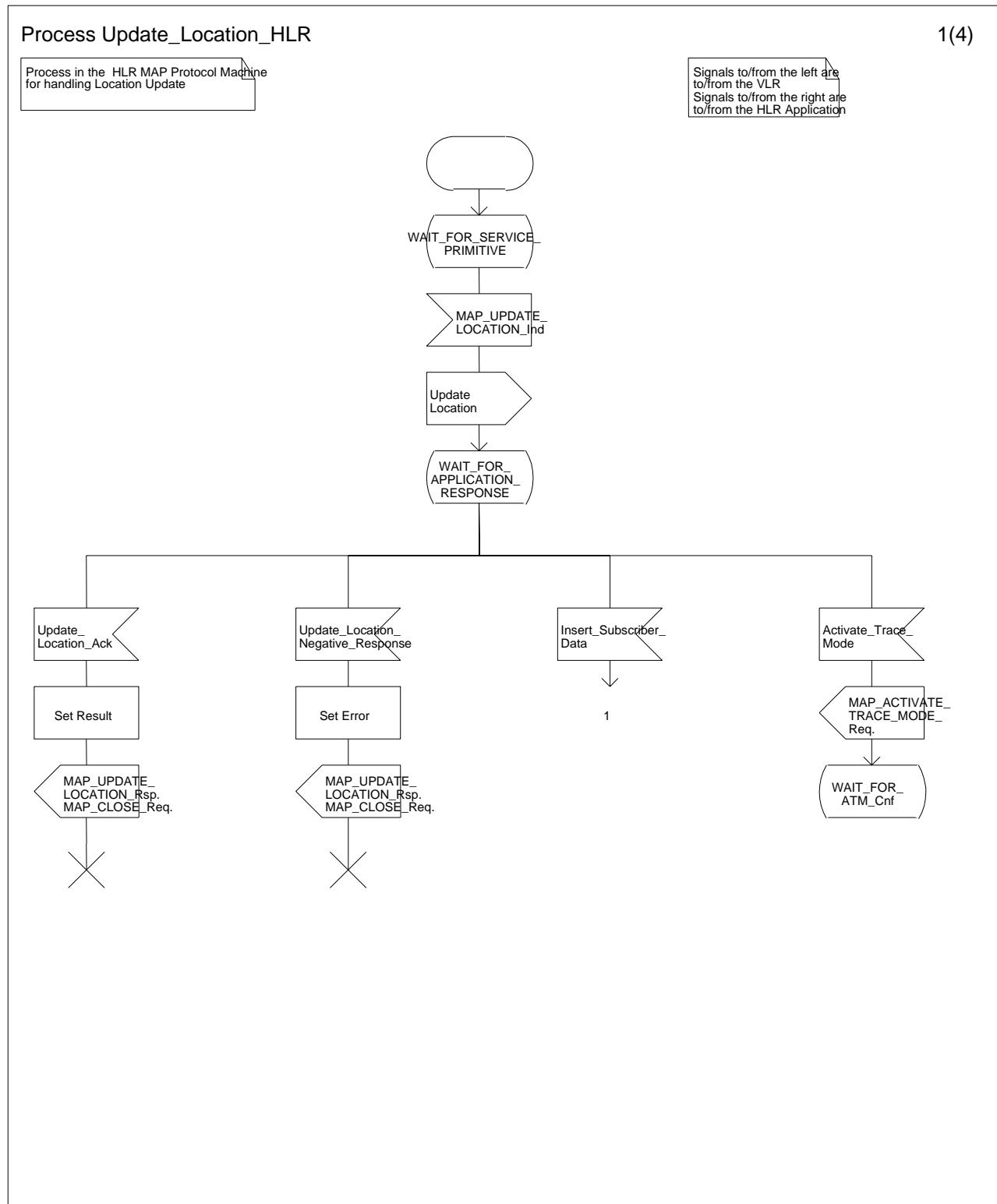
Figure 19.1.1/9 (sheet 1 of 4): Process Update\_Location\_HLR
