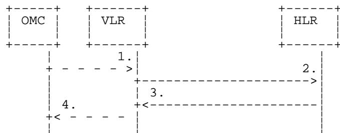
**Figure 20.4/1: The subscriber identity procedure**
