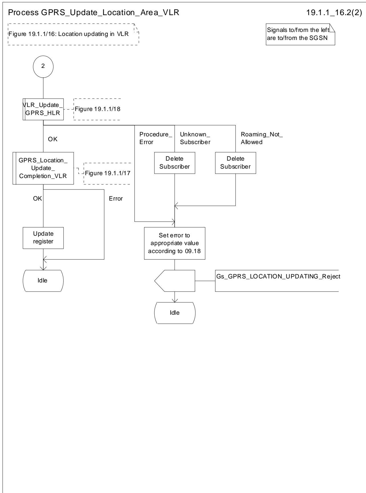
Figure 19.1.1/16 (sheet 2 of 2): Process GPRS\_Update\_Location\_Area\_VLR
