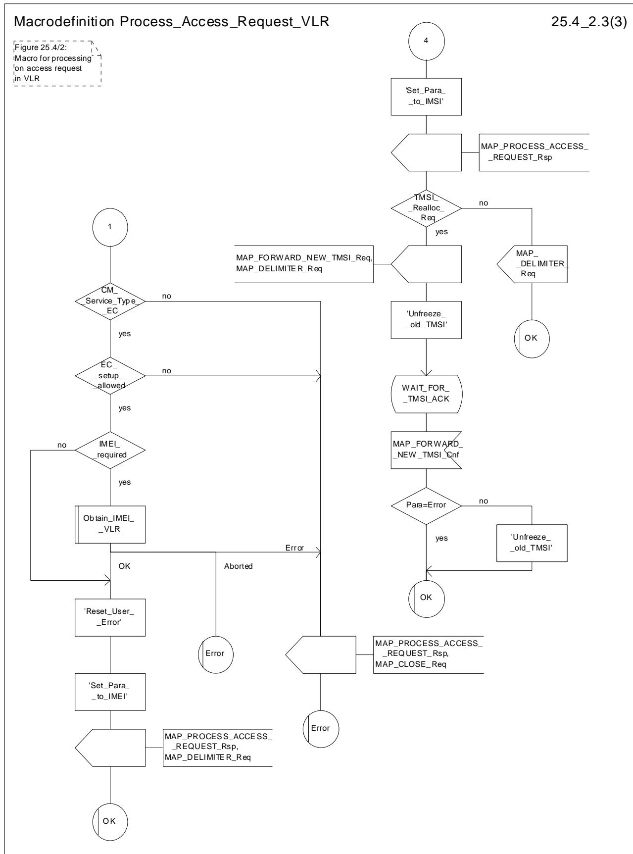
Figure 25.4/2 (sheet 3 of 3): Macro Process\_Access\_Request\_VLR
