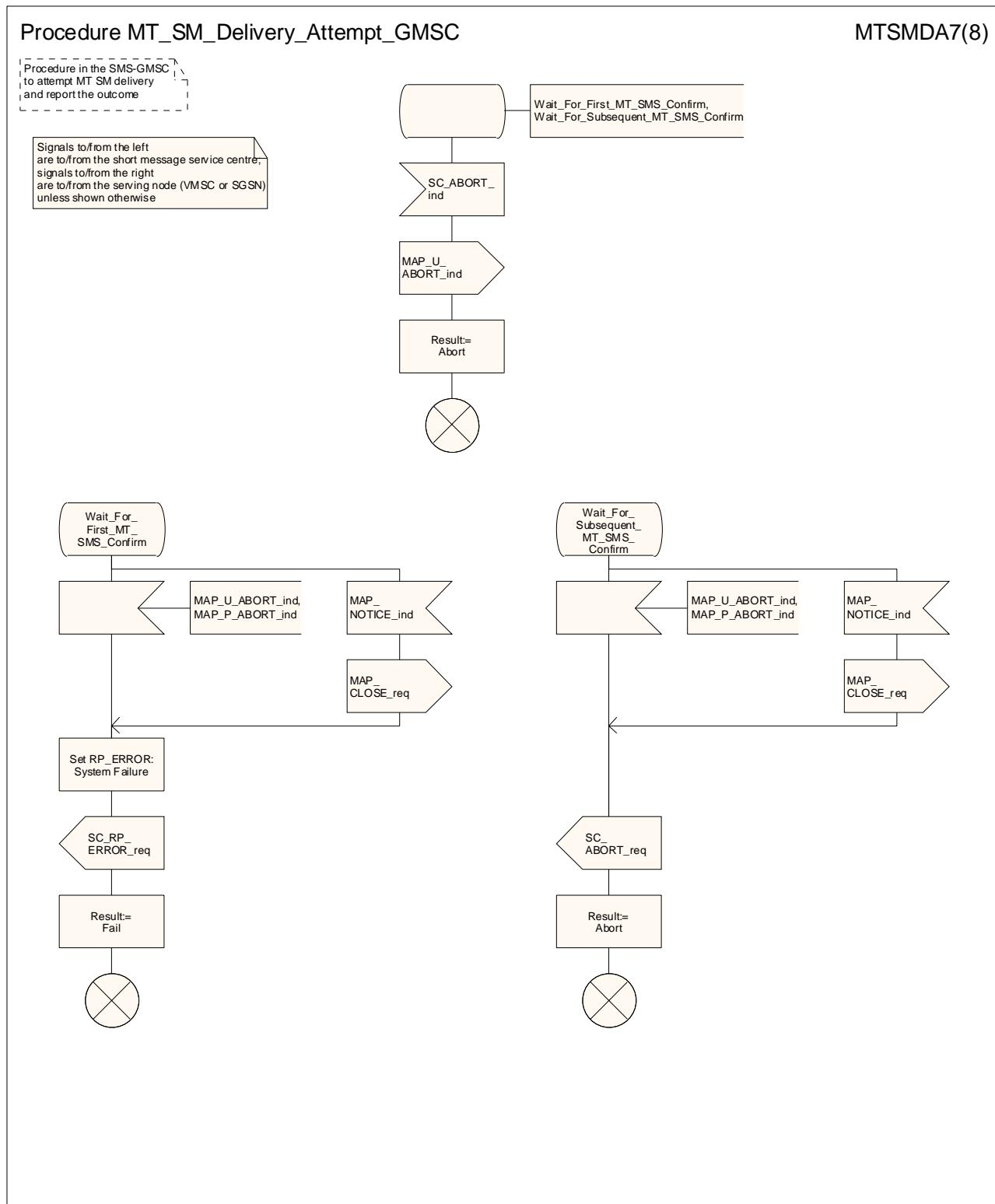
Figure 23.3/4 (sheet 7 of 8): Procedure MT\_SM\_Delivery\_Attempt\_GMSC
