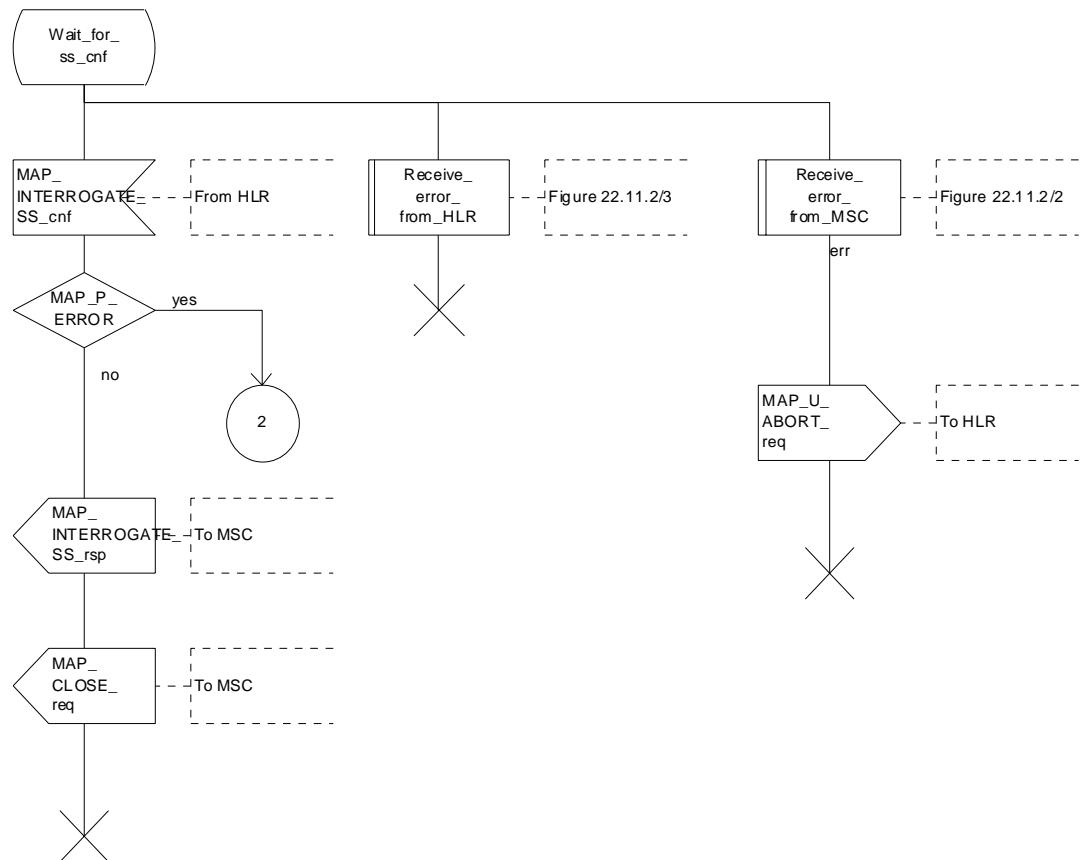
Figure 22.6.3/1 (sheet 3 of 3): Procedure Interrogate\_SS\_VLR
