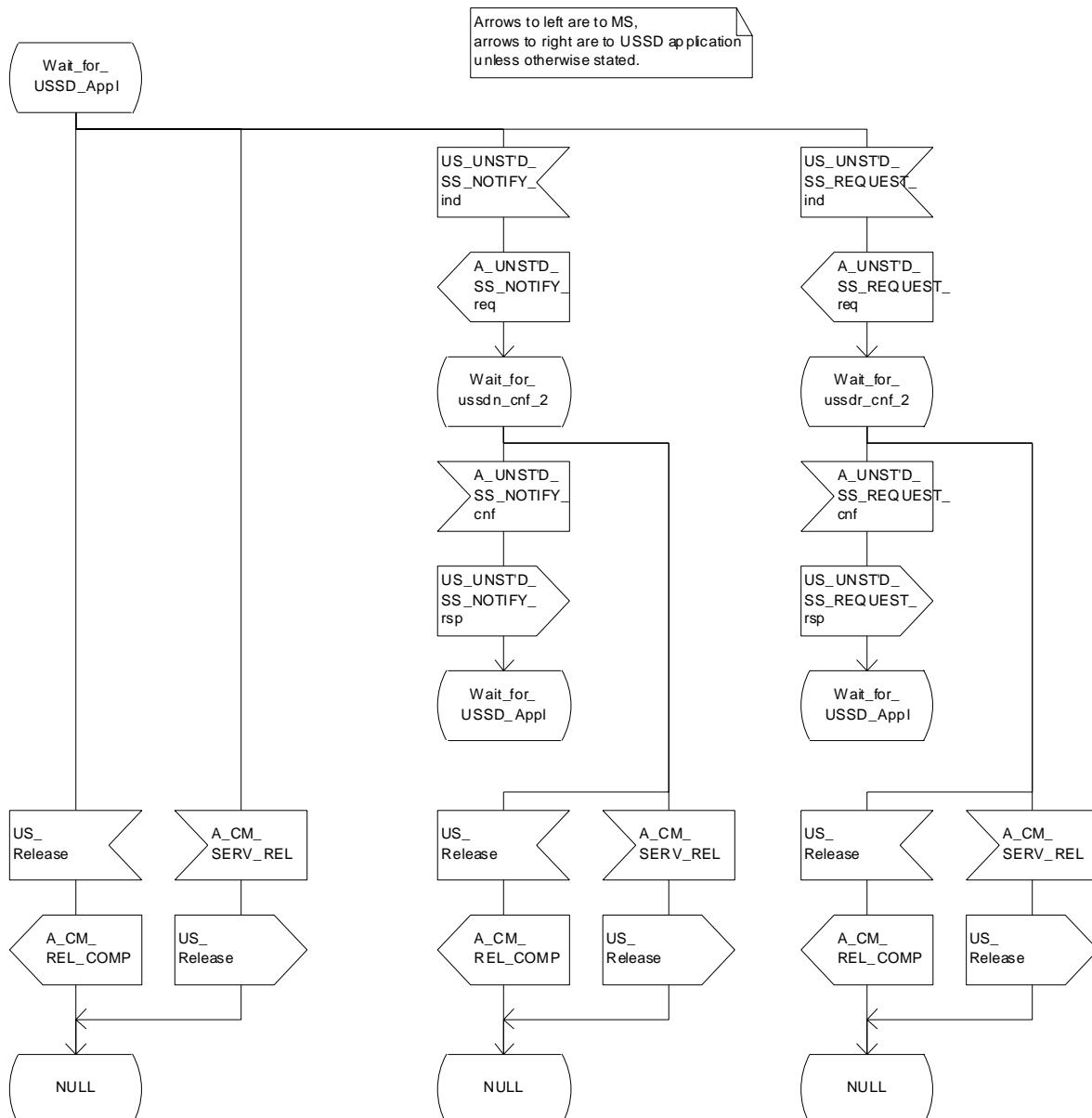
Figure 22.10.2/1 (sheet 4 of 4): Procedure NI USSD MSC
