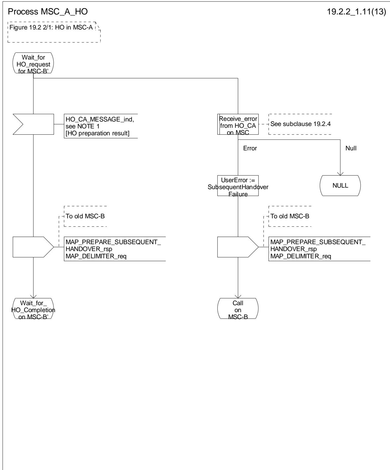
Figure 19.2.2/1 (sheet 11 of 13): Process MSC\_A\_HO
