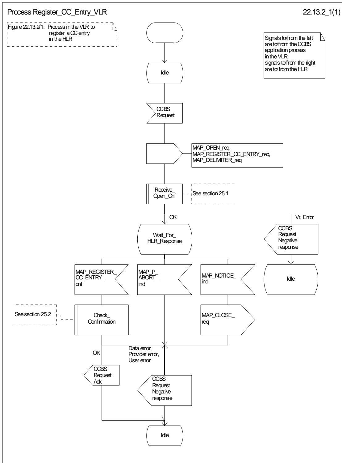
Figure 22.13.2/1: Process Register\_CC\_Entry\_VLR
