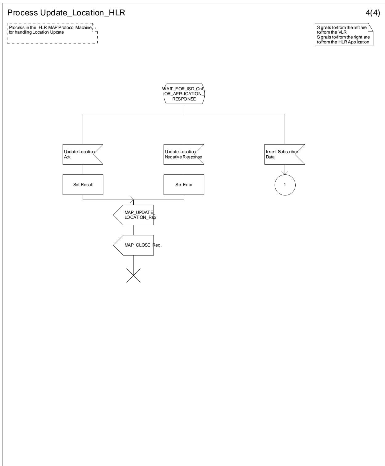
Figure 19.1.1/9 (sheet 4 of 4): Process Update\_Location\_HLR
