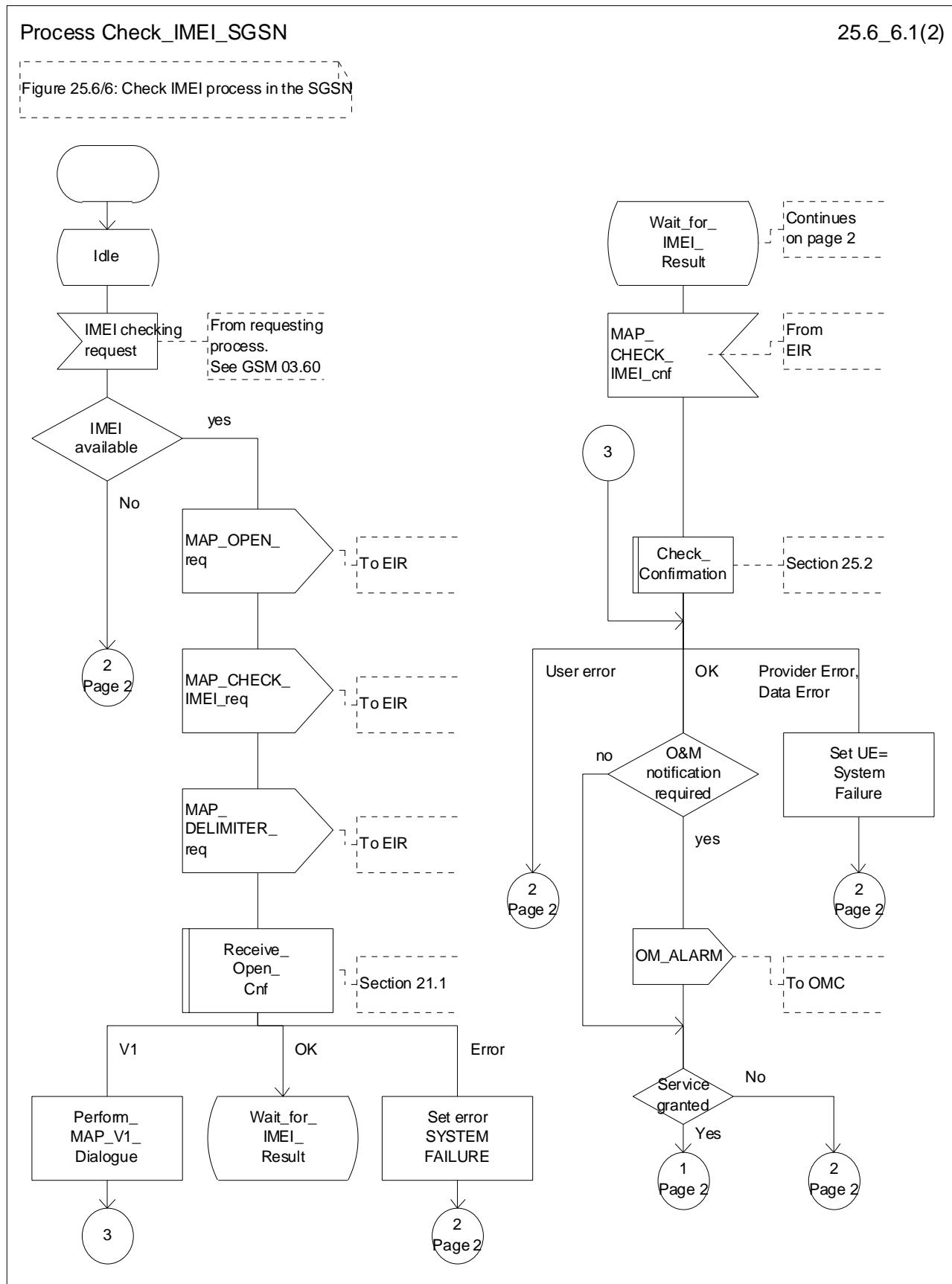
Figure 25.6/6 (sheet 1 of 2): Process Check\_IMEI\_SGSN
