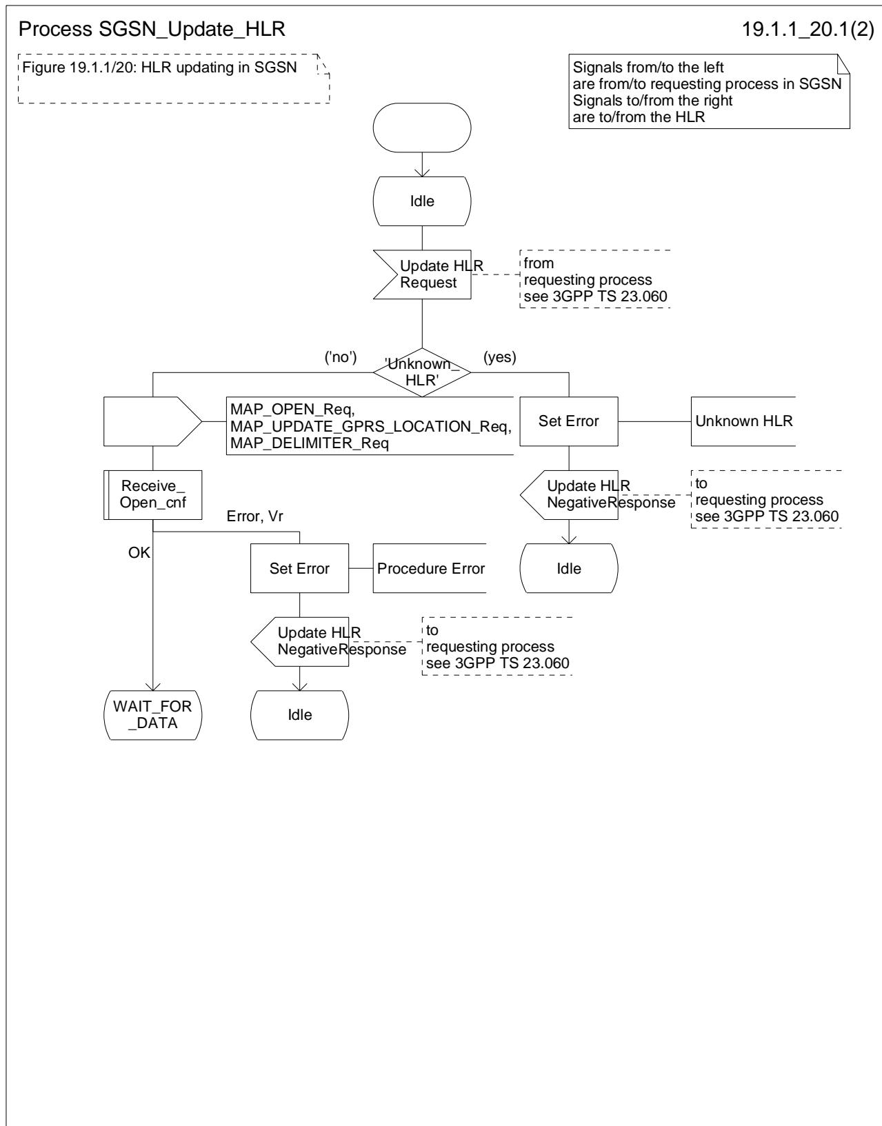
Figure 19.1.1/20 (sheet 1 of 2): Process SGSN\_Update\_HLR
