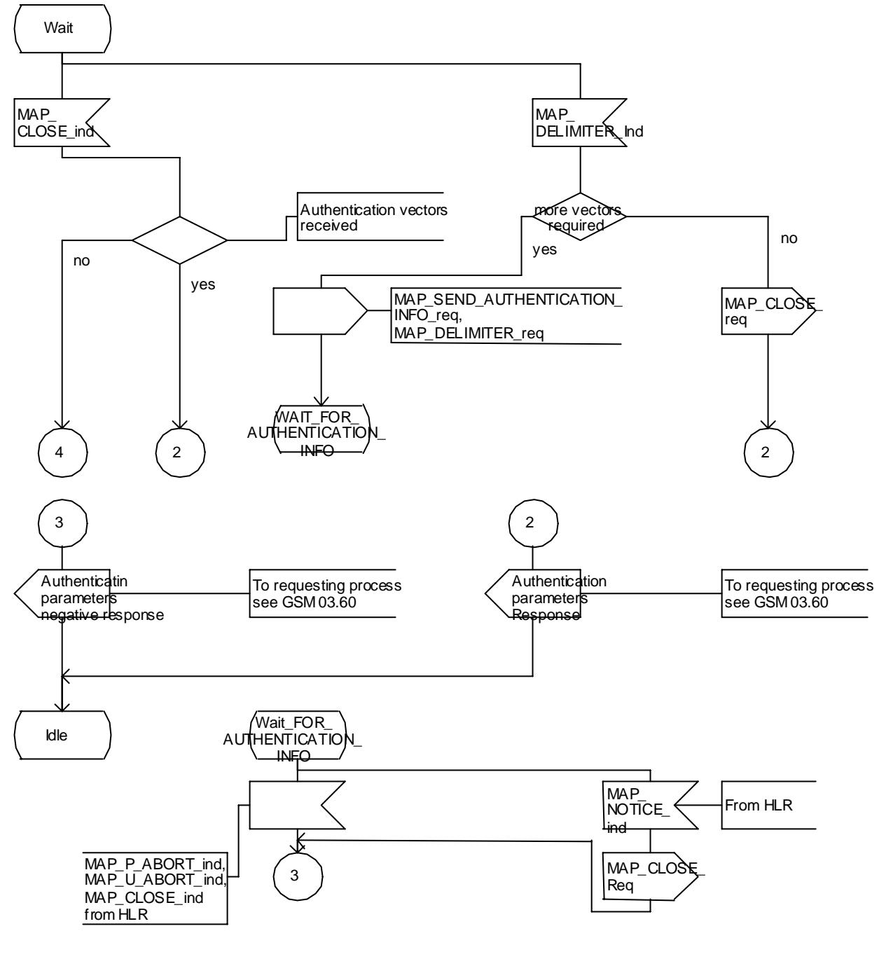
Figure 25.5/6 (sheet 3 of 3): Process Obtain\_Authen\_Para\_SGSN
