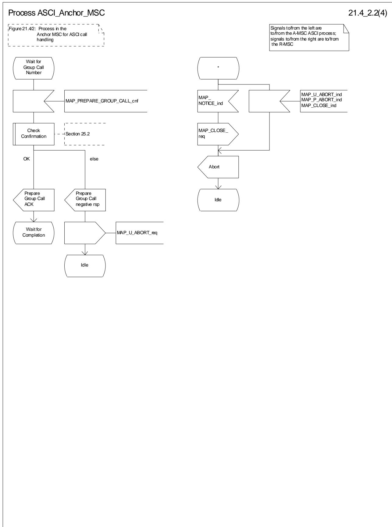
Figure 21.4/2 (sheet 2 of 4): Process ASCI\_Anchor\_MSC
