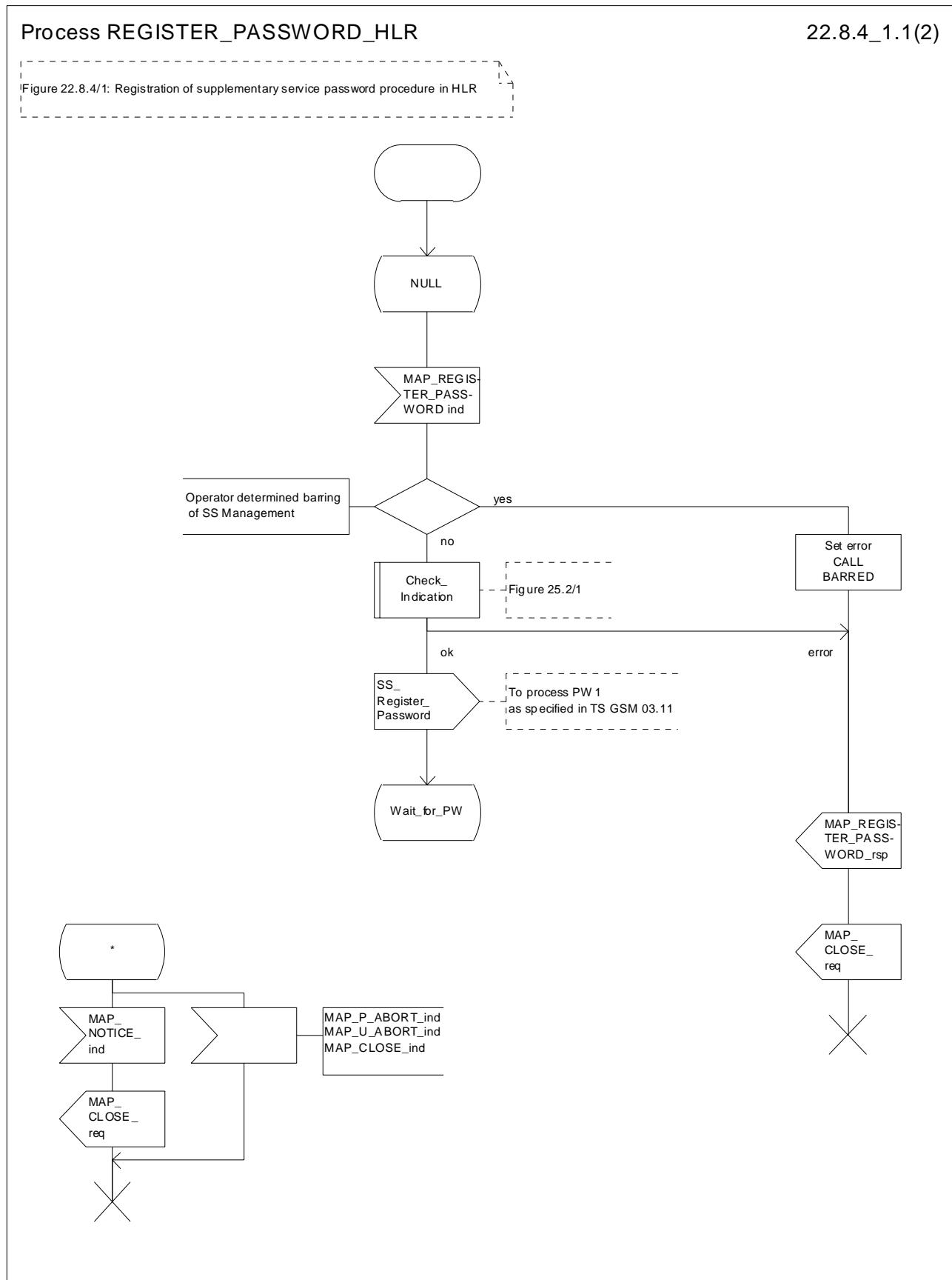
Figure 22.8.4/1 (sheet 1 of 2): Procedure Register\_PW\_HLR
