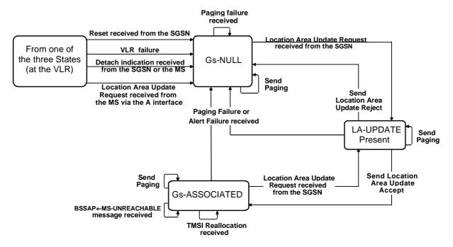
Figure 4.1/3GPP TS 29.018: State diagram at the VLR
