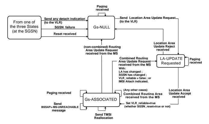
Figure 4.2/3GPP TS 29.018: State diagram at the SGSN
