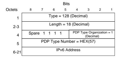
Figure 37: End User Address Information Element for IPv6
