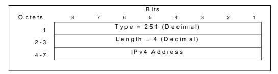
Figure 59a: Ipv4 Charging Gateway Address Information Element
