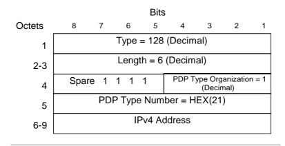
Figure 36: End User Address Information Element for IPv4
