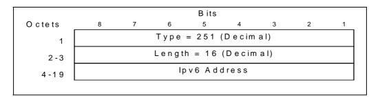
Figure 59b: Ipv6 Charging Gateway Address Information Element
