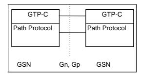
Figure 63: Signalling Plane - Protocol Stack
