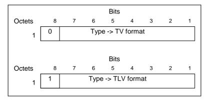
Figure 8: Type field for TV and TLV format
