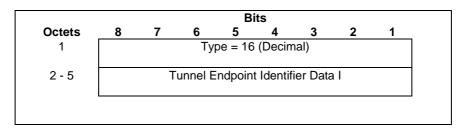
Figure 21: Tunnel Endpoint Identifier Data I Information Element
