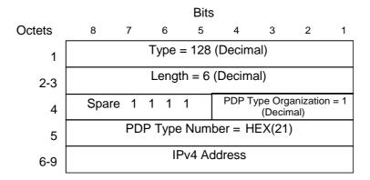
Figure 36: End User Address Information Element for IPv4
