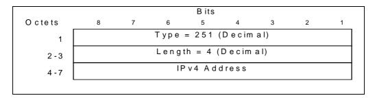
Figure 59a: Ipv4 Charging Gateway Address Information Element
