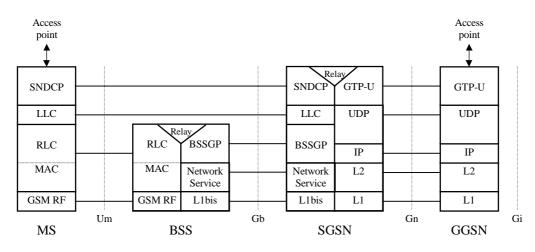
Figure 2a: User Plane for Packet Domain services in GSM
