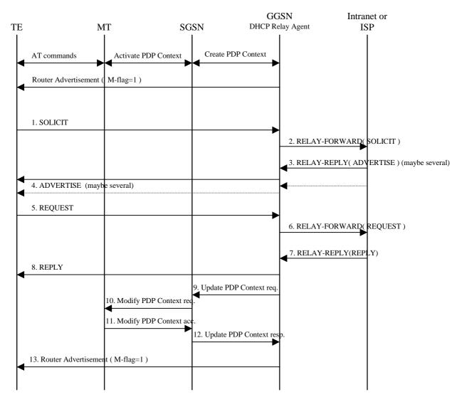
Figure 16e: DHCPv6 signal flow
