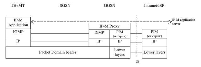
Figure 12: Protocol configuration for IP-Multicast handling (control plane)
