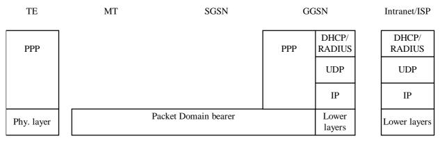
Figure 14: Protocol stack for direct access to IP-based Intranets/ISPs
