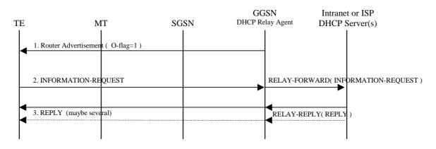
Figure 16f: DHCPv6 Other configuration signal flow
