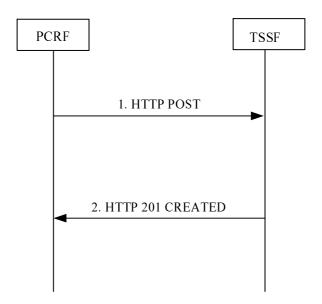
Figure A.2.1: Traffic Steering Control Information Provisioning
