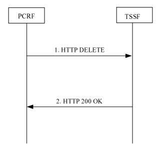
Figure A.4.1: Traffic Steering Control Information Removal
