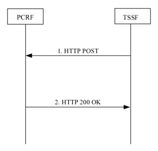
Figure A.5.1: Traffic Steering Control Notification
