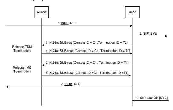
Figure 43: Session release from CS network side for ISUP (message sequence chart)
