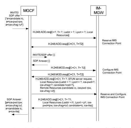
Figure 9.2.12.4.1.1: Procedure for interactive connectivity establishment using ICE lite towards the offerer
