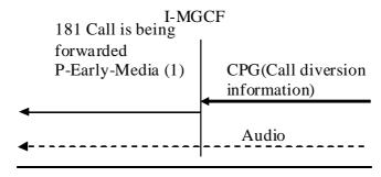
NOTE 1: Whether the P-Early-Media header field is included if the received INVITE contains a P-Early-Media header field with the "supported" parameter as described in IETF RFC 5009 [89] or based on local policy.
