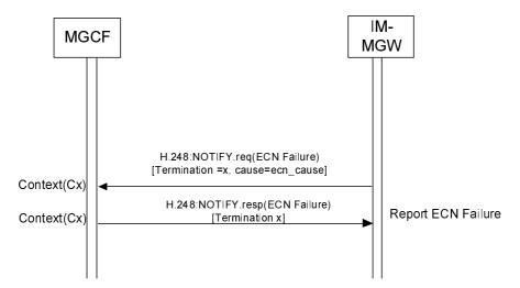
Figure 9.2.11.2.2: Procedure to Report ECN Failure
