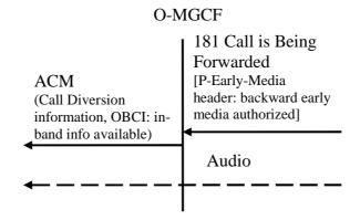
Figure 16c: Sending of ACM (Receipt of first 181 Call is Being Forwarded that includes authorization of early media)
