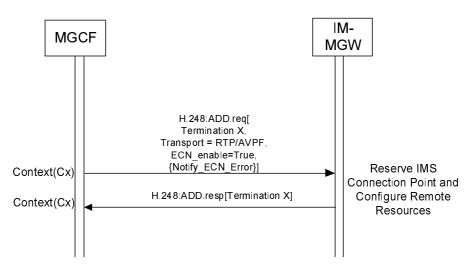
Figure 9.2.11.2.1: Procedure to Request ECN
