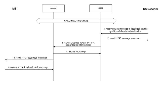
Figure E.4.2.8.3.2.1: Interactions between H.245 and RTCP for CS network originated H.245 feedback on the quality of the media distribution
