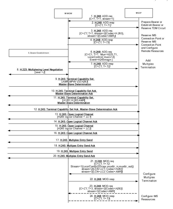
NOTE 1: All H.245 messages (from Signal 9 to Signal 18) are transported through the IM-MGW between the MGCF and the CS side, using the procedures described in clause E.4.2.3
