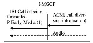
NOTE 1: Whether the P-Early-Media header field is included depends on whether the received INVITE contains a P-Early-Media header field with the "supported" parameter as described in IETF RFC 5009 [89] or based on local policy.
