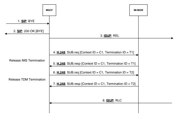
Figure 41: Session release from IM CN subsystem side for ISUP (message sequence chart)
