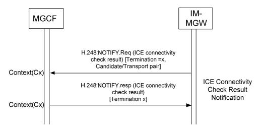
Figure 9.2.12.4.3.1: Procedure to report ICE connectivity check result
