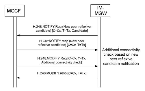
Figure 9.2.12.4.4.1: Procedure to perform additional connectivity check upon the report of new peer reflexive candidate
