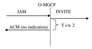
Figure 17: Sending of ACM (Ti/w2 elapses)
