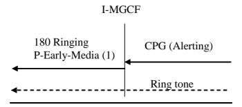
NOTE: Whether the P-Early-Media header field is included depends on whether the received INVITE contains a P-Early-Media header field with the "supported" parameter as described in IETF RFC 5009 [89] or based on local policy.
