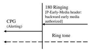
Figure 18a: Sending of CPG(Alerting) (Receipt of 180 Ringing response with authorization of early media)
