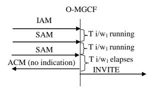
Figure 15: Sending of ACM T i/w1 elapses
